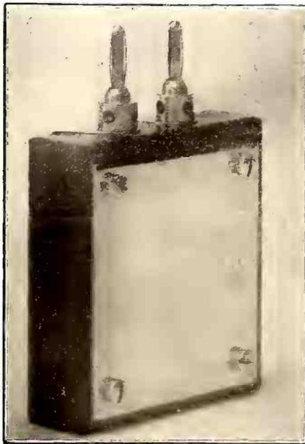
Quartz plate holder for piezo oscillator assembled
