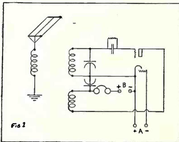
Fig. 1. Wiring diagram of short wave receiver used by Arthur A. Collins for receiving messages and broadcasts from WNP, the *Bowdoin* of the MacMillan Arctic expedition. The two stage amplifier when used is added in the usual fashion. The circuit is the conventional regenerative patterned after Armstrong.
