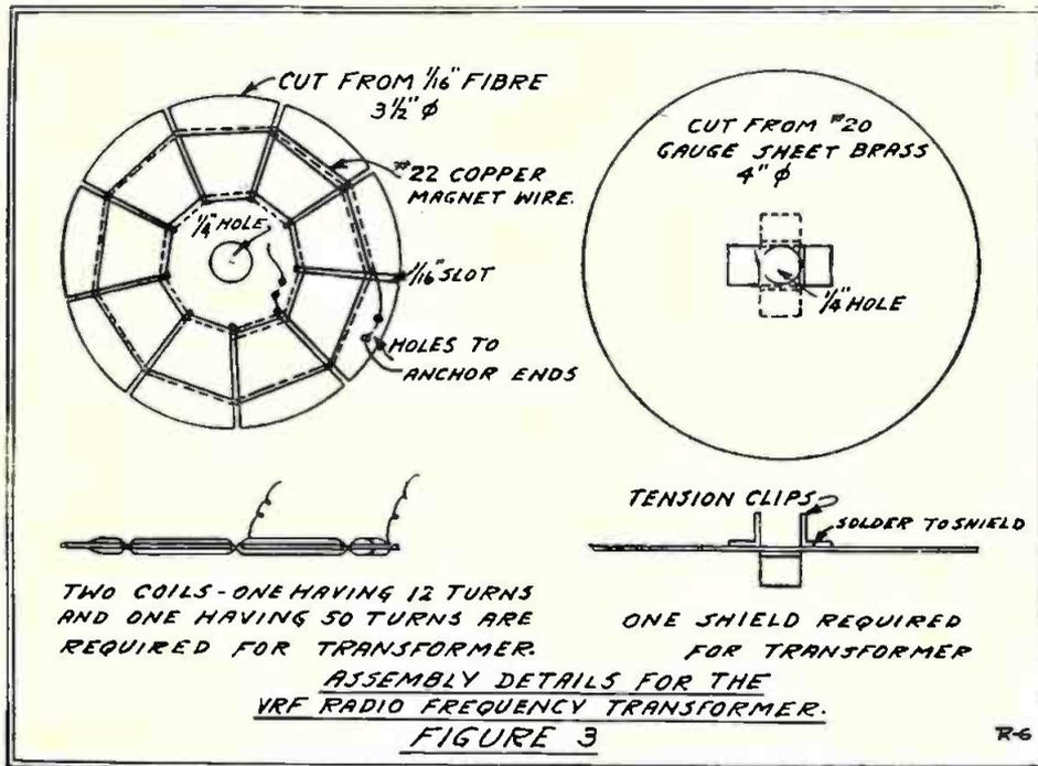
radio frequency transformer (VRF) is shown in figures 2 and 3, together with the assembly of the completed unit.
