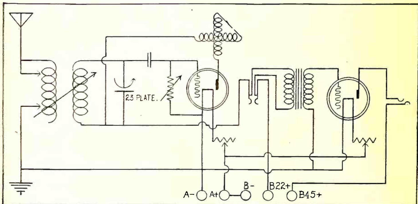
Circuit contributed by Mr. Frederiksen. It is a modified form of the Ultra-Audion. This circuit possesses all of the desirable qualities of the "single" plus the selectivity of the three circuit tuner.
