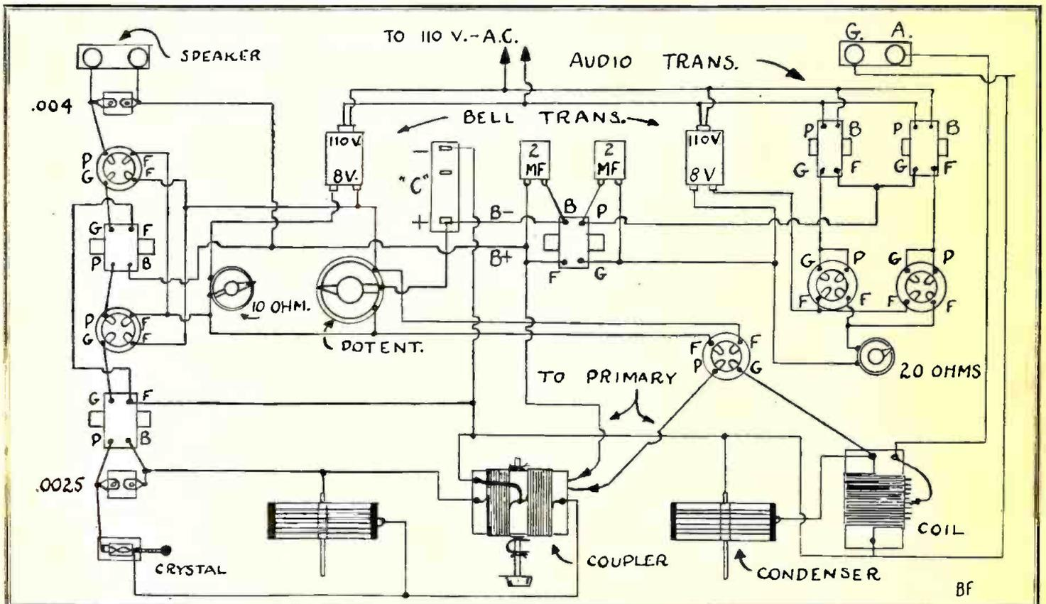
Complete wiring for a receiver operated on the A. C. house current. The only battery used is a 1-2 volt "C" battery—this being included in the set. There are five tubes in all; it's a three tube and crystal detector set, the extra two tubes furnishing the rectified current for the "B" voltage.
