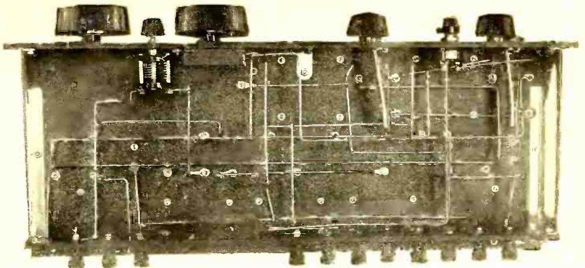
A bottom view of the super-heterodyne receiver, showing the wiring arrangement before the parts are installed. After studying this diagram and the others in this article, the fan should have no trouble in placing the parts. Every part is clearly marked by a number in the diagrams on the opposite page.
