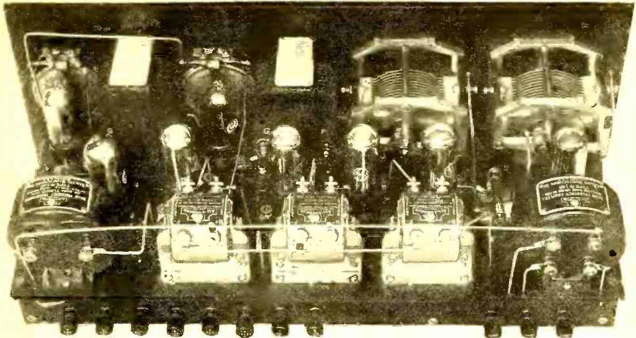
An unusual photo showing a rear panel view of Mr. Calcattera's 8-tube super-heterodyne. Note the compact arrangement, which, though utilizing every inch of space, is not crowded.
