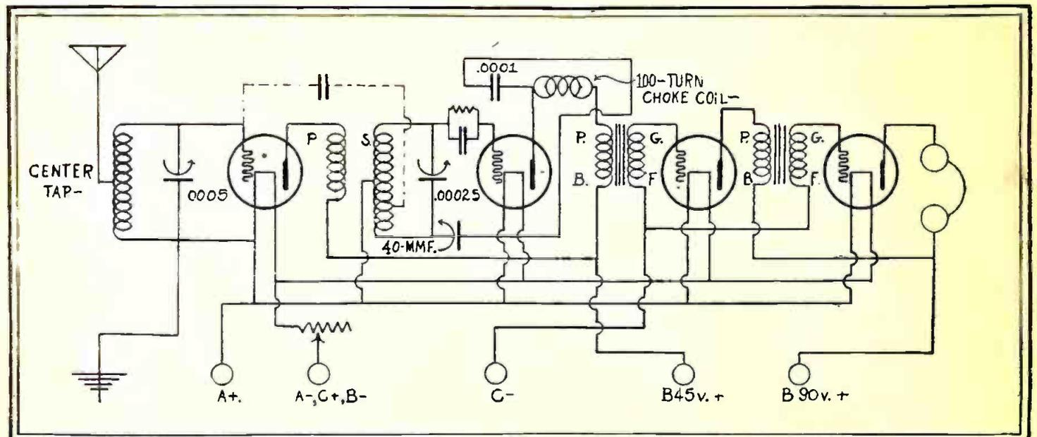
The wiring layout of Mr. McCullah's four tube receiver. Regeneration is obtained with a small variable condenser. In the diagram above it will be noticed that there is a small fixed condenser in series with the regenerative condenser, for the reason the so-called regenerative condenser has too high a zero capacity to prevent the detector tube from oscillating at the lower end of the scale
