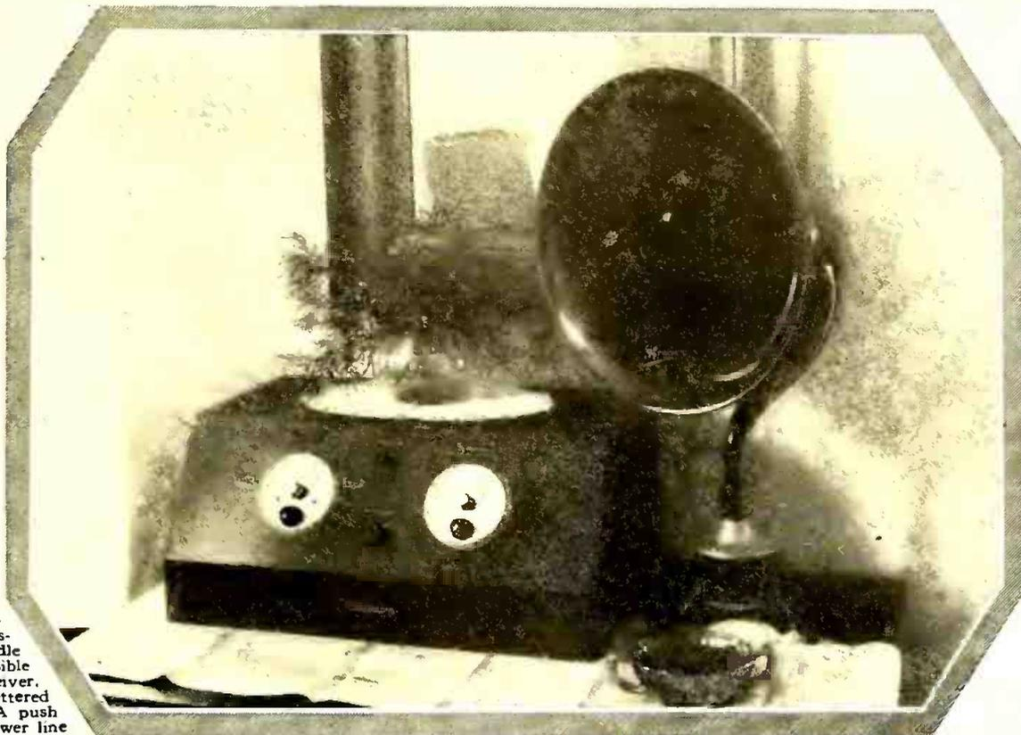
Does the appearance please you? "Two hand" tuning control, with vernier dials, an R. F. coupling adjustment for sensitivity and the crystal control-handle form the only visible parts of the receiver. Station calls are lettered on the dials. A push switch in the power line turns the set on and off.
