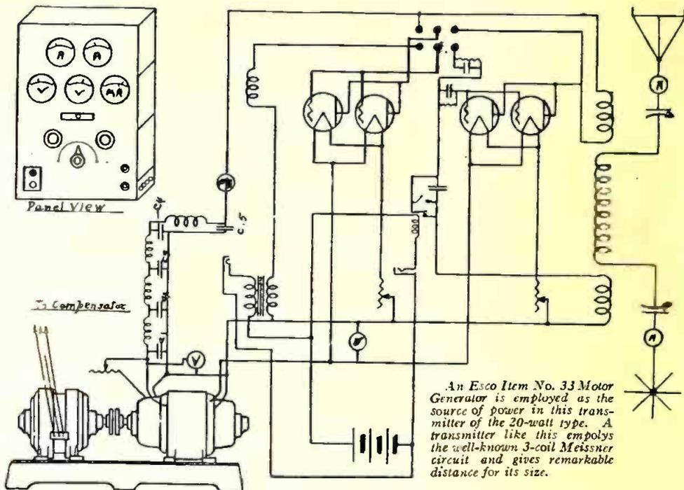
An Esco Item No. 33 Motor Generator is employed as the source of power in this transmitter of the 20-watt type. A transmitter like this employs the well-known 3-coil Meissner circuit and gives remarkable distance for its size.
