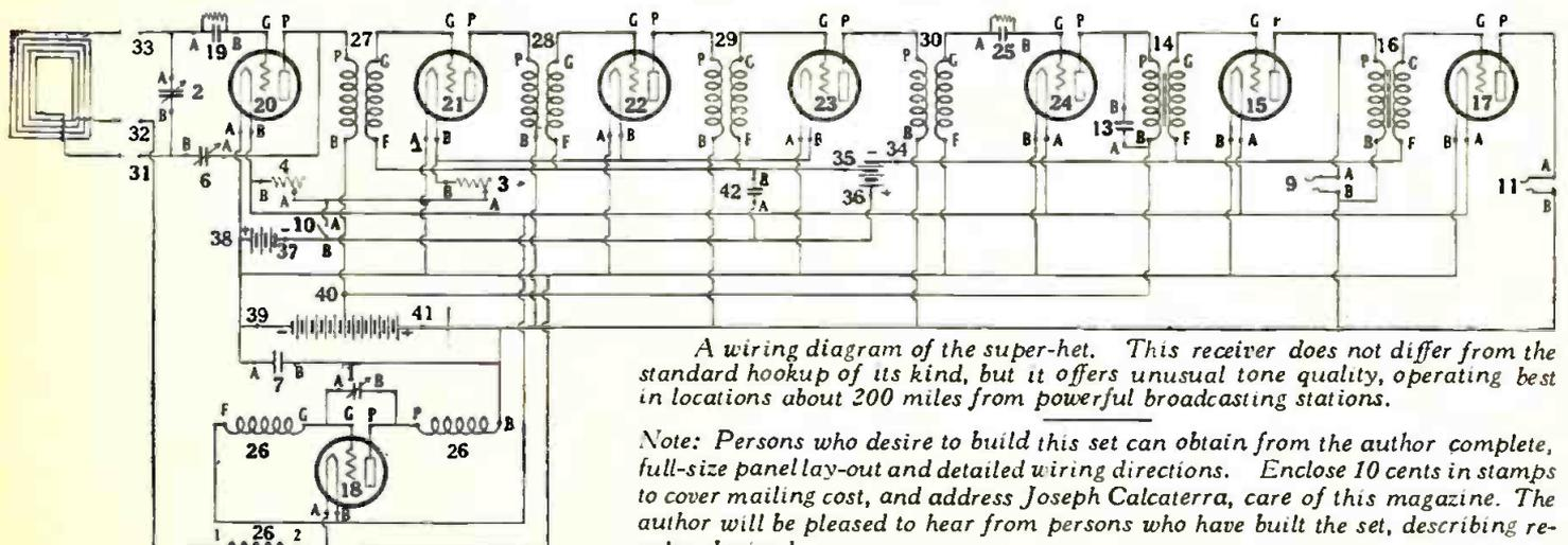
A wiring diagram of the super-het. This receiver does not differ from the standard hookup of its kind, but it offers unusual tone quality, operating best in locations about 200 miles from powerful broadcasting stations.
