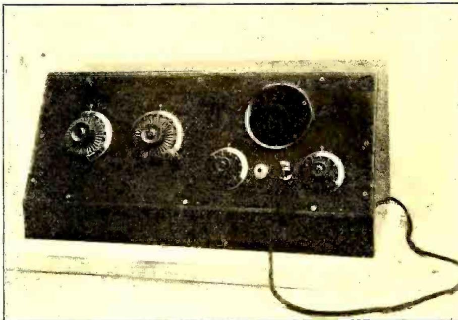
*If you like a sloping model of cabinet, here's one that is particularly handsome. The three circuit tuner is used for reception, with a two stage amplifier, and the outfit has a self-contained loud speaker. Make yourself one!*
