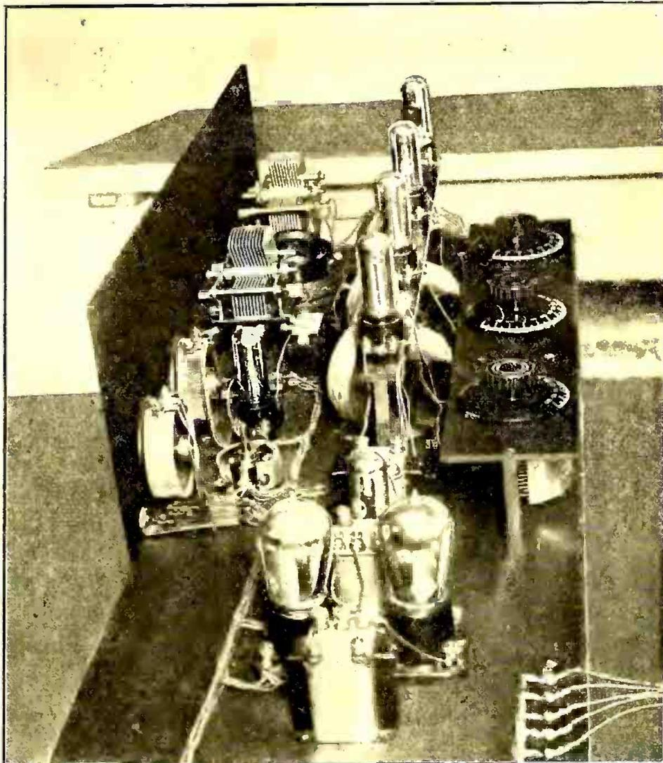
*A side view of the super-heterodyne, showing the method of installing the 201A tubes in the push-pull audio amplifier.*
