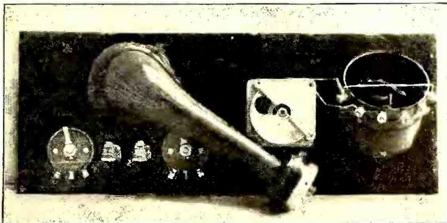
*The parts mounted to the panel are few and their arrangement is neat. The loud speaker horn is a novel feature, being included in the cabinet. Any high quality type of three circuit coupler will answer the purpose.*
