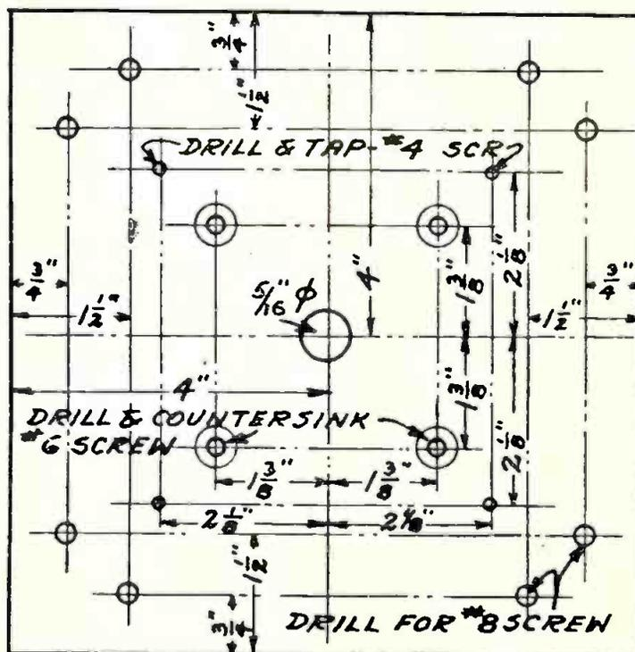
Fig. 2A—Showing the drillings in the 8"x8"x3-16" panel.
