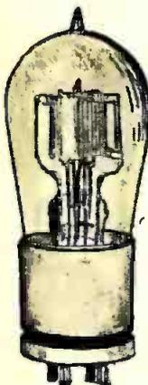
Test No. 30. **FEDERAL TYPE 201-A VACUUM TUBE.** This tube was submitted for test by the Service Lamp Co., 112-114 Trinity Place, New York City, N. Y. Due to the efficient manner in which the tube is packed, it arrived in good condition. Although no tests were made to determine the life of the tube, it gave very good results.
