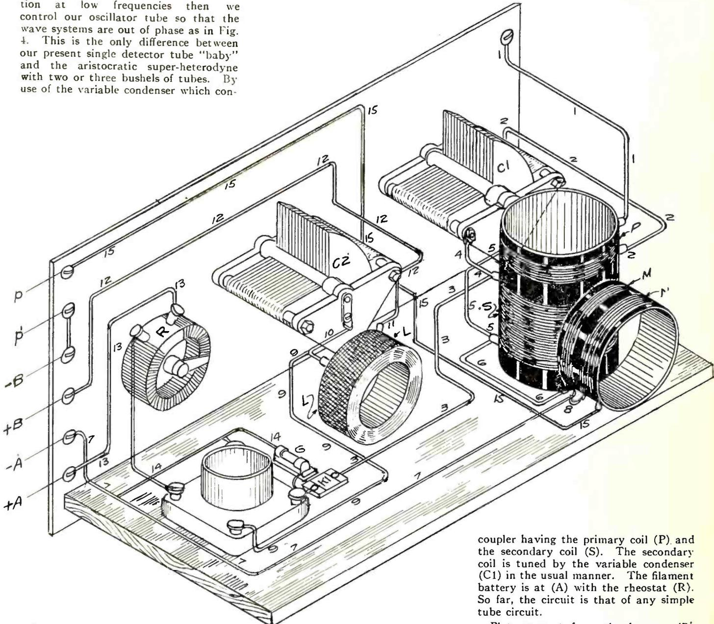
coupler having the primary coil (P) and the secondary coil (S). The secondary coil is tuned by the variable condenser (C1) in the usual manner. The filament battery is at (A) with the rheostat (R). So far, the circuit is that of any simple tube circuit.
