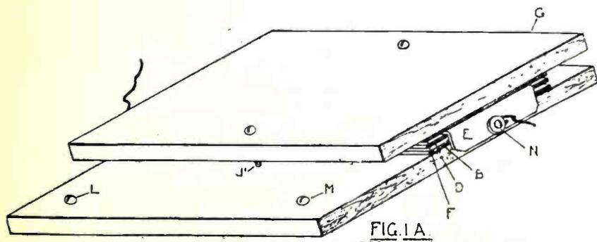
The wooden blocks are of dry wood smoothed up with sandpaper and given a coat or two of varnish which will not absorb moisture, or treated with paraffin as described in Circular No. 120.
