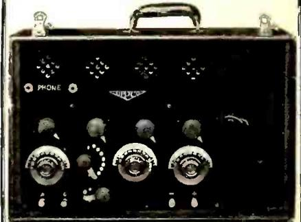
The set herewith illustrated is a four tube Radio-frequency set built into a light-weight, portable case with nickel-plated hardware, making a handsome, simple and salable set. Prices on sets range from \$65.00 to \$190.00, including tubes, B Batteries and head phone. These sets can be taken wherever you go, being light and convenient to carry.
