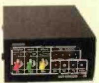
Packet, AMTOR, CW SSV, Fax, RTTY NAVTEX, SYNOP PC Software included. Connect between Transceiver and PC and feed with 12V DC. Includes receiver audio filtering and tuning indicator.
