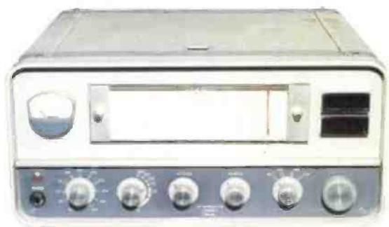
The KW Electronics KW201 double conversion receiver, the indicators on the top right show either upper sideband (u.s.b.) or lower sideband (l.s.b.) is selected. The main tuning knob is on the lower right.
