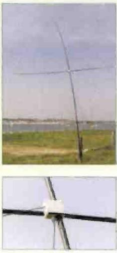
The loop antennas, Syon tells *PW*, are very effective DX antennas due, they say, to their low radiation angle which is achieved at relatively low heights. Syon also says that this antenna offers good signal levels on all bands (7-28MHz).
