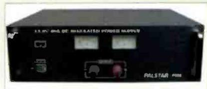
Firstly, you could get a closer look at the Palstar PS50 p.s.u. which, according to Nevada, delivers 40A continuous output (50A peak) with high stability. It features both short circuit and overload protection and has a thermostatically controlled fan cooling system.
