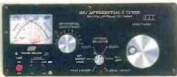
MFJ-986 is the ideal ATU for use with linear amplifiers. Covering 1.8 - 30MHz it is rated at 3kW and features a roller coaster coil plus PEP watt meter and will handle coax cable, balanced feeder and long wire.
