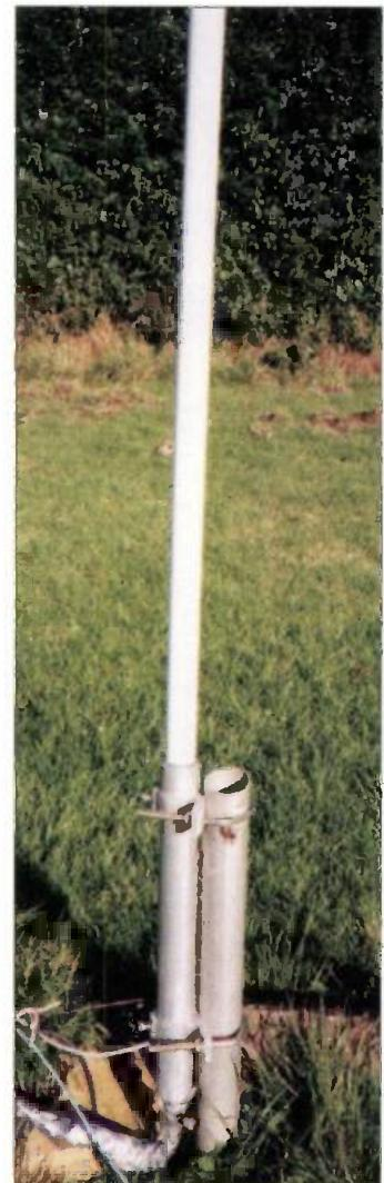
Fig. 1: Close-up view of the antenna's base and feed-point, suitably waterproofed.
