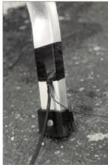
Fig. 6: Connections to the vertical antenna. The wire radial is connected to the outer of the coaxial cable and must be insulated from the antenna.
