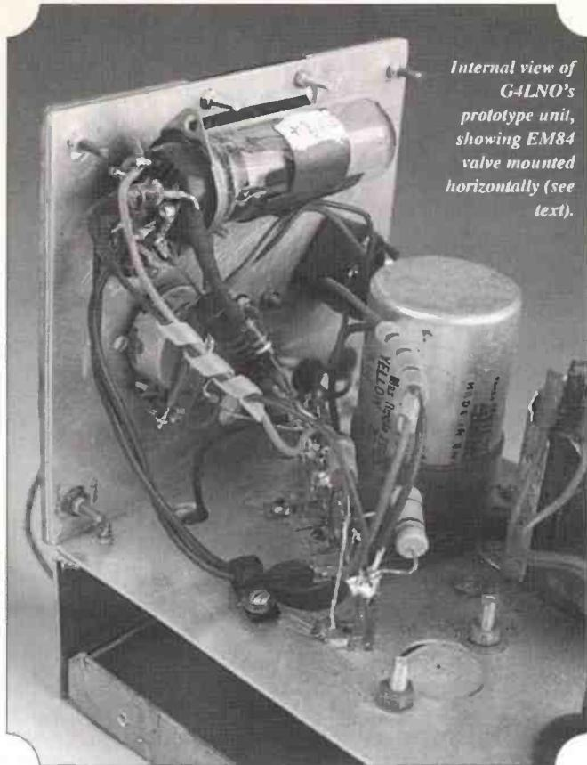
*Internal view of G4LNO's prototype unit, showing EM84 valve mounted horizontally (see text).*
