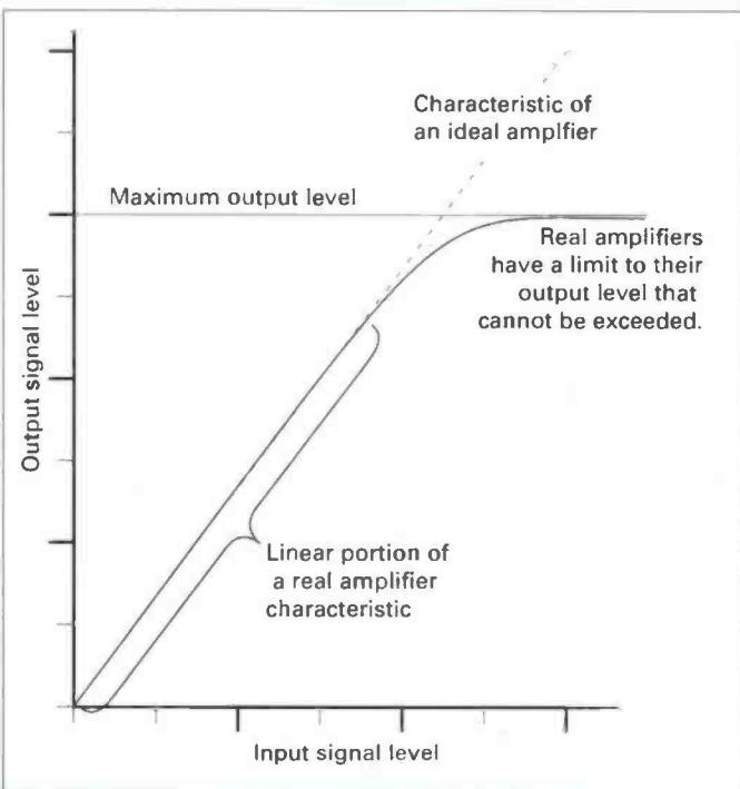
Fig. 1: Characteristic of an r.f. amplifier.
