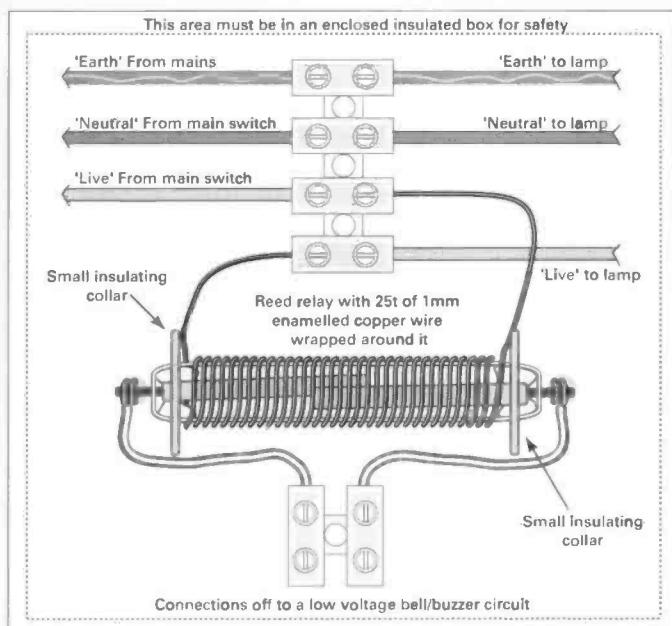
comes on there is an immediate current of about 20A flowing. This current settles down to about 1-2A after a very short time. So a safe and sure current sensing relay was needed.
