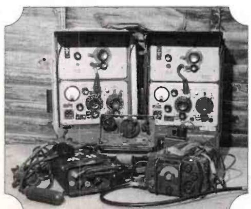
*Other sets available for the collector include the WS18 (rear), WS38 MkII (centre), WS38 MkIII (front right) and the WS88 (front left). All are relatively small and lightweight, and all but the 88 set use large octal valves. The 88 set uses 15 miniature valves.*
