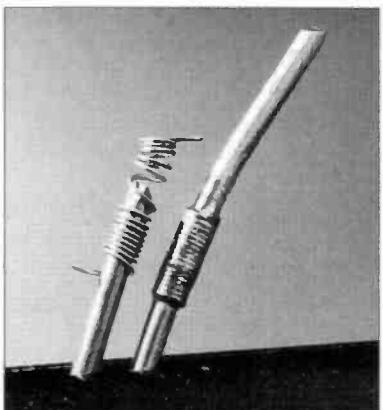
You should now have a length of insulation without any strands of copper wire through the middle.
