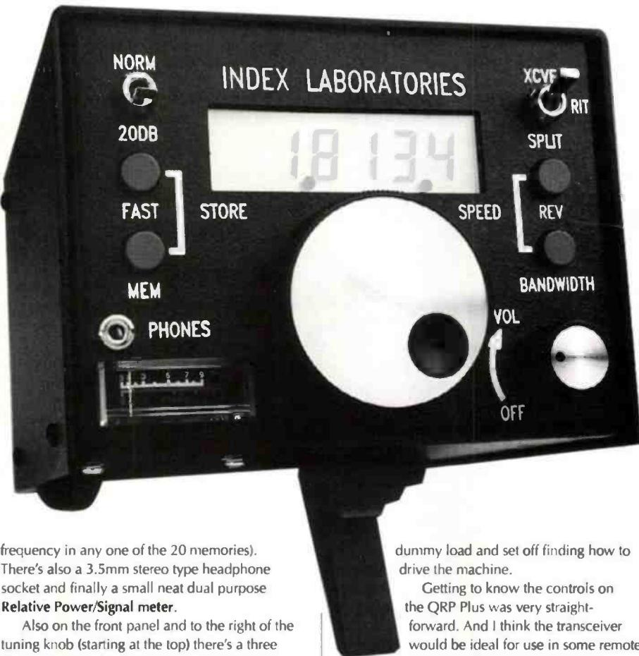
frequency in any one of the 20 memories). There's also a 3.5mm stereo type headphone socket and finally a small neat dual purpose **Relative Power/Signal meter**.
