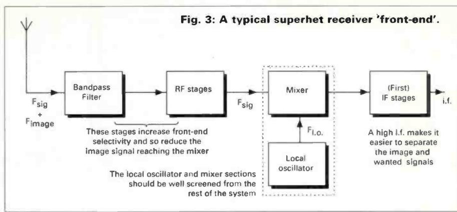
double superhet has two i.f.s. Selectivity (that is the ability of the circuit to respond to the frequency we want and reject all others) is provided by the second i.f. which is low compared with the first. In fact, a high first i.f. has two advantages: it minimises the risk of second channel interference; and the designer can, more easily, provide continuous coverage over a wide frequency range.
