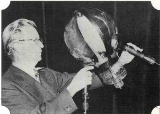
*Although Baird demonstrated the two-beam 'Telechrome' colour TV tube (on left), he suggested a suitable arrangement for three colours (centre). Unfortunately his death at the early age of 58 in 1946 robbed television engineering of one of the greatest pioneers.*
