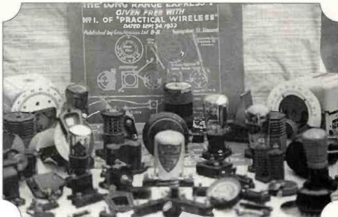
**Fig. 1:** A typical selection of valves and components available when Ron Ham built his first 'one valver' receiver in 1939 (from the Amberley Chalk Pits Vintage Wireless collection).
