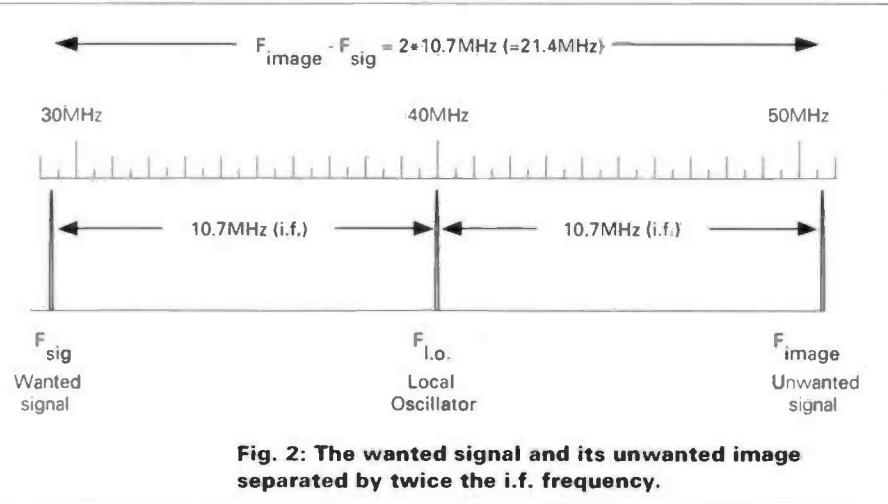
Fig. 2: The wanted signal and its unwanted image separated by twice the i.f. frequency.
