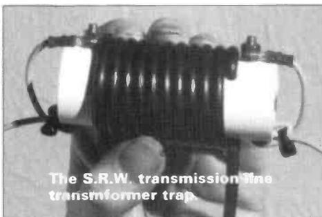
The S.R.W. transmission line transformer trap
