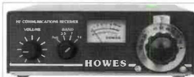
receiver designed to cover the 3.5, 7 & 14MHz bands as standard. There is a provision for a plug-in 'band module' so that additional short wave bands can be added.
