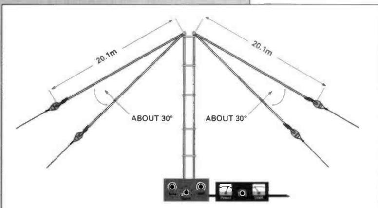
**Fig. 4: This is the form of the Skelton Cone antenna (see text for more details).**
