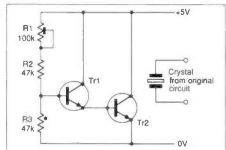
Fig. 1: Circuit of the crystal 'oven' unit for the PW Robin frequency counter, as built by the original designer Mike Rowe G8JVE.
