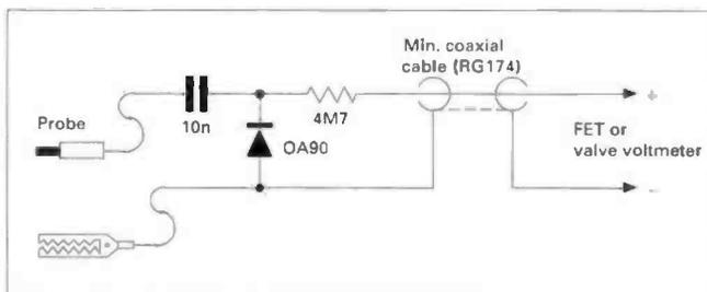
Fig. 1: Circuit of the simple r.f. probe described by G4RAW.
