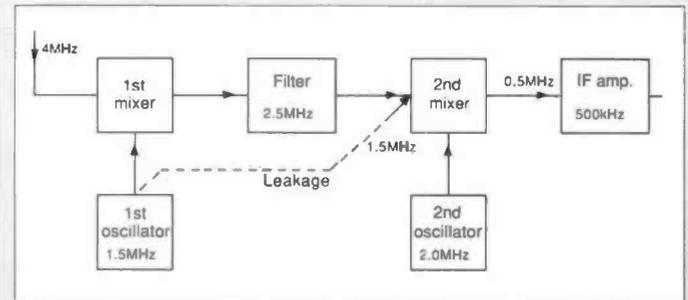
Fig. 1: A simple example of spurious signal generation in a receiver.
