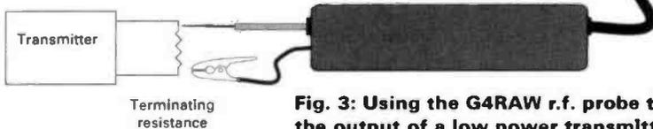
Fig. 3: Using the G4RAW r.f. probe to measure the output of a low power transmitter (see text).
