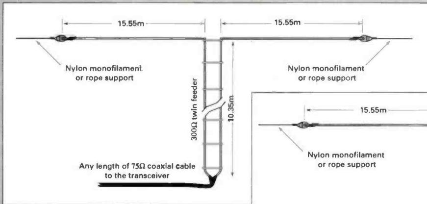
**Fig. 2: The G5RV antenna in its traditional guise.**
