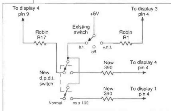
**Fig. 4: Modified decimal point switching.**
