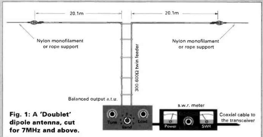
**Fig. 1: A 'Doublet' dipole antenna, cut for 7MHz and above.**
