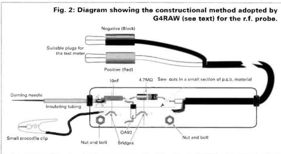
Fig. 2: Diagram showing the constructional method adopted by G4RAW (see text) for the r.f. probe.
