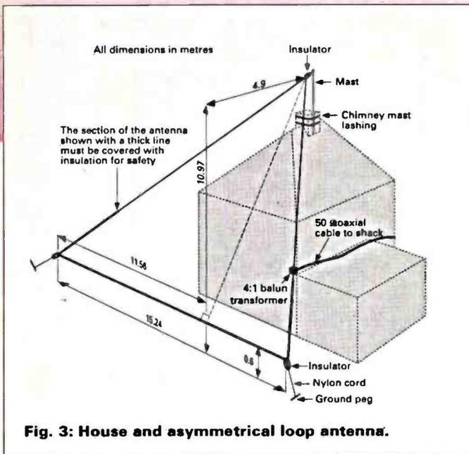
**Fig. 3: House and asymmetrical loop antenna.**
