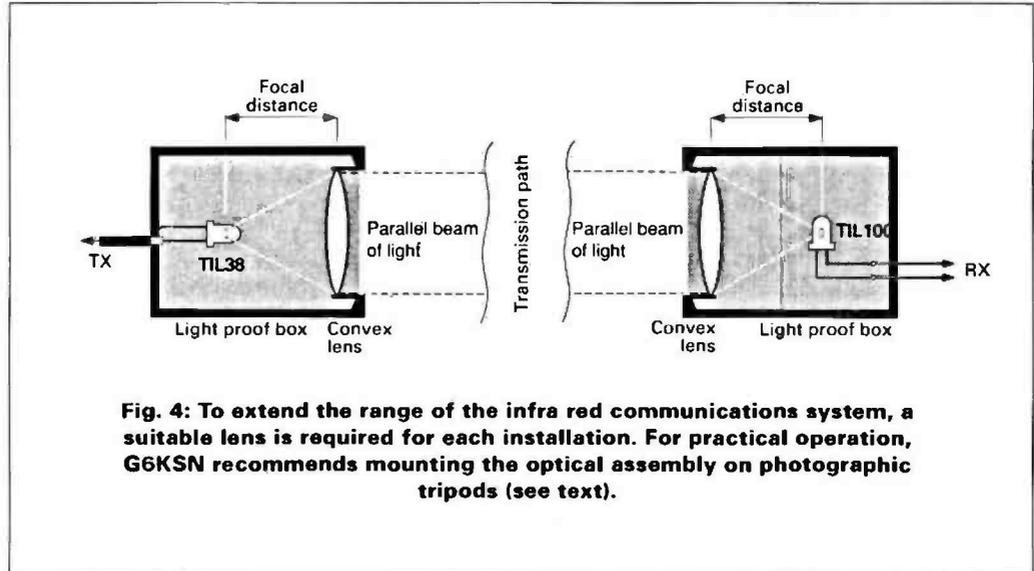
**Fig. 4: To extend the range of the infra red communications system, a suitable lens is required for each installation. For practical operation, G6KSN recommends mounting the optical assembly on photographic tripods (see text).**
