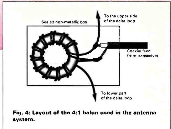
**Fig. 4: Layout of the 4:1 balun used in the antenna system.**
