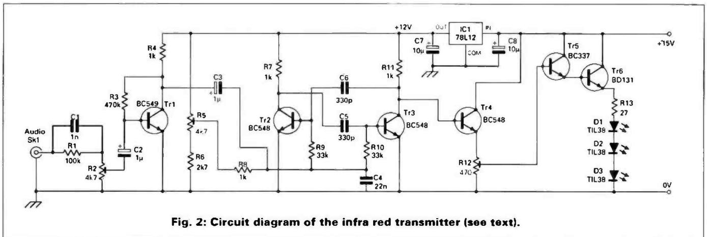
Fig. 2: Circuit diagram of the infra red transmitter (see text).
