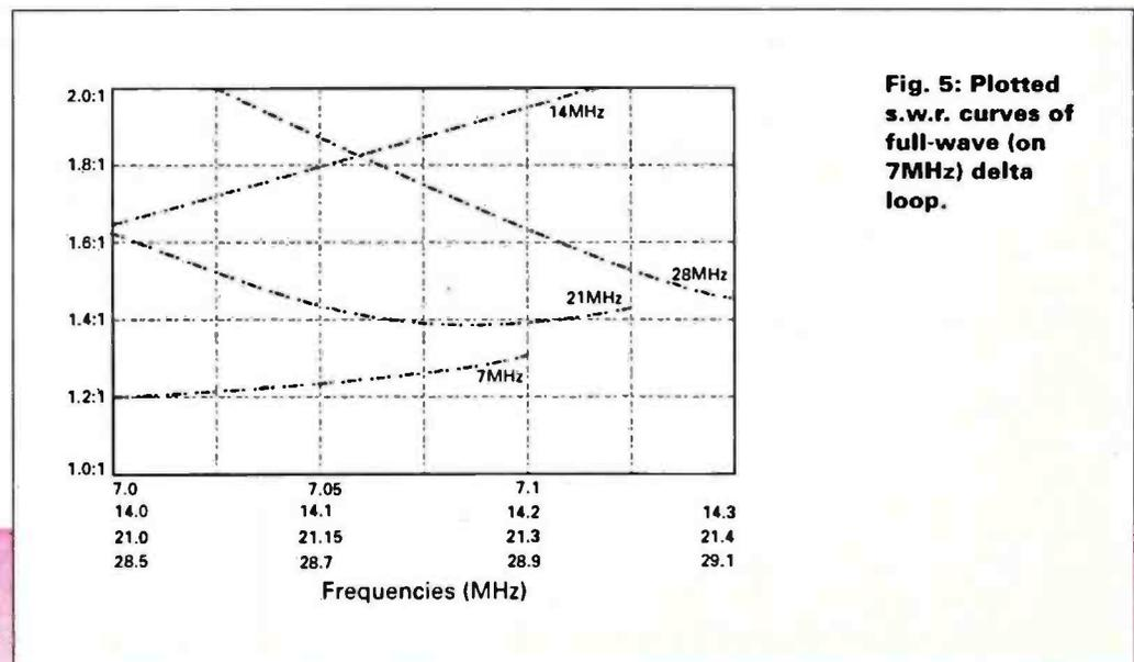
**Fig. 5: Plotted s.w.r. curves of full-wave (on 7MHz) delta loop.**
