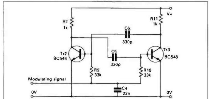
Fig. 1: A simple square wave generator, capable of being frequency modulated, forms the basis of the G6KSN infra red communications project (see text).
