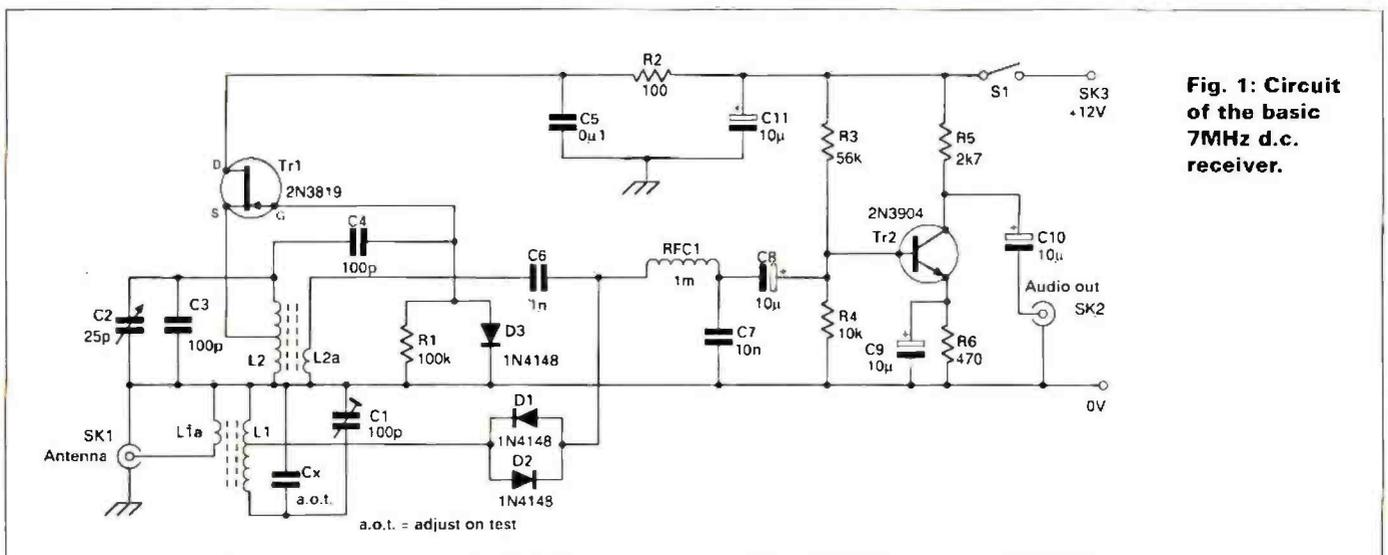
Fig. 1: Circuit of the basic 7MHz d.c. receiver.
