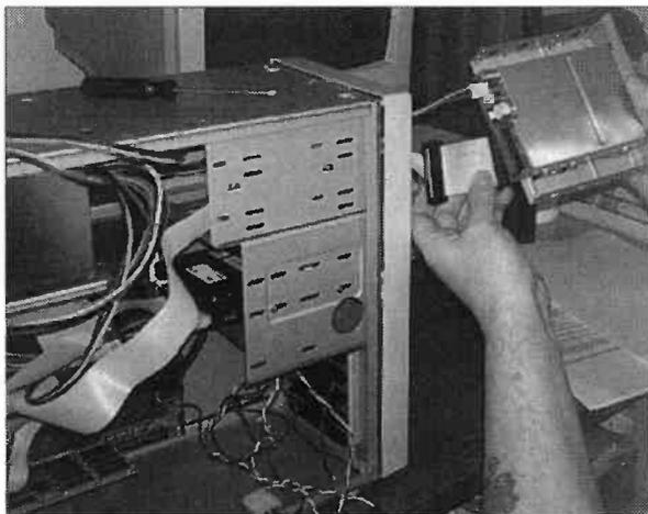
*When fitting the floppy drives, it may be easier to feed cables through the opening first*
