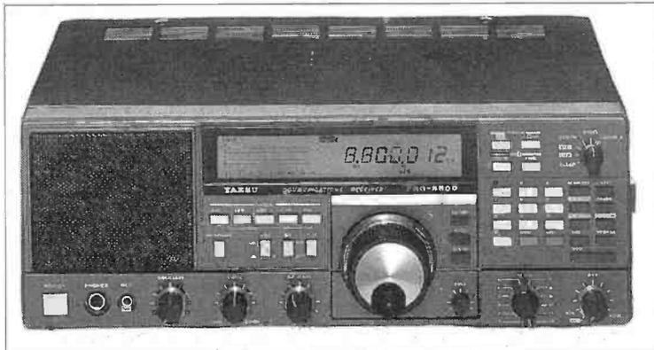
I used the BBC micro, as I had one laying around, although any computer that has the facility of a serial port that has a capability of running at 4800 bauds could be used to control the FRG-8800.
