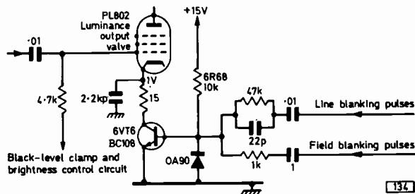
Fig. 1: Flyback blanking in the cathode circuit of the luminance output pentode.
