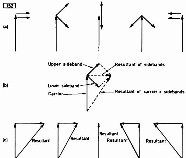
**Fig. 4:** A phase-modulated carrier is of constant amplitude but the phase rocks to and fro. An envelope detector therefore cannot "read" the modulation. (a) Sideband phasors for a phase-modulated carrier. (b) The resultant of the carrier plus its sidebands is obtained as shown here. (c) Resultants of the carrier plus the sidebands shown in (a).
