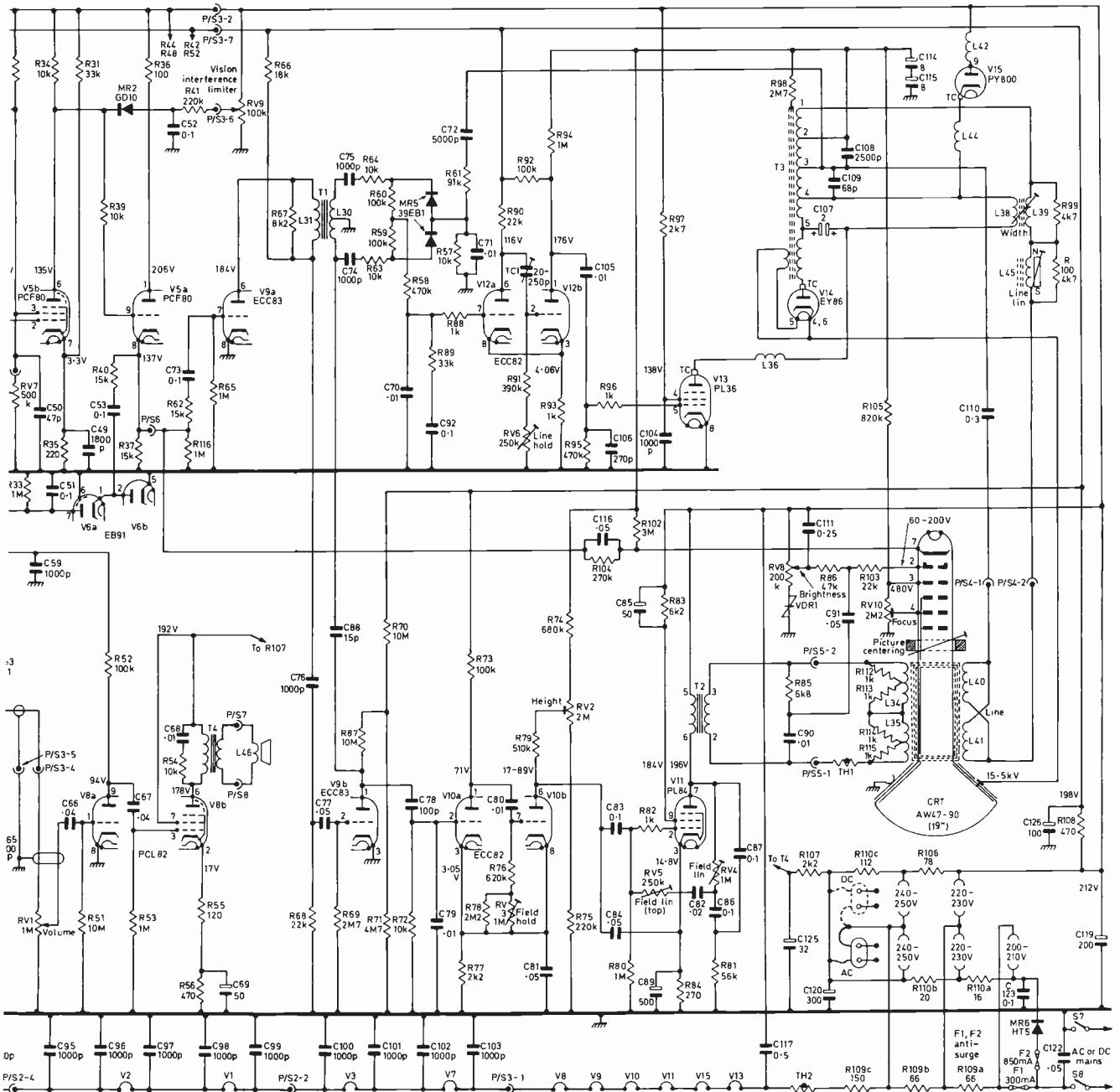
Fig. 3: Circuit diagram, Bush Models TV103, TV105, TV108, T105c and T108c. Model TV109 (21in.) is similar.
