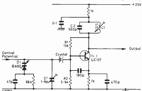
Fig. 2: Typical crystal-controlled reference oscillator circuit (Baird 700 series).
