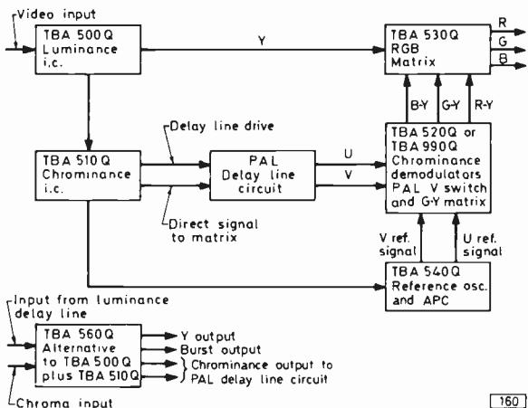
Fig. 1: Decoding with the Mullard TBA series i.c.s.
