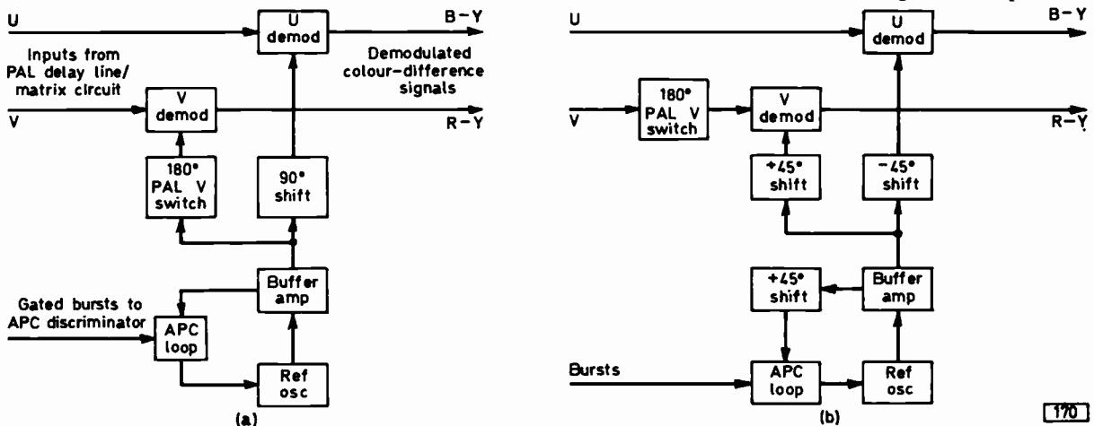
Fig. 3: The usual demodulation system (a) and the arrangement adopted in the CVC5 chassis (b).
