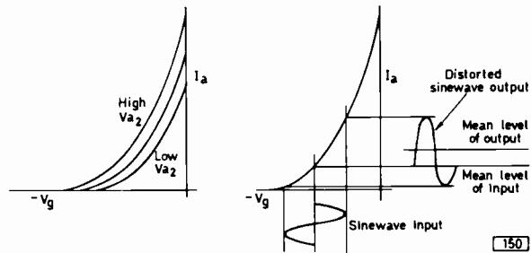
Fig. 2: (a) Beam current/grid voltage curves for a typical c.r.t. (b) The curved  $I_a/V_g$  characteristic of a c.r.t. causes an increased d.c. component of beam current output due to subcarrier rectification.
