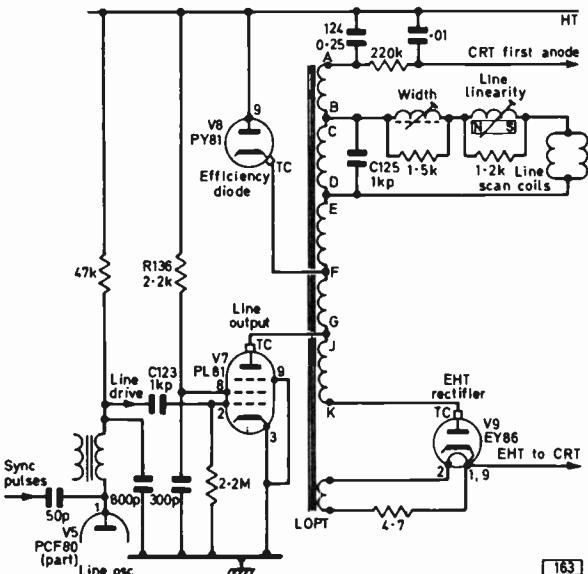
Fig. 1: Line output stage, Models 306T and 308T.
