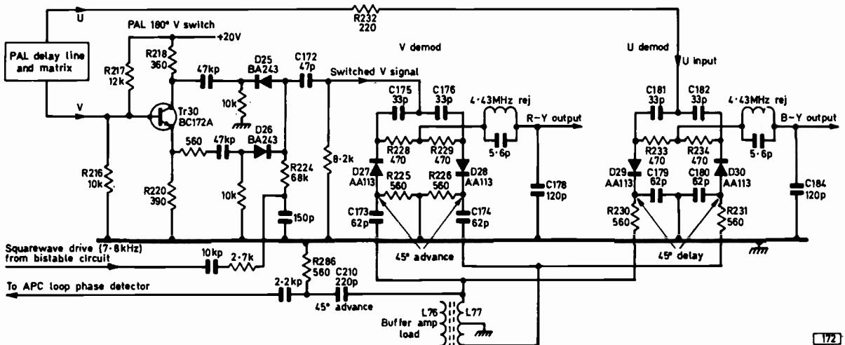
Fig. 2: The chrominance synchronous demodulator and PAL V switch circuits.
