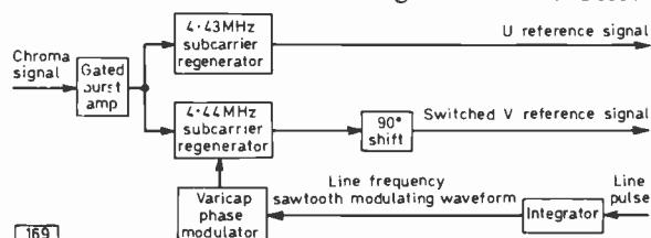
Fig. 1: GC's approach to PAL decoding.
