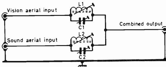
Fig. 1: Diplexer for channel F2.
