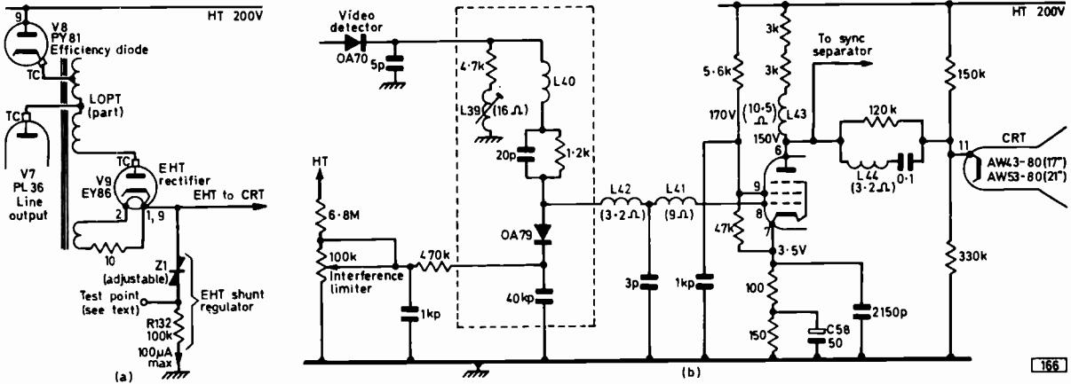
*Fig. 4: E.H.T. circuit (a) and video output stage (b), Models 406T and 408T. D.C. resistances are approximate.*
