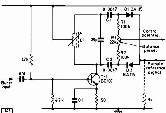
*Fig. 7: Typical phase detector circuit (Baird 700 series).*
