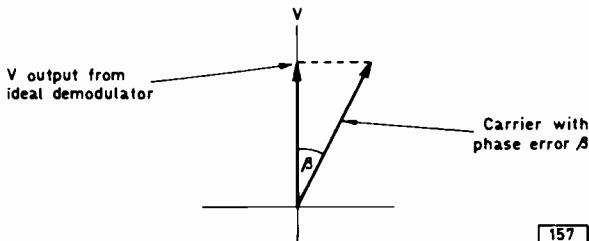
Fig. 9: Perfect demodulation of an imperfect V signal gives a pure V output although at reduced saturation.
