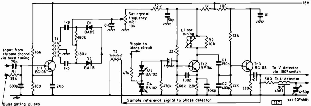
*Fig. 6: Complete reference signal channel (Decca dual-standard) from gated burst amplifier to buffer amplifier. In some circuits, as this one, two variable-capacitance diodes are used in the oscillator control section.*
