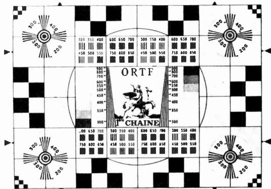
**France:** The test card for both chains is similar, with an identification below the circle to indicate the chain. At present the test card above left is used by both chains though at times the alternative version with the horse may be used. The second chain colour card is shown below.
