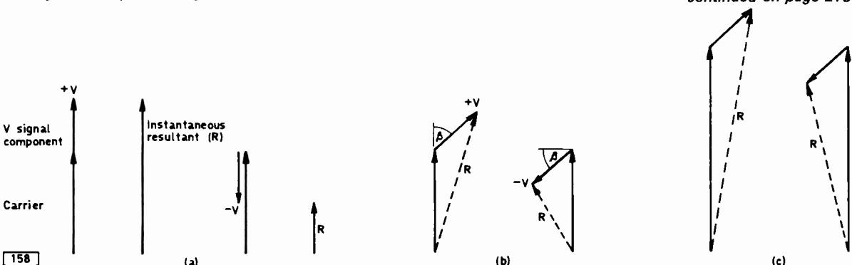
Fig. 10: Imperfect demodulators are not immune to quadrature crosstalk or phase errors in the subcarrier. (a) Correct signal phase. (b) With phase error  $\beta$  the resultant is changed as shown here. (c) Using a larger amplitude reference carrier the effect of the errors shown at (b) is reduced.
