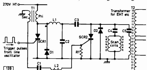
Fig. 4: Simplified thyristor line output circuit.
