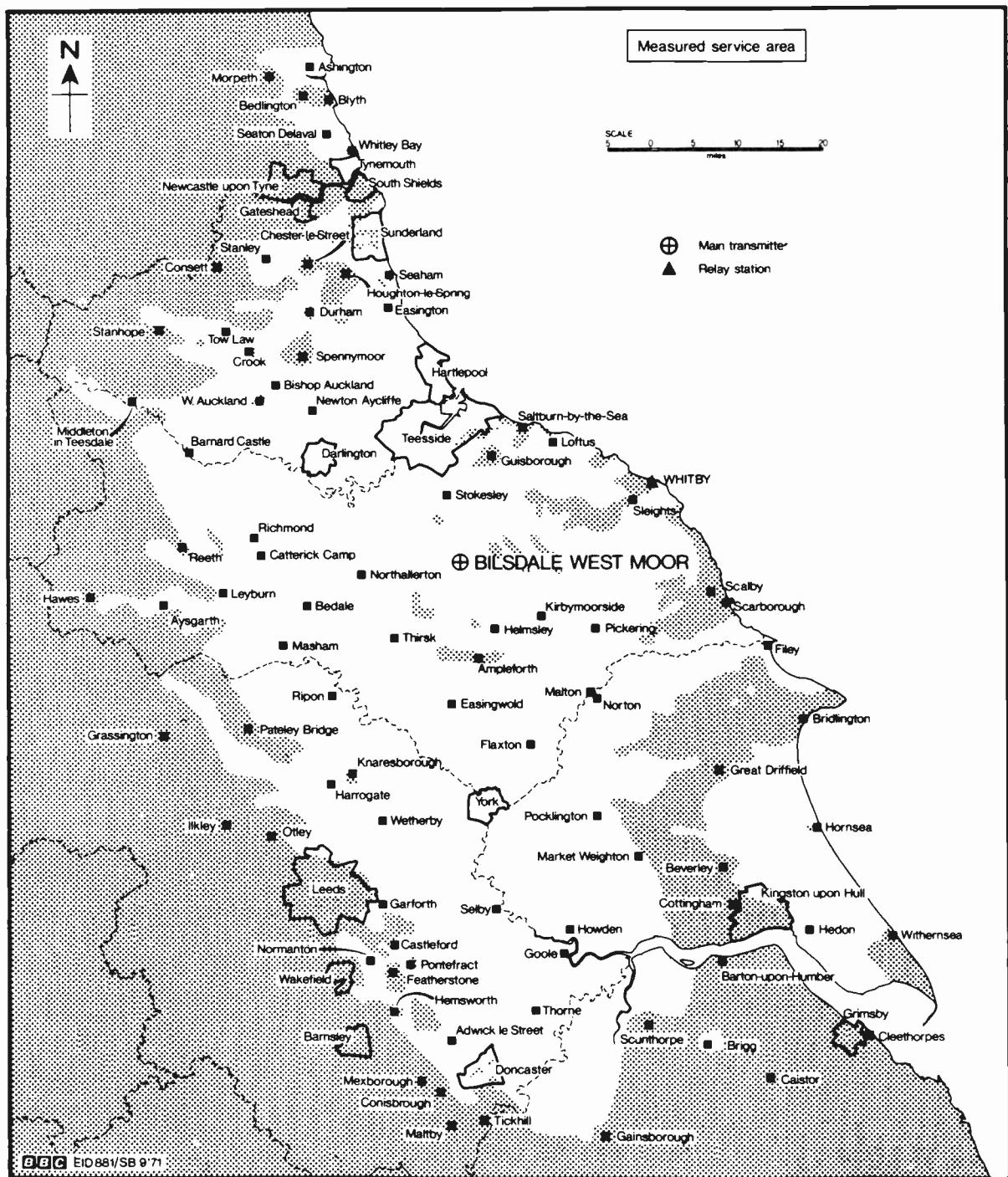
The approximate measured service area of the **Bilsdale West Moor** u.h.f. transmitter is indicated by the unshaded area of the above map. Channels: BBC-1 33; BBC-2 26; ITA 29; fourth 23. Maximum e.r.p. 500kW. Receiving aerial group A, horizontal polarisation. Map courtesy BBC Engineering Information Service.
