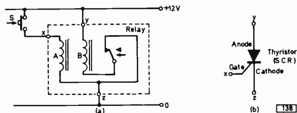
Fig. 2: Relay/thyristor analogy.
