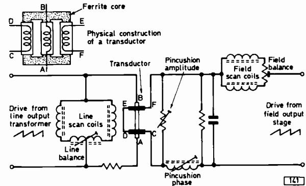
Fig. 6: Simplified  $90^\circ$  pincushion correction circuit.
