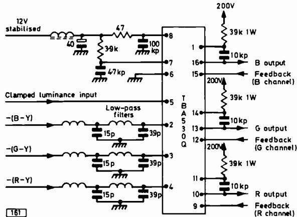
Fig. 3: External connections to the TBA530Q i.c. as used in the Philips G8 chassis.
