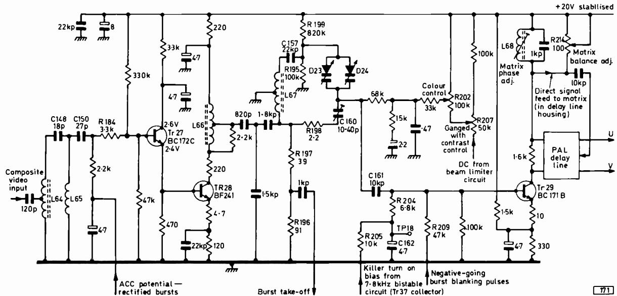
Fig. 1: The chrominance amplifier circuitry of the ITT/KB CVC5 chassis.
