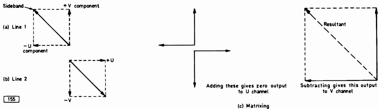
Fig. 7: The effect of single-sideband operation on a PAL chrominance signal (carrier omitted).
