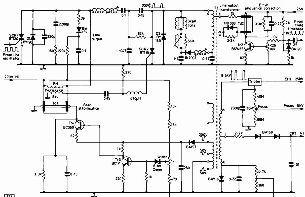
Fig. 3: Complete ITT 110° thyristor line output stage for colour receivers.
