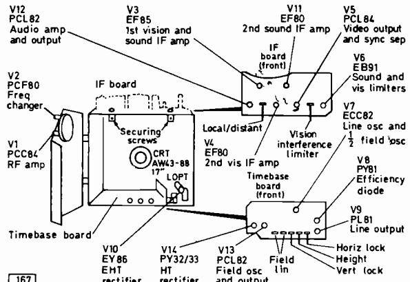
Fig. 5: Chassis layout, 506T series.
