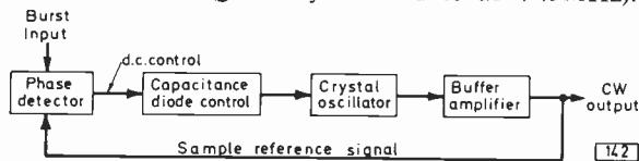
*Fig. 1: Block diagram of the reference signal channel.*
