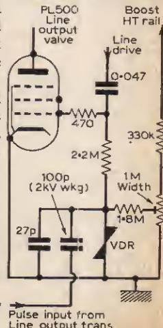
Fig. 1: Line output valve grid circuit.
