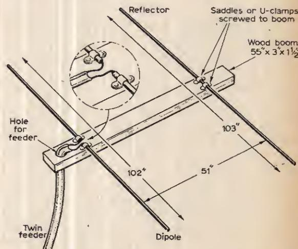
Fig. 1: The Band I aerial comprises a dipole plus reflector.
