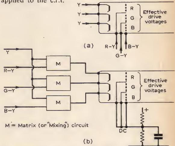
Fig. 21: Adding luminance (Y) and chrominance (R-Y, G-Y and B-Y) information to obtain a colour picture, (a) Colour-difference drive, (b) R, G, B drive.
