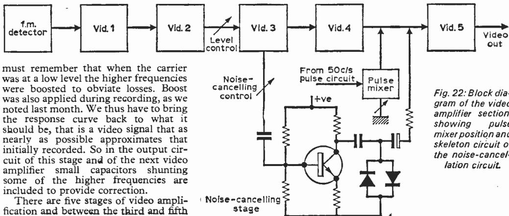
Fig. 22: Block diagram of the video amplifier section, showing pulse mixer position and skeleton circuit of the noise-cancellation circuit.
