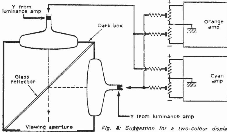
Fig. 8: Suggestion for a two-colour display system using two direct-viewed tubes and feeding them with orange and cyan colour-difference signals from the set-up shown in Fig. 7 or matrixed as shown from the "orange" (i.e. R-Y) and "cyan" (i.e. B-Y) outputs of a standard decoder.
