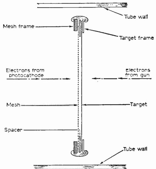
Fig. 3: Vibrating components of image orthicon.
