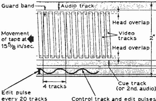
Fig. 8: Arrangement of tracks with a standard four-head video tape recorder.
