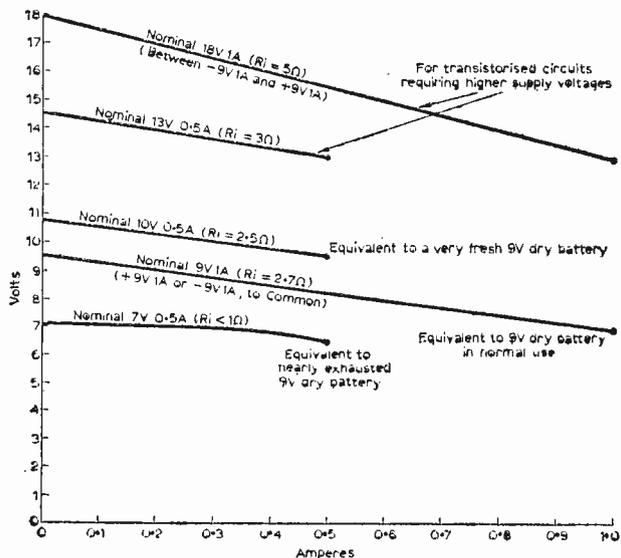
Fig. 2: Load characteristics of L.T./D.C. outputs. Except for very small currents (bias circuits) of a few mA do not take outputs between the 7/10/13V 0.5A sockets. For high currents these outputs MUST be used with the common positive socket. The -9V/ Common/+9V 1A outputs may be used in any combination even at high current.
