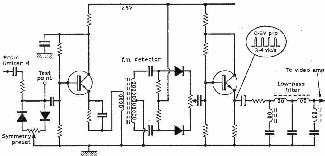
Fig. 21: Final limiter stage and f.m. detector. The detector output is fed to the video amplifier section via an emitter-follower and low-pass filter.
