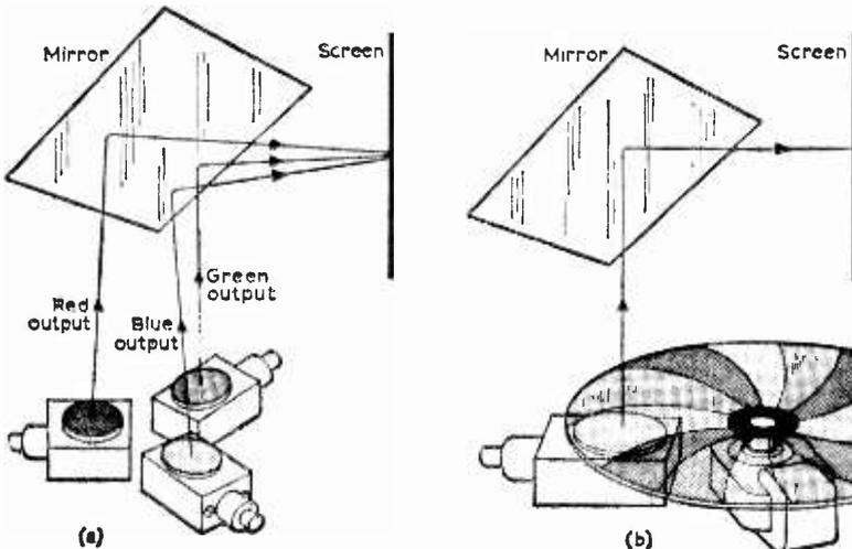
Fig. 5: Using projection units to provide a three-colour display. The snags are that the three optical units in (a) would be difficult to register while synchronising (b) would be just as hard as three into fifty does not go!
