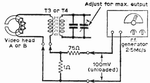
Fig. 19c: Tuning head transformer circuits requires an r.f. generator tuned to 2.5Mc/s with a matching pad in the head return lead.
