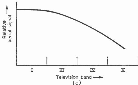
Fig. 1: (a) Fall in receiver sensitivity with increase in channel number. (b) Required increase in aerial signal with channel number increase to maintain the same signal-to-noise performance. (c) General effect of signal fall-off with increase in channel number.
