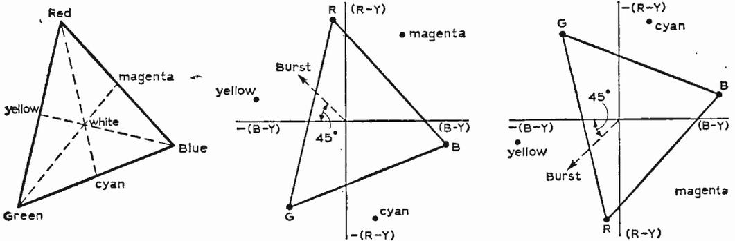
Fig. 6: Maxwell's colour triangle for lights (painters note: the mixtures don't work with pigments!). (a) Showing how white light comes from mixing a primary colour and its complementary intermediate. (b) Vectors for one line of PAL with the triangle of (a) superimposed. (c) Inverted vectors for the succeeding line in the PAL system.
