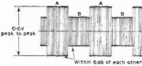
Fig. 19b: The outputs from the preamplifiers appear at TP9 as successive "blocks" which should be within 6dB of each other for correct playback conditions, with a minimum peak-to-peak voltage of 0.4V.
