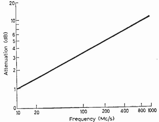
Fig. 7: Attenuation increase with increase in signal frequency
