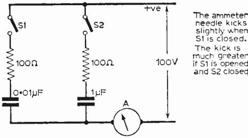
Fig. 2: Effect of capacitance on charging current.
