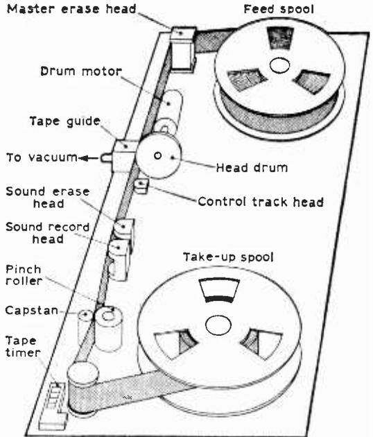
Fig. 7: Basic deck layout of the Ampex 1000 video tape recorder.
