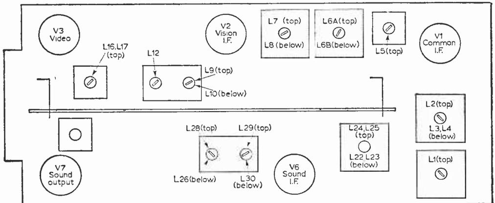
Fig. 7: Valve and coil positions on the receiver printed panel.
