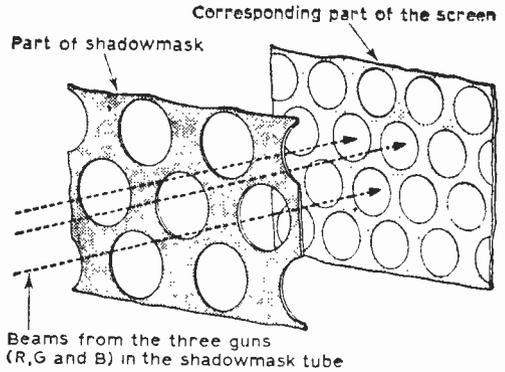
Fig. 4: Why shadowmask tubes prefer a dark corner. The spaces between the coloured dots on the screen contribute nothing towards illumination while the shadowmask itself has only one hole for each group of three dots on the screen. Thus only a quarter of the beam current is turned into useful light.
