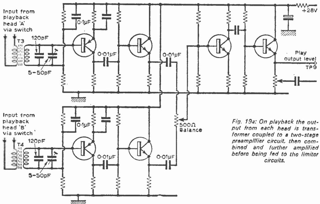
Fig. 19a: On playback the output from each head is transformer coupled to a two-stage preamplifier circuit, then combined and further amplified before being fed to the limiter circuits.
