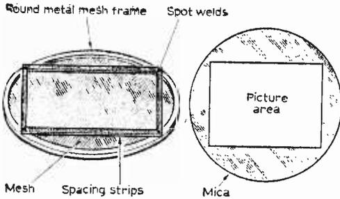
Fig. 4: Target spacing strips.
