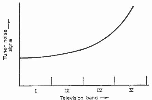
Fig. 4: Increase in tuner noise with increase in channel number.
