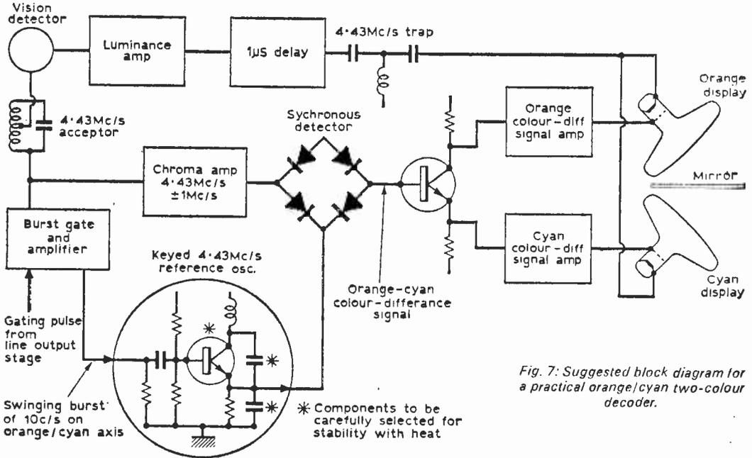
Fig. 7: Suggested block diagram for a practical orange/cyan two-colour decoder.
