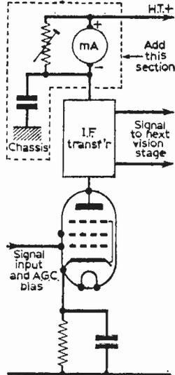
It now remains to see how any change in receiver signal due to altering the aerial system can be detected. The best way, of course, is to measure the signal on a signal-strength meter while aerial adjustments are being made, but very few readers will be in possession of such an instrument, especially for the u.h.f. bands.
