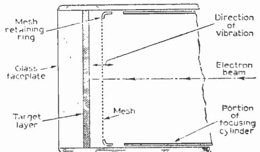
Fig. 1: Microphonic portion of vidicon tube.
