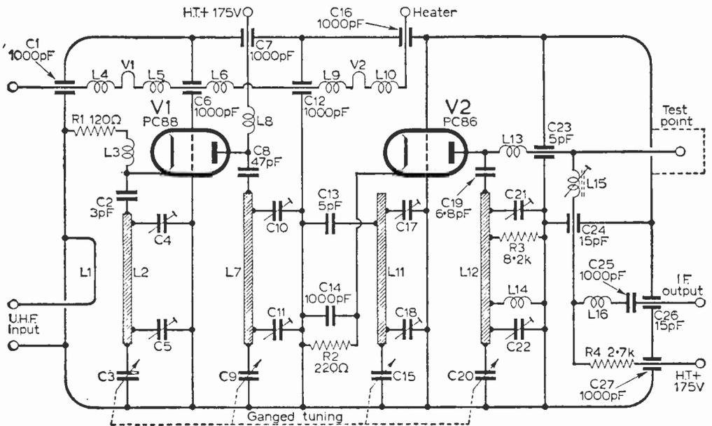
Fig. 6: Circuit diagram of the u.h.f. tuner unit.
