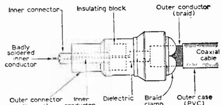
Fig. 8: Correct way of connecting a coaxial plug. Avoid badly soldered inner conductor to plug inner connection, especially at u.h.f.
