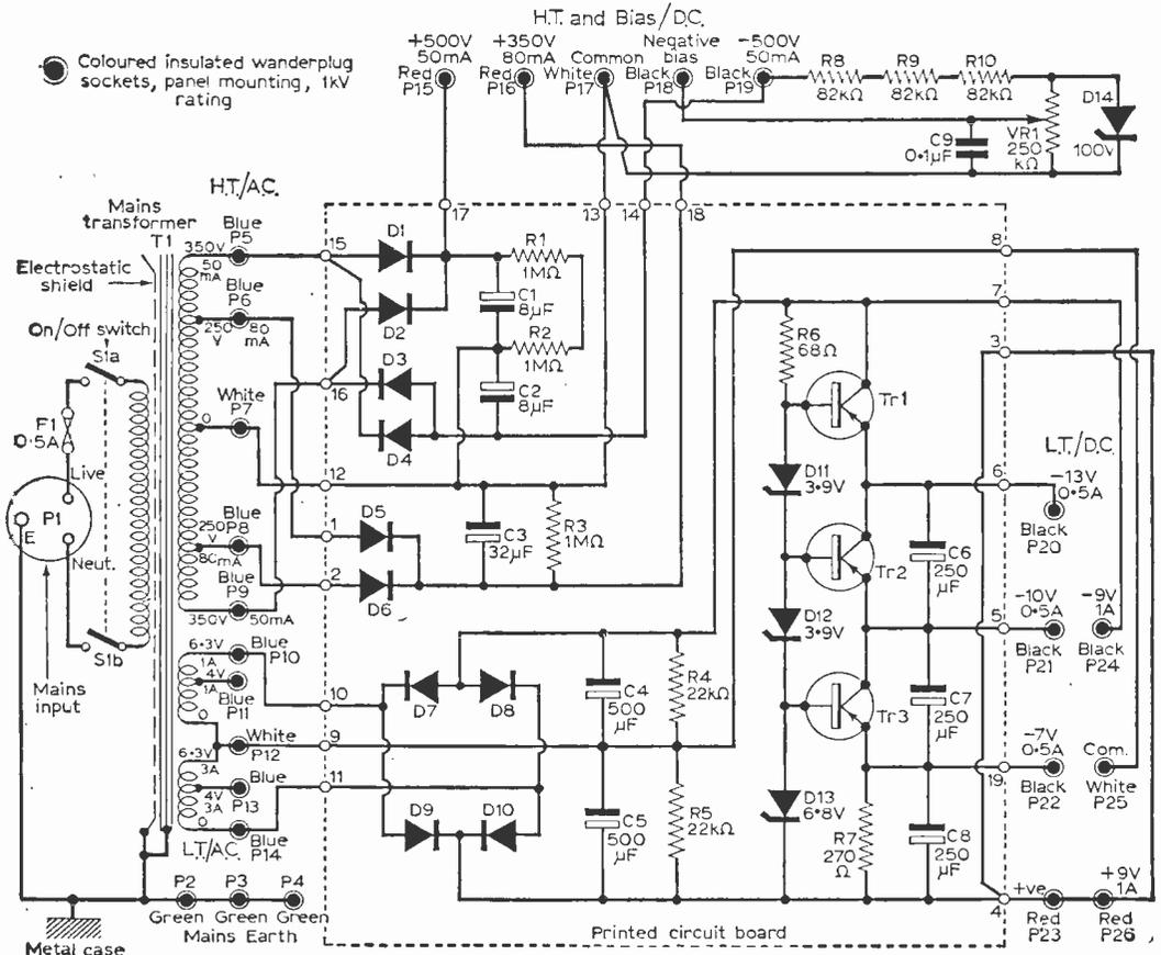
Fig. 1: Complete circuit of the bench power unit.
