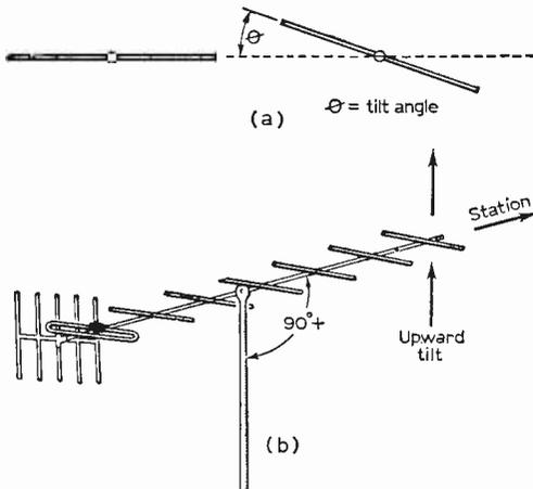
Fig. 6: Tilting the aerial (a) to line up with the plane of polarisation and (b) to increase effective aerial height.
