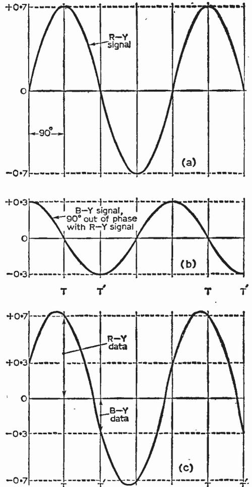
Fig. 6: The principle of synchronous demodulation.
