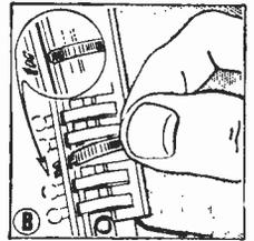
Fig. 53: Fixed spring blade contacts can be adjusted as in A and removed and replaced as in B. Correct lift (Thorn 950 tuner) at the spring tip should be between 1 and 2½mm. Working contact pressure should be about 60 grammes. Block is soldered into place and can be eased out by melting the support with a heavy-duty iron. Some care is needed when repositioning. Excessive pressure soon weakens contacts.
