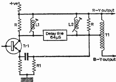
Fig. 5: Technique suggested by Mullard for adding and subtracting in conjunction with their DL1 delay line to provide separate R-Y and B-Y outputs (simplified circuit).
