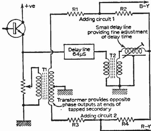
Fig. 4: Practical aspects of a PAL delay line circuit.
