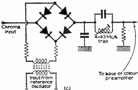
Fig. 7c: Semiconductor bridge demodulator.
