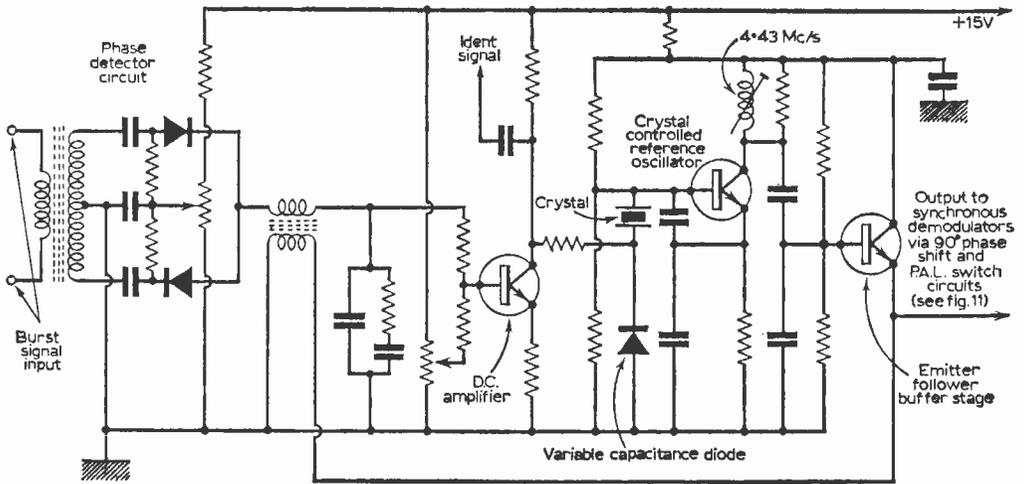
Fig. 11 (above): Simplified circuit of a crystal reference oscillator with phase detector and control circuits.
