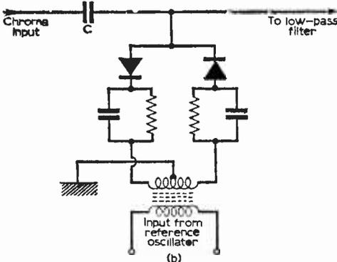
Fig. 7b: Synchronous demodulator using two diodes.
