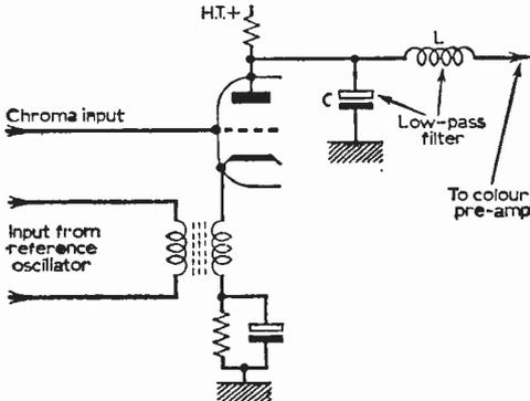
Fig. 7a: A simple synchronous demodulator circuit using a triode valve. A low-pass filter and subcarrier rejector are included in the output circuit.
