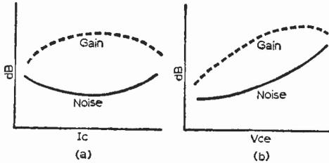
Fig. 51: Noise and gain levels vary with both collector voltage and current. Exact setting for optimum conditions in a transistor tuner can be important.
