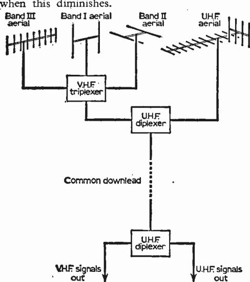
Fig. 2: While the existing v.h.f. downlead can also be arranged to carry the u.h.f. signal by the use of top and bottom u.h.f. diplexers, as shown, this technique should be avoided in areas of weak signal or where picture grain is troublesome.
