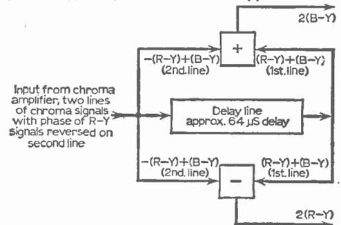
Fig. 2 (above): How the delay line circuit separates the B-Y and R-Y signals and carries out averaging over successive pairs of lines.
