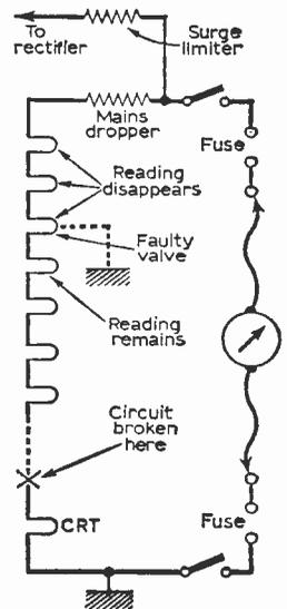
Fig. 1: Testing for heater/cathode leaks with an ohmmeter.
