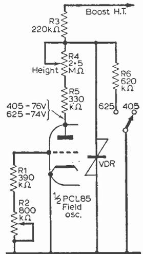
Fig. 1: Height stabilising circuit used in Ferguson/HMV/Ultra 16in. range of portables.
