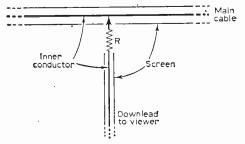
Fig. 37—Simple resistive tap for signal take-off from coaxial spur or main cable. The value of R determines the amount of signal taken from the line and the amount of loss introduced to it. Practical values range from about  $180\Omega$  to  $2700\Omega$ .
