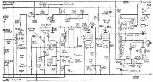
Fig. 6-The line timebase circuit.
