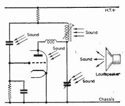
Fig. 4—Microphony symptoms can arise from the exciting vibrations modulating the local oscillator in the tuner. This occurs mainly from the sound causing a change in one of the components used for frequency control of the oscillator in the tuner, as this diagram shows.
