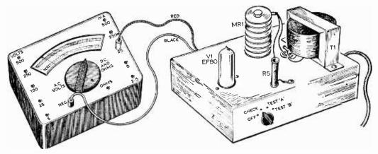
Fig. 3-The above-chassis layout.
