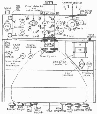
Fig. 2—An example of stage and valve layout (Ferranti 14T3 series).
