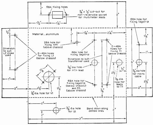
Fig. 2—The chassis drilling.
