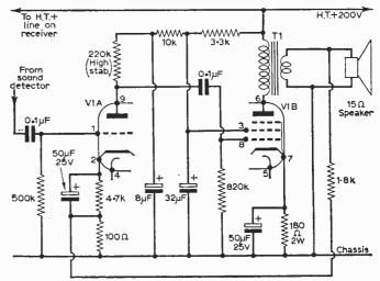
Fig. 4—Experimental audio stage for giving improved sound in conjunction with a good quality extension speaker system. VI Mullard PCL86; T1 primary impedance 7kΩ. primary inductance 10H, primary resistance 350Ω. All resistors ½W and capacitors 300V working unless otherwise stated. Extension loudspeaker isolation must be adopted as described in the text.
