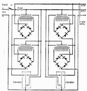
Fig. 2—12V vibratory power unit—part of ZA21531, Power Supply and Amplifier Unit No. 1. The chokes and capacitors are not shown. A photograph of the converted unit is shown in the heading.
