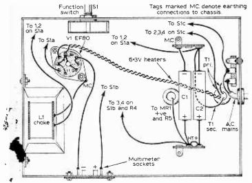
Fig. 5—The underchassis wiring diagram and component layout.
