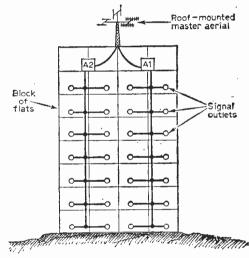
Fig. 35—Flat system. Here the master aerials are mounted on the roof and the signals are divided between two amplifiers Al and A2. Each amplifier feeds its own main cable which is tapped for signal at each dwelling. In some systems a single amplifier system is used and the two main cables are then fed through a circuit splitter (see Fig. 36).
