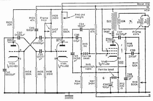
Fig. 7—The frame timebase stage.
