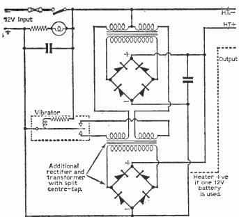
Fig. 3—The modification of a Type No. 9 vibratory power unit by the addition of an extra transformer and rectifier.
