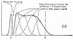
Fig. 1—Vision receiver i.f. response characteristics, as discussed in the text.
