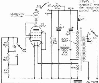
Fig. 1—The circuit diagram of the unit. The switch SI is shown in the "off" position.
