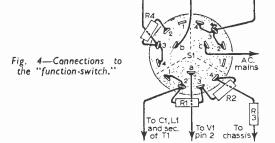
Position 4. "TEST B." Grid bias is now further reduced to approximately 1.5V, and the meter reading will rise to about 25mA for a good valve.
