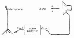
Fig. 1—Showing basic microphony. A feedback path is established partly acoustically from microphone to loudspeaker and partly electrically from the input to the output of the amplifier.
