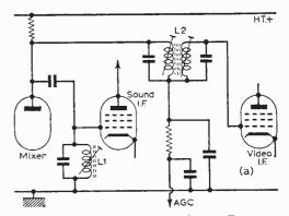
Fig. 2a (above)—Capacitive sound take-off circuit.
