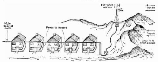
Fig. 34—Small shared aerial system. Signals picked up by the hill-sited aerials are fed into the shielded area through coaxial cable after first being amplified at the aerial by AI and by A2 at the start of distribution. Feeds to houses are taken through resistive taps as described last month.
