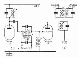
Figs. 2c and d—Absorption sound take-off circuits.
