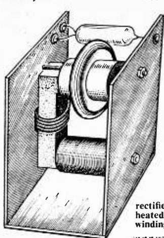
Fig. 8.—Typical line output transformer. The high voltage rectifier slung at the top is heated by the four-turn winding on the side limb.
