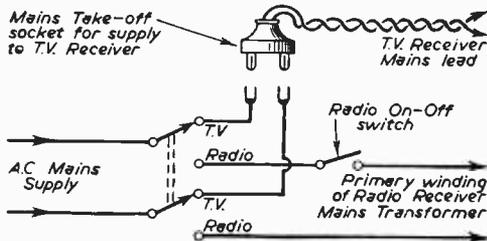
Fig. 2.—Changeover switching for mains supply to TV or radio.
