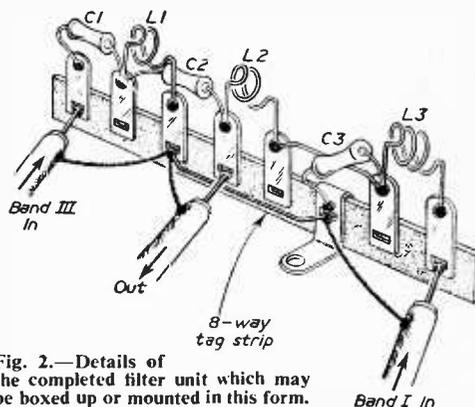
Fig. 2.—Details of the completed filter unit which may be boxed up or mounted in this form.
