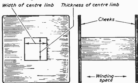
Fig. 2.—Bobbin and core size.
