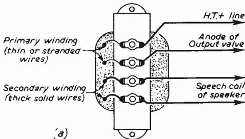
Fig. 3a.—Connections to output transformer before modification.
