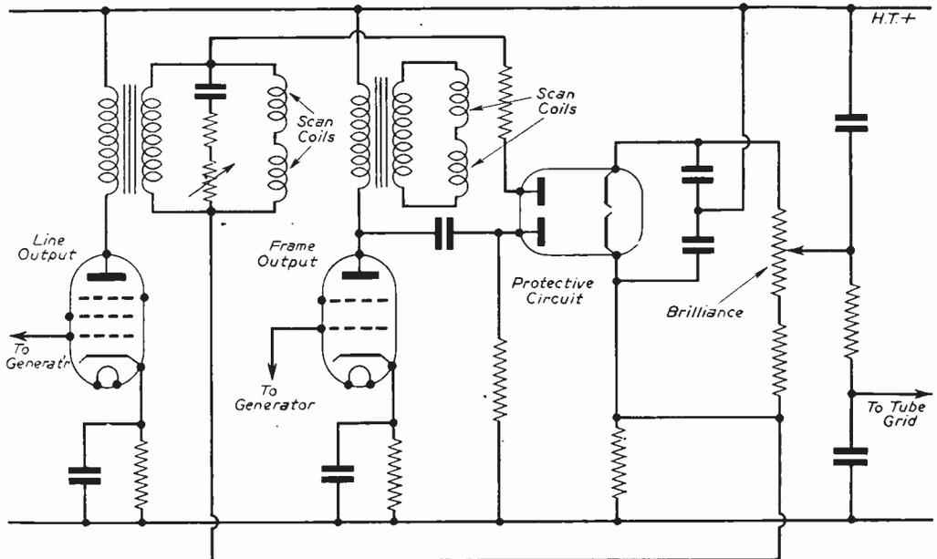
Fig. 49.—Projection tube protection circuit.
