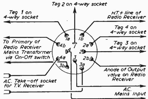
Fig. 5.—Connections to 4-pole, two-way switch.
