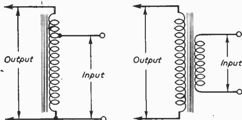
Fig. 1.—Auto and two-winding transformers.
