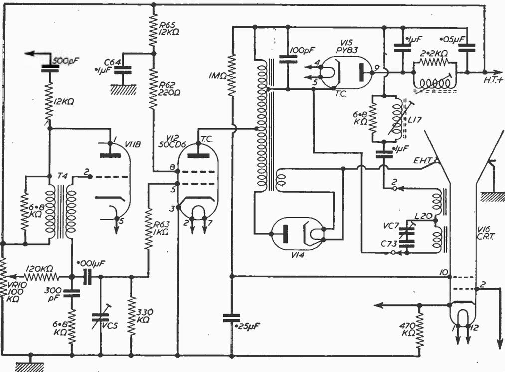
Fig. 3.—Line timebase circuit.
