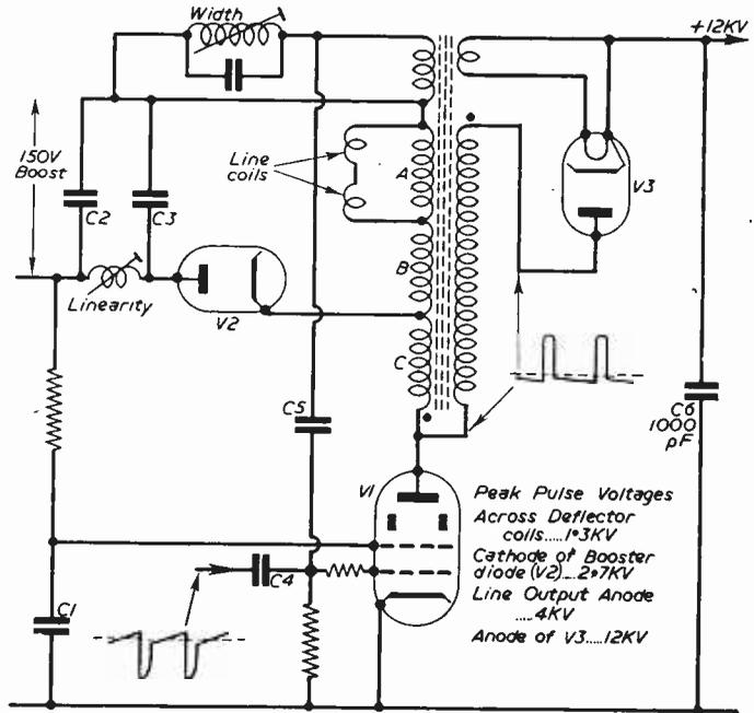
Fig. 7.—Line output stage for 17in. tube.
