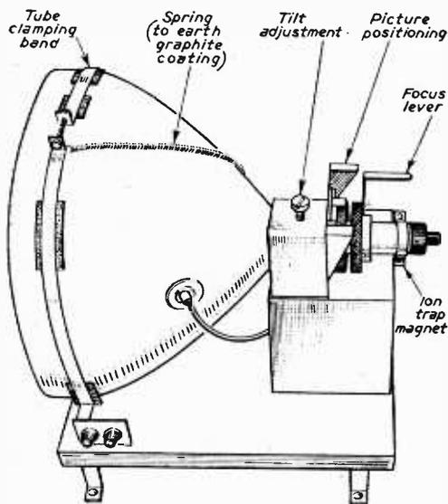
Fig. 5.—Cossor 945; chassis with cabinet removed.
