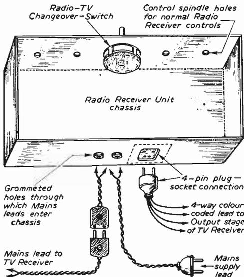
Fig. 6.—Suggested layout and interconnections between radio chassis and TV receiver.
