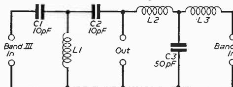
Fig. 1.—A complete high-pass/low-pass filter network for Band III and Band I frequencies.
