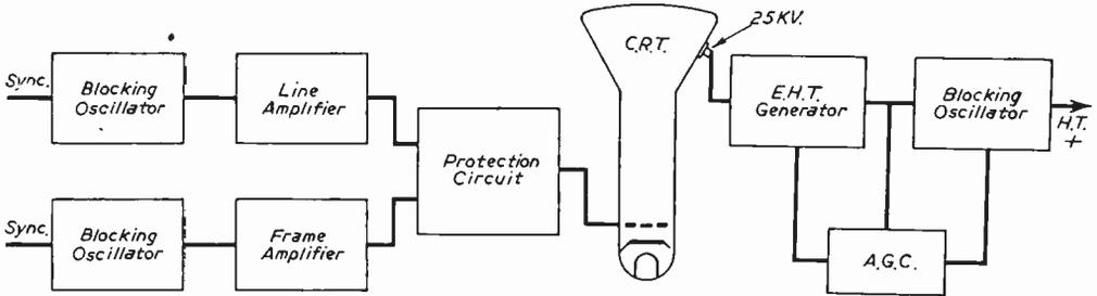
Fig. 48.—Block diagram of time bases and EHT generator in projection receivers.
