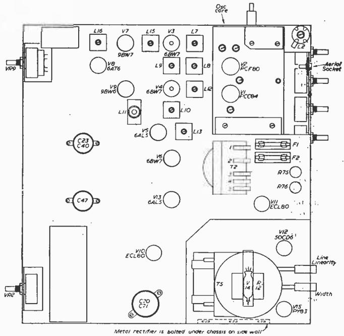
Fig. 2.—Plan view of chassis.
