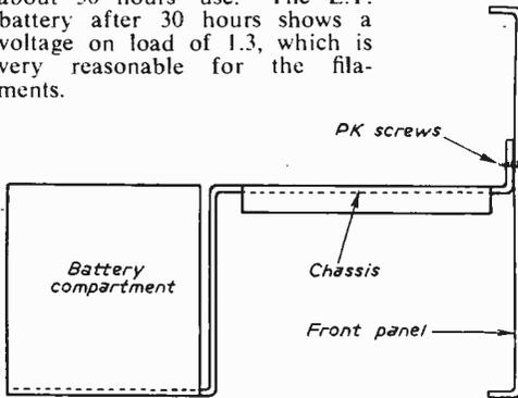
Fig. 4.—Assembly of the chassis and battery compartment.
