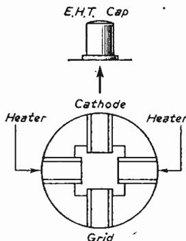
Fig. 3.—Base connections of the 10in. Cossor 108K ion trap triode.
