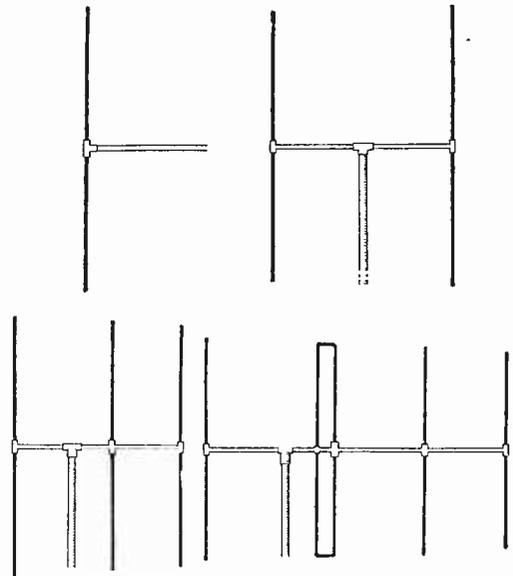
Fig. 1.—The four basic types of aerial, is the simple dipole, the 'H' and 'H' with one director, and a folded dipole with reflector and two directors.
