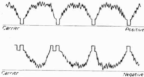
Fig. 3.—Positive and negative modulation.
