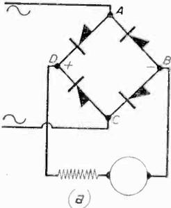
Fig. 1(a) The basic bridge rectifying circuit used in meters.
