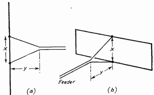
Fig. 17.—On the left a delta match, and on the right a delta applied to a slot.
