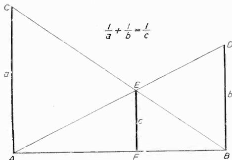
Fig. 1. — The basic principle of the calculator. See also Note 1 (page 369).
