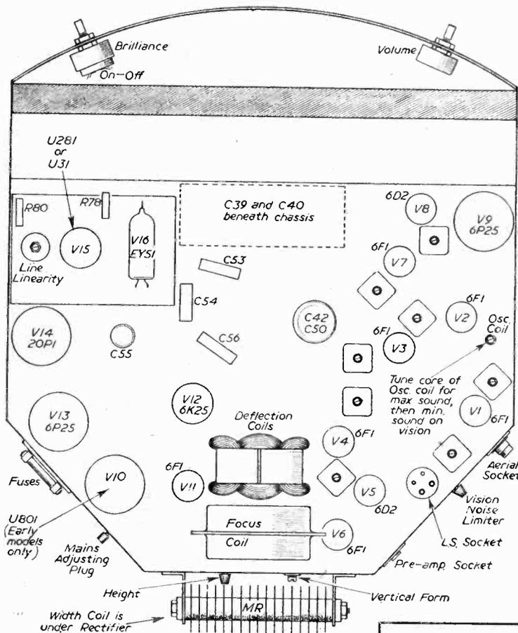
Fig. 3.—Top of chassis view.
