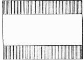
Fig. 2.—Shape of CinemaScope 2.35 to 1 picture on TV screen, reproducing full width, but masking top and bottom.
