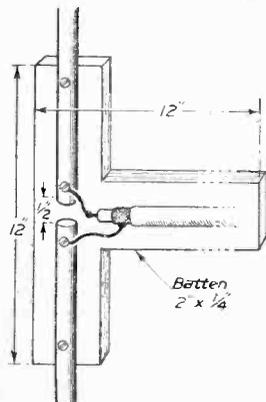
Fig. 2.— A simple and effective method of connecting the feeder to a dipole.
