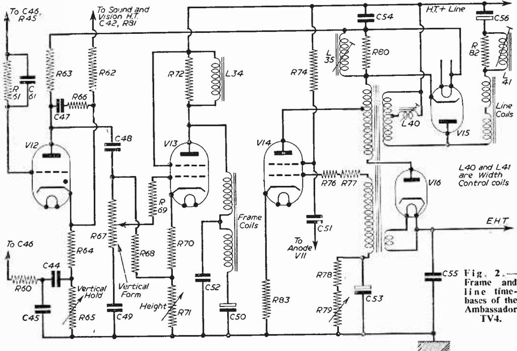
Fig. 2.— Frame and line timebases of the Ambassador TV4.
