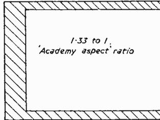
Fig. 1.—Shaded area indicates section of old silent film frame which is not reproduced on television. "Academy" area is fully reproduced.
