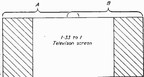
Fig. 3.—When reproduced to the full height of the TV screen, each side of CinemaScope picture is cropped (in section shaded above). This restricts the choice of CinemaScope film sequences for TV to those with main action in the centre. A-TV's new scanning system permits a panoramic shift from "A" to "B" to follow the main action.
