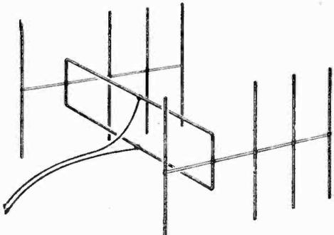
Fig. 18.—A Yagi array with slot aerial.
