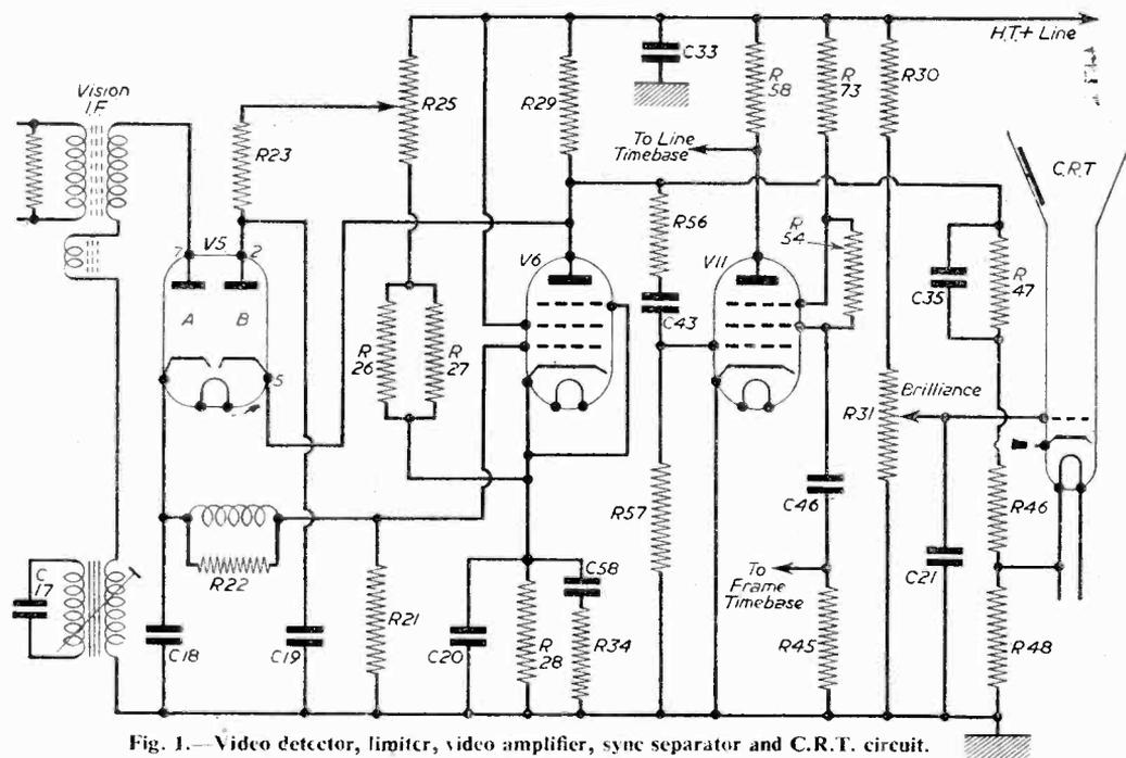
Fig. 1.—Video detector, limiter, video amplifier, sync separator and C.R.T. circuit.
