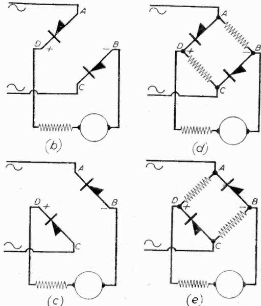
Fig 1 (b) to (e). How the bridge rectifier works.
