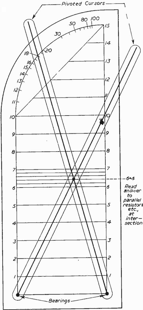
Fig. 5.—The finished calculator.
