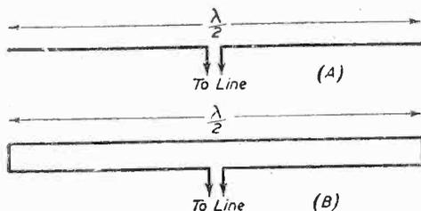
Fig. 3.—The simple dipole and a folded dipole aerial.
