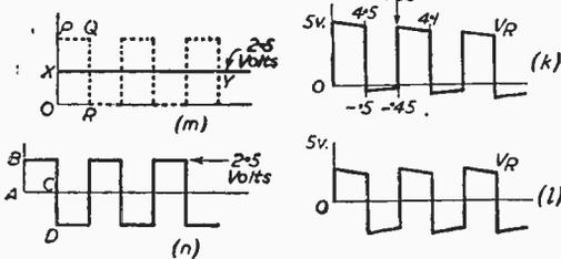
The pulse period will be referred to as the positive half-cycle and the interval between as the zero half-cycle. Assume that the frequency is related to the time constant of the circuit so that the capacitor C (Fig. 1) will charge to one-tenth of the applied voltage.
