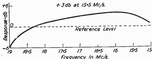
Fig. 3.—Response curve of the I.F. alignment before rejectors are fitted.
