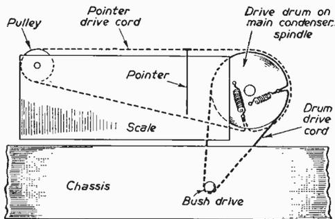
Fig. 3.—Suggested dial and condenser drive arrangement.
