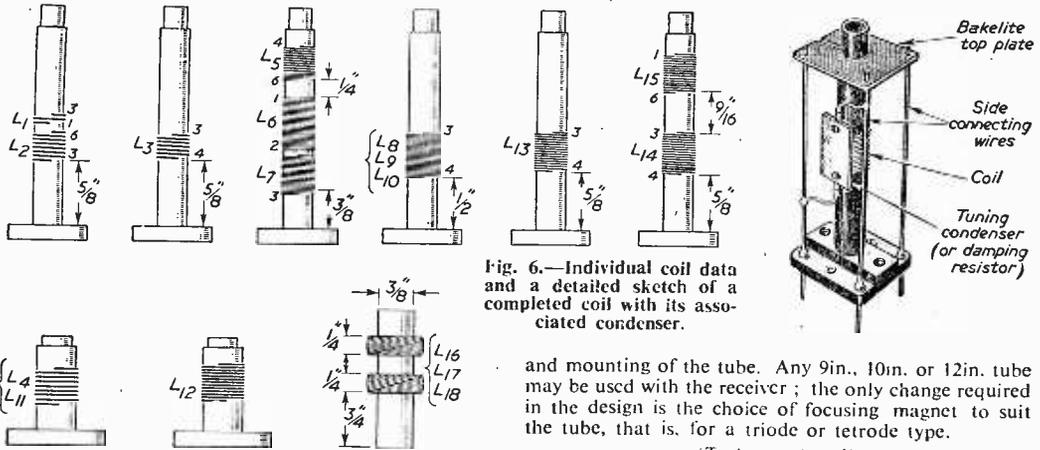
Fig. 6.—Individual coil data and a detailed sketch of a completed coil with its associated condenser.
