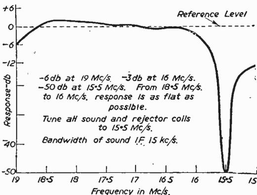
Fig. 4.—I.F. response after rejectors are tuned.
