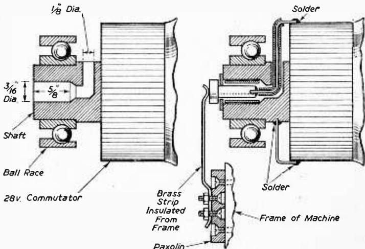
Fig. 2.—Details of holes for A.C. lead.
