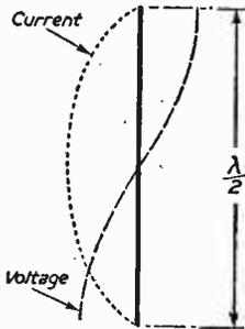
Fig. 1.—Voltage and current distribution along a wire which is a half wavelength long.
