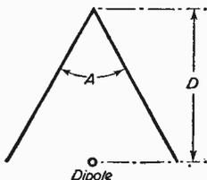
Fig. 5.—A corner layout for use in restricted places. Netting may be used for the reflector.
