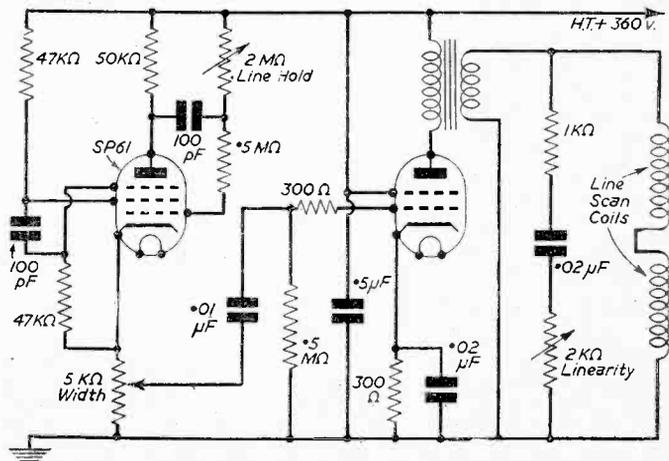
Fig. 1.—Experimental line time-base circuit.
