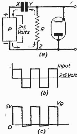
Fig. 7.—Action of circuit during D.C. restoration.
