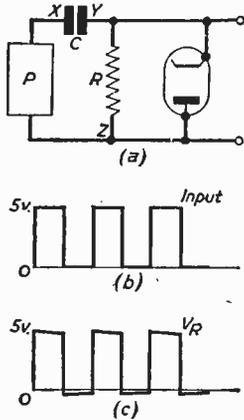
Fig. 5 (left).—The circuit of Fig. 1 with diode added. Fig. 6 (above).—Diode conducts during zero half-cycle.
