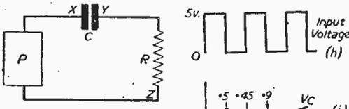
Fig. 1 (above).—The basic series circuit.
