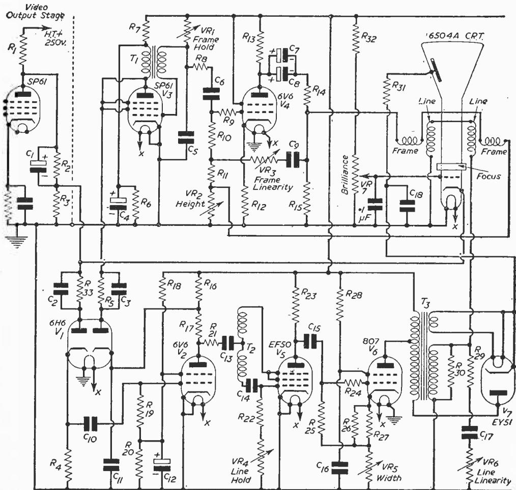
Fig. 2.—Complete circuit of the final arrangement.
