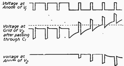
Fig. 2.—The action of V2 is illustrated in this diagram.
