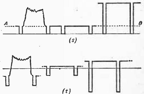
Fig. 4.—Three typical signal waveforms as they appear (s) after detection and (t) with D.C. component removed
