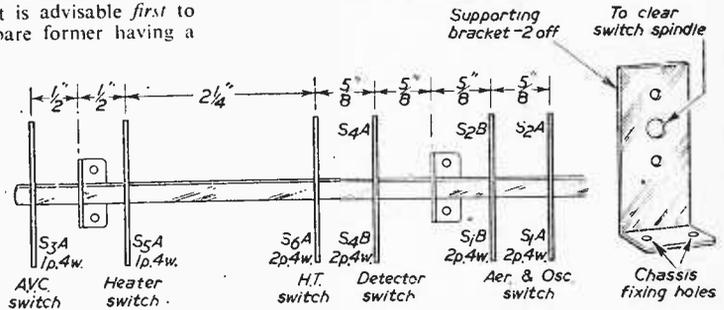
Fig. 5.—Ganged switch details.
