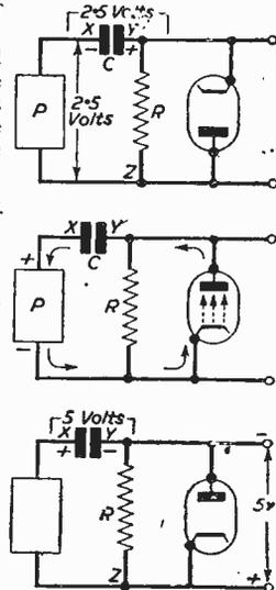
Figs. 8, 9, 10.—Diode can be used to invert the waveform.
