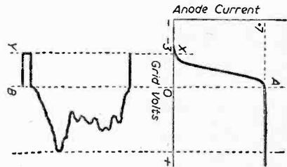
Fig. 12.—Valve characteristics required for sync separation.
