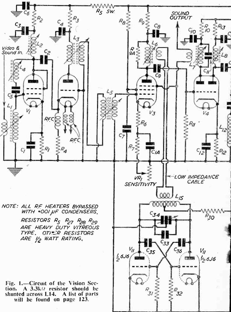
NOTE: ALL R.F. HEATERS BYPASSED WITH 0.001  $\mu$ F CONDENSERS. RESISTORS R<sub>5</sub> R<sub>27</sub> R<sub>28</sub> R<sub>29</sub> ARE HEAVY DUTY VITREOUS TYPE. OTHER RESISTORS ARE 1/2 WATT RATING.
