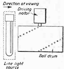
Fig. 3.—The ball drum scanner.
