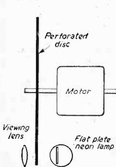
Fig. 1.—The simple disc apparatus.
