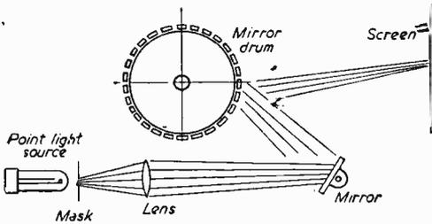
Fig. 5.—The mirror drum projection arrangement.
