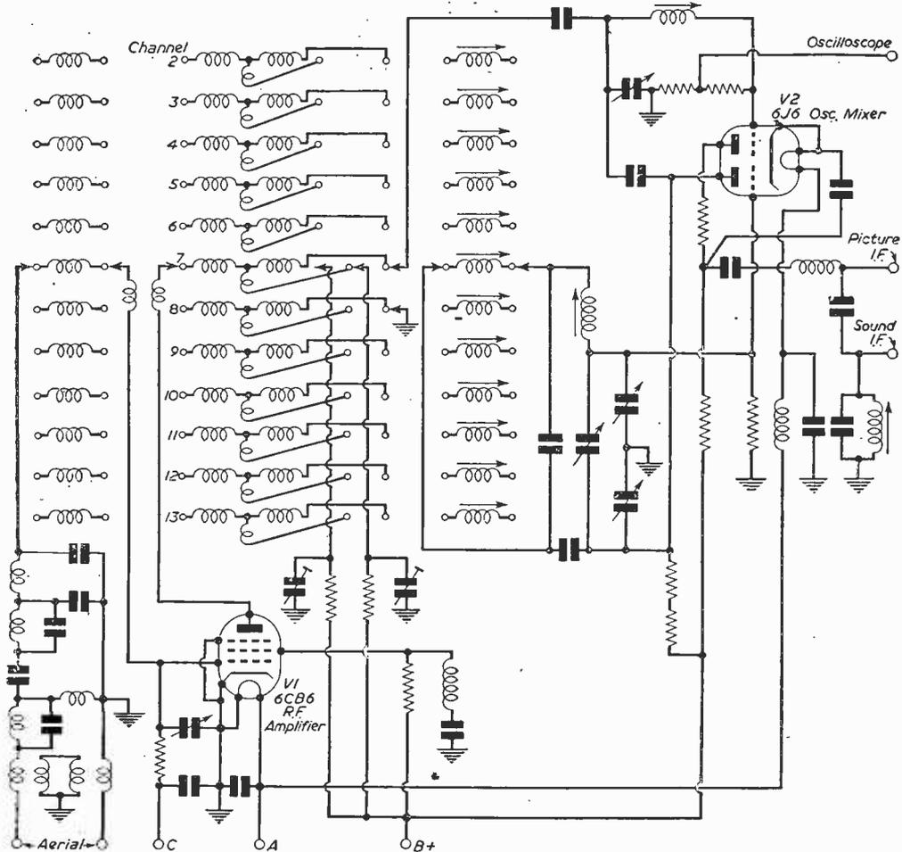
Circuit of the American tuner referred to in this article. The heater and cathode of V2 are earthed.
