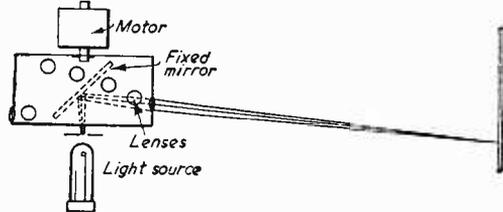
Fig. 7.—A lens-drum projector.
