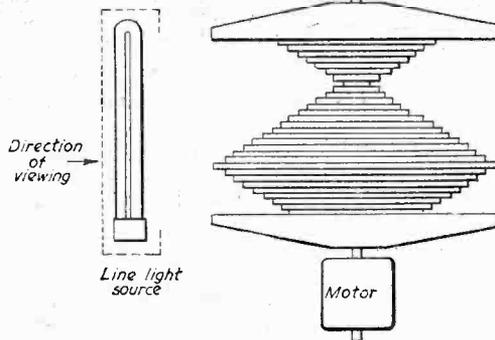
Fig. 2.—The mirror screw apparatus.
