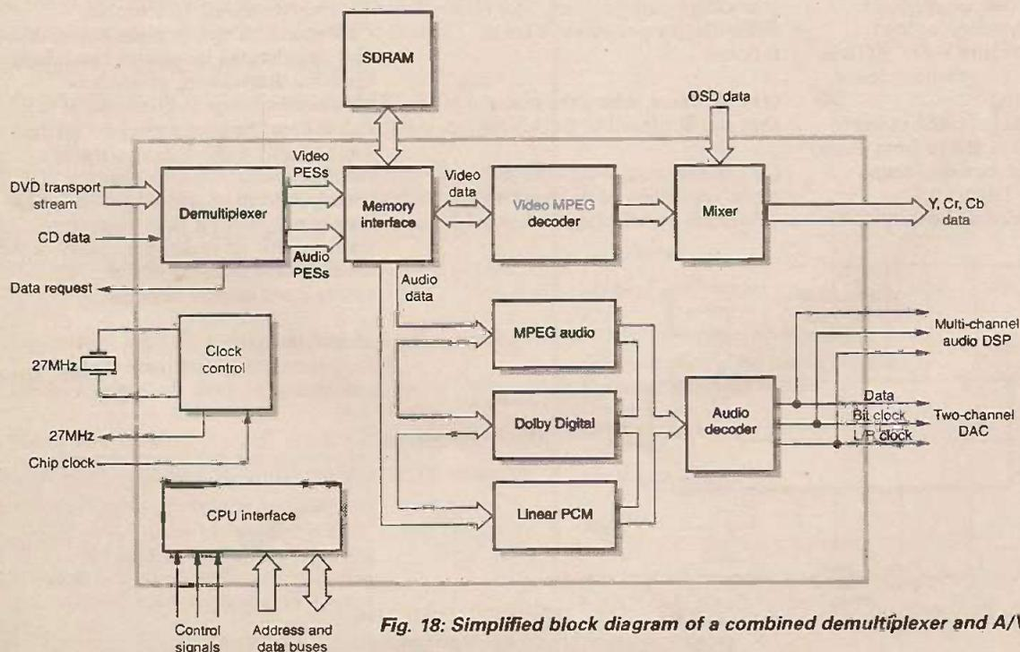
Fig. 18: Simplified block diagram of a combined demultiplexer and A/V decoder chip.
