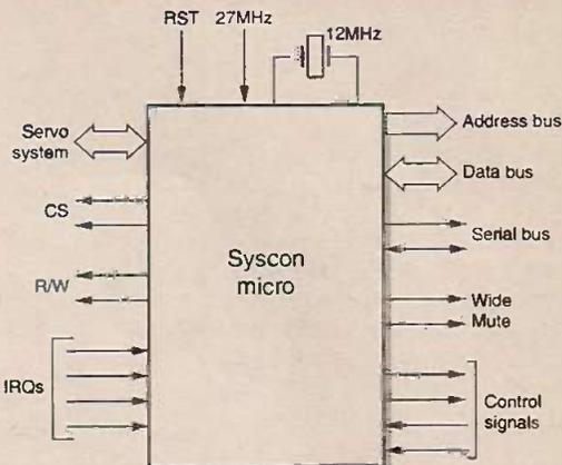
Fig. 17: Connections to a chip that combines the syscon microprocessor and gate-array functions.
