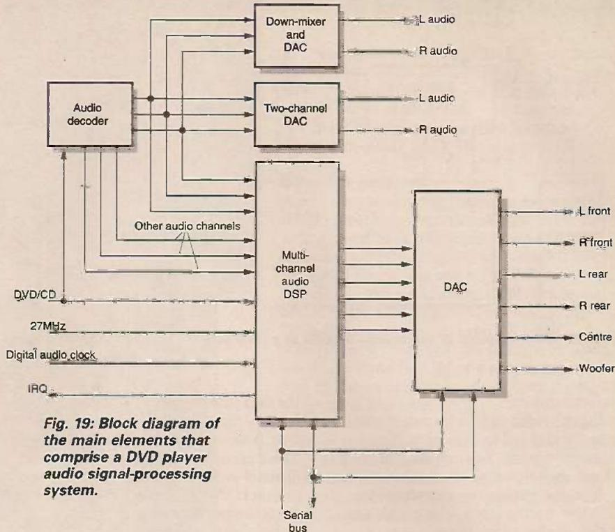
Fig. 19: Block diagram of the main elements that comprise a DVD player audio signal-processing system.
