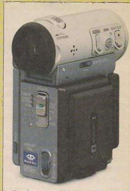
*Sony's DCR-IP7 camcorder is one of the first two models to use the company's newly developed MicroMV format. The cassettes are 70 per cent smaller than MiniDV standard cassettes. For further details see the Berlin Radio Show report, page 20.*
