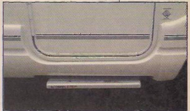
*The motorised step retracted for driving.*
