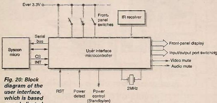
Fig. 20: Block diagram of the user interface, which is based on a dedicated microcontroller chip.
