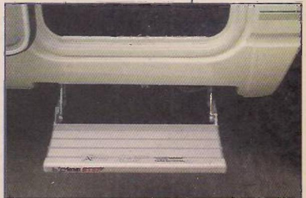
*The motorised step extended while the motor home is stationary.*
