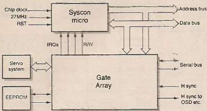
Fig. 16: Block diagram of the syscon section of a DVD player.
