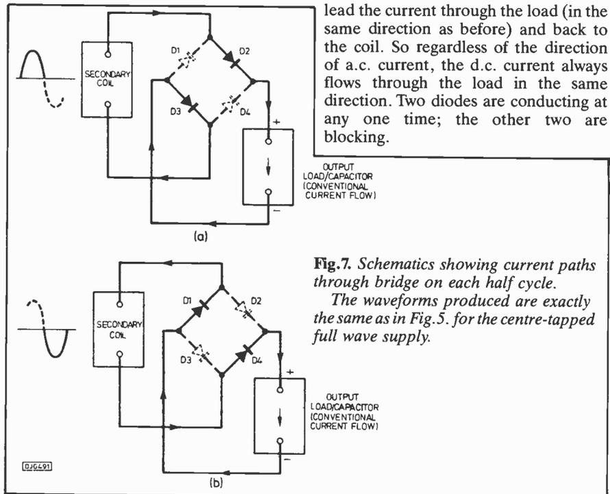
**Fig.7.** Schematics showing current paths through bridge on each half cycle.
