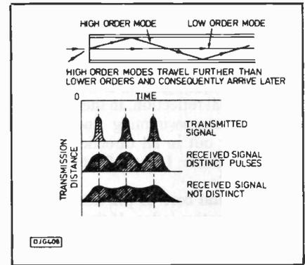
Fig. 12. Signal dispersion caused by multiple ray paths.
