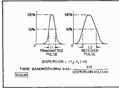
Fig. 11. Measurement of dispersion
