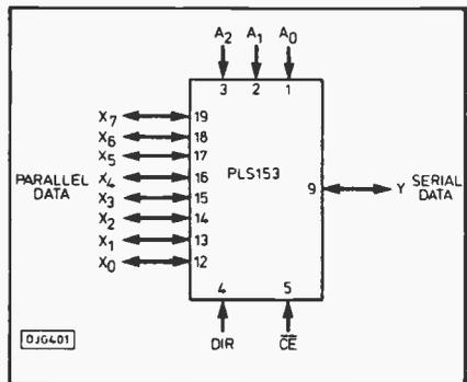
Fig. 14. FPLA 8:1 bidirectional multiplexer/demultiplexer
