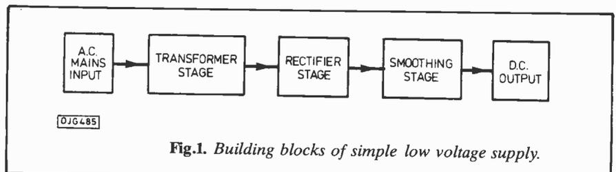
Fig.1. Building blocks of simple low voltage supply.
