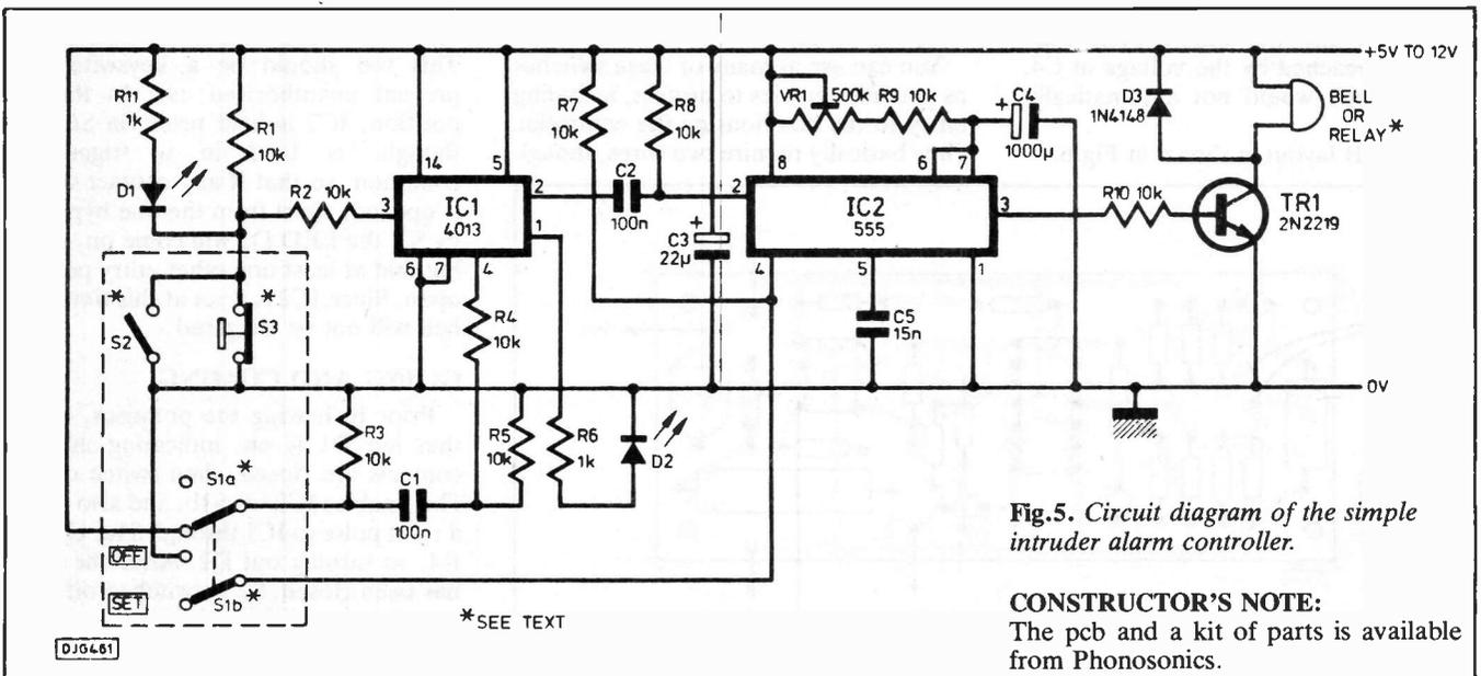
Fig.5. Circuit diagram of the simple intruder alarm controller.
