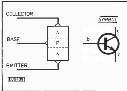
Fig. 3. Junction transistor.
