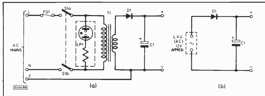
**Fig.2.** Half wave PSU. (a) Mains version. (b) Low V.a.c. version.
