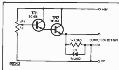
Fig. 12. A method of obtaining a variable output voltage
