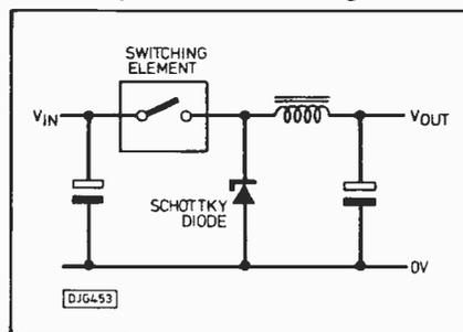
Fig.16. Part of switched mode power supply
