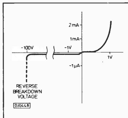
Fig.2. Diode characteristics.
