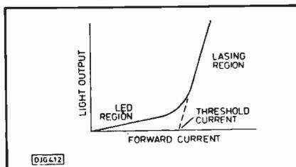
Fig.15. Output characteristic of a semiconductor laser
