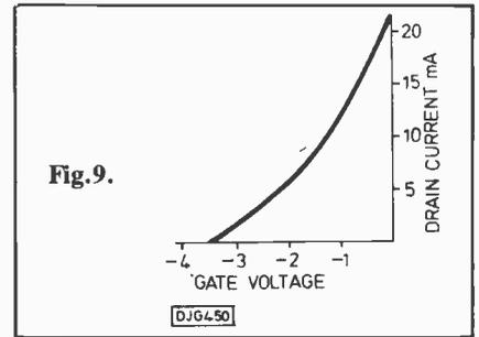
It is also possible to produce a f.e.t. which is normally in the non-conducting state, and which can be made to conduct by application of a gate voltage. In this case, the gate must be insulated from the channel, or else the gate-channel junction would be forward biased and gate current would flow.
