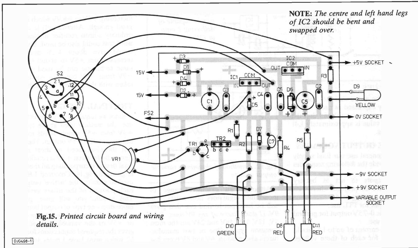
Fig.15. Printed circuit board and wiring details.
