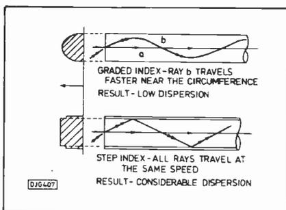
Fig.9. Transmission of graded and stepped index fibres
