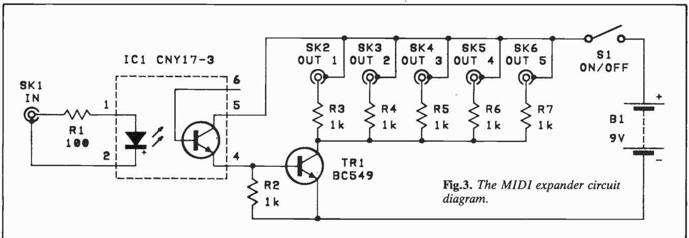
Fig. 3. The MIDI expander circuit diagram.
