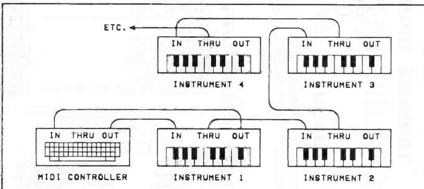
Fig.1. The "chain" method of connection
