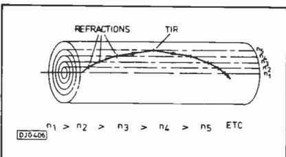
Fig.8. Stepped index model of a graded index fibre
