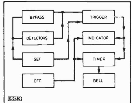
Fig.4. Block diagram of simple controller.
