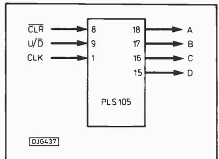
**Fig.16.** PLS105 FPLS as an up/down counter with clear.
