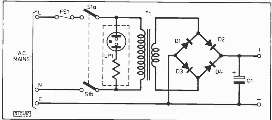
**Fig.6.** Basic bridge rectifier circuit (mains version)
