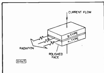
Fig.14. Schematic diagram of a semiconductor laser.
