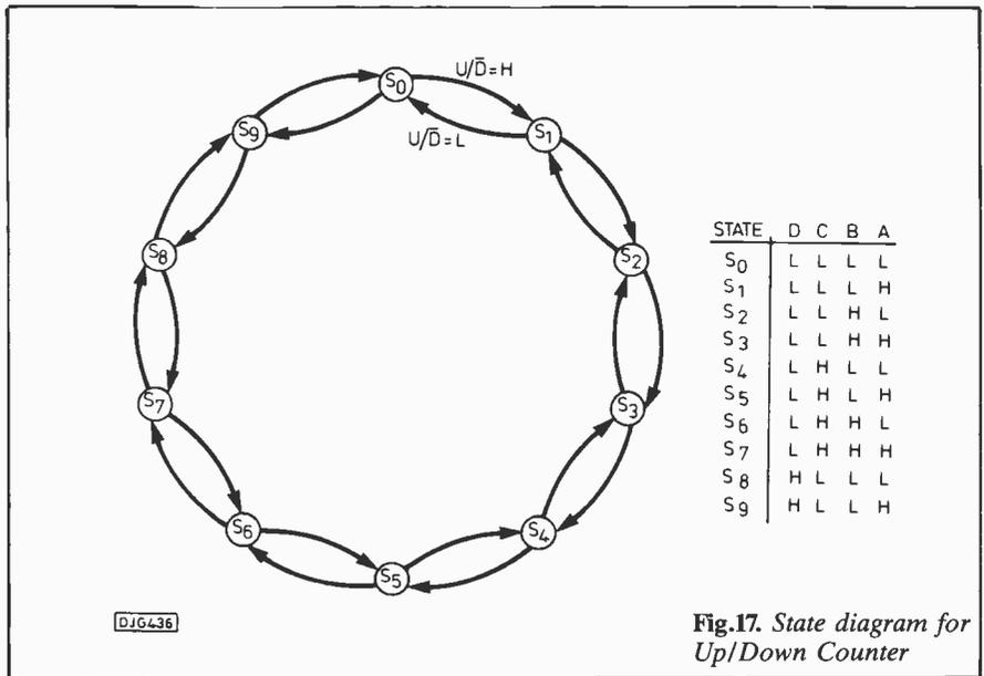
**Fig.17.** State diagram for Up/Down Counter
