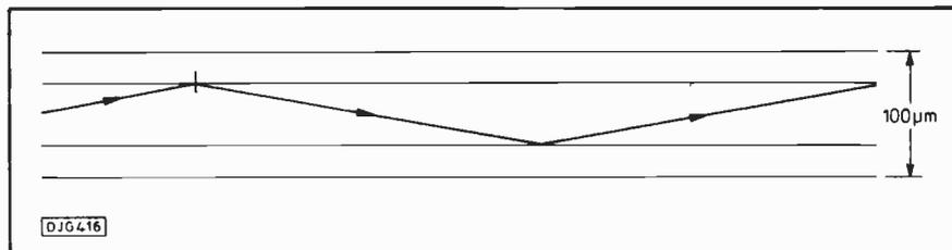
Fig. 3. Total internal reflection in optical fibre
