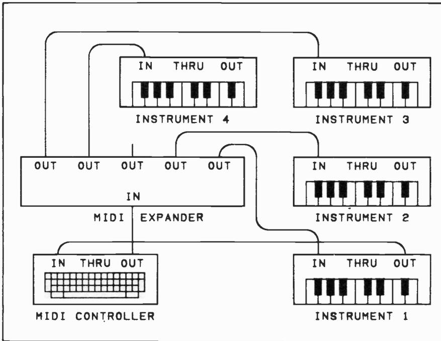
Fig. 2. The "star" method of connection.
