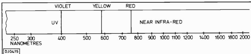
Fig. 2. Optical Spectrum
