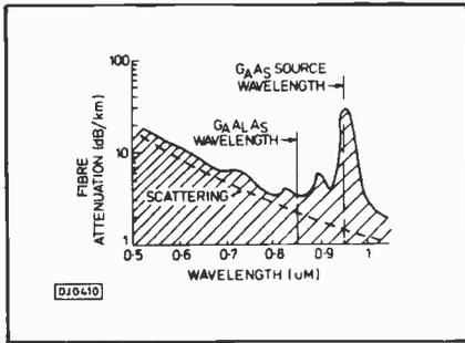
Fig. 10. Spectral response of a silica fibre
