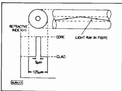
Fig.6. Monomode transmission
