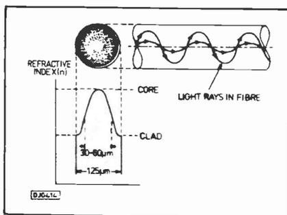
Fig.5. Multimode transmission
