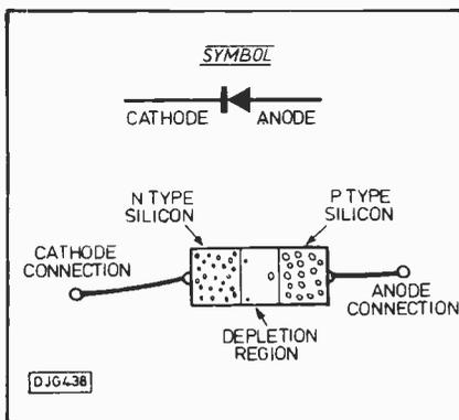
Fig.1. The diode
