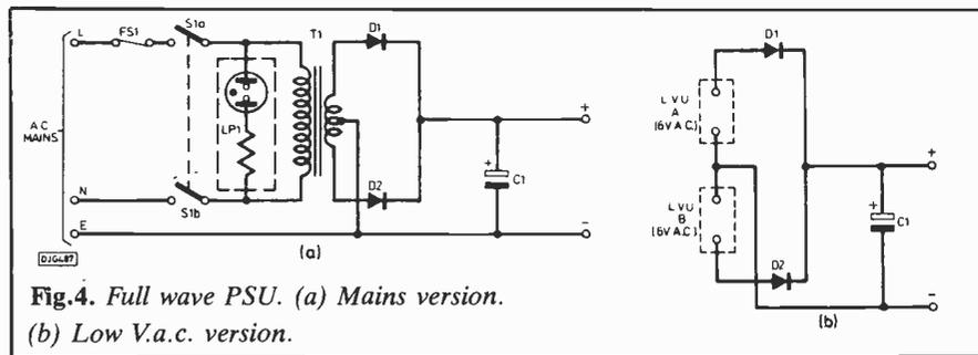
**Fig.4.** Full wave PSU. (a) Mains version. (b) Low V.a.c. version.
