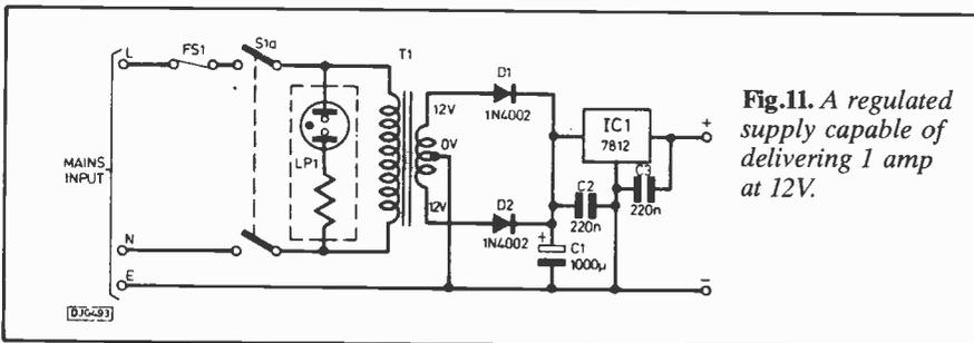
Fig. 11. A regulated supply capable of delivering 1 amp at 12V.
