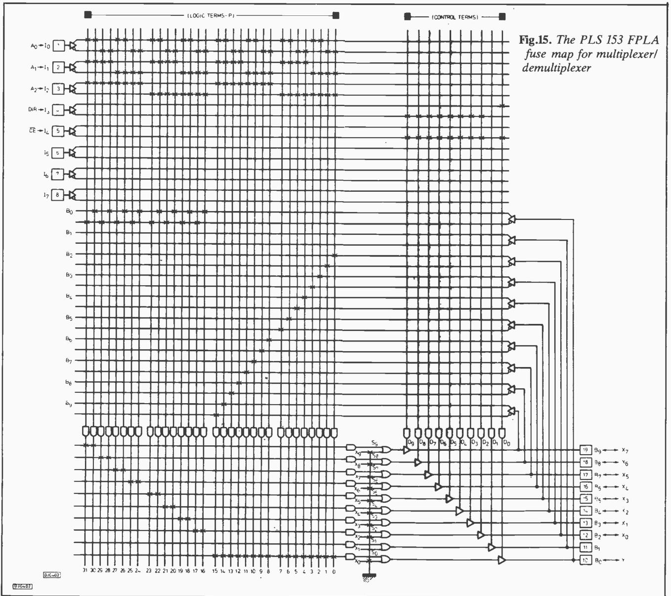
**Fig.15.** The PLS 153 FPLA fuse map for multiplexer/demultiplexer
