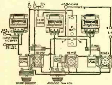
The Thordarson Autoformer, used as a straight impedance, makes an ideal coupling medium for the new Hi-Mu tubes UX-240 and CX-340.
