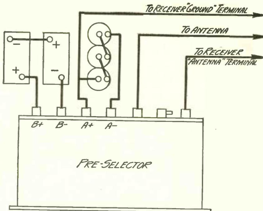
CONNECTIONS FOR THE USE OF SEPARATE BATTERIES
