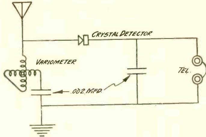
**A SIMPLE CRYSTAL CIRCUIT FOR A PORTABLE SET**
