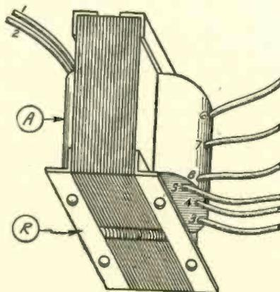
FIGURE 8: This drawing shows how the transformer leads are numbered and indicates the proper way to fasten the brass brackets to the core.
