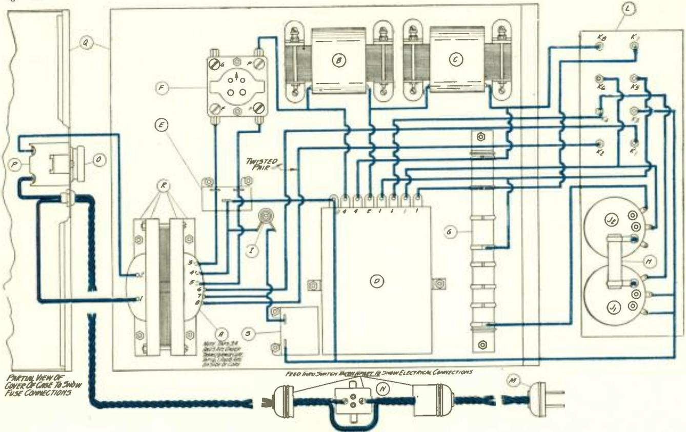
THE PICTURE WIRING DIAGRAM
