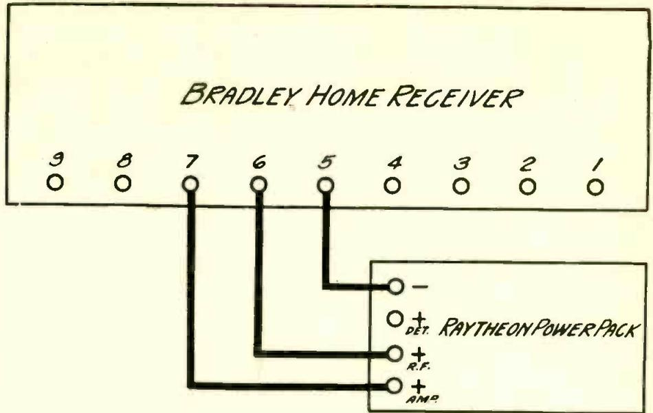
**CONNECTIONS FOR USING THE POWER-PACK**
