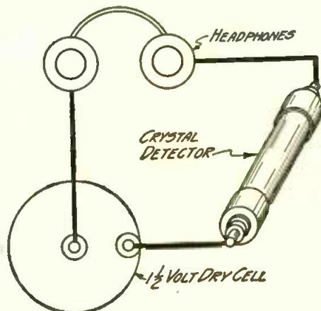
THE TEST FOR THE CRYSTAL DETECTOR
