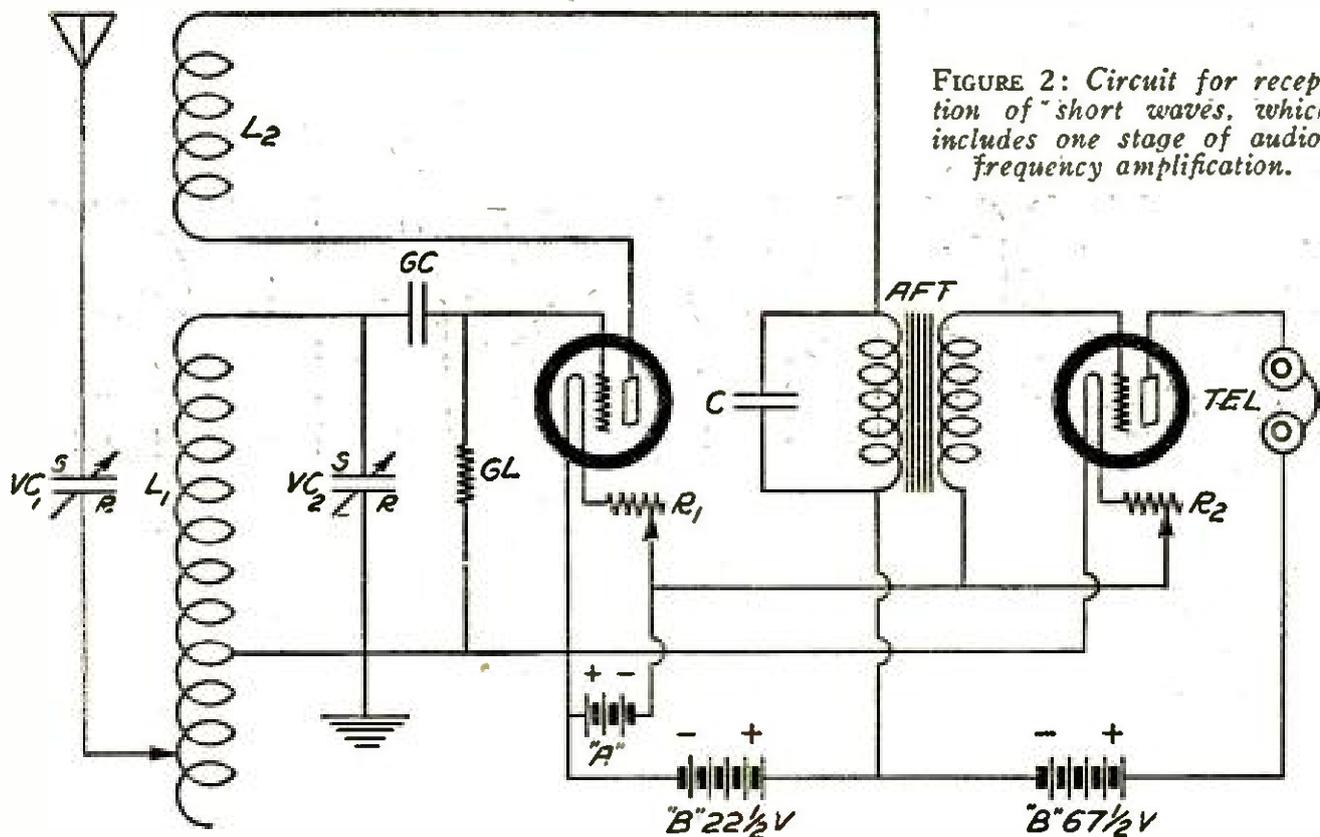
FIGURE 2: Circuit for reception of "short waves," which includes one stage of audio-frequency amplification.
