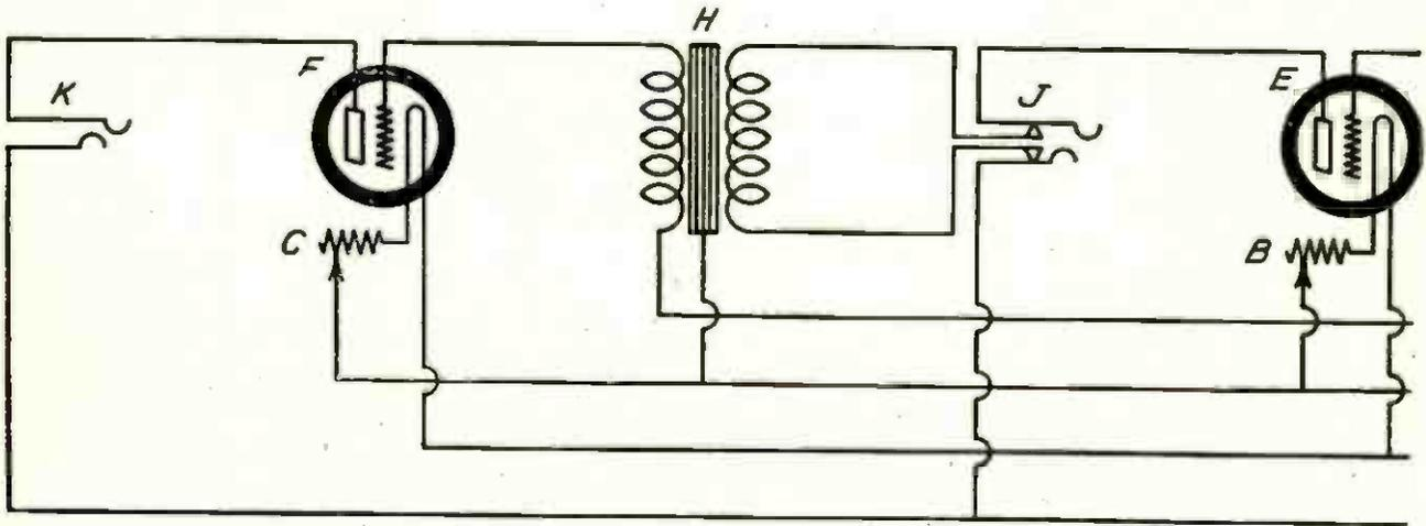
circuits in a cabinet separate from the tuner. For the man who is doing any considerable amount of experimental work, this construction is particularly good because it permits all kinds of tests to be made on the tuning unit without disturbing the detector-tube wiring or the audio amplifier.
