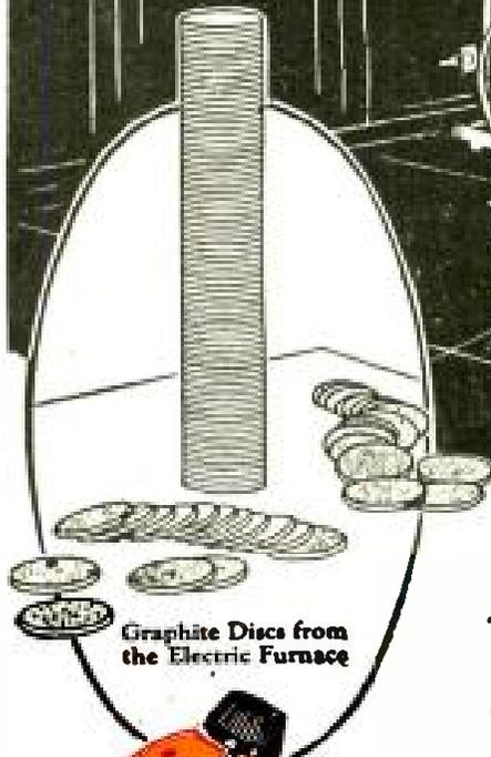
Graphite Discs from the Electric Furnace
