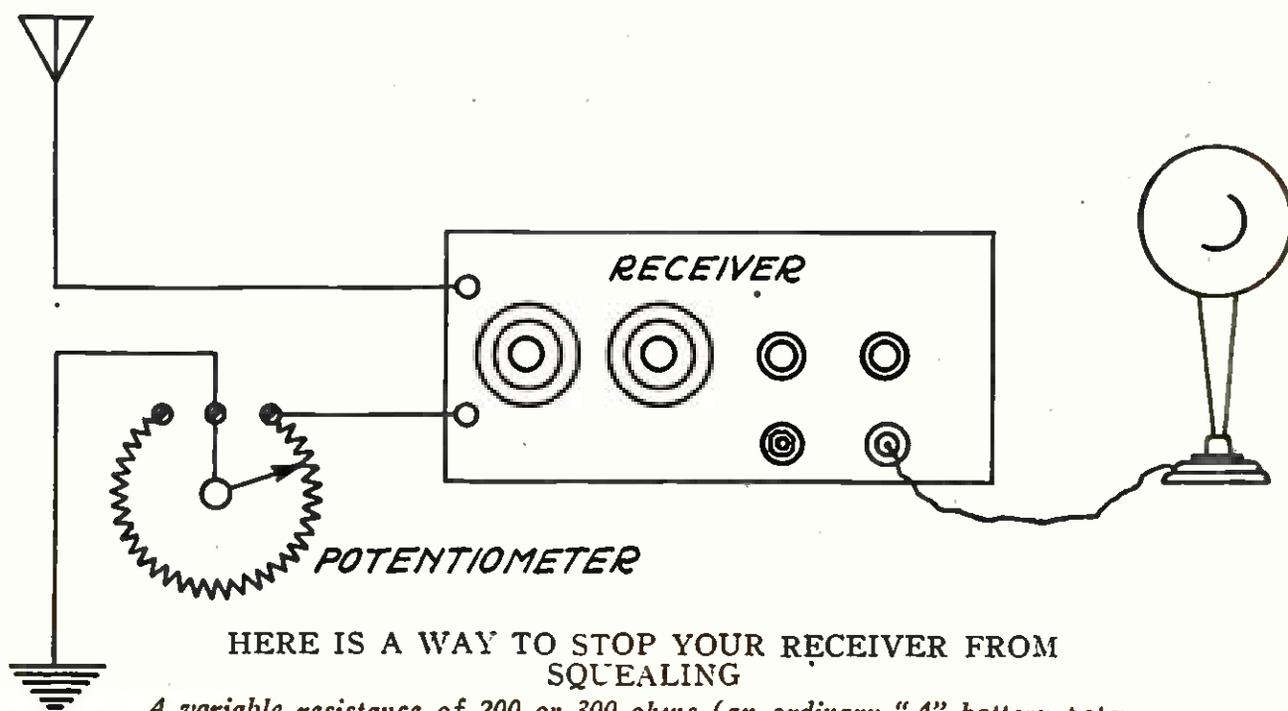
*A variable resistance of 200 or 300 ohms (an ordinary "A" battery potentiometer) connected in series with the ground lead can be adjusted to prevent the tendency of the receiver to oscillate on certain wavelengths.*
