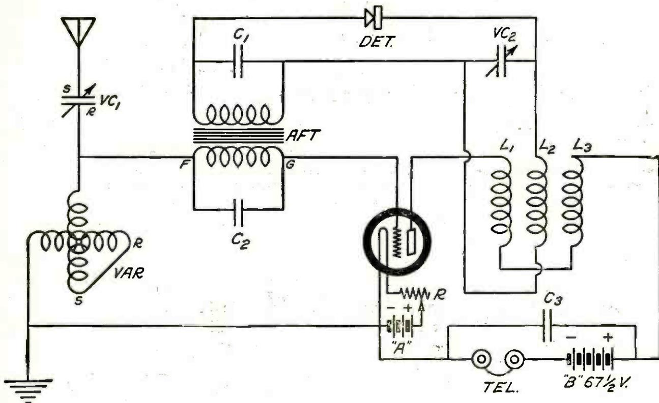
**SIMPLIFIED REFLEX WITH HONEYCOMB-COIL, RADIO-FREQUENCY COUPLING**
