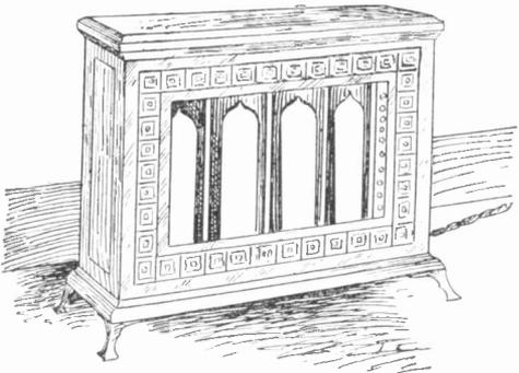
FIG. 7. ELECTRIC LUMINOUS RADIATOR
