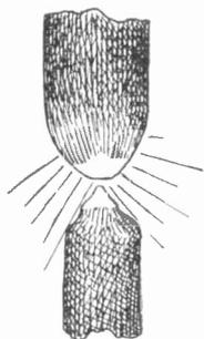
FIG. 2. ARC LAMP ELECTRODES
