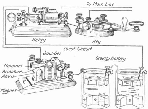
FIG 5. ESSENTIAL PARTS OF A TELEGRAPH CIRCUIT
