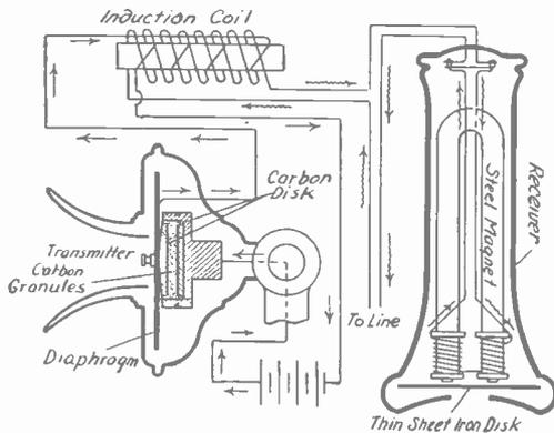
FIG. 4. ESSENTIAL FEATURES OF A TELEPHONE TRANSMITTER AND RECEIVER
