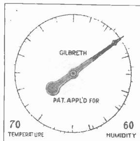
SPECIAL CHRONOMETER WITH LONG HAND MOUNTED BESIDE THE WORKMAN AND APPEARING IN EACH PICTURE OF THE FILM
