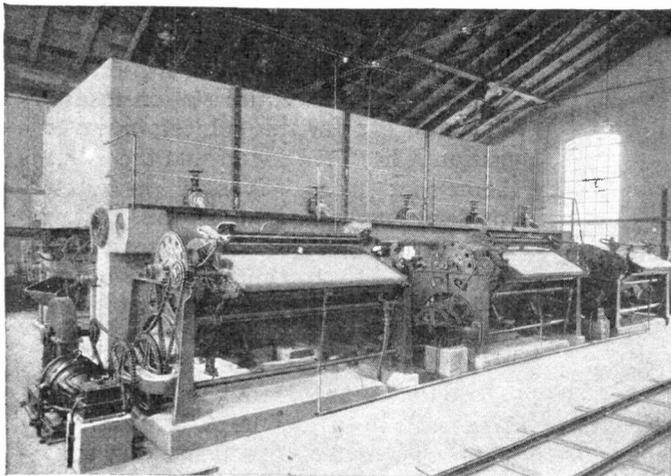
SEPARATOR WITH DISTRIBUTING TANKS BEHIND
