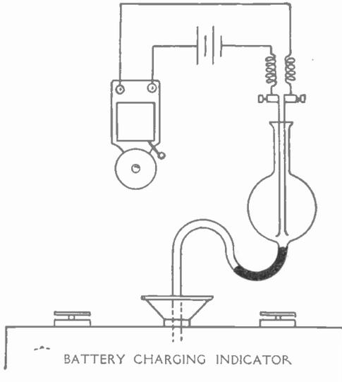
mercury is in connection with the space above the battery, which is enclosed. When the charging is complete and gas in excessive quantities begins to be given off, the pressure pushes the mercury in the tube until it forms a connection between two wires which form part of the circuit of an electric bell. A sort of safety valve is also provided for the escape of any accidental sudden pressure, caused for instance by the pressure of the stopper or by the sudden expansion of heated gas.
