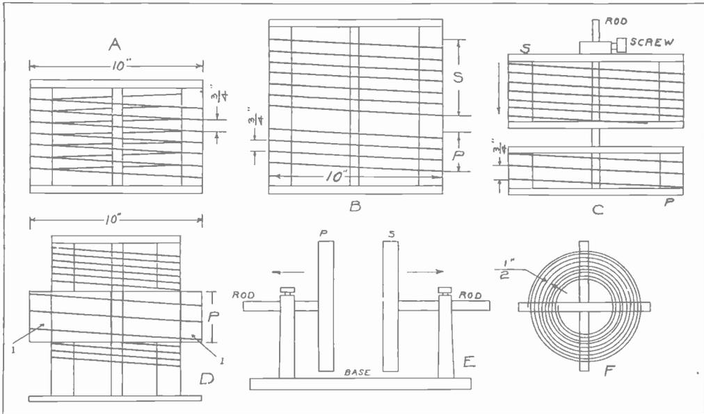
FIG. 6. TYPES OF OSCILLATION TRANSFORMERS
