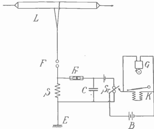
FIG. 2. CONNECTIONS OF STORM INDICATING SYSTEM
