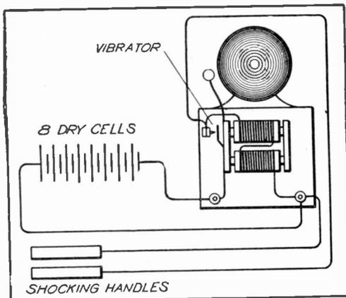
FIG. 2. SUBSTITUTE FOR SHOCKING COIL
