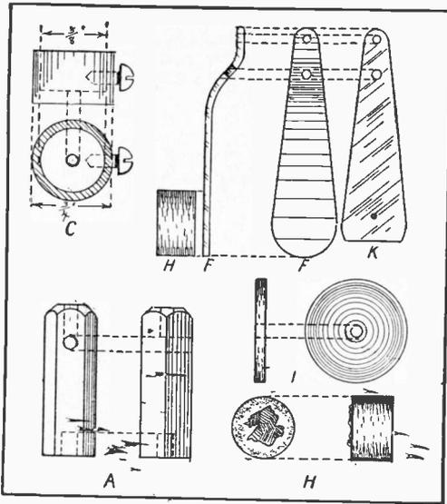
FIG. 2—DETAILS OF GALENA DETECTOR
