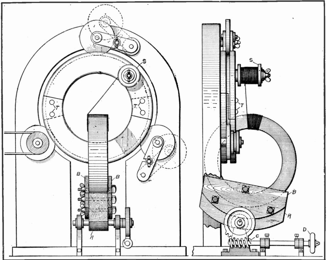
MACHINE FOR WINDING RING ARMATURES
