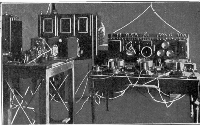
PRINTING TELEGRAPH (LEFT) TUNING FORK TRANSMITTER AND RECEIVER (RIGHT)
