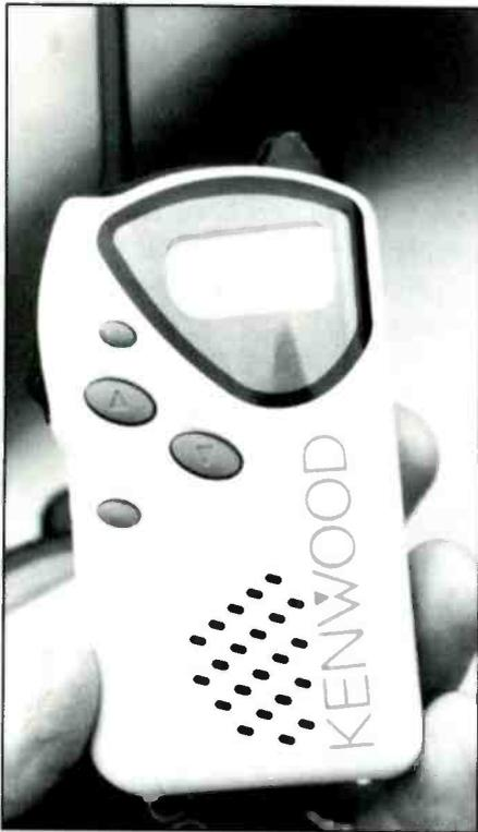
*Compact Family Radio Service (FRS) transceivers can communicate over 50 miles under the right conditions.*
