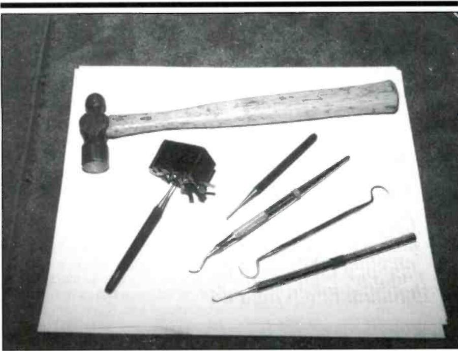
*Tools of the trade for successfully rebuilding the Philco block capacitors: 1/16 inch drift pinches, a 4 oz. hammer, and dental tools. Your dentist can supply you with worn instruments on your next visit.*
