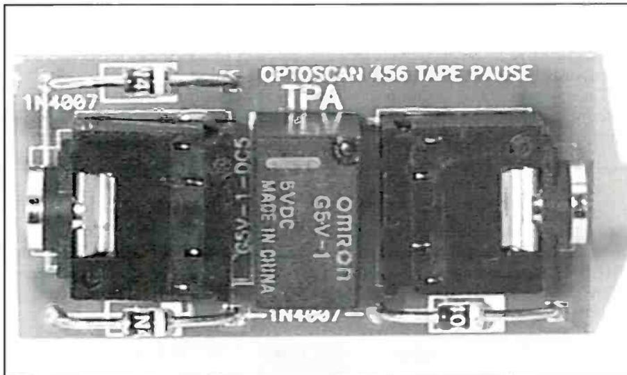
*The OS-456 Tape Pause Adapter. You will need this if you're using an OS-456 interface and controlling a tape recorder with the software. If using a VOX recorder, there is no connection to the OS-456 tape remote jack.*
