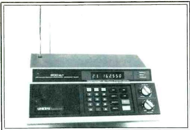
Many better grade modern scanners, such as this Bearcat 800XLT can receive frequencies higher in the spectrum than the old 512 MHz UHF-T band limit. Converters are also available to permit older scanners to receive various frequencies above 500 MHz.
