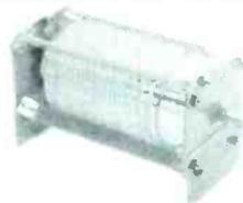
High quality roller inductor used in 1 KW HF transmitter; 21 non-linear turns of 0.25" silver-plated ribbon which forms 4.75" Lx3.63" dia coil, approx. 21 UH. Fiberglass end-plates; shaft 1" Lx0.375" dia. O/a 8.75x4x5, 3 lbs sh. Harris #938-0505-001, NEW .....\$45.00
