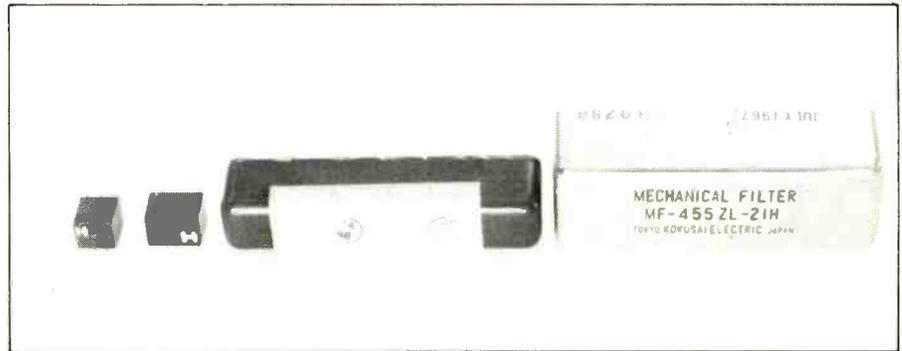
Figure 1. Here are some various IF filters showing old and new mechanical style filters and ceramic types.
