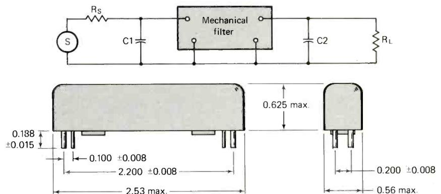
Termination circuits should be designed to eliminate DC currents and voltages from the filter. Satisfactory results may be obtained with current up to 2 ma DC, but in no case to exceed 3 ma DC. DC voltage should not exceed 100 volts DC.
