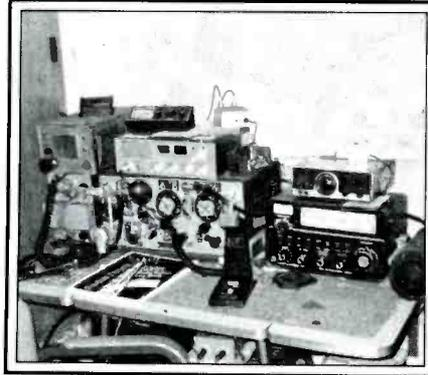
Shown left-center atop the desk in this photo of the station operated by Floyd in Corpus Christi, Texas, is an old WWII mil surplus rig called the MARK II. This was designed and built in the U.S. for export use in the USSR (in tanks). It operates on the HF bands as well as UHF but is a monster to convert to civilian use, especially since all of the writing on the front panel is in Russian!
