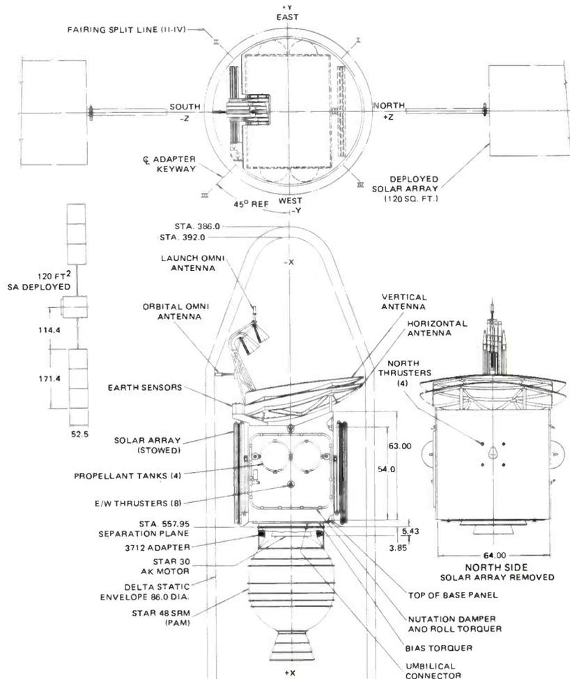
Figure 3. Advanced RCA Satcom general arrangement drawing. (Courtesy of RCA Government Systems Division)
