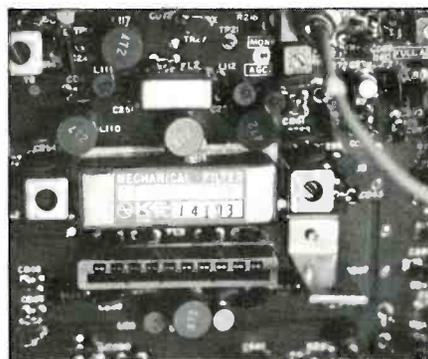
Figure 2. This is the mechanical as placed in the Japan Radio NRD-515 communications receiver.
