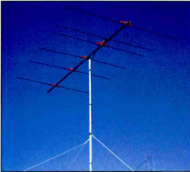
Photo F. The six-element 50 MHz OWA, working DX from the W6ZE 2007 Field Day site in Los Alamitos, California.
