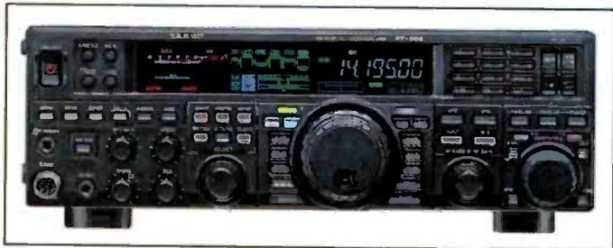
Yaesu's FT-950 transceiver features a triple-conversion, super-heterodyne receiver with selectable first-IF roofing filters of 3, 6, and 15 kHz.
