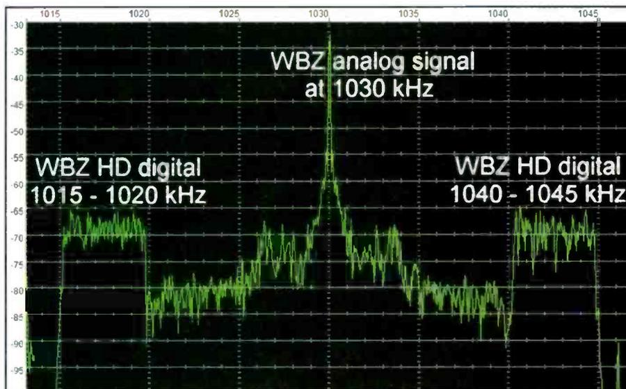
*This is what the WBZ daytime analog and digital signals look like on a spectrum analyzer.*
