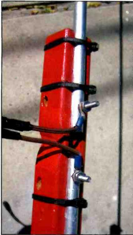
Photo E. Detail of the driven element and the attachment of the leads from the 1:1 balun connected to your coaxial cable.
