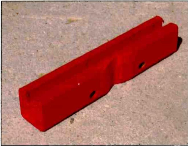
*Photo A. This is the finished mount for an element. Note the square lengthwise slot that will help hold the element level and the curved cutout that helps hold the mount snugly on the boom.*
