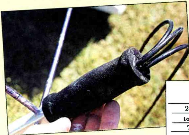
The duplexer slides up into the handle with pre-assembled coax cables and connectors.
