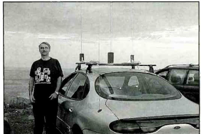
*Mark Connelly and his loop versus whip phased antenna array mounted on the roof of his car. The loop is aimed east over the Atlantic Ocean.*
