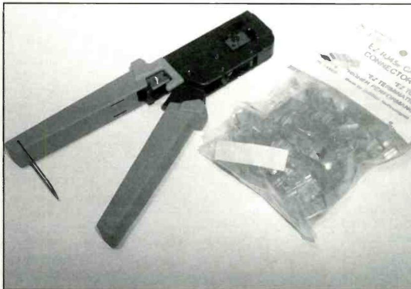
*Every now and then a product comes along that solves a perennially annoying problem in an elegant fashion. When it comes to making LAN cables, putting the connectors on each end is easy with the EZ-45 crimping tool (with matching connector bodies). For information on making LAN connectors as easy to install as modular telephone connectors, check out the Action Electronics web site at [www.action-electronics.com/ez45.htm](http://www.action-electronics.com/ez45.htm).*
