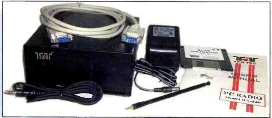
*This is what you get when you open the cardboard box that ships your RX320. The only thing not shown is the phono plug you can use to attach an external antenna to the receiver.*
