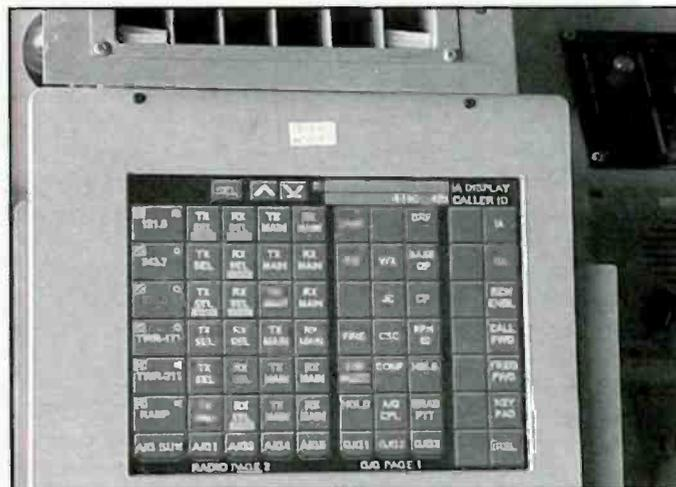
*The touch-screen radio control panel used by the air traffic controllers at Eielson AFB.*
