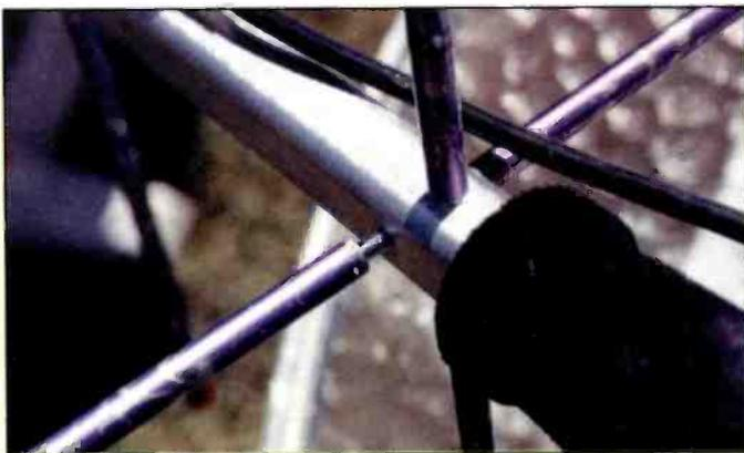
The Arrow antenna elements screw into place
