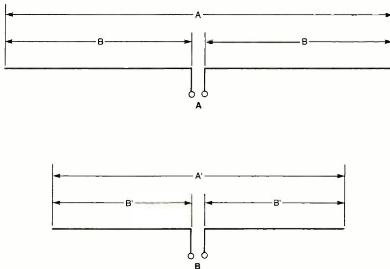
Fig. 1A. 40-meter dipole, Fig. 1B. Scaled-down 30-meter dipole.
