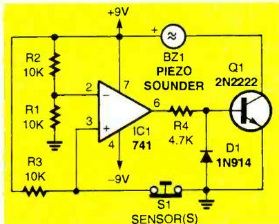
Fig. 4. This voltage-sensing circuit uses a standard op-amp to sound a buzzer when the external sensor(s) path opens up.
