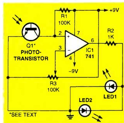
Fig. 3. Here's a neat light-operated sensing circuit. In the absence of light on photo-transistor Q1, LED2 lights. When light impinges on Q1, the op-amp switches current to turn on LED1.
