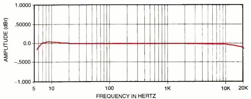
Fig. 3. The frequency response of the DVD-A300U is virtually ruler-flat over the entire audible audio range.
