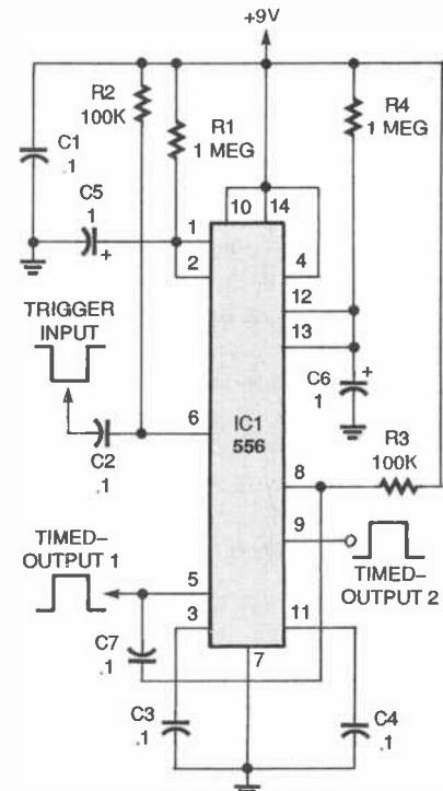
Fig. 2. Two are sometimes better than one. This dual timer contains a 556 IC, which contains two 555 timers in one package.
