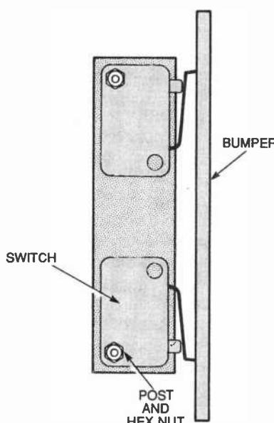
**Fig. 9.** Here's an overhead diagram of the bumper-switch assembly. The switches pivot on their mounting bolts when the bumper is hit.
