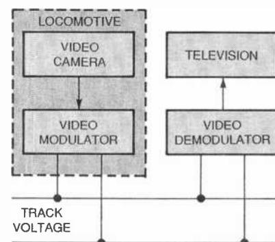
*Fig. 4.* In the Lionel Rail Scope system, a miniature electronic video camera is mounted inside a toy train. The video signal is transmitted from the locomotive over the rails to a receiver that is also connected to the rails.
