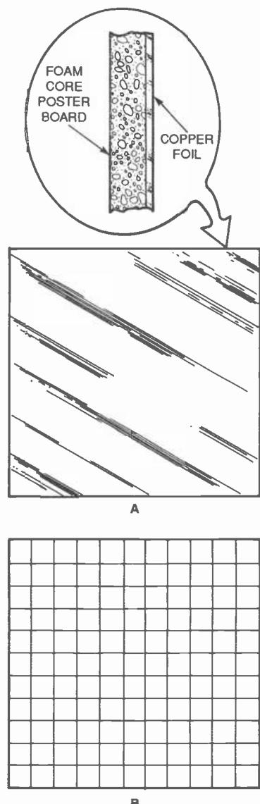
Fig. 7. The reflector plane can be made from a variety of materials. For example, copper foil over a wood, plastic, or foam-core poster board (A) or a wire grid made of #12 solid wires, or metal rods (B).
