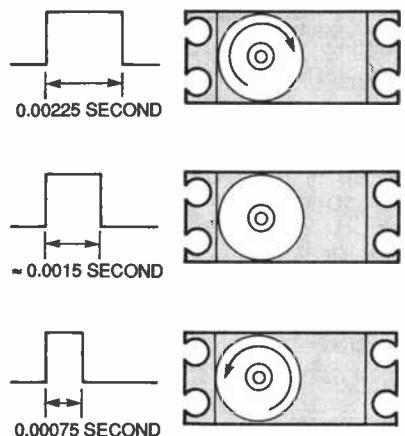
**Fig. 7.** On a modified servo, pulse-width modulation controls complete circular motion.
