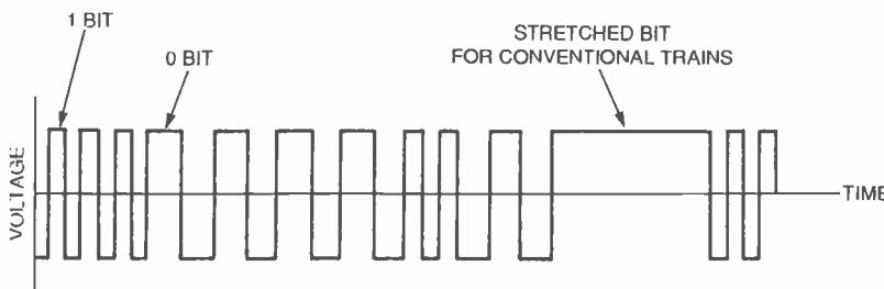
*Fig. 3.* As shown here, DCC is a pulse-width modulated system. Controllers transmit power and data in the same signal, and a decoder aboard the locomotive then extracts the information.
