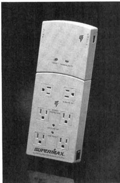
Supermax includes "ground OK" and "line fault" diagnostic lights, an always-on outlet, a master on/off switch, and a six-foot power cord. It has six receptacles plus two modular phone jacks. The Supermax offers an automatic or manual reset when voltage returns to a safe range. It also has a thermal fuse that, in the event of extended overvoltage, shuts off power to connected equipment.
