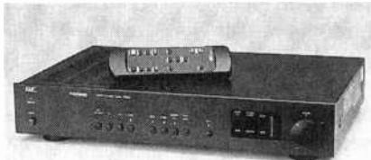
By pressing the LLC button on either the remote control or front panel, the LLC circuit corrects all channels when volume markings fall below 12 o'clock on the level. The LLC circuit adjusts each channel progressively in both amplitude and frequency, so there is no loss of the Dolby sound field when volume is reduced.
