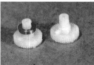
*Fig. 5. The bullgear on the left (with the bearing) has had its tab removed, while the bullgear on the right is unmodified.*
