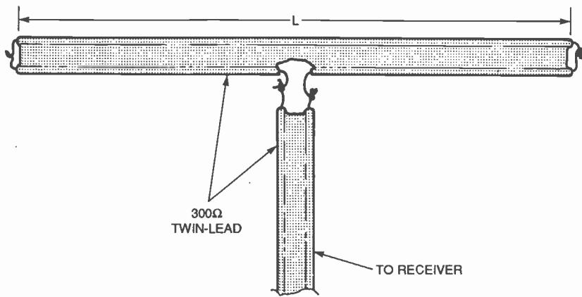
*Fig. 3. TV-type 300-ohm twin-lead is ideal for making a folded dipole. Be sure to short the conductors together at both ends as shown.*
