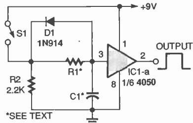
Fig. 4. Want a simple timer at practically no cost? Depending on what parts you have on hand, you can build this circuit for less than a dollar.
