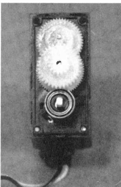
*Fig. 4. The servo geartrain is shown here, with the bull gear removed. Note that the clip is off the potentiometer shaft and the shaft is aligned lengthwise.*
