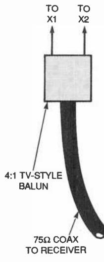
Fig. 9. The two bow-tie dipoles are connected together by a 400-ohm transmission-line harness (A). To use coax to connect to your rig, again use a 4:1 BALUN transformer.
