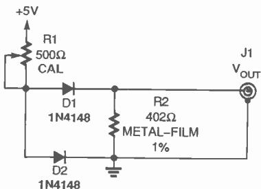
Fig. 7. This simple circuit uses two 1N4148 diodes to form a temperature-compensated millivolt reference.
