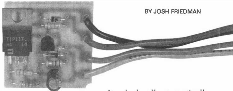
*It unlocks all automatically locking vehicle doors when you turn off the ignition.*
