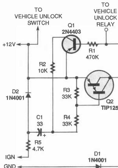
Fig. 1. When the *Unlock-Too* is connected to a vehicle, shutting the ignition switch off results in a forward biasing of Q2, which applies almost full car-battery voltage to the door unlock relay.
