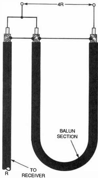
Fig. 10. If you do not want to buy a BALUN, one can be made from sections of 75-ohm coax cable.
