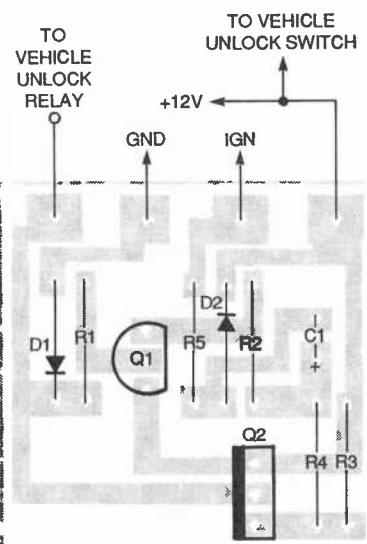
Fig. 3. When building the Unlock-Too on a PC board, use this parts-placement diagram as a guide.
