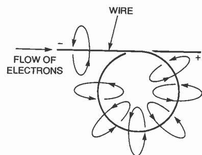
Fig. 3. In a loop of wire with current flowing through it, magnetic-field lines converge at the center and all point in the same direction.
