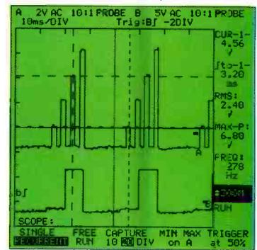
12:58 PM, Air Conditioner overheating. Resistance shows corroded connection.
