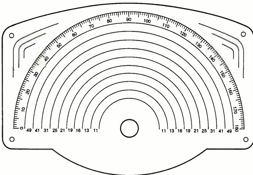
Fig. 6. The author started out with a blank tuning-dial pattern like this one, and added the appropriate frequency markings to the dial during the calibration procedure.
