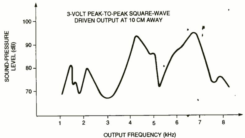
Fig. 7. Sound pressure level can vary greatly with even small changes in output frequency, as you can see from this graph.
