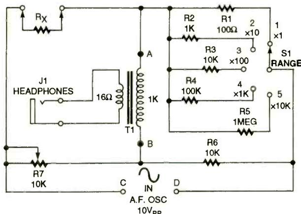
Fig. 3. When the Wheatstone Resistance Bridge is balanced, the voltage at pints A and B are equal, a null that can be detected ear is produces.
