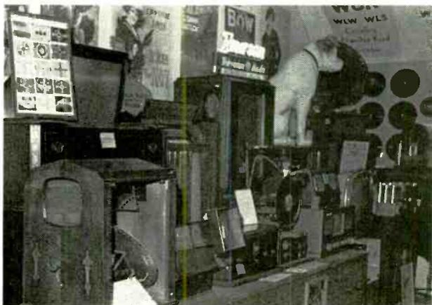
*The "television corner" featured a selection of early TV receivers. At the left is a very rare Jenkins 60-hole mechanical scanner; at the right, on the same counter (just below the big RCA "Little Nipper"), are a couple of small screen sets, including a working 3-inch Pilot. Note the projection receiver above the Jenkins.*
