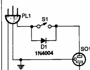
Fig. 6. This custom soldering-iron outlet can save your elements, tips, money, and time, and help save the environment. Pretty darn good for a one-evening project!
