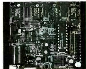
Two independently adjustable audio outputs are provided. One high-level output will drive an 8-ohm speaker to 400 mW; the other can be used for output to an external amplifier or transmitter. An on-board regulator allows use from 8 to 15 VDC. An open-collector output for keying a transmitter or external device during playback is also available, as is customizing.
