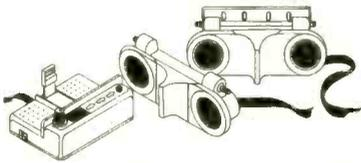
The ED-100 was designed for use as an auto/truck/RV back-up alarm. A digital display and audible beeper inside the vehicle inform the driver of the distance to impact beginning when the vehicle is within 14 feet of another object. Two 40 kHz ultrasonic emitter/detector modules, measuring 5.81" long X 1.9" wide, 2.05" thick, attach to the rear of the vehicle. The device operates on 12 or 24 Vdc.
