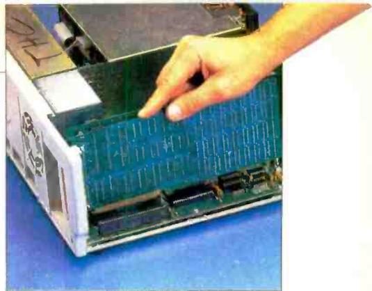
**The 1000 can accommodate three IBM-compatible expansion boards.**
