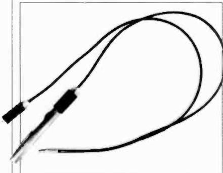
Light is injected into one branch of the Y where it evenly illuminates as pot directly below the end of the merged cables. Some of the light reflected from the paper enters the end of the merged fiber cable. Half this light travels up the side of the Y terminated by the photosensor.
