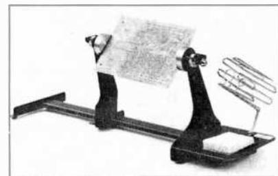
The PCBH-50 from OK Machine and Tool Co. is designed for use as a printed circuit board holder and solder station. The unit is spring-loaded for easy board removal and a self-locking end support adjusts to different board widths (up to 10" × 12"). A board can be rotated 360° and locked at any angle. Also included is a soldering iron holder and a cleaning tip sponge. The PCBH-50 can be either free-standing or mounted on a workbench.
