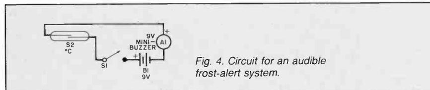
Fig. 4. Circuit for an audible frost-alert system.
