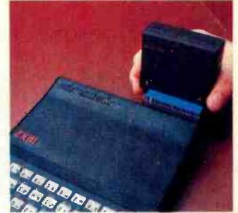
**16K MEMORY MODULE:** Like any powerful, full fledged computer, the ZX81 is expandable. Sinclair's 16K memory module plugs right onto the back of your ZX81. Cost is \$49.95, plus shipping and handling.
