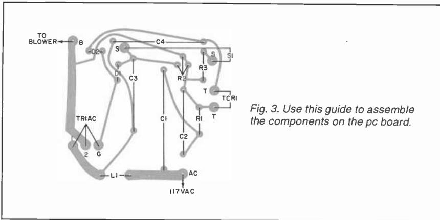
Fig. 3. Use this guide to assemble the components on the pc board.
