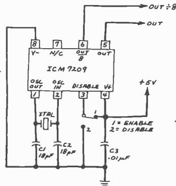
Fig. 8. Clock-pulse generator.
