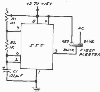
Fig. 5. Adjustable-frequency driver circuit.
