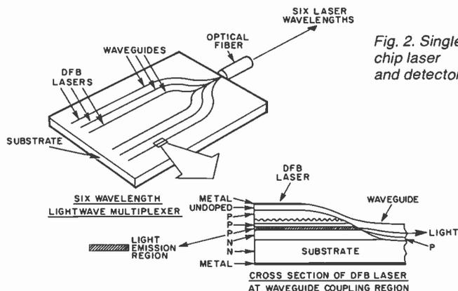
Fig. 2. Single-chip laser and detector.
