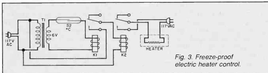
Fig. 3. Freeze-proof electric heater control.
