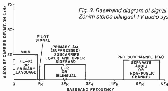
Fig. 3. Baseband diagram of signal in the Zenith stereo bilingual TV audio system.
