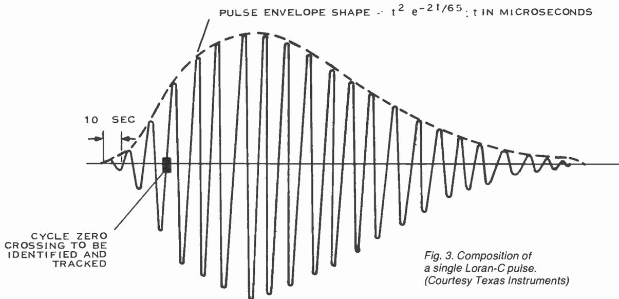
Fig. 3. Composition of a single Loran-C pulse. (Courtesy Texas Instruments)
