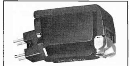
Shure Brothers has announced a new direct plug-in phono cartridge especially designed for use with linear-tracking turntables. Designated Model M96LT, it has a telescoped shank structure and a lightweight magnet reported to give a frequency response flat from 20 to 20,000 Hz. The cartridge has a bi-radial elliptical diamond stylus that tracks at 1.25 g. \$80.
