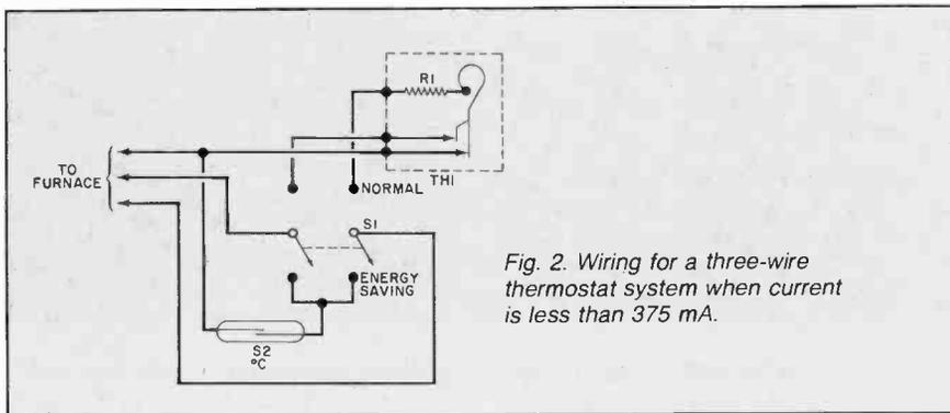
Fig. 2. Wiring for a three-wire thermostat system when current is less than 375 mA.
