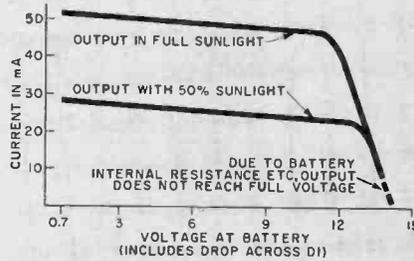
Fig. 3. Using a low-power solar charger on a digital meter having a 750-mA current requirement. The device is seldom used so the 50-mA output is adequate.
