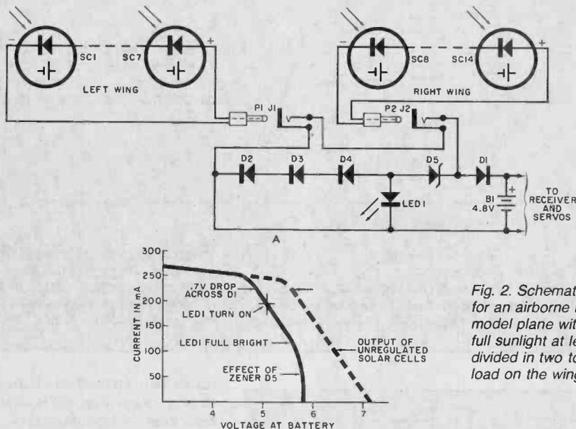
Fig. 2. Schematic of a solar charger for an airborne radio-control model plane with its output in full sunlight at left. The array is divided in two to balance the load on the wings of the plane.
