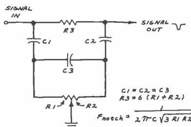
Fig. 1. A passive bridged, differentiator tunable notch filter.
