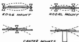
Fig. 2. Three mounting arrangements for piezoelectric alerter elements.
