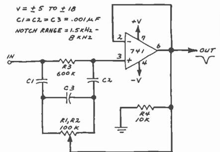
Fig. 2. Circuit for an active tunable notch filter.
