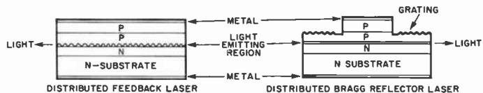
Fig. 1. Two kinds of semiconductor lasers suitable for photonic integrated circuits.
