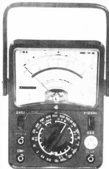
As a transistor tester, the instrument checks alpha from 0 to 0.9965 and beta from 0 to 285. Collector-to-base leakage current is checked in two ranges at 12 and 48  $\mu$ A full-scale for both npn and pnp transistors.
