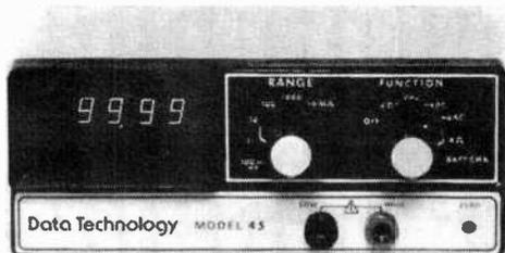
power supply and amplifier circuits. It has five ac and dc voltage ranges with 10- $\mu$ V resolution, six resistance ranges with 10-milliohm resolution, and five each direct and alternating current ranges with 10-nA resolution. The instrument will operate for 10 to 12 hours on fully charged batteries. Power consumption is 3 watts, and the 7-segment display measures 0.33" high. The calibration chart is silk-screened inside the case so that it cannot be mislaid. Price is \$399.
