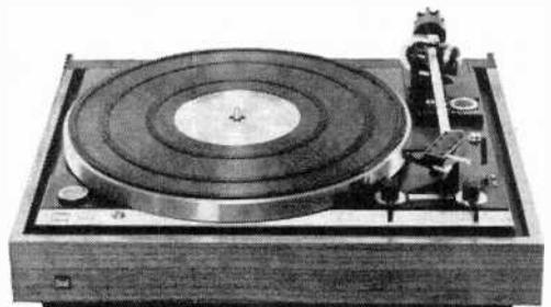
A stylus force gauge on the pivot structure is calibrated from 0 to 3 grams in increments of 0.1 gram up to 1.5 grams and 0.25 gram from 1.5 to 3 grams. The anti-skating compensation dial has two calibration scales (for conical and elliptical styli) that correspond to the tracking force in use. The cartridge mounts in a plastic insert, the latter supplied with a plastic jig that accurately locates the stylus for minimum tracking error.
