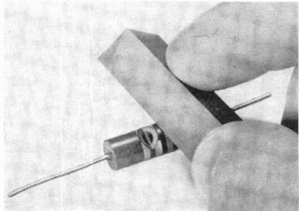
Fig. 4. The resistance of an ordinary carbon resistor can be trimmed by using a file.
