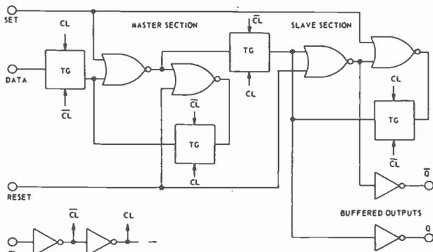
Fig. 6. Block diagram of one section of an RCA CD4013AE COS/MOS type D flip-flop unit.
