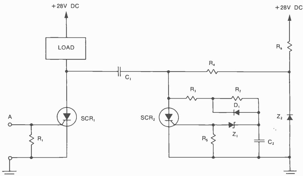
Fig. 1. Unitorde thyristor circuit for high-power interval timer.
