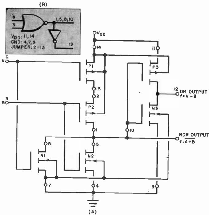
Fig. 2. A CD4007AE or CA3600E can be interconnected as shown to create NOR or OR logic (A). Symbol is at (B).
