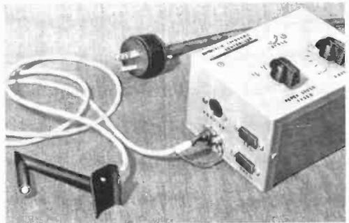
Fig. 3. Overall view of controller. Bracket which holds the LDR sensor is extreme left.
