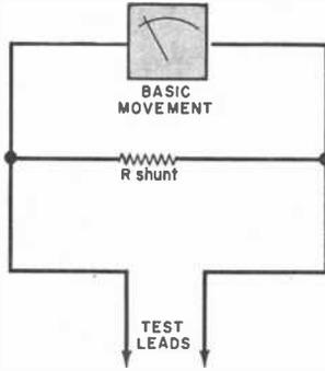
Fig. 5. The basic setup to be used for determining shunt resistor for an ammeter.
