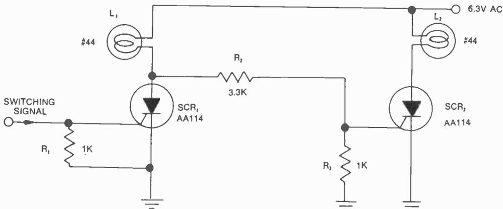
Fig. 2. Circuit for a complementary ac power switch using SCR's.
