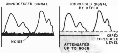
Fig. 4. Waveforms show how Kepex device effectively cancels leakage between mikes.
