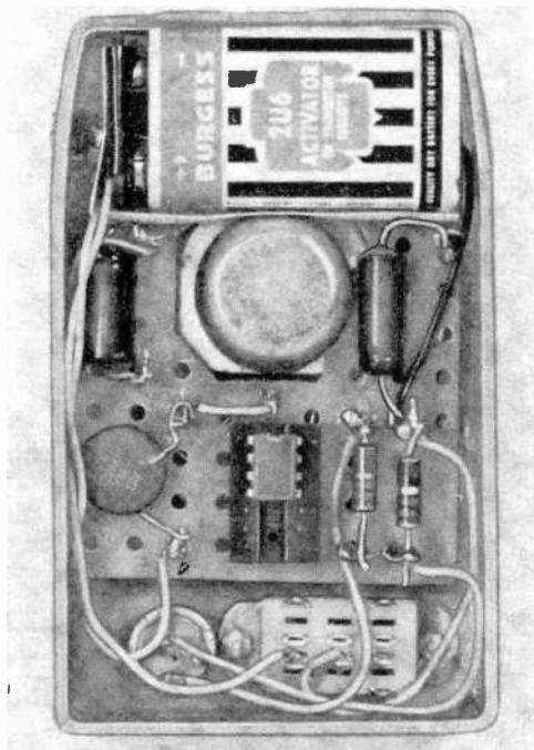
Photo shows how author's prototype, using perf board, fits in transistor radio case.
