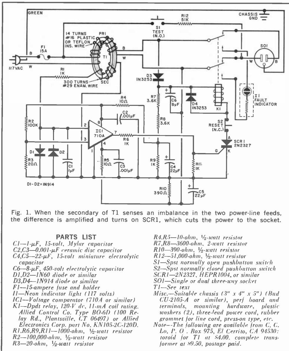
Fig. 1. When the secondary of T1 senses an imbalance in the two power-line feeds, the difference is amplified and turns on SCR1, which cuts the power to the socket.
