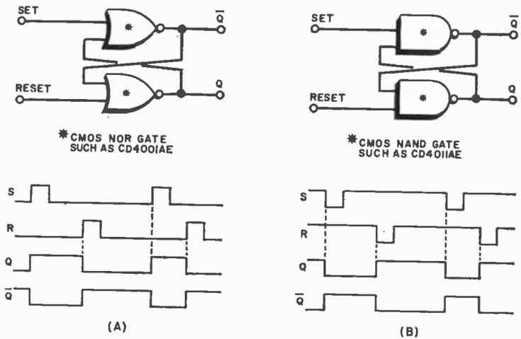
Fig. 5. Cross-coupled NOR gates respond to positive-going input signals (A) while cross-coupled NAND gates respond to negative-going.
