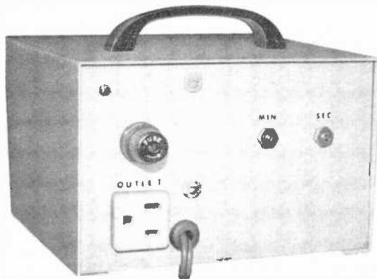
Mounted on the back panel are the power outlet, the fuse, and adjustments R2 and R3.
