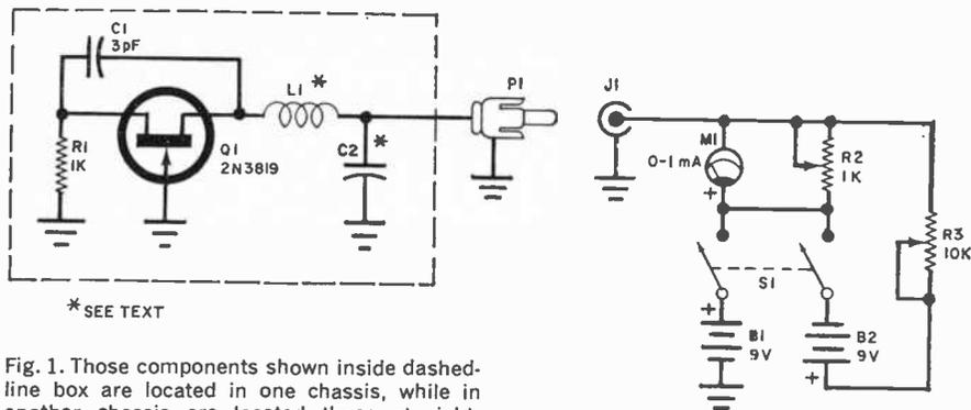
Fig. 1. Those components shown inside dashed-line box are located in one chassis, while in another chassis are located those at right.
