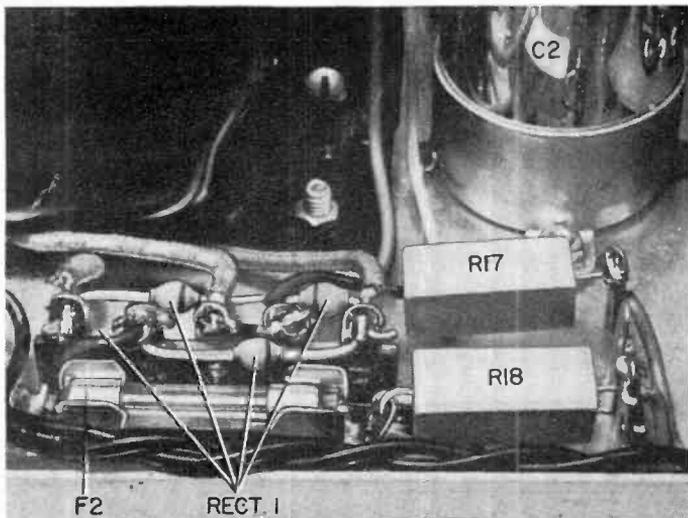
the power supply (see Fig. 4). Now, referring to Fig. 3, wire together the power supply circuit, using #18 or larger stranded hookup wire. (Note: Where #18 or larger wire is specified, do not substitute a smaller size wire. The circuits to which these wires connect carry as much as 10 amperes when the amplifier is driven to full power. If too small a wire size is used, power will be sacrificed and damping will suffer.)
