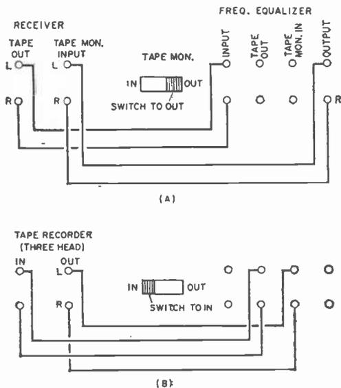
Fig. 5. Wiring diagram (A) shows how to connect equalizer to integrated stereo system. Diagram (B) shows how to make hookup for a tape recorder.
