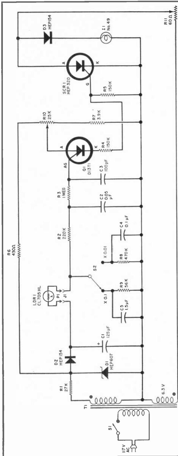
Fig. 1. The setting of R10 and resistance value of LDR1 (under various lighting levels) determine triggering time of Q1.
