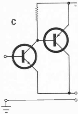
supply voltage. This simplifies design demands. Second, it is possible to keep distortion down to much lower levels in the driver circuit if it does not have to develop full supply positive and negative excursions. Additional temperature stability, by using 50 percent feedback in the output stage, is yet another advantage.
