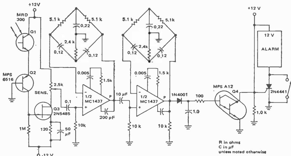
Fig. 2. Motorola-designed intrusion alarm amplifier/control circuit employs modulated light (source not shown) to foil burglars; Q1, sensitive to frequency-modulated light, is detector.
