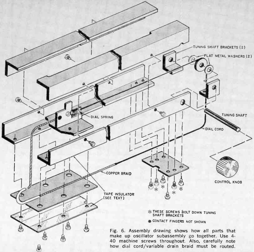
Fig. 6. Assembly drawing shows how all parts that make up oscillator subassembly go together. Use 4-40 machine screws throughout. Also, carefully note how dial cord/variable drain braid must be routed.
