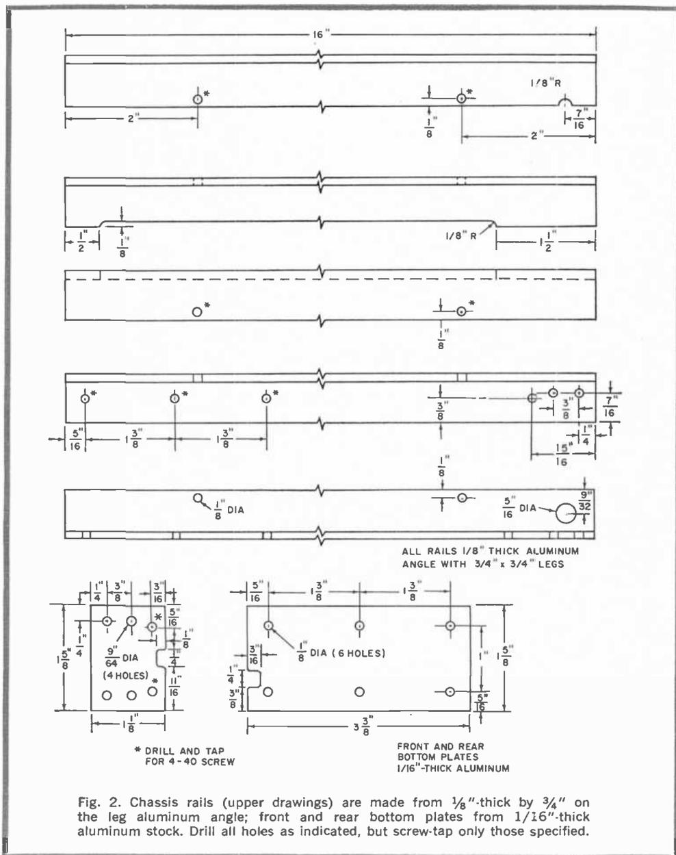
Fig. 2. Chassis rails (upper drawings) are made from  $\frac{1}{8}$ "-thick by  $\frac{3}{4}$ " on the leg aluminum angle; front and rear bottom plates from  $\frac{1}{16}$ "-thick aluminum stock. Drill all holes as indicated, but screw-tap only those specified.
