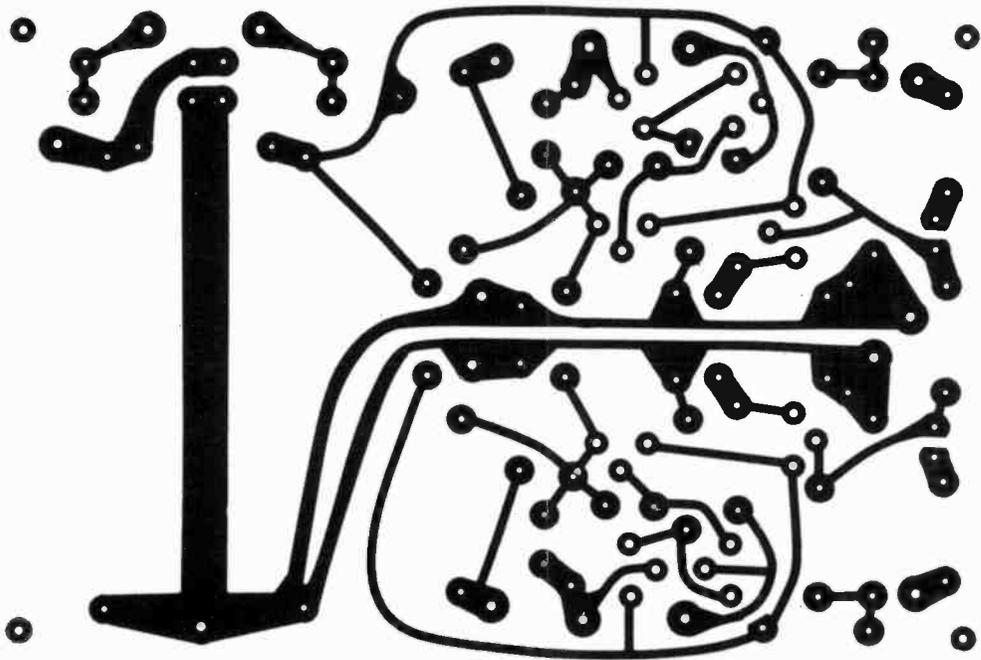
Fig. 2. This actual size etching guide can be used to duplicate circuit board used in original prototype. Dots in corners locate board mounting holes.
