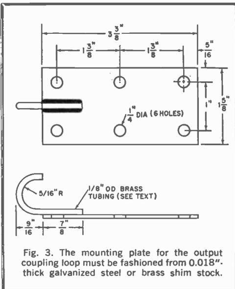
Fig. 3. The mounting plate for the output coupling loop must be fashioned from 0.018"-thick galvanized steel or brass shim stock.
