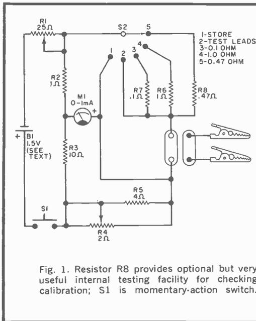
Fig. 1. Resistor R8 provides optional but very useful internal testing facility for checking calibration; S1 is momentary-action switch.
