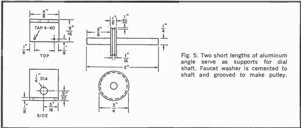
Fig. 5. Two short lengths of aluminum angle serve as supports for dial shaft. Faucet washer is cemented to shaft and grooved to make pulley.
