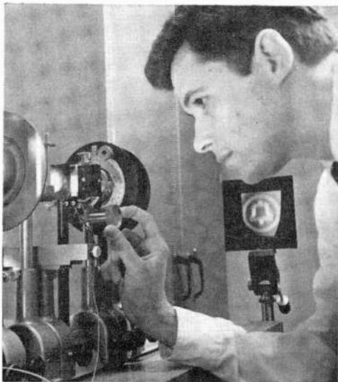
Bell Laboratories' Juan Maldonado adjusts focus of image from ferpic device on small viewing screen.
