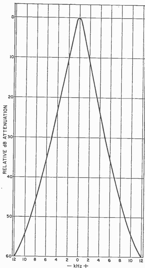
Clean symmetrical selectivity curve of the R-195 results from the use of ceramic filters in the i-f stages. Unfortunately, good selectivity cannot be used to maximum advantage due to poor bandwidth.
