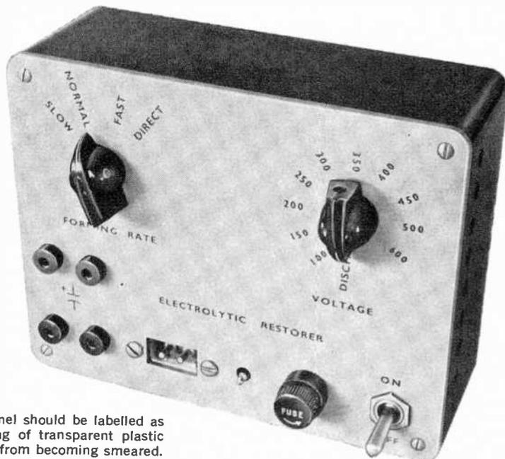
The finished front panel should be labelled as shown here. A coating of transparent plastic spray keeps lettering from becoming smeared.
