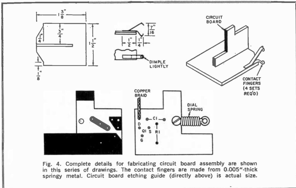
Fig. 4. Complete details for fabricating circuit board assembly are shown in this series of drawings. The contact fingers are made from 0.005"-thick springy metal. Circuit board etching guide (directly above) is actual size.
