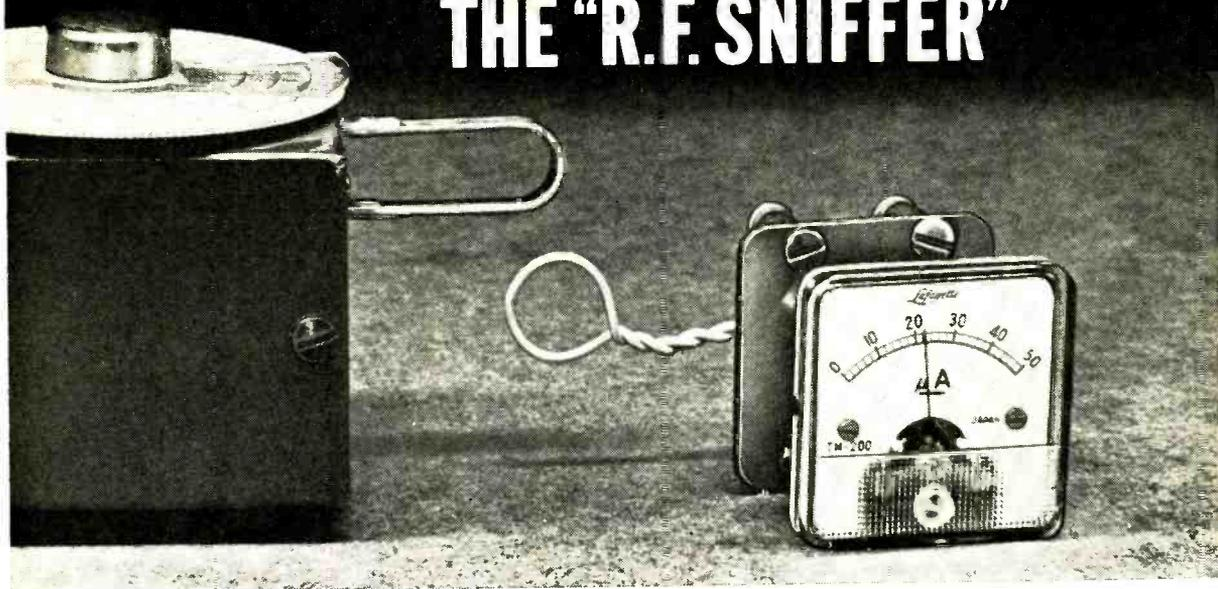
**N**O HAM OR CB'ER should be without some type of r.f. signal indicator for trouble-shooting and operating transmitters, r.f. amplifiers, and oscillators. A simple r.f. field strength meter fits the bill nicely. This device is almost as versatile in r.f. circuits as a multimeter is in d.c. and low-frequency a.c. circuits. Furthermore, it is easier to use and it is more compact than most multimeters.
