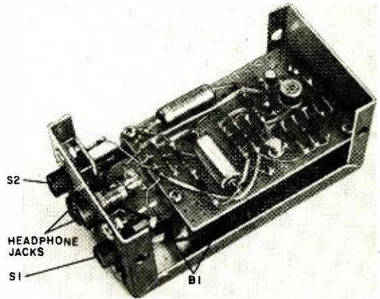
The two series-connected 9-volt batteries comprising  $B1$  are tucked away under the circuit board. The headphone jacks and switches are panel-mounted.
