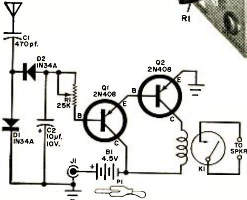
Parts layout and placement are not critical, but keep component leads as short as possible and neatly dressed.
