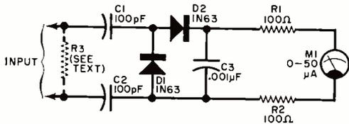
Fig. 1. Values shown for C1, C2 and C3 are for frequencies up to about 3 MHz. For higher frequencies, smaller value capacitors are required.
