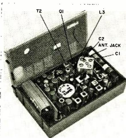
Spread FM oscillator coil *L3* as much as possible without breaking or shorting any components. Shift the FM broadcast band as far down as it will go by adjusting *C2*. Tune in a station at about 150 MHz and adjust *C1* for maximum volume. There is no need to make any other adjustments in the receiver.
