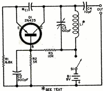
ary winding of a small 455-kHz transistor-type i.f. transformer. Capacitor C1 is a gimmick made of two 1-inch pieces of No. 20 cotton-covered wire twisted together. You can try a small 25-pF capacitor instead of the gimmick, if you wish. The leads should be twisted just enough to furnish a small amount of feedback and stable operation.
