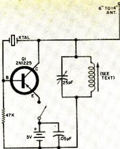
value of the resistor must be adjusted to suit the transistor—try a nominal value of 47,000 ohms; it will never be less than 10,000 ohms and rarely more than 75,000 ohms.
