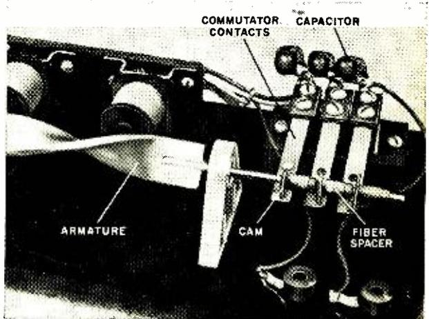
The armature is fabricated from a 5/8"-wide x 6"-long strip of 1/8"-thick soft iron twisted as shown in Fig. 4; aluminum or other non-ferrous metal *cannot* be used. You can start with a strip about 2' long. Put one end in a vise and attach a long wrench on the other end. Twist the strip until you wind up with 1 complete revolution (360°) within a 6" length. Mark this piece off and use a hacksaw to cut away the unused portions. Cut a notch on each end as shown.
