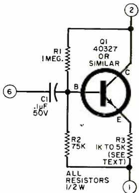
N.J. 07105. In addition, one of our readers has submitted the accompanying diagram for converting the circuit to eliminate the use of the 1LE3.
