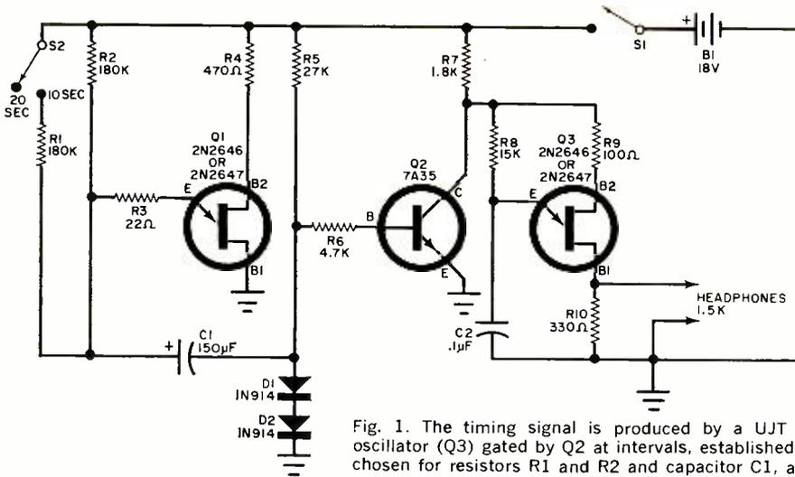
Fig. 1. The timing signal is produced by a UJT relaxation oscillator (Q3) gated by Q2 at intervals, established by values chosen for resistors R1 and R2 and capacitor C1, and by Q1.
