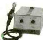
The workstation is engineered to meet the needs of today's electronic industry. Wide range of adjustments of air volume and temperature (212°F to 754°F) permits soldering of most surface mount devices. Comes with an A1138 nozzle QFP 28 x 28mm (1.1 x 1.1").
