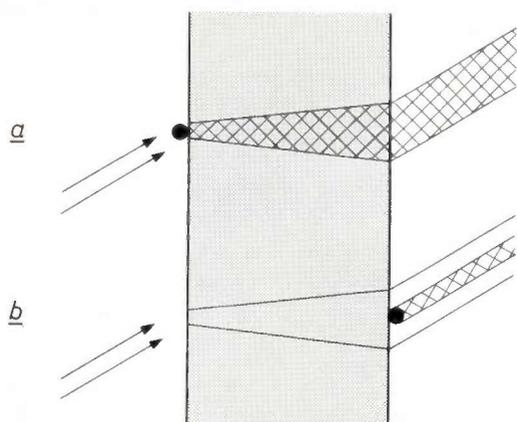
Fig. 12. Ray diagram showing formation of diffuse (a) and sharp images (b) for wires on front and back surfaces respectively.
