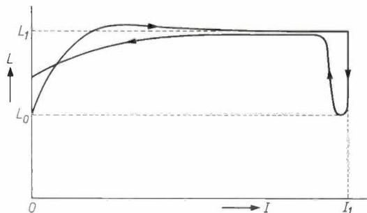
Fig. 6. When the current  $I$  through a superconducting coil is increased from zero to  $I_1$  and then returned to zero again, the inductance  $L$  varies in the manner shown by the curve. The value  $L_1$  is the inductance of a coil of normally conducting copper wire. The much lower value at low field strength and immediately after reversal of the current (minimum value  $L_0$ ) is due to the magnetization of the coil wire.
