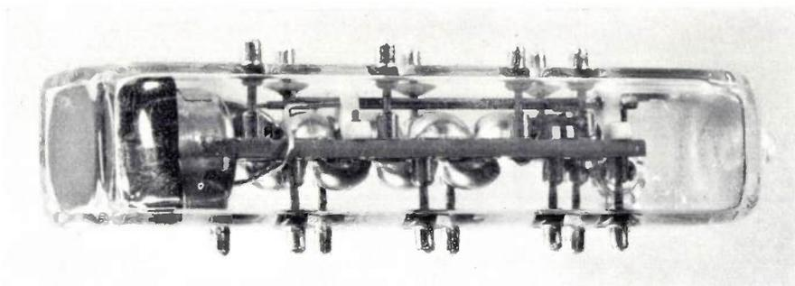
Fig. 21. Ruggedized version of the 152 AVP, type PM 400. Length 9 cm.
