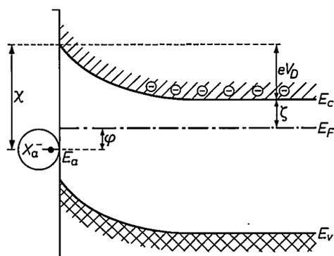
Fig. 8. As fig. 7, for the case where the negative surface charge is carried by adsorbed, strongly electronegative ions. The electrons then occupy a quantum state whose energy  $E_a$  is lower than  $E_F$  by an amount  $\varphi$ . The difference  $\chi$  between  $E_c(0)$ , the value of  $E_c$  at the surface, and  $E_a$  is independent of  $E_c$ : if  $E_c(0)$  rises as a result of an increase in the band curvature ( $eV_D$  greater) then  $E_a$ ; also rises and  $\varphi$  becomes smaller.
