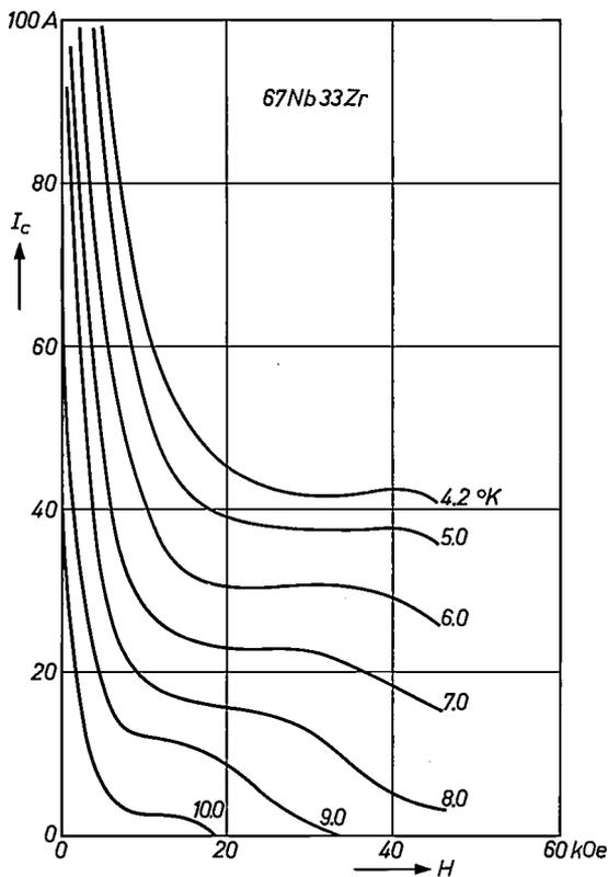
Fig. 4. The critical current  $I_c$  at various temperatures as a function of the magnitude  $H$  of the magnetic field for short samples of a given type of wire (67Nb33Zr,  $\frac{1}{4}$  mm dia.). The transition temperature of this material is between 10 and 11 °K. The field strength at which  $I_c$  becomes zero is the value of  $H_{c2}$  for the temperature in question.
