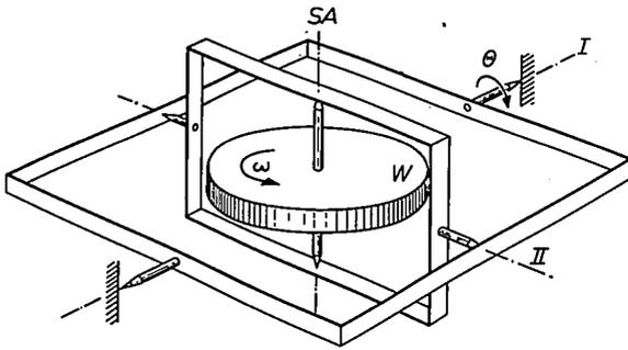
Fig. 5. Schematic diagram of a free gyroscope. SA spin axis of the wheel W, which has an angular velocity ω. I and II are the gimbal axes.
