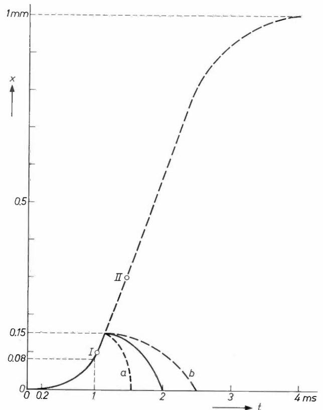
Fig. 7. Movement  $x(t)$  of the moving parts for a current pulse of 1 millisecond. The curves are calculated from the equation derived in the text and using values measured with the experimental model:  $K = 10, \alpha = 700 \text{ A/s}$  and  $m = 2 \text{ g}$ . Points I and II correspond to times measured on the oscillograms in fig. 9 when the needle travels 0.1 and 0.3 mm respectively.
