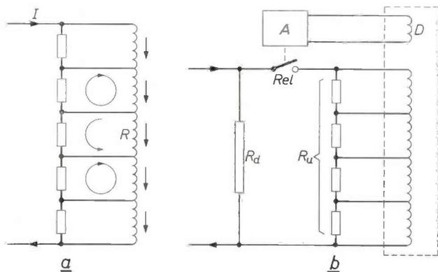
Fig. 13. *a)* Schematic circuit of coil divided into five sections each of which is short-circuited to distribute evenly the heat generated when a part of the coil goes normal. The arrows indicate where and how current starts to flow in the circuit when the part of the coil that has gone normal ( $R$ ) is in the central section.
