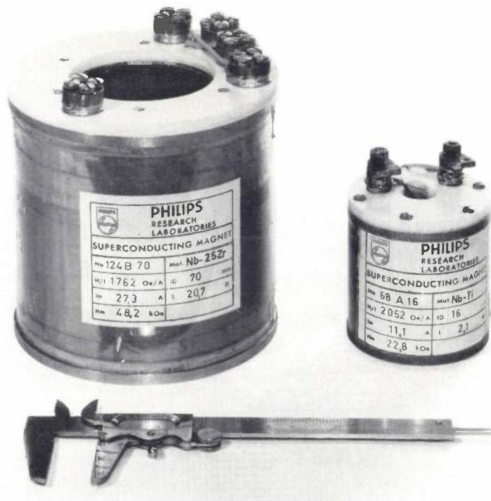
Fig. 10. Two superconducting wire-wound coils, which can generate a magnetic field of 90 kOe when the small coil is placed in the bore of the larger one.
