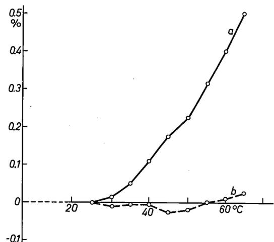
Fig. 5. Temperature error of the resistance-to-period converter: *a*) absolute error, and *b*) compared with the frequency of a reference oscillator whose frequency-determining capacitors were thermally connected to those of the converter by mounting oscillator and converter in the same case.
