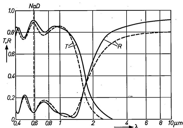
Fig. 2. Solid curves: spectral transmission  $T$  and reflection  $R$  of an indium oxide film. Spraying temperature  $500^{\circ}\text{C}$ ; film thickness  $0.31\ \mu\text{m}$ ; concentration of free charge carriers  $5 \times 10^{20}\ \text{cm}^{-3}$ ; mobility of the free carriers  $50\ \text{cm}^2/\text{Vs}$ .
