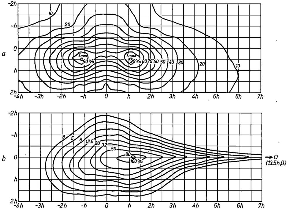
Fig. 4. a) Light distribution of a lantern, represented by lines of equal luminous intensity (isocandela diagram) in a horizontal plane. The light source is at a height  $h$  above point  $(0,0)$ . b) Isoluminance diagram, obtained as a product of the distribution (a) with the luminance-factor diagram in fig. 3a.
