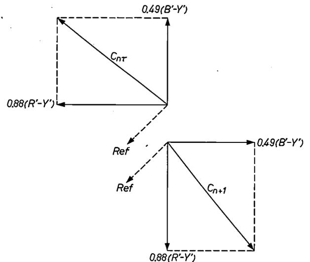
*Fig. 2.* The chrominance signal  $C_{n\tau}$  of a line, delayed by exactly  $64 \mu\text{s}$ , together with the non-delayed signal  $C_{n+1}$  of the next line. In this case the two components can *not* be obtained by simple addition and subtraction of the two signals.
