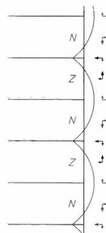
Fig. 3. Domain structure at the edge of a magnetic particle and the resultant image distortion. The electrons pass along the edge in paths perpendicular to the plane of the drawing.
