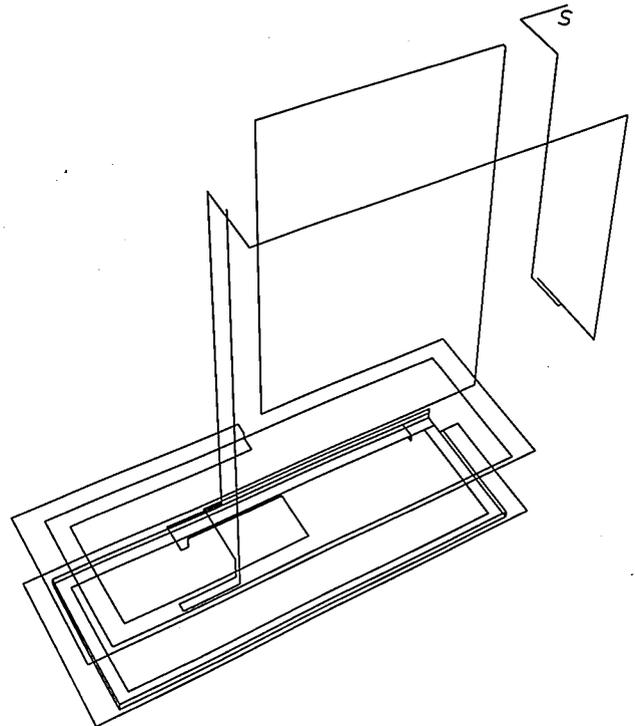
Fig. 5. Perspective drawing of the cutter path in fig. 2, made with the same workpiece programme. The cutter path here can be followed clearly;  $S$  is the starting point of the path. The dimensions in this figure are of course considerably distorted. The path is seen in the right perspective when the drawing is viewed from a distance of about 20 cm.
