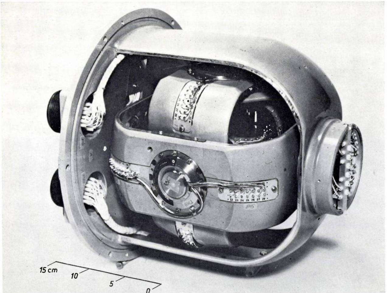
Fig. 15. The complete inertial platform, with two RAMP units and a directional gyro.
