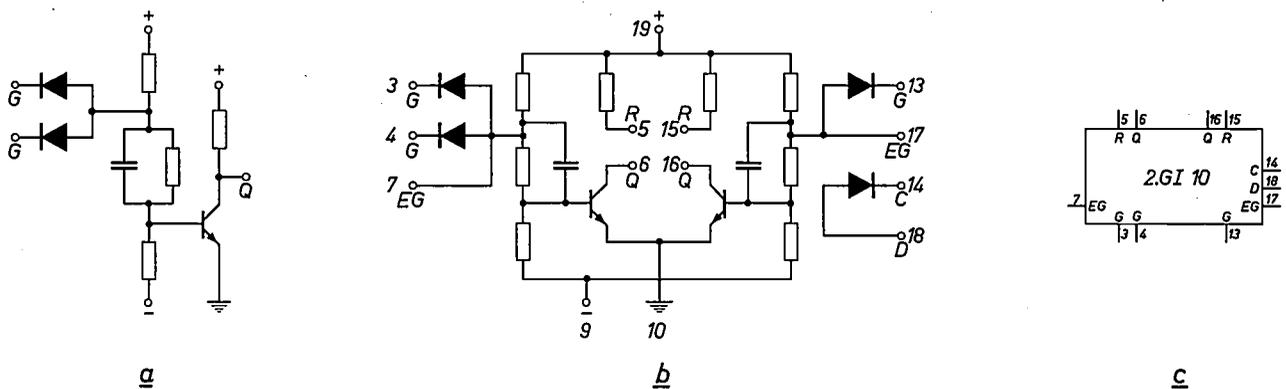
Fig. 2. a) The logic circuit of the GI blocks.  $G$  inputs.  $Q$  output.
