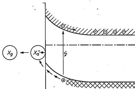
*Fig. 9.* Photo-desorption of negative ions ( $X_a^-$ ) adsorbed on an *N*-type semiconductor. The holes freed by the light move towards the surface and discharge the atoms, which then leave the surface ( $X_a^- + e^+ \rightarrow X_a \rightarrow X_g$ ).
