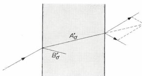
Fig. 8. The ratio of the transmitted and reflected intensities for a beam incident at an angle slightly different from the Bragg angle can be determined from the vector parallelogram of the energy flow vectors.
