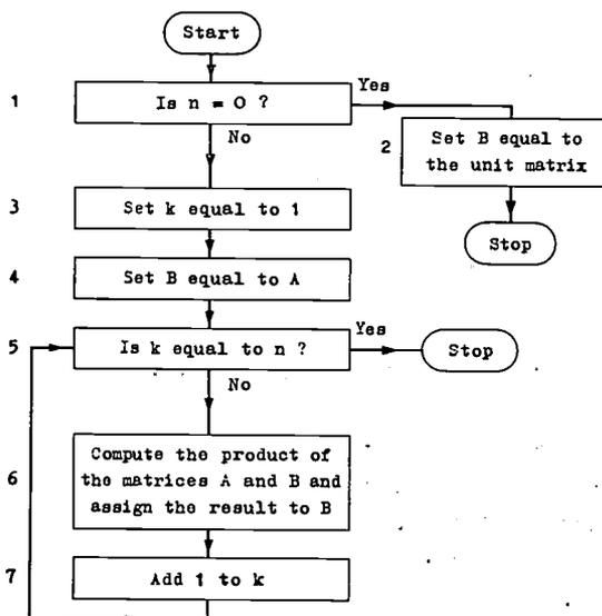
Fig. 2. Procedure that computes  $B$ , the  $n^{\text{th}}$  power of a square matrix  $A$ .
