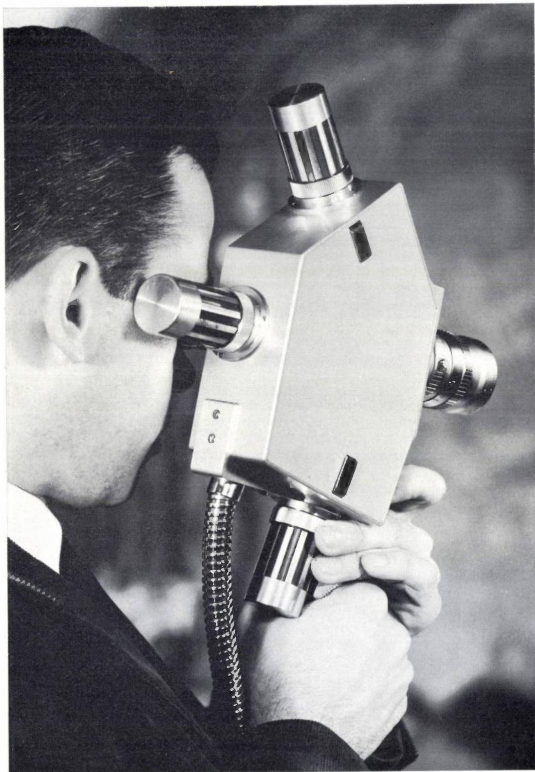
A "Plumbicon" camera tube of reduced size (1.6 cm dia., 13 cm length), which gives very sharp pictures in spite of the small size of the image, has recently been developed at Philips Research Laboratories, Eindhoven. Three tubes of this new type are used in the small colour television camera shown, whose
