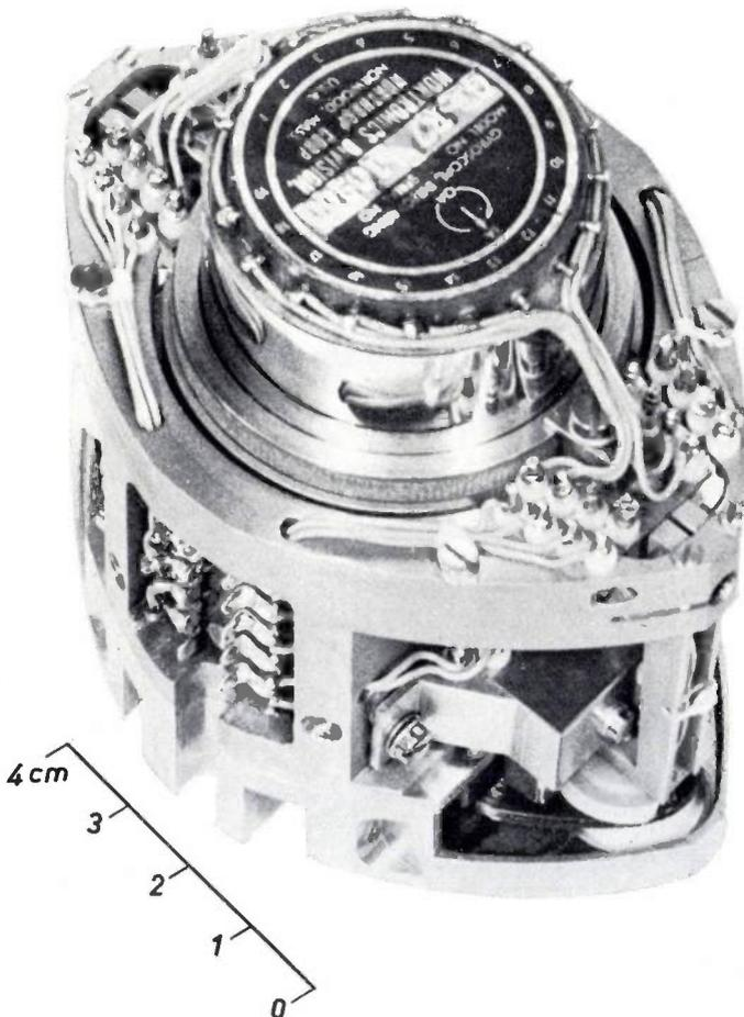
Fig. 12. Complete pendulum for the RAMP navigation system.
