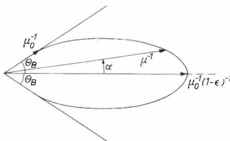
Fig. 9. Polar diagram showing the variation of the reciprocal absorption coefficient  $\mu^{-1}$  with the angle  $\alpha$  which the power flow makes with the reflecting planes for mode  $A_{\sigma}$ .
