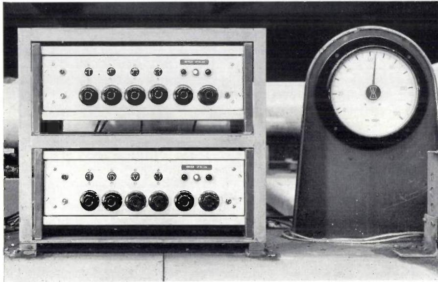
Fig. 20. The cabinets containing the digital circuits (one complete circuit for each pair of cutting blades; cf. fig. 19). The indicator tubes and the indicator lamps can be seen on each cabinet, and below them the switches for presetting the length and the tolerances (in this model the switches were similar to those of fig. 10 but with knobs instead of thumbwheels). The meter at the right of the cabinets indicates the speed of the cardboard strip.
