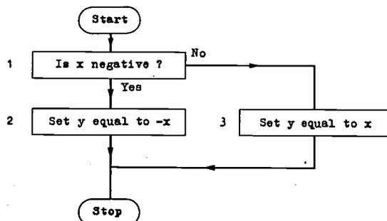
Fig. 1. Layout of procedure that evaluates  $y$ , the absolute value of a given variable  $x$ .
