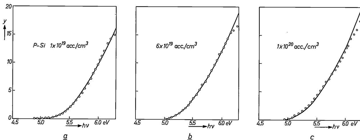
Fig. 7. Comparison of measured and calculated spectral distribution of the photoemission for *P*-type silicon. a)  $1 \times 10^{19}$  acceptors/ $\text{cm}^3$ , b)  $6 \times 10^{19}$  acceptors/ $\text{cm}^3$ , c)  $1 \times 10^{20}$  acceptors/ $\text{cm}^3$ . The calculation (see Appendix) was carried out for a stabilized Fermi level with  $\phi = 4.9$  eV and an escape depth of  $d = 2.0$  nm. These values give the best fit with the experimental results.
