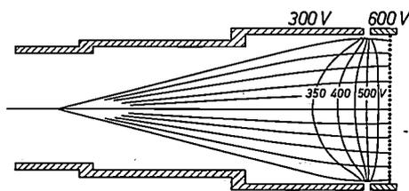
Fig. 6. Central trajectory of the beam in a number of deflected positions. The correction lens makes the electrons "land" at right angles to the photoconducting layer.
