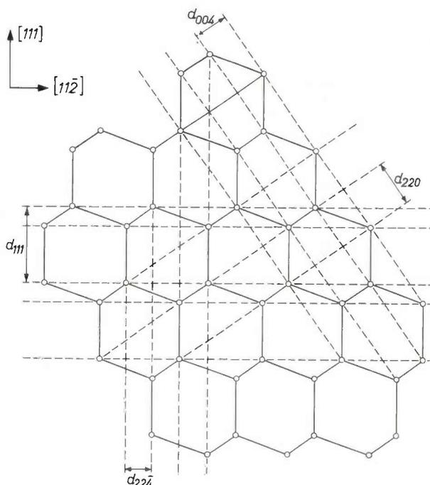
Fig. 13. Projection of a germanium lattice on to a  $(1\bar{1}0)$  plane. Planes like (220), (224) and (004) contain all the atoms present in the lattice whereas (111) planes do not.
