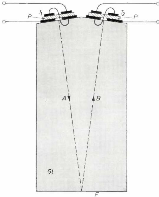
Fig. 6. Form of the delay line.  $Gl$  glass block.  $T_1$  input transducer.  $T_2$  output transducer.  $P$  piezoelectric plates.  $A$  and  $B$  direction of propagation of the ultrasonic shear waves.  $F$  reflecting face.
