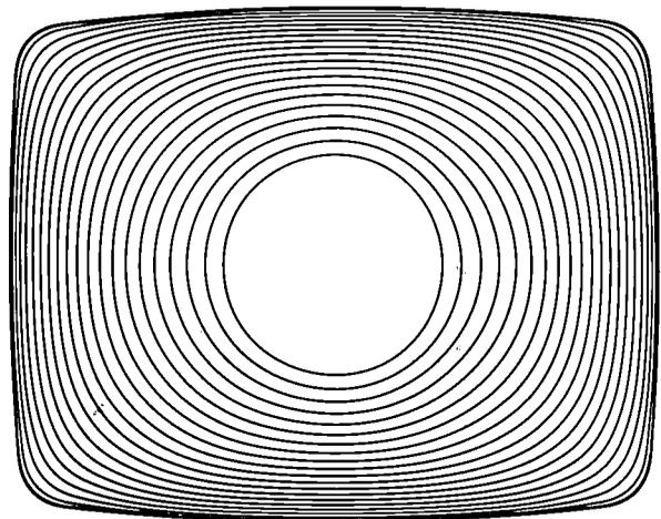
Fig. 1. Check drawing of the workpiece programme used for milling one of the moulds for pressing a television picture tube. The drawing represents an orthogonal projection on the  $x,y$ -plane of various paths which the cutter centre will follow during the milling operation.
