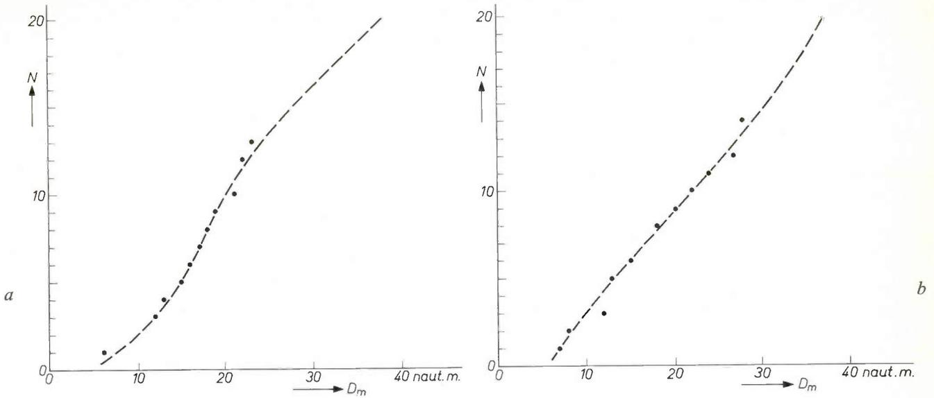
Fig. 24. Distribution of the errors in longitude (a) and in latitude (b) indicated by the RAMP equipment during six-hour flights over the European continent and over the Atlantic Ocean. The dots show the number of flights  $N$  with a maximum error less than  $D_m$  (in naut. miles). Errors larger than about 30 naut. miles occurred only in the beginning.
