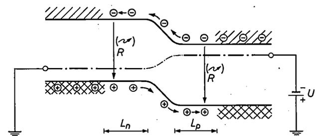
Fig. 2. The photo-e.m.f.  $U_f$  has the same magnitude as the external voltage  $U$  that must be applied in the forward direction to cause a current equal and opposite to the photocurrent to flow through the barrier. The arrows  $R$  represent recombinations, which may be accompanied by the emission of light.
