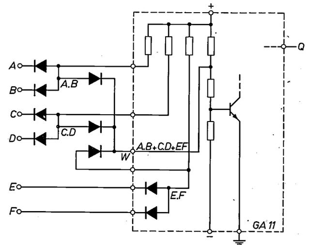
Fig. 4. Realization of the AND-OR function  $A \cdot B + C \cdot D + E \cdot F$  using diodes and a GA 11 block. The logic circuit is built up partly from external diodes and resistors included in the circuit block. The amplifier of the GA 11 is used as output stage. The logic circuit is connected to the input *W* of the amplifier. A high load can be applied to the output *Q*.
