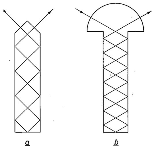
Fig. 3. Double-pass internal-reflection elements developed at Philips Laboratories, Briarcliff Manor (U.S.A.) by N. J. Harrick [5]. The element (b) is a more versatile type than (a) since the angle of incidence can be varied.
