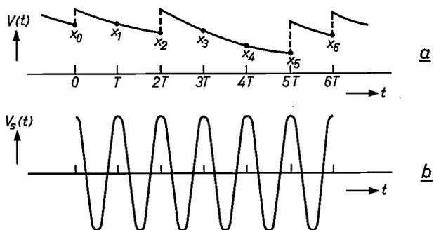
Fig. 10. a) Typical curve for the output voltage  $V(t)$ : it is assumed that no more than one discharge can take place in each positive half-cycle of the supply voltage  $V_s(t)$  shown in (b), and that the discharge always takes place at the peak value of the supply voltage, i.e. at the moment  $t = nT$ . The values of  $V(t)$  at these times are  $x_0, x_1, x_2$ , etc.
