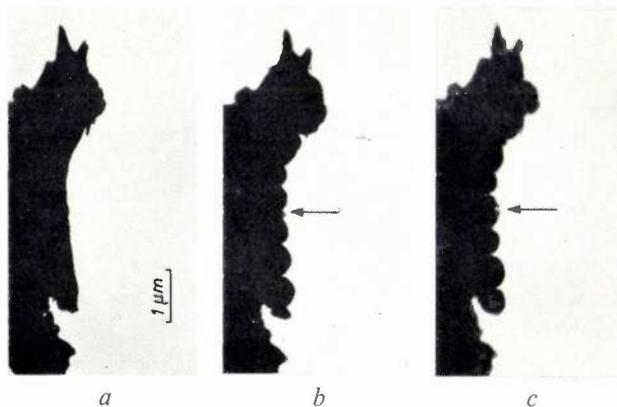
Fig. 2. Electron-photomicrographs of the edge of an MnAl particle (dark). Image  $a$ ) with sharply focused microscope,  $b$ ) with increased focal length,  $c$ ) with reduced focal length.
