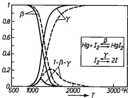
Fig. 6. Distribution of the iodine not combined with Na, Tl and In in the temperature range from 1000 to 2000 °K, similarly calculated for  $p_I = 10$  millibars (solid lines) and 100 millibars (dashed lines).  $\beta$  is the fraction present in the form of  $HgI_2$ ,  $\gamma$  is the fraction present in atomic form, and  $1 - \beta - \gamma$  is the remaining fraction of molecular  $I_2$ .
