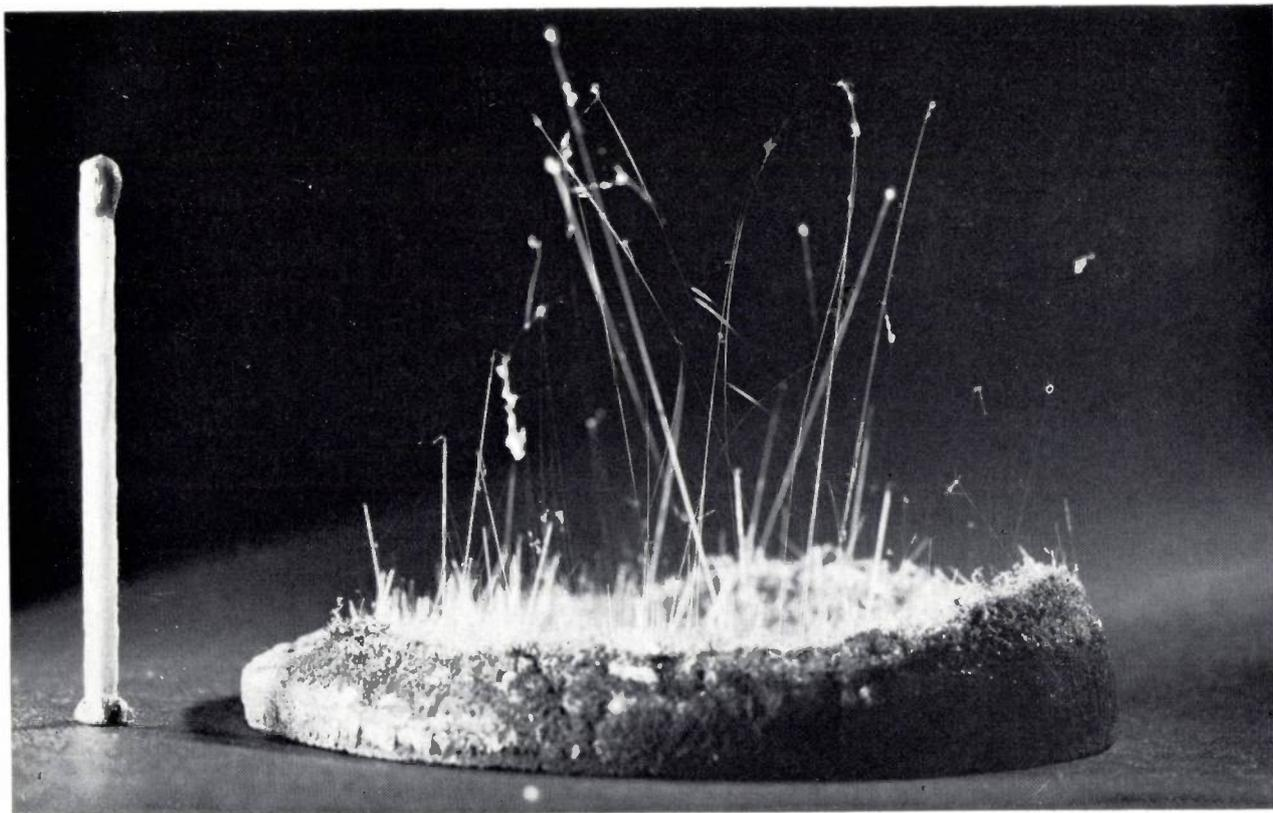
Fig. 1. Whiskers of silicon carbide, up to 6 cm long, with diameters up to 10  $\mu\text{m}$ .
