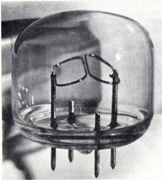
Fig. 2. The cold-cathode tube type 155 UG. If the voltage between the electrodes is sufficiently high, a self-sustaining gas discharge is produced when UV radiation is incident on the electrodes. Since molybdenum has been used as electrode material, the tube responds only to UV.
