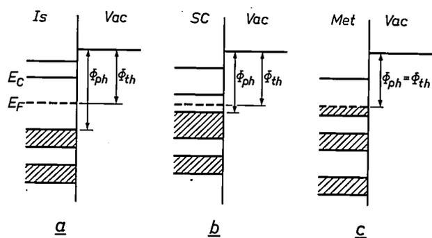
Fig. 3. Model of energy bands in an insulator (*Is*), an intrinsic semiconductor (*SC*) and a metal (*Met*), all with the same thermionic work function  $\Phi_{th}$  but with different photoelectric work functions  $\Phi_{ph}$ . The occupied energy zones are shown hatched.
