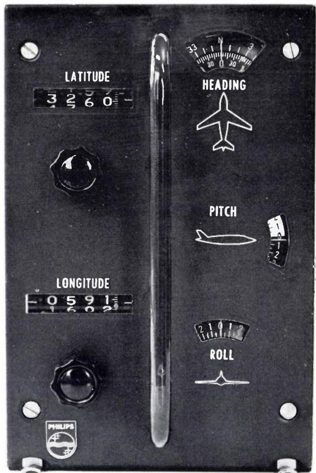
Fig. 17. The display unit, which indicates latitude, longitude, heading, roll and pitch of the aircraft.
