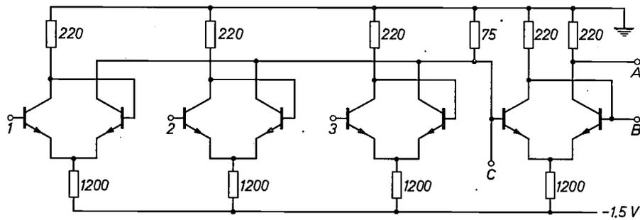
Fig. 9. The basic circuit used for threshold logic. The circuit gives a high voltage at A as soon as two or more of the inputs 1, 2 and 3 have a high voltage. This can be used in forming a carry digit in binary addition.
