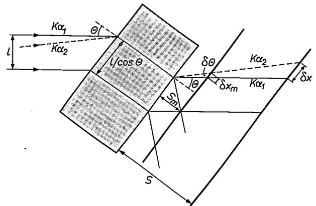
Fig. 24. Diagram to illustrate calculation of the minimum distance  $\delta x_m$  of  $\text{CuK}\alpha_1$  and  $\text{K}\alpha_2$  images on the film.
