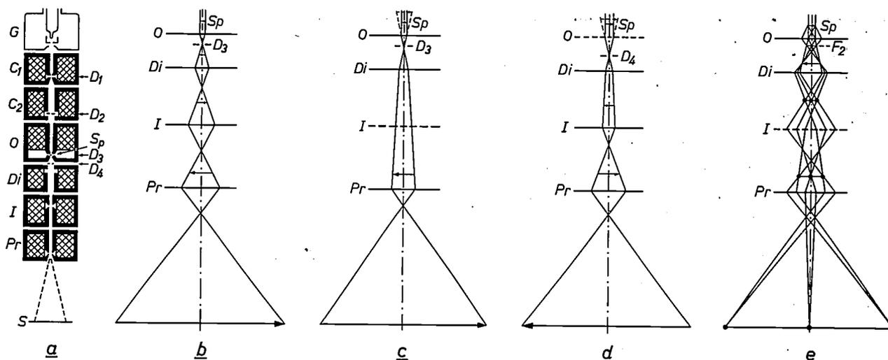
Fig. 4. *a*) Schematic arrangement of the microscope tube. *G* emission chamber with electron gun. *C*<sub>1</sub> first condenser lens. *C*<sub>2</sub> second condenser lens. *O* objective lens. *Sp* specimen. *Di* diffraction lens. *I* intermediate lens. *Pr* projector lens. *S* fluorescent screen. *D*<sub>1</sub> and *D*<sub>2</sub> condenser diaphragms. *D*<sub>3</sub> objective diaphragm. *D*<sub>4</sub> selector diaphragm.
