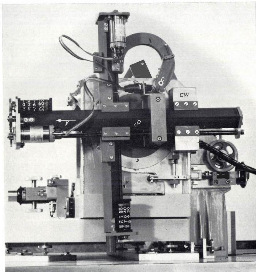
Fig. 8. The linear-tracking mechanism is mounted on the diffractometer. The mechanical Ewald construction has been translated and rotated with respect to the construction shown in figs. 6 and 7.  $CW$  counterweight.  $O$  origin.  $CP$  link.
