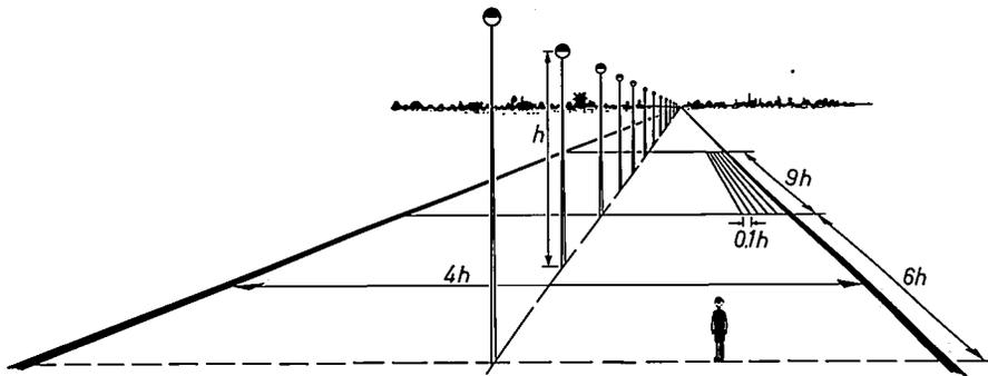
Fig. 10. Standard configuration of a road with lanterns. Any conceivable configuration for which the average luminance is to be calculated can be built up from the strips into which the road is divided. If there are more rows of lanterns the calculation is done in steps and the results added.
