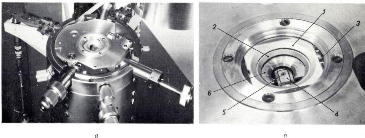
Fig. 10. *a*) The standard specimen stage in the microscope. The upper section of the tube shown here is the ring *W* (fig. 9) of the objective lens. *b*) A detailed view of the central section. 1 upper cross-table slide. 2 lower slide. 3 push-rod for the movement of the upper slide. 4 specimen holder. 5 specimen. 6 cooling element ( $-180^{\circ}\text{C}$ ); this accessory does not belong to the stage but is introduced separately from the side.
