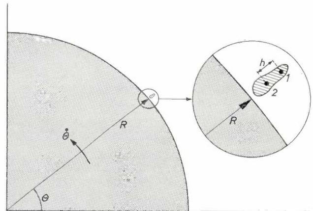
Fig. 3. Indication of the local vertical with a physical pendulum.  $R$  Earth's radius;  $\Theta$  latitude; 1 pivot; 2 centre of gravity;  $h$  distance between 1 and 2.
