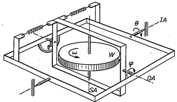
Fig. 6. Schematic diagram of a gyro with a spring restraint about one of the axes. The deviation φ about this axis (the output axis OA), which can be read from the scale, is now proportional to the angular velocity  $\dot{\theta}$  of the gyro-wheel about the other axis (the input axis IA). This device is known as a rate gyro.
