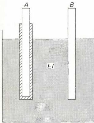
Fig. 2. Schematic diagram of a conventional electrolytic capacitor. *A* electrode covered with an insulating oxide film. *B* counter electrode. *El* electrolyte. The electrodes are usually of aluminium. The electrolyte used is frequently water or glycol containing a mixture of boric acid and sodium borate or ammonium borate.
