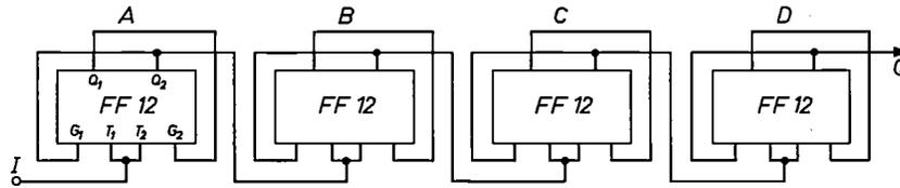
Fig. 7. Circuit of a scale-of-16 counter made up from four FF 12 circuit blocks.
