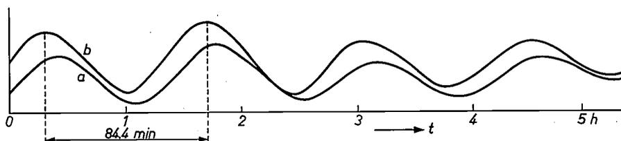
Fig. 20. Part of a recording of the velocity signals from the X-RAMP (a) and from the Y-RAMP (b) at an initiated oscillation of about 1' amplitude during a 12-hour laboratory test.
