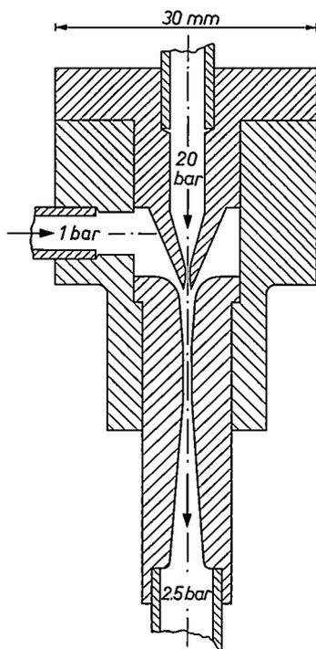
Fig. 2. Cross-section of the expansion ejector. The helium gas flowing from above (20 bar) expands to 2.5 bar, giving cooling through the Joule-Thomson effect. At the same time, through the opening on the left, helium gas of 1 bar is drawn in from the collector vessel (*C* in fig. 1) and again compressed to 2.5 bar.
