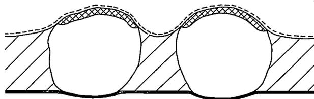
Fig. 4. After the strongly *N*-type CdS grains are embedded in the resin, a *P*-type layer of  $\text{Cu}_{2-\delta}\text{S}$  is grown epitaxially on the protruding surfaces of the grains. On the side where the light will be incident (top), the grains are connected together by a transparent gold film.
