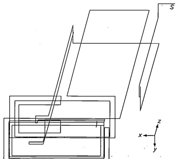
Fig. 6. Oblique projection of the cutter path of fig. 5.  $S$  starting point. This drawing has the advantage that the dimensions correspond to the actual dimensions not only in the  $x, y$ -plane, but also in the  $z$ -direction. The cutter path is not so easy to follow, however, as in fig. 5.
