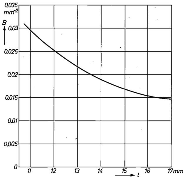
Fig. 5. Spherical-aberration coefficient  $B$  as a function of the spacing  $l$  between anodes  $A_1$  and  $A_3$ .
