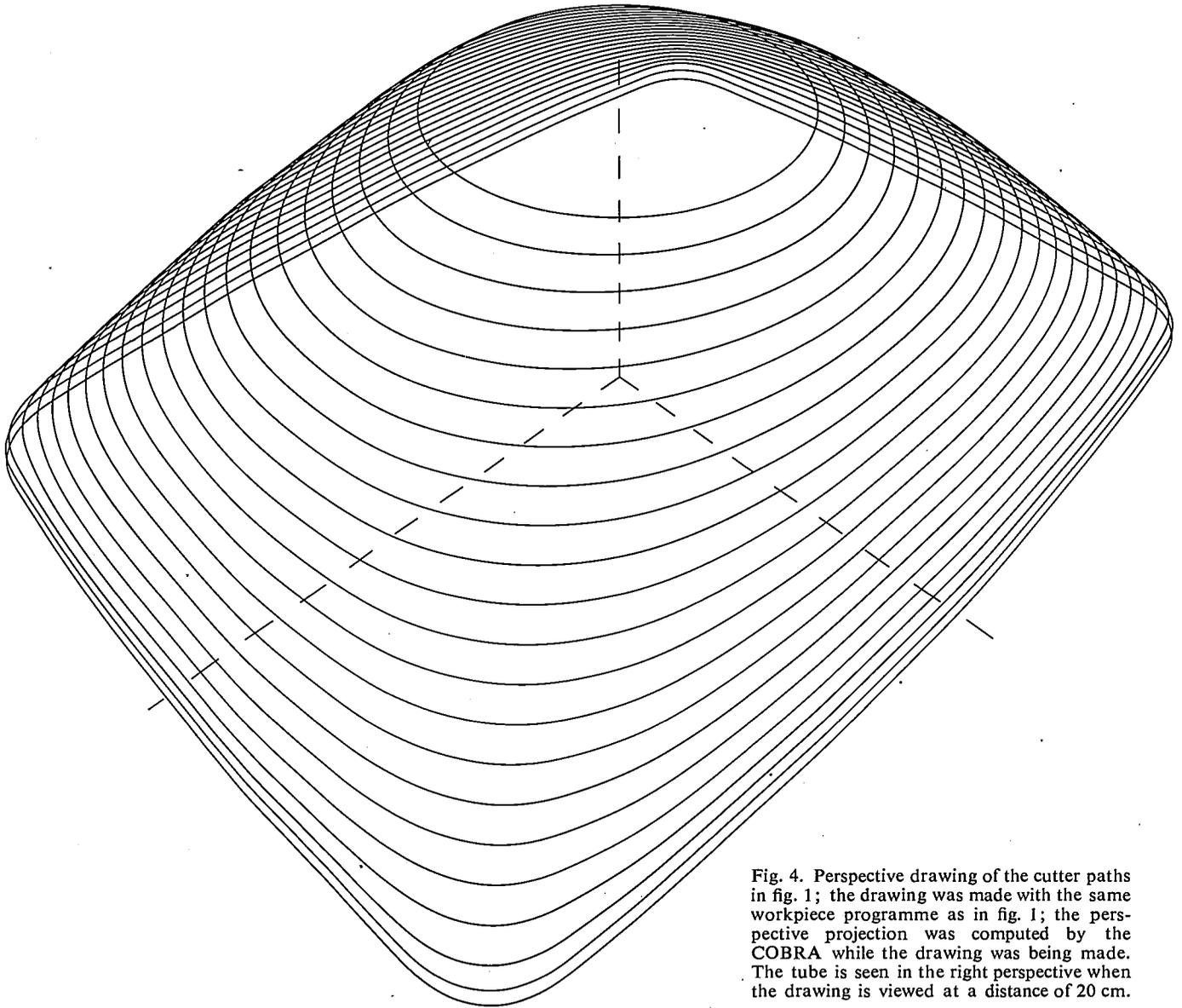
Fig. 4. Perspective drawing of the cutter paths in fig. 1; the drawing was made with the same workpiece programme as in fig. 1; the perspective projection was computed by the COBRA while the drawing was being made. The tube is seen in the right perspective when the drawing is viewed at a distance of 20 cm.
