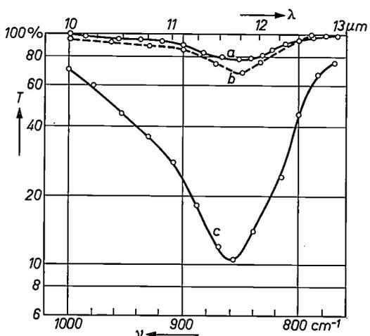
Fig. 13. As fig. 12 for thermally produced germanium dioxide films on Ge, with different conditions of measurement. The dip in the spectrum is the absorption band due to the GeO stretching vibration.
