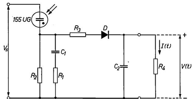
*Fig. 7.* Circuit for the cold-cathode tube in which the discharge is self-quenching: at each discharge a short pulse of current passes through the tube, but the average value of this current — i.e. the dissipation in the tube — is low. The supply voltage to the circuit is 220 V from the a.c. mains; the output voltage  $V(t)$  is a measure of the intensity of the UV radiation incident on the tube.
