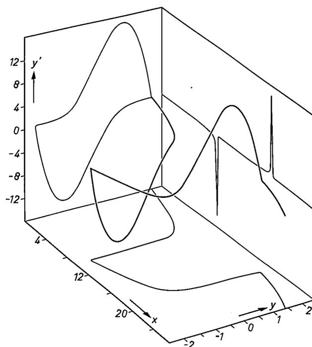
Fig. 1. Stationary solution (independent of the initial values) of the Van der Pol equation for  $\epsilon = 10$ . The three-dimensional curve and its orthogonal projections on the three co-ordinate planes were calculated by a computer; so also was the complete projection on the plane of the drawing.
