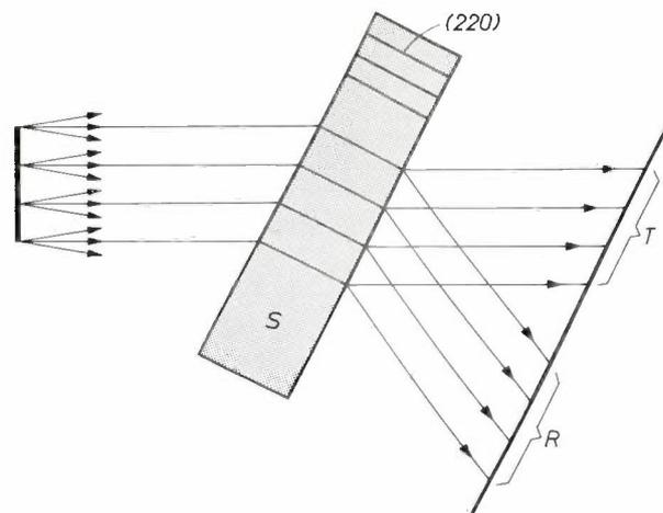
Fig. 22. Principle of the Barth-Hosemann technique for revealing dislocations. A divergent X-ray beam is incident on the crystal *S*. Only those rays which are incident at an angle differing not more than a few seconds from the Bragg angle will be anomalously transmitted; all the other rays will be strongly absorbed in the thick crystal. Dislocations situated in the illuminated region of the crystal are visible on the film in both the *T* and *R* images as regions of low intensity.
