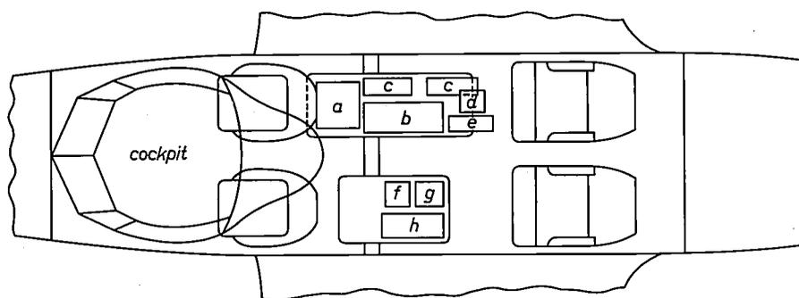
Fig. 21. Installation of the test equipment in the De Havilland Dove. a platform. b electronic units. c power converters. d mode control units. e display unit. f auxiliary equipment. g recorder. h oscilloscope.
