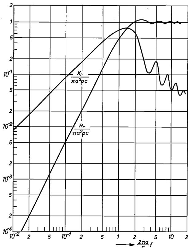
Fig. 1. The radiation reactance  $X_r$  and the radiation resistance  $R_r$  of a loudspeaker as a function of frequency  $f$  (on relative scales).  $a$  radius of the cone.  $\rho$  air density.  $c$  velocity of sound in air. At high frequencies the radiation resistance per unit area approaches  $\rho c$ , the specific acoustic impedance of air.  $X_r/2\pi f$  is known as the radiation mass.
