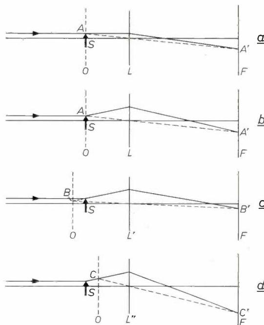
Fig. 1. Illustrating the formation by an electron beam of an image of the edge of a specimen  $S$  with magnetic properties, causing Lorentz forces to act on the electrons.  $F$  image plane.  $O$  object plane.  $L$  electron lens.
