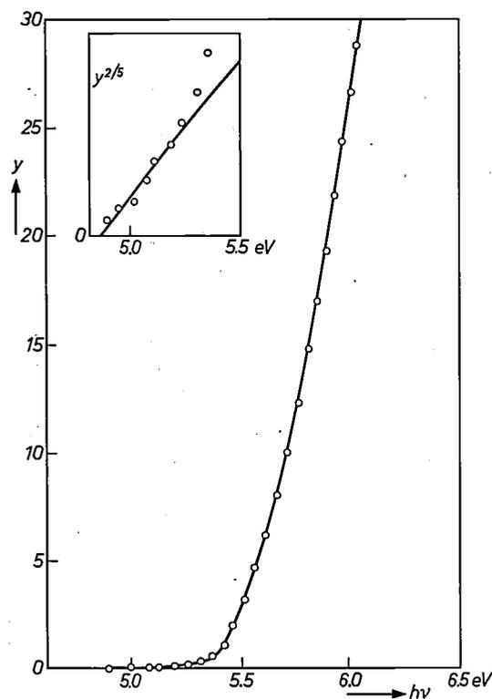
Fig. 8. Photoemission of silicon with weak *P*-type doping ( $1.6 \times 10^{16}$  Ga/cm<sup>3</sup>): the yield  $y$  as a function of photon energy  $h\nu$ . In the inset,  $y^{2/5}$  is plotted against  $h\nu$ . The solid curve represents the relation
