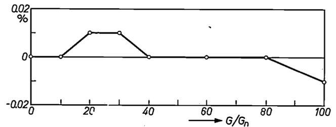
Fig. 9. Linearity error (relative to the maximum load) of a frequency analogue measuring system consisting of the strain-gauge load cell PR 9228/05 C and the  $\Delta R/R \rightarrow \Delta f/f$  converter.
