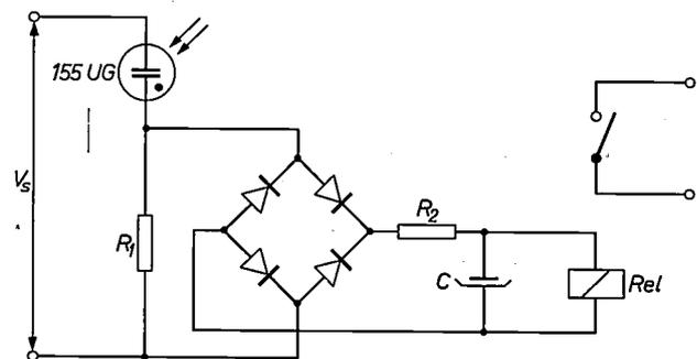
Fig. 9. Circuit in which the mean tube current is sufficiently high to energize directly a relay  $Rel$ . The 155 UG tube can withstand this high dissipation without damage.
