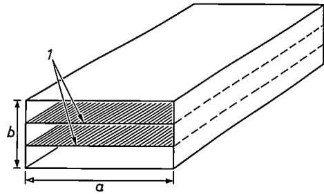
Fig. 9. Filter for the modes  $E_{mn}$  and  $H_{mn}$  with  $n \neq 0$ . These modes are attenuated by the resistive sheets 1, unless they happen to have no tangential  $E$ -component at the sheets. The  $H_{10}$  mode is unperturbed since its  $E$ -field is perpendicular to the sheets.
