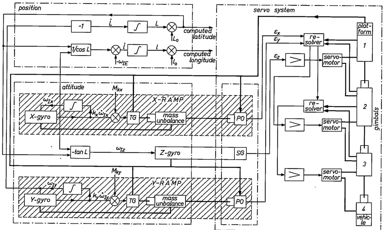
Fig. 27. Signal flow diagram of the complete RAMP navigation system. The bold lines correspond to mechanical connections, the thin lines to electrical connections.
