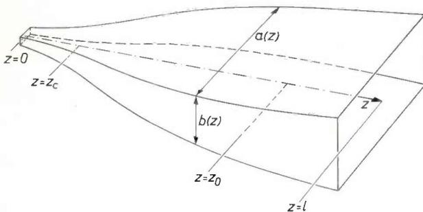
Fig. 13. The taper for transferring the  $H_{10}$  mode from standard-size to oversized waveguide. The design is based on a minimum  $H_{10} \rightarrow H_{30}$  mode conversion for a given length of the taper. The width  $a$  is a function of  $z$  with a bottle-like shape, the height  $b$  a linear function of  $z$ .
