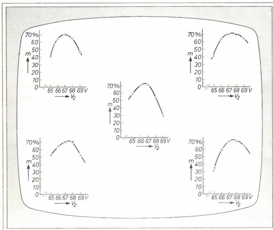
Fig. 8. Modulation depth  $m$  as a function of the voltage  $V_2$  on electrode  $A_2$ , measured with white light, at the centre and at the four corners of the picture. The frequency used was 3 MHz and the beam current 0.2  $\mu\text{A}$ . At  $V_2 \approx 67$  V the resolving power is optimum over the whole area.
