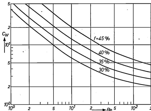
Fig. 8. The resistance factor  $C_w$  — see equation (4) — as a function of  $Re$  for the same four values of the packing factor  $f$  as in fig. 6. For small  $Re$ ,  $C_w \propto 1/Re$ .
