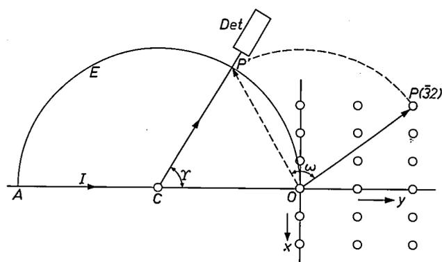
Fig. 6. The Ewald construction. With the aid of this construction one can determine the angles at which the crystal and the detector have to be placed with respect to the incident X-ray beam  $AC$  in order to bring the plane ( $hk$ ) into reflection. The origin of reciprocal space is at point  $O$ , diametrically opposite point  $A$ . The diffracted beam is parallel to  $CP$ .  $E$  Ewald circle.
