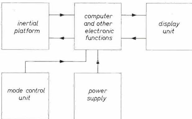
Fig. 16. Block diagram of the RAMP navigation equipment.
