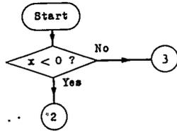
Fig. 3. Flow diagram symbolism representing a branch operation.
