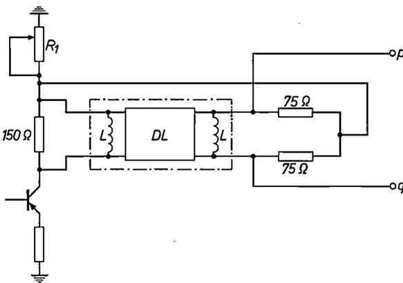
Fig. 14. Circuit of a decoder for a PALd receiver. The transistor amplifies the chrominance signal. The value of the resistor  $R_1$  is such that the signal voltage across it is equal to half the output signal of the delay line  $DL$ , so that the  $(B' - Y')$  component and the  $(R' - Y')$  component of the chrominance signal appear at the output terminals  $p$  and  $q$ .
