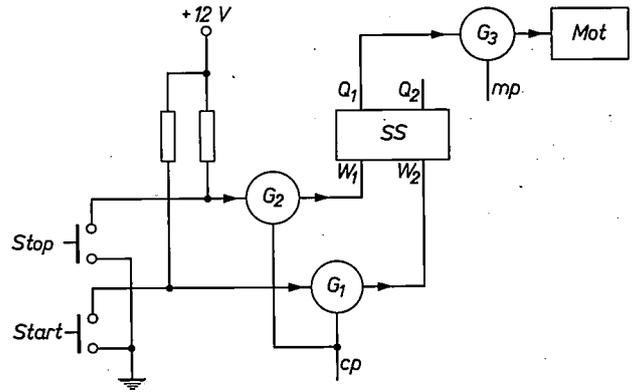
Fig. 18. Motion of a stepping motor *Mot* can be controlled by applying motor pulses  $mp$ . Pulse gate  $G_3$  is controlled by a bistable circuit *SS* whose state can be changed with *Start* and *Stop* push-button switches. Clock pulses are denoted by  $cp$ .
