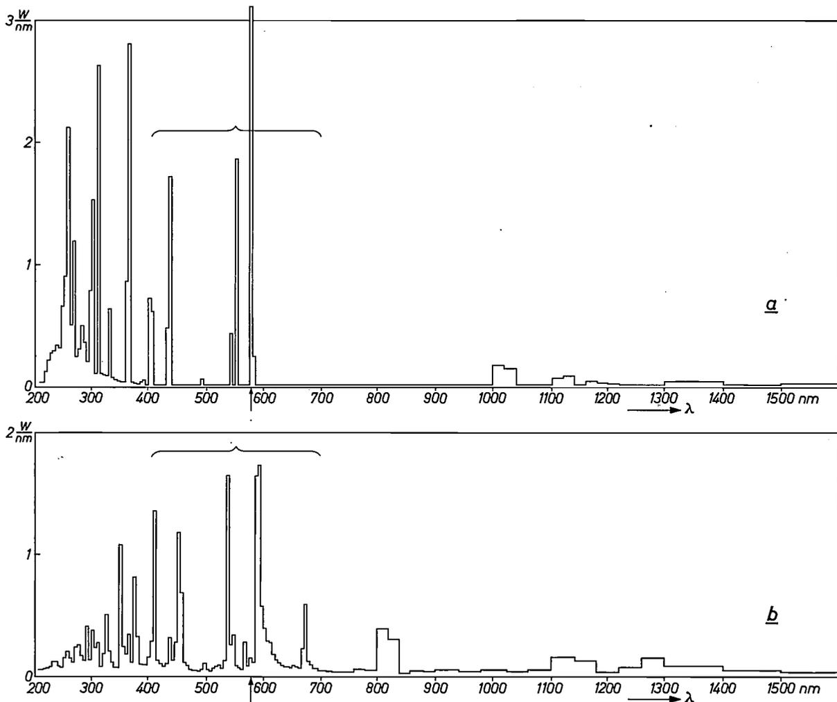
Fig. 2. Spectral energy distributions of two geometrically identical 500 W discharge lamps whose bulbs are made entirely of quartz glass: a) HP lamp, b) HPI lamp. The visible part of the spectrum is indicated by the bracket. It can be seen that the HPI lamp emits less radiation in the ultra-violet than the HP lamp but rather more radiation in the infra-red. It is also noticeable that the emission in the visible part of the spectrum is more uniform in the HPI lamp than in the HP lamp.
