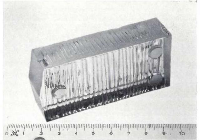
Fig. 7. The glass block of the delay line. The side walls have been "roughened" to minimize unwanted reflections of the ultrasonic waves. The three small protruding faces are used for fixing the block when the reflecting face is ground away.
