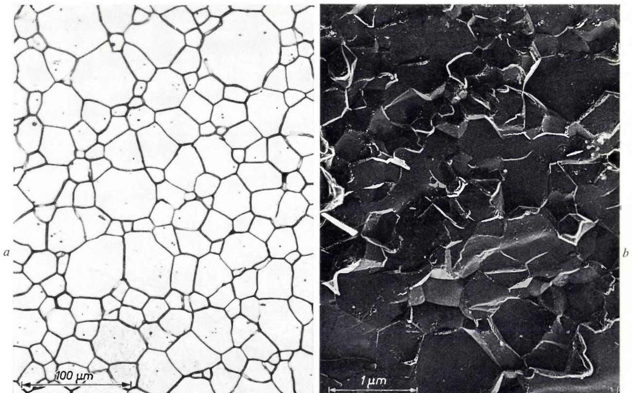
**Fig. 6.** Specimens of  $\text{Ni}_{0.36}\text{Zn}_{0.64}\text{Fe}_2\text{O}_4$  of the same porosity (0.3%) and the same resistivity ( $10^7 \Omega\text{cm}$ ), prepared in various ways: *a*) by the conventional method (20 h at 1275 °C), *b*) by continuous hot pressing (30 min at 1025 °C and 1000 bar); *a*) is a polished and thermally etched cross-section photographed with the aid of a microscope; *b*) is a fracture surface as shown by the EM 200 electron microscope.
