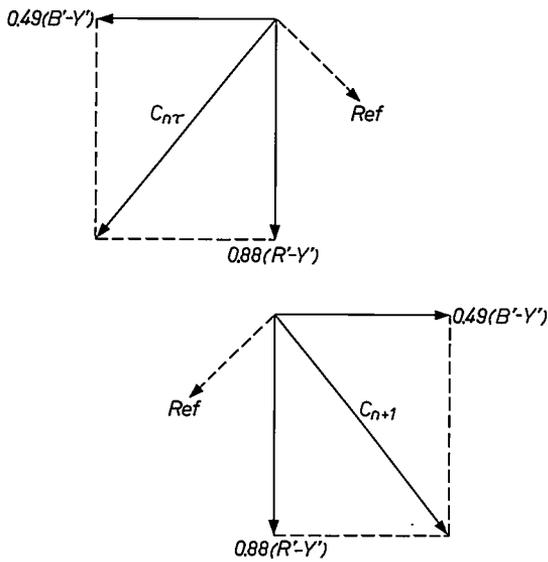
Fig. 3. When the delay line causes a phase shift of an odd multiple of  $\pi$  radians, the  $(R' - Y')$  signal can be obtained by the addition of the  $C_{nr}$  and  $C_{n+1}$  signals, and the  $(B' - Y')$  signal by their subtraction.
