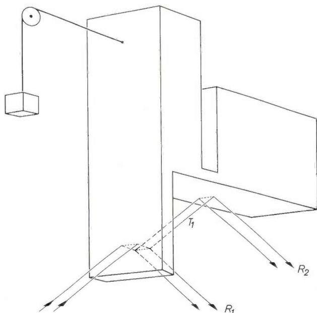
*Fig. 15.* Special crystal form for experiments as indicated in *fig. 14a*. By applying different loads the narrow bridge of the crystal can be bent elastically and in this way the angle of incidence on the base of the L is varied. (The regions of the crystal where the diffraction takes place are *not* deformed.)
