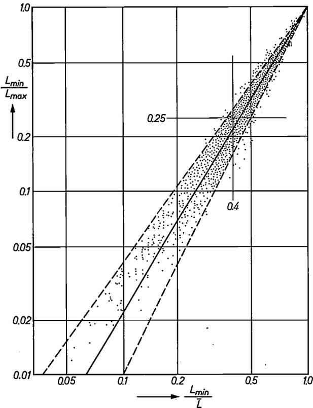
Fig. 5. The values of  $L_{min}/\bar{L}$  and  $L_{min}/L_{max}$  for 2160 lighting installations. The condition  $L_{min}/\bar{L} \geq 0.4$  is met by nearly all installations for which  $L_{min}/L_{max} \geq 0.25$ .
