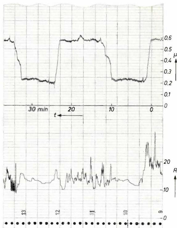
Fig. 1. The coefficient of friction  $\mu$  of gold on gold and the contact resistance  $R$  as a function of time, measured in a stream of nitrogen to which benzene vapour was periodically added. During the addition of benzene vapour the coefficient of friction is reduced from about 0.6 to about 0.2.  $R$  is indicated in arbitrary units.
