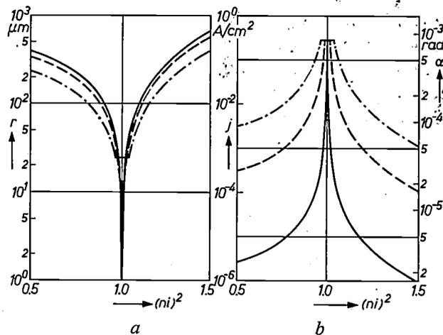
Fig. 5. *a*) Variation of the radius *r* of the electron spot on the specimen as a function of the excitation of *C*<sub>2</sub> with constant excitation of *C*<sub>1</sub> (*ni* is the number of ampere-turns in arbitrary units) and constant diameter of the condenser diaphragms.
