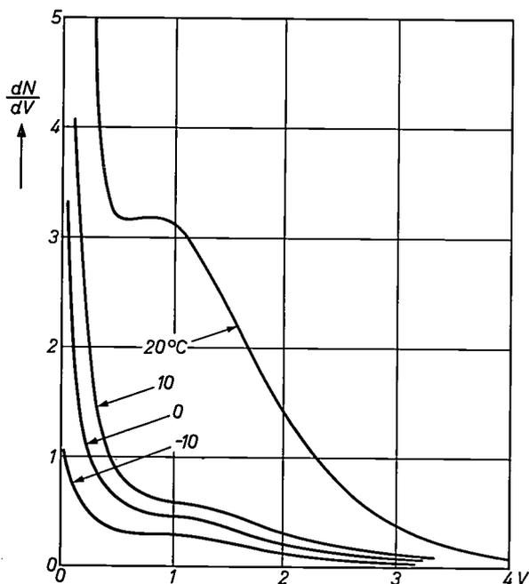
Fig. 9. Pulse-amplitude distribution of the dark current in a photomultiplier, for various temperatures. The probability density  $dN/dV$  (in arbitrary units) is shown as a function of pulse amplitude  $V$ . (The pulse amplitudes have been normalized to the mean amplitude of the pulses for single photoelectrons, as determined by the measurement of the single-electron spectrum, see p. 272.)
