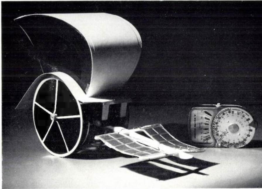
Fig. 5. Two-wheel toy "cab" driven by two miniature electric motors, fitted under the axles and powered by two "solar sheets". The left-hand sheet supplies the right-hand wheel and the right-hand sheet the left-hand wheel. The cab moves forward when placed in a beam of light (and the cross-over in the feed keeps it within the beam).
