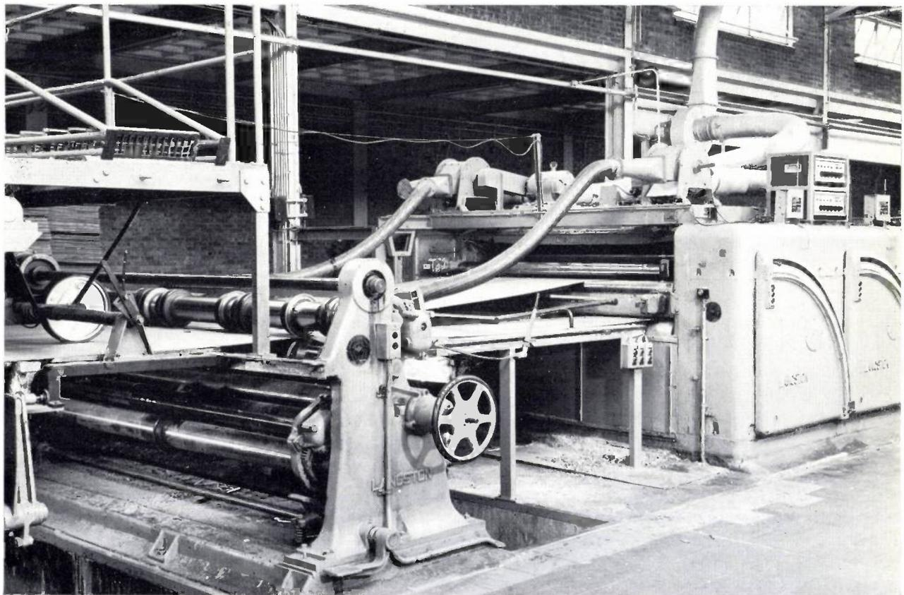
Fig. 18. The part of the production machine where the corrugated-cardboard strip is cut (cf. fig. 16). On the left can be seen the wheel which measures the speed at which the strip is travelling, and on the right of it the cutting wheels which cut the strip lengthwise. The two cabinets containing the digital circuits are on the right, one for each pair of cutting blades. Below them can be seen the mechanism for adjusting the speed of rotation of the cylinders.
