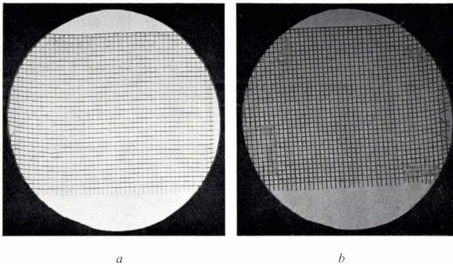
Fig. 11. Illustration of the Borrmann delta effect. *a*) A grid of  $25 \mu\text{m}$  wires when placed on the front surface of the crystal (facing the X-ray source) produces an image in which the shadow of the vertical wires, which are parallel to the diffracting planes, is diffuse. In *b*) the grid is on the back surface and the shadow of the wires is sharp.
