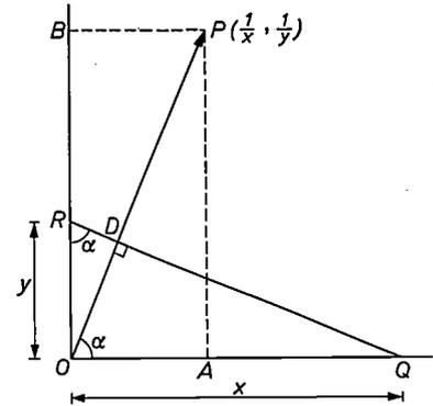
Fig. 4. The vector  $OP$  is the reciprocal vector for the set of parallel planes parallel to the line  $QR$  and whose spacing  $d'$  equals the length  $OD$ .
