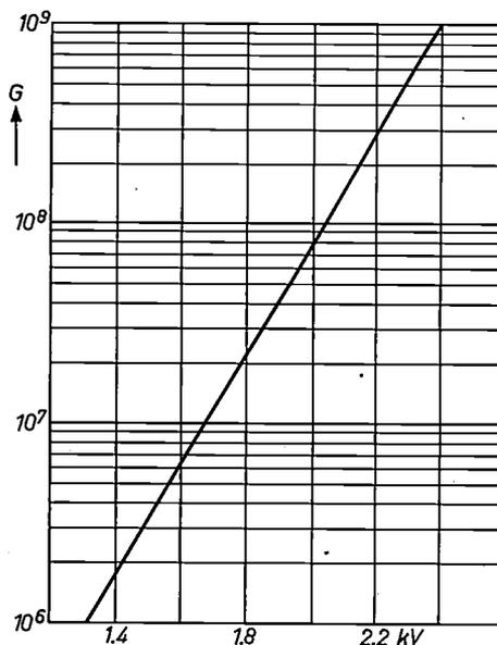
Fig. 6. Variation of the gain  $G$  of a multiplier with 14 dynodes of Ag-MgO-Cs as a function of the high voltage.
