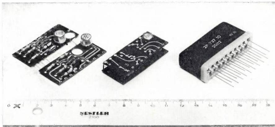
Fig. 1. One of the 10-series circuit blocks, containing two logic circuits. The circuits are mounted on printed wiring boards which fit into a metal case.
