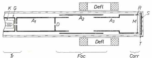
Fig. 3. Diagram of the construction of a "Plumbicon" tube with electrostatic focusing. *Tr* triode gun, consisting of the cathode *K*, the control electrode *G* and the anode *A*<sub>1</sub>. The focusing lens *Foc* is formed by the electrodes *A*<sub>1</sub>, *A*<sub>2</sub> and *A*<sub>3</sub>. *D* diaphragm. The ring *R* and the mesh screen *M* together with *A*<sub>3</sub> form the correction lens *Corr*. *T* photoconducting layer. *S* signal plate. *Defl* deflection coils.
