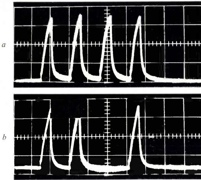
Fig. 3. Oscillograms of the heat radiated by the silicon bridge used in the arrangement of fig. 4 (horizontal scale: 1 square for 2 ms).
