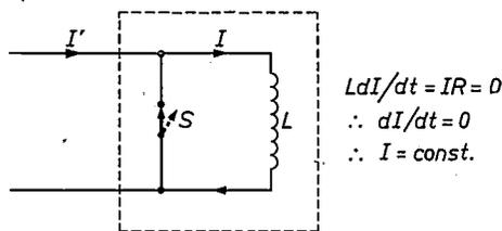
*Fig. 1.* When the coil in which a current  $I$  is flowing is short-circuited by means of a superconducting switch  $S$ , thus forming a closed superconducting circuit — i.e. one whose resistance  $R$  is zero — the current  $I$  then no longer reacts to variations in the current  $I'$  in the external circuit. Variation of  $I'$  only causes a change in the current flowing in  $S$ .
