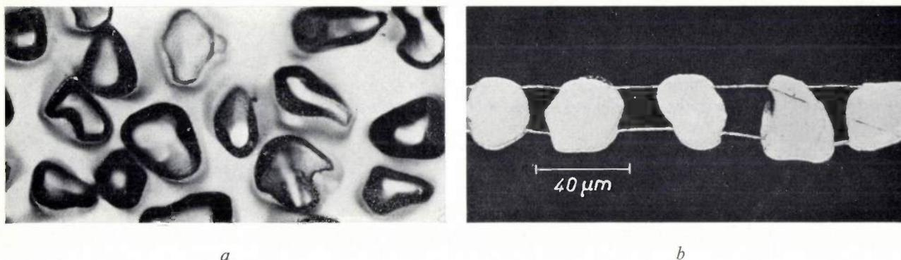
Fig. 2. *a*) Surface view and *b*) cross-section of a photoconducting CdS sheet as seen through a microscope.
