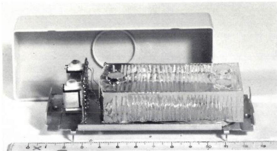
*Fig. 11.* Delay line with the cover removed.
