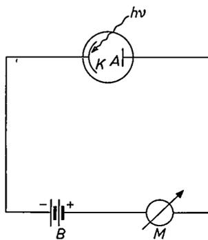
Fig. 1. Principle of photoemission. *K* cathode, *A* anode, *B* battery, *M* microammeter. A measurable current flows in the circuit only when the cathode is exposed to light radiation.
