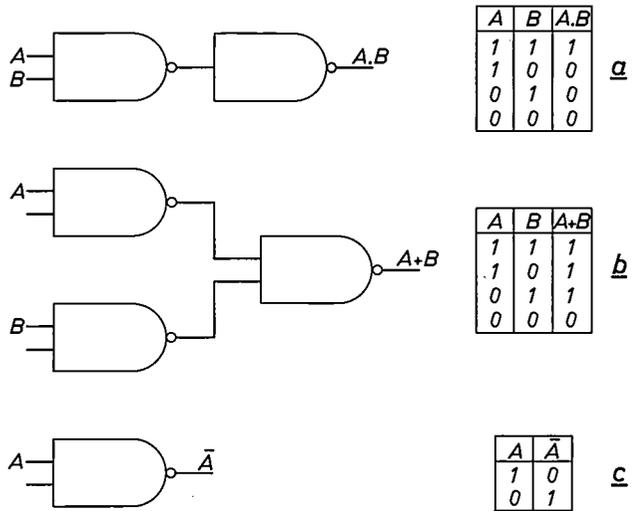
Fig. 3. The basic logic functions realized with NAND circuits. a) The AND function  $A \cdot B$ . b) The OR function  $A + B$ . c) The NOT function  $\bar{A}$ . The truth table for each function is given.
