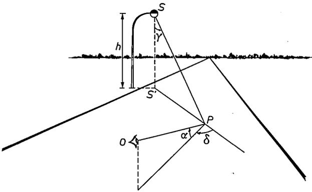
Fig. 1. Configuration of a road lighting installation. S light source, P a point of the road surface, O observer.
