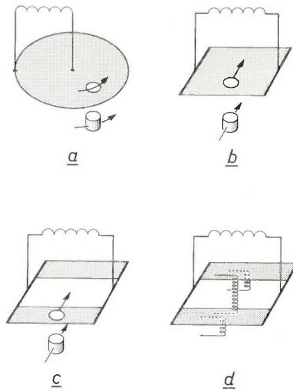
Fig. 12. Examples of the four most important types of design of the superconducting dynamo for the generation of a persistent current in a superconducting circuit. *a*) With a rotating field provided by a rotating permanent magnet. *b*) With a displacement field. *c*) and *d*) Variations of (*b*) with a superconductor divided into two strips; in (*d*) the displacement field is obtained by means of coils.
