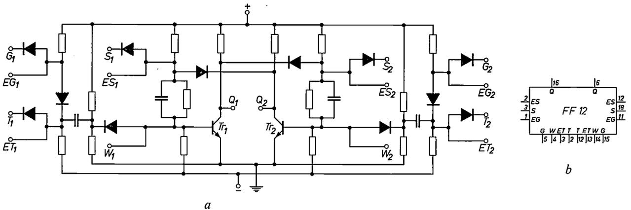
Fig. 5. a) The bistable circuit with trigger gates in the circuit block FF 12. b) Symbol for this circuit block.
