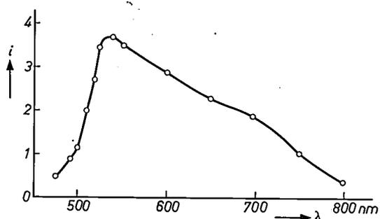
Fig. 3. Spectral sensitivity curve of a photoconducting CdS sheet. The photocurrent  $i$  is indicated in arbitrary units. (The measurements were made by J. H. Haanstra of these Laboratories.)
