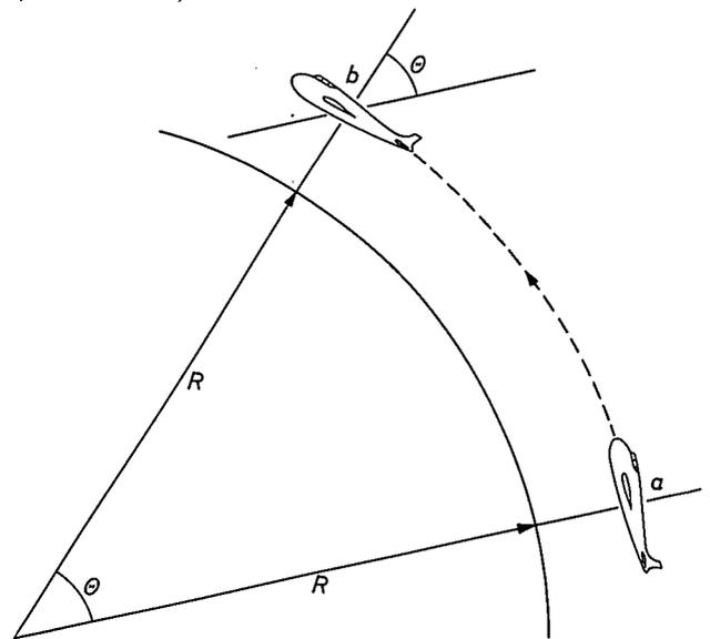
Fig. 1. The change of position of a vehicle moving from *a* to *b* can be found from the change  $\Theta$  of direction of the local vertical. *R* is the radius of the Earth. The RAMP system is based on this principle.
