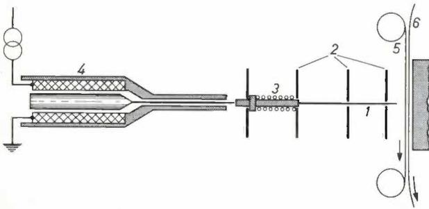
Fig. 6. Printing element in mechanical process. 1 needle. 2 guide-plates. 3 return spring. 4 electromagnet. 5 inking ribbon. 6 paper.
