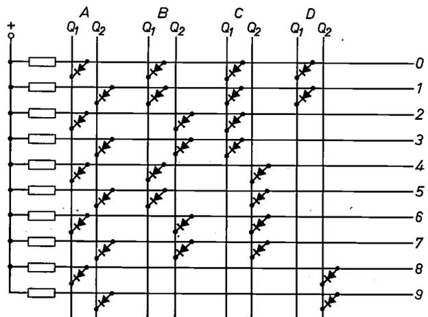
**Fig. 9.** Circuit for decoding the contents of a decade counter using four scale-of-two counters *A*, *B*, *C* and *D*. The outputs  $Q_1$  and  $Q_2$  of *A*, *B*, *C* and *D* are connected to the vertical wires; a horizontal wire goes to the “high” voltage when the counter reads the corresponding number.
