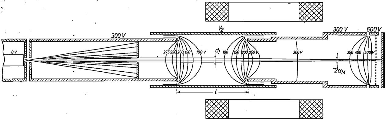
Fig. 4. Some equipotential surfaces and electron paths for an undeflected beam. The voltages at the electrodes  $A_1$ ,  $A_3$  and  $R$  (see fig. 3) are given with respect to the cathode. The voltage  $V_2$  of  $A_2$  is used for focusing the beam.  $d_f$  beam diameter at the centre of the focusing lens.  $2\alpha_M$  aperture angle of the beam at the mesh.  $l$  spacing between  $A_1$  and  $A_3$ .
