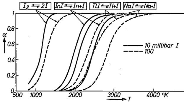
Fig. 5. The degree of dissociation  $\alpha$  of  $I_2$ ,  $InI$ ,  $TlI$  and  $NaI$  as a function of temperature  $T$ , calculated for values of the partial vapour pressure of iodine  $p_I$  of 10 millibars (solid curves) and 100 millibars (dashed curves).
