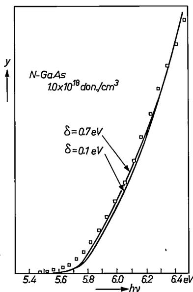
Fig. 11. The yield  $y$  as a function of  $h\nu$  for *N*-GaAs,  $1 \times 10^{18}$  donors/cm<sup>3</sup>, as found theoretically for two values of  $\delta$  and an escape depth  $d$  of 2.0 nm. The experimental points (squares) are the same as in fig. 10. The curves have again been reduced to the same  $y$ -value at  $h\nu = 6.35$  eV.
