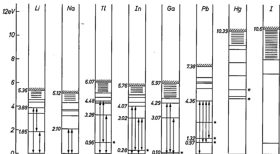
Fig. 3. The principal energy levels of the elements to be used for producing the light. The metastable levels, which cannot be "emptied" by emission, are indicated with an asterisk. It can be seen that Hg and I (apart from a metastable level at 0.94 eV) are more difficult to excite and to ionize than the other elements.
