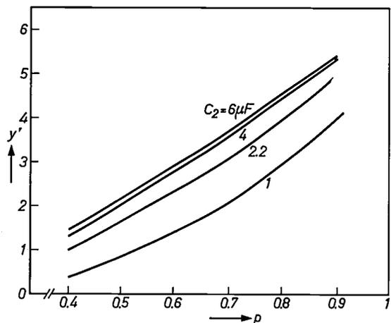
Fig. 16. Since the lower and upper limits for every value of  $C_2$  are found to lie close together (see fig. 15), the lower limits can very suitably be used as an alarm level. These lower limits  $y'$  are shown here for the four values of  $C_2$  as a function of  $p$ .
