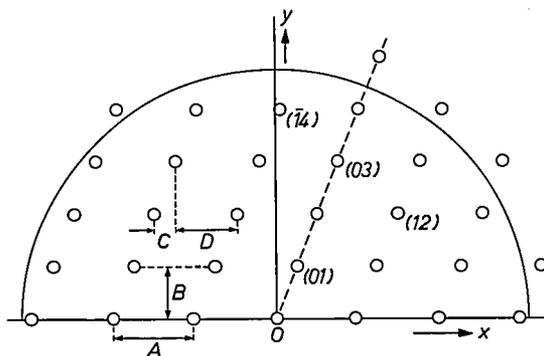
Fig. 10. The reciprocal cell in an *oblique* net can be defined by the parameters  $A$ ,  $B$ ,  $C$  and  $D$  where  $C + D = A$ . For an orthogonal net only the parameters  $A$  and  $B$  are required.
