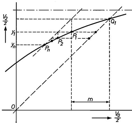
Fig. 4. Effect of identical noise voltages (of magnitude  $m$ ) in a long chain of logic circuits in which the output voltage  $V_2$  of one circuit acts as the input voltage of the next.
