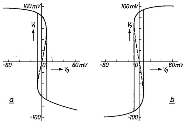
Fig. 6. Measured characteristics a) for  $V_1$  (NOR output) and b) for  $V_2$  (OR output).
