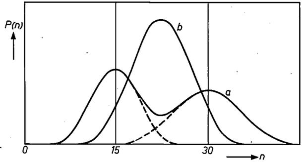
Fig. 11. Illustrating the effect of non-uniformity in the sensitivity of the photocathode on the pulse-height resolution of a photomultiplier.
