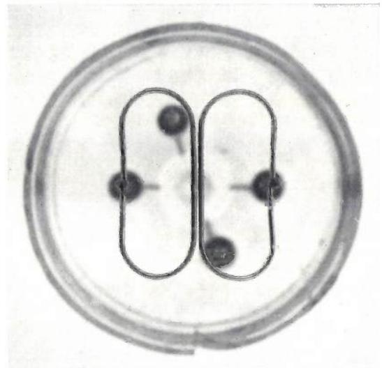
Fig. 4. Cut-away view of the 155 UG, showing the electrodes. The effective part of the electrodes consists of closely-spaced straight pieces of wire at a short distance apart. The electrodes are identical and, since the supply is a.c. they serve alternately as cathode and anode.
