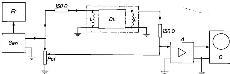
Fig. 10. Circuit that can be used when grinding off a reflecting face in a delay line for setting the correct phase shift. *A* amplifier with very low input impedance. *Pot* potentiometer. *Fr* frequency meter.
