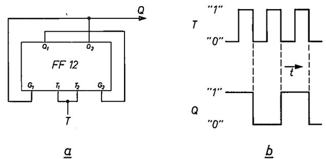
Fig. 6. a) The FF 12 used as a scale-of-two counter. When a series of pulses is applied to point  $T$ , pulses with a period twice as long appear at the output  $Q$ . b) Voltage waveform at points  $T$  and  $Q$ .
