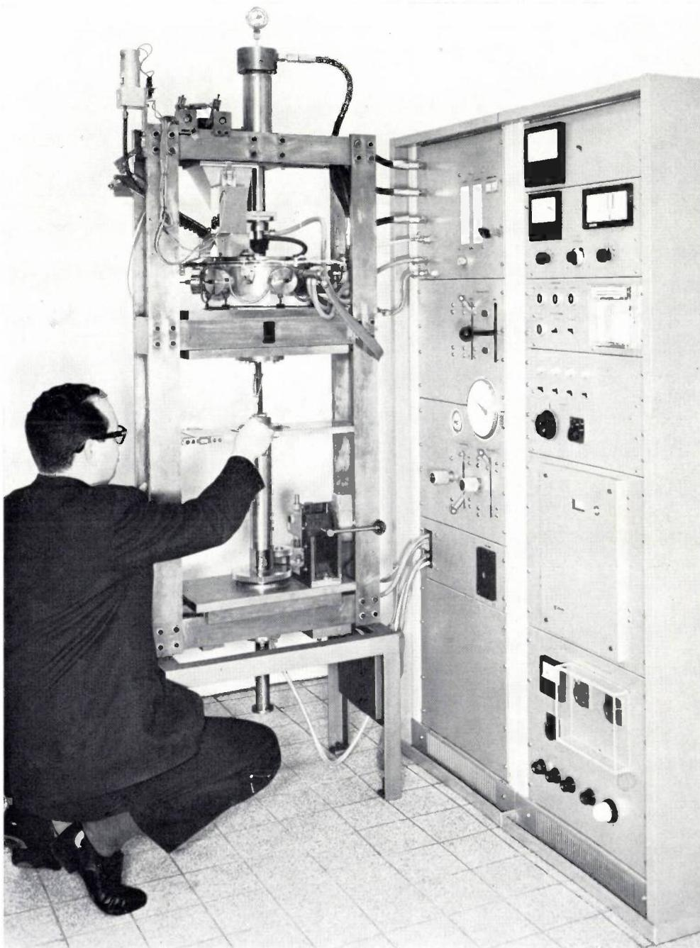
Fig. 2. The equipment at Philips Research Laboratories, Eindhoven, which is used for making ceramic rods by continuous hot pressing.
