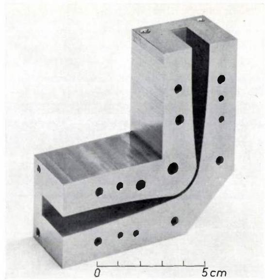
Fig. 15. The 90° *E*-plane bend designed from a “waveguide approach” in which the wave is split up into waveguide modes. Conversion into  $E_{1n}$  and  $H_{1n}$  can occur, but these modes do not propagate in the flat guide provided  $b_1 < \lambda/2$ . In a design for use at  $\lambda \geq 4$  mm the following dimensions were chosen:  $a \times b = 22.86 \times 10.13$  mm,  $r = 420$  mm;  $b_1 = 2$  mm.
