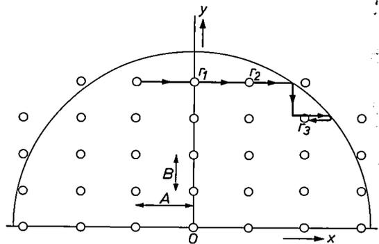
Fig. 9. During automatic data collection the position of the nut ( $P$  in fig. 7) of the linear-tracking mechanism is moved from one reflection site to the next. Reflections are measured in the order in which they occur in reciprocal space in a direction parallel to the  $x$ -axis. After all reflections on one line have been measured, those on the line below it are measured one by one and so on. The semicircle corresponds to the maximum detector angle.
