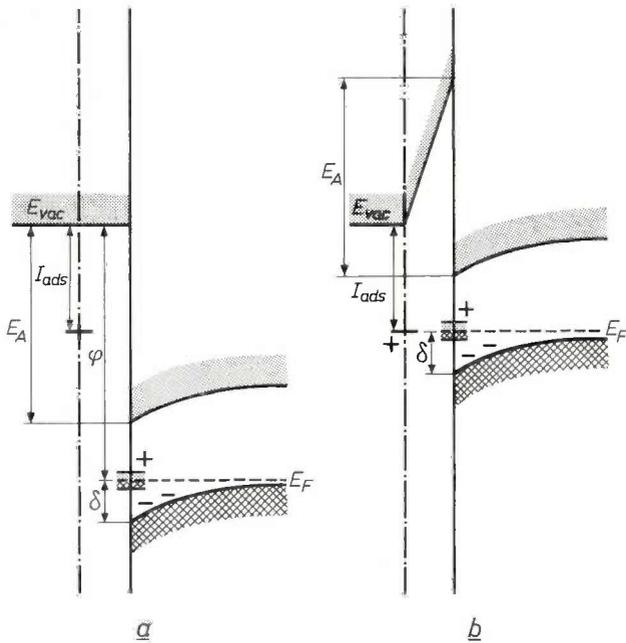
Fig. 14. Adsorption of metal on a  $P$ -type semiconductor with stabilized Fermi level. If the ionization energy  $I_{ads}$  of an adsorbed atom is lower than the work function  $\phi$  of the semiconductor without metal (see a), the metal atoms give up electrons to the surface levels. The dipole layer formed raises the levels in the semiconductor with respect to the vacuum level. In the optimum situation (b),  $\phi$  is again equal to  $I_{ads}$ .
