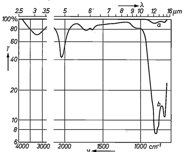
Fig. 12. The spectral dependence of transmission  $T$  of a film consisting of germanium dioxide and germanium hydride on a germanium single crystal.
