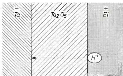
Fig. 6. Current conduction in the forward direction with Ta/Ta<sub>2</sub>O<sub>5</sub> electrodes. This conduction is due to the migration of hydrogen ions through the Ta<sub>2</sub>O<sub>5</sub>. The same thing happens with Al/Al<sub>2</sub>O<sub>3</sub> electrodes.
