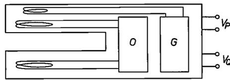
Fig. 15. Diagram of a Vane Switched Oscillator (VSO). The oscillator  $O$ , which operates when a supply voltage  $V_p$  is applied, stops when a metal vane enters the gap between the two coils. The output voltage  $V_Q$  of the rectifier  $G$  then drops from a positive value to zero.
