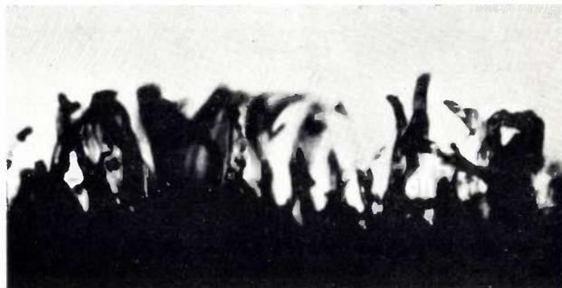
Fig. 6. Molybdenum-oxide crystals, which can form on the electrodes of the 155 UG if the peak current through the tube is too low. Magnification 30x.
