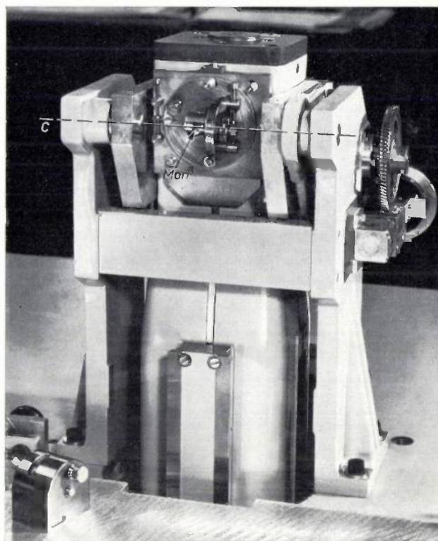
Fig. 15. The X-ray tube housing and the monochromator assembly. The combination can be rotated about the axis *C*. *Mon* monochromator crystal.
