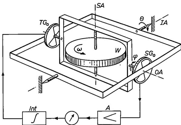
Fig. 8. By inserting an integrator *Int* in the feedback loop the angle of rotation  $\varphi$  about the output axis *OA*, and thus also the signal read on the meter, becomes proportional to the angular acceleration  $\ddot{\theta}$  about the input axis *IA*.
