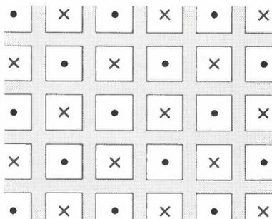
Fig. 3. In the actual heat exchangers there are in fact many channels, not just two as in fig. 2a. The two opposing flows (denoted by crosses and dots) are distributed in such a way that each channel is surrounded by four others carrying the opposite flow.
