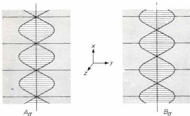
Fig. 2. The two modes  $A_\sigma$  and  $B_\sigma$ , activated by a plane wave linearly polarized in the  $y$ -direction ( $\sigma$ -polarization) and incident exactly at the Bragg angle. The reflecting planes, drawn as thick horizontal lines, are normal to the surface. The modes, which are similarly polarized in the  $y$ -direction, behave as standing waves in the  $x$ -direction and as travelling waves in the  $z$ -direction.
