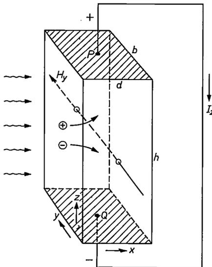
Fig. 6. The photomagnetolectric effect (PME effect) occurs under the same conditions as give the Dember effect (fig. 5) if there is also a magnetic field parallel to the illuminated surface. The PME effect may be regarded as the Hall effect of the two diffusion currents (of holes or electrons respectively). A potential difference appears between the electrodes  $P$  and  $Q$  or, if these are connected, a current  $I_z$  flows in the external circuit.
