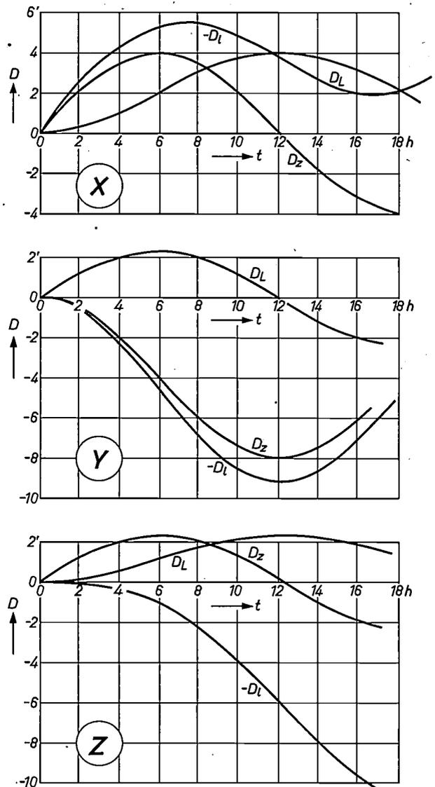
Fig. 18. Recordings of analogue computer investigations on the inertial navigation system. The recordings show the longitude error  $D_l$ , the latitude error  $D_L$ , and the direction error  $D_z$ , all resulting from the application of a step-function gyro drift of  $0.01^\circ/h$  successively to the X-gyro, the Y-gyro and the Z-gyro, as a function of the time  $t$  (in hours). The roll and pitch errors were very small.
