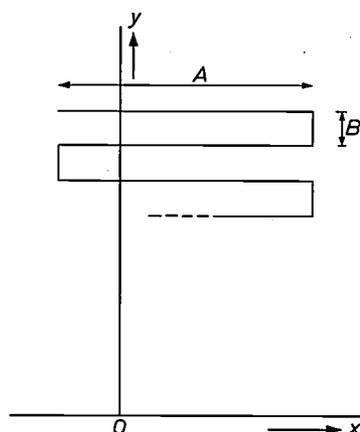
Fig. 26. The lattice scan is a semi-automatic mode of operation. When started positive,  $x$  is increased by  $A$ ,  $y$  decreased by  $B$ ,  $x$  decreased by  $A$ , etc.
