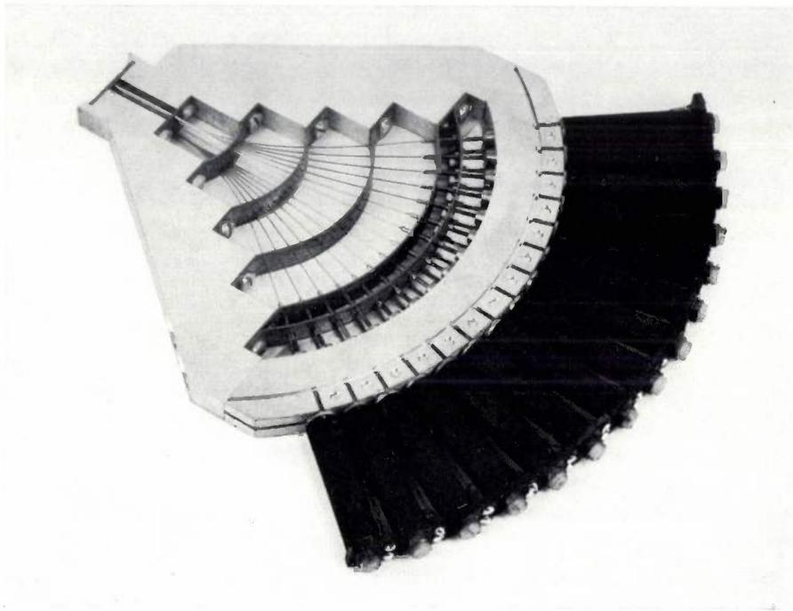
Fig. 14. Unit containing the printing elements for three neighbouring characters in the line printer (15 needles aligned along an axis perpendicular to the general plane of the unit).
