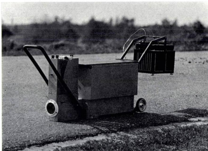
Fig. 9. The reflectometer in position on a road surface.
