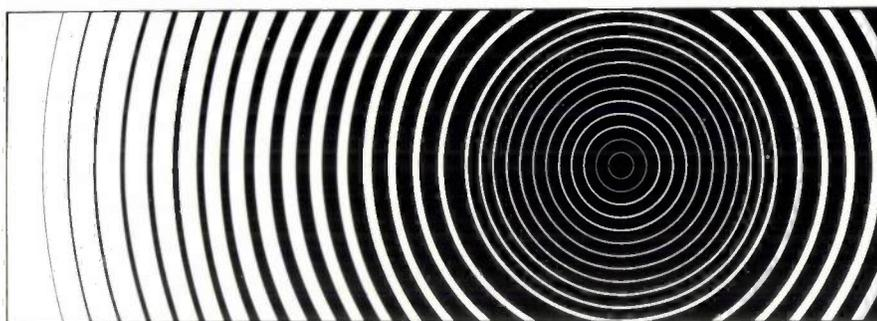
Fig. 8. Mask of opaque circles on the ceiling of the road surface reflectometer. The luminance is measured at the point perpendicularly below the centre of the circles.
