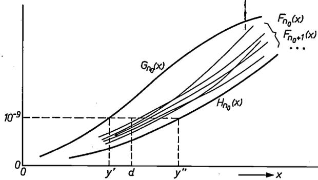
Fig. 14. Determination of the lower limit  $y'$  and the upper limit  $y''$  for the alarm level  $d$ .
