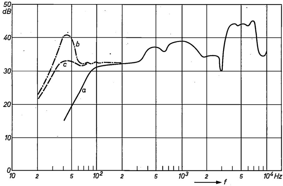
Fig. 11. Amplitude characteristics measured on the system of fig. 7, the loudspeaker being mounted in a completely closed cabinet with a volume of 10 litres, a) without motional feedback, b) with acceleration feedback, c) with both acceleration and velocity feedback.
