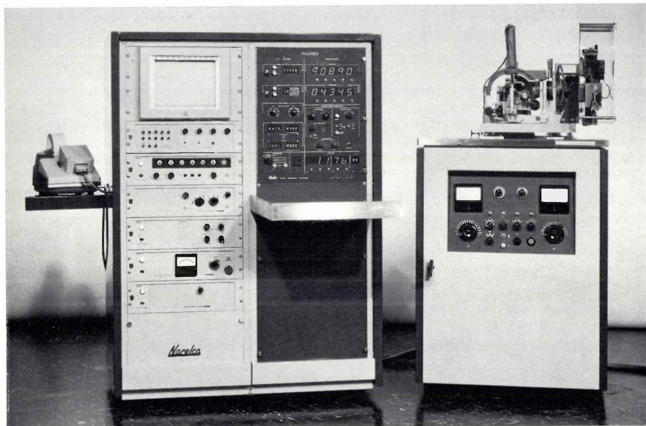
Fig. 1. The heart of the PAILRED automatic single-crystal diffractometer system is the diffractometer, which is located on top of the X-ray generator on the right. The motions of the diffractometer are controlled by automatic control circuits and the X-ray intensities are measured and recorded in the radiation-measuring circuits located in the console on the left.
