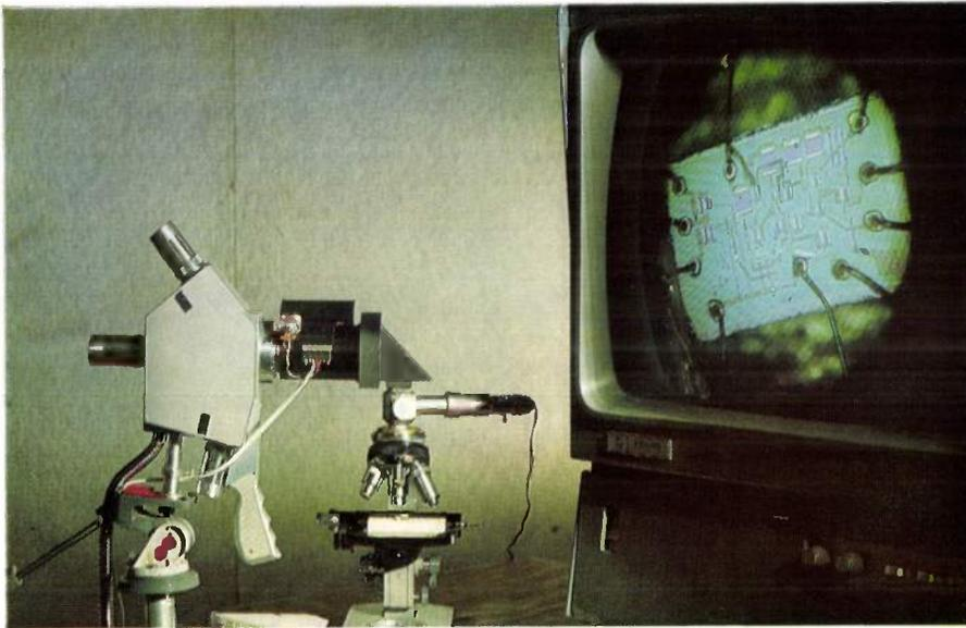
Fig. 1. The miniature camera connected directly to a microscope. The monitor is showing a picture of an integrated circuit which is placed under the microscope.
