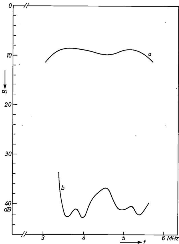
Fig. 12. Insertion loss  $\alpha_1$  as a function of frequency  $f$ ; curve  $a$  for the wanted signal,  $b$  for the unwanted signal due to the  $3\tau$  reflection.
