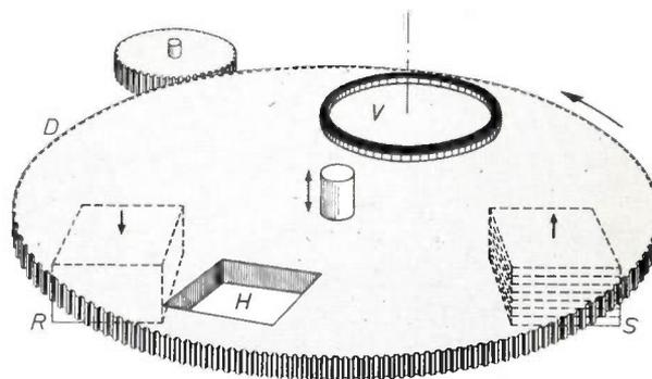
Fig. 11. Schematic representation of plate camera. The toothed disc *D* meshing in a smaller gear is motor-driven. *S* plate magazine. *R* box for receiving exposed plates. *V* vacuum valve. When the opening *H* arrives above *S*, a plate is pushed in. This travels around with the disc into position under the microscope tube, where it is exposed and then dropped into *R*.
