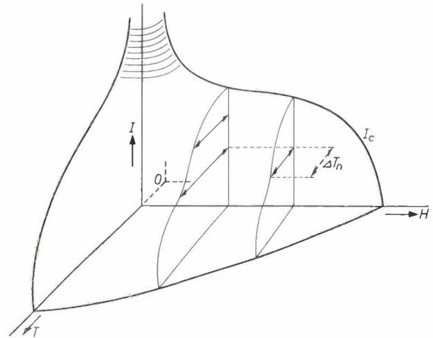
Fig. 8. Schematic representation of the three-dimensional surface in the  $I$ - $H$ - $T$  space inside which the points correspond to the combinations of  $I$ ,  $H$  and  $T$  which give the superconducting state. At a given temperature  $T$  the temperature increment  $\Delta T_n$  which just causes the sample to go normal increases with  $H$  and  $I$ . The  $I$ - $H$  plane (cf. fig. 9) is drawn at the  $T$ -value corresponding to the operating temperature.
