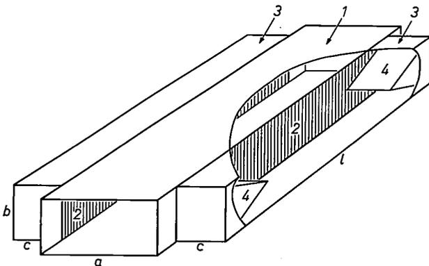
Fig. 12. Filter for the  $H_{30}$  mode. Power in the  $H_{30}$  mode in the main waveguide 1 is transferred by means of dielectric sheets 2 into the  $H_{10}$  mode in the subsidiary guides 3, which is absorbed in the loads 4. For the filter to be effective the phase velocities of  $H_{30}$  in 1 and  $H_{10}$  in 3 must be equal, i.e.  $c$  must be equal to  $a/3$ .
