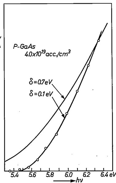
Fig. 12. As fig. 11, but now for *P*-GaAs,  $4 \times 10^{19}$  acceptors/cm<sup>3</sup>. Only a few of the corresponding experimental points of fig. 10 are shown (the circles). The zero point of the theoretical curve (i.e. the threshold energy  $E_A$ ) for  $\delta = 0.7$  eV is at  $E_A + E_g - \delta = 5.57 - 0.7 = 4.87$  eV.
