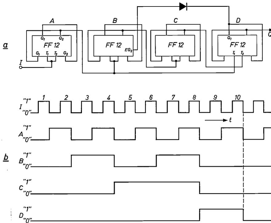
Fig. 8. a) A decade counter derived from the scale-of-16 counter of *fig. 7* by the addition of a feedback diode. b) Voltage waveform at the circuit input  $I$  and at the outputs of the four stages  $A$ ,  $B$ ,  $C$  and  $D$ . For every ten input pulses a single pulse appears at the output of  $D$ , and this can be passed to the next counter unit which therefore indicates the tens.
