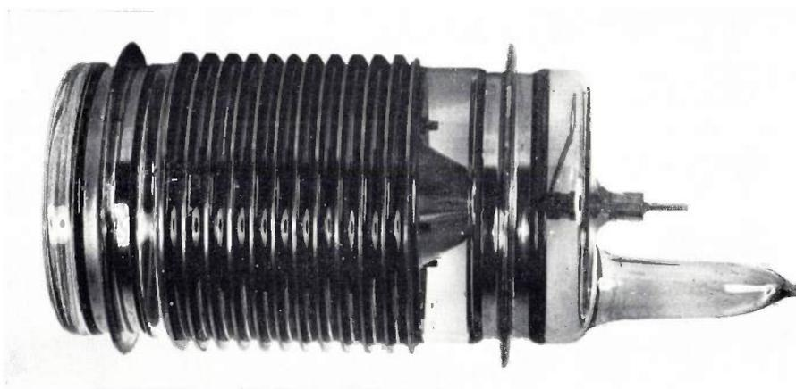
Fig. 17. Experimental photomultiplier type PM 994, used for the heterodyne detection of modulated light. Total length 14 cm.
