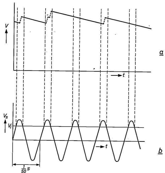
Fig. 8. Illustrating the variation of the output voltage  $V$  of the circuit in fig. 7 as a function of time (a). The waveform of the supply voltage  $V_s(t)$  is shown in (b). A UV photon incident on the tube can initiate a discharge in those parts of the cycle in which  $V_s$  is greater than the ignition voltage  $V_i$  of the tube. On account of the statistical character of this process there is a fluctuation in  $V(t)$ .
