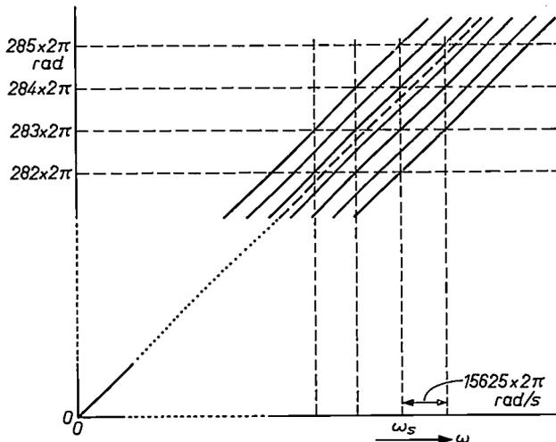
Fig. 5. Phase characteristics of the delay line. For all lines the group delay is  $64 \mu\text{s}$ . The dashed line for the subcarrier does not correspond to a phase shift amounting to an integral multiple of  $\pi$  rad and therefore cannot be used. The solid lines satisfy the necessary conditions.
