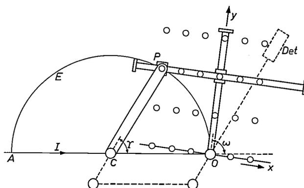
Fig. 7. The Ewald construction can be performed with a mechanical device constituting an  $x, y$ -coordinate system. The nut  $P$  slides along the  $x$ -axis, which in turn can slide in the  $y$ -direction. The nut can be positioned by means of motors and lead-screws to the desired  $x$ - and  $y$ -coordinates in the reciprocal  $x, y$ -plane. When  $OP$  corresponds to the reciprocal vector of a given crystal plane ( $hk$ ) this plane is then in the reflecting position.
