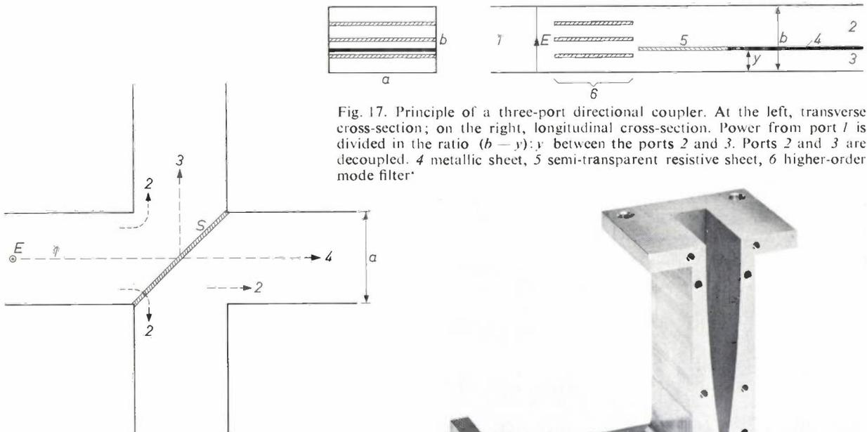
Fig. 17. Principle of a three-port directional coupler. At the left, transverse cross-section; on the right, longitudinal cross-section. Power from port 1 is divided in the ratio  $(b - y) : y$  between the ports 2 and 3. Ports 2 and 3 are decoupled. 4 metallic sheet, 5 semi-transparent resistive sheet, 6 higher-order mode filter
