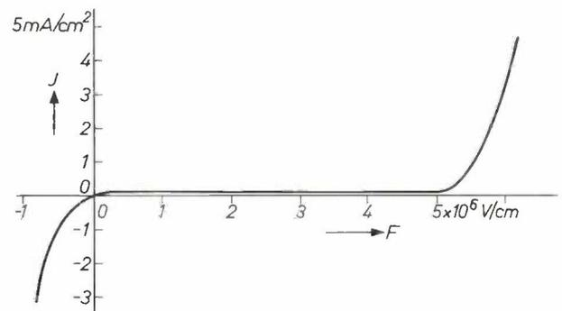
Fig. 4. Current density *J* measured as a function of field strength *F* in an oxide film formed by anodic oxidation of aluminium.
