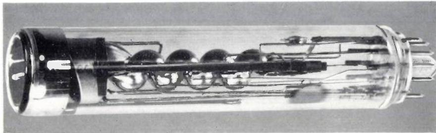
Fig. 20. Small-diameter photomultiplier 152 AVP. Length 10 cm.
