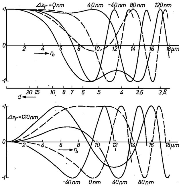
Fig. 7. Contrast transfer curves for the objective lens of the EM 300, derived from the curves of fig. 6; upper curves for amplitude gratings and lower curves for phase gratings.
