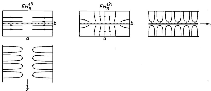
Fig. 10. The electric field pattern of the longitudinal-section (LS) modes with  $m = n = 1$ ,  $EH_{11}^{(1)}$  and  $EH_{11}^{(2)}$ , in a mode filter with one symmetrically located resistive sheet. The LS modes do not undergo mode conversion in a filter of the type of fig. 9.
