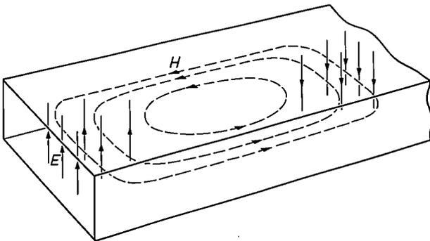
Fig. 1. Field pattern of the  $H_{10}$  mode in rectangular waveguide.
