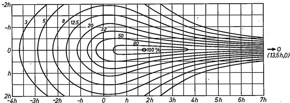
Fig. 3a. Example of a luminance-factor diagram. The light source is at a height h above point (0,0), and the observer is at the point (13.5h,0).
