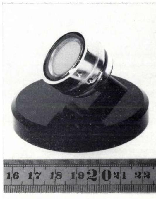
Fig. 18. Ultra-fast photoemissive cell TVHC. It contains a photocathode deposited on a metal disc and a grid-type anode. The distance between these two planar electrodes is about 2 mm, which reduces the transit time of the photoelectrons and hence the duration of the current they induce. This cell is produced by the transfer technique and may be integral with one end of a coaxial cable.
