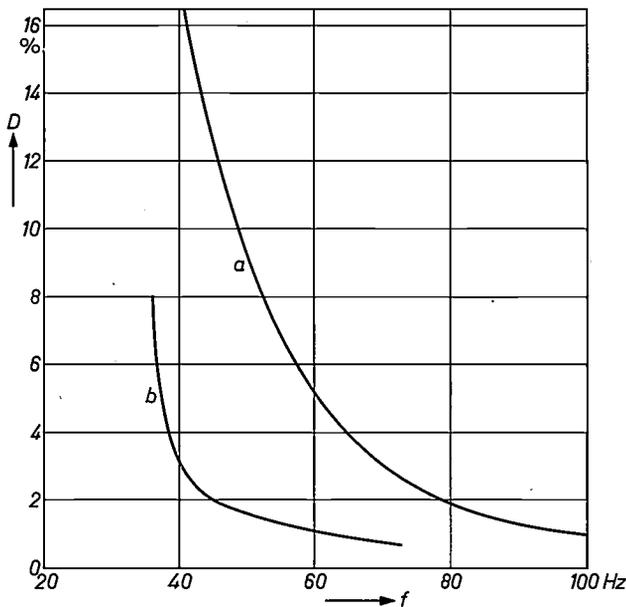
Fig. 13. Non-linear distortion  $D$  as a function of frequency  $f$  for loudspeaker 9710 A.M. The radiated power is kept the same at all frequencies; the electrical power supplied to the loudspeaker is 4.5 W at 40 Hz. Curve  $a$  is obtained with no motional feedback, and curve  $b$  is obtained when acceleration and velocity feedback are combined in such a way as to give the amplitude characteristic  $c$  of fig. 11.
