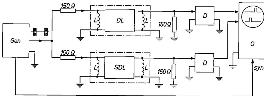
Fig. 9. Diagram for comparing the group delay of any given delay line *DL* with that of a standard delay line *SDL*. *Gen* generator delivering bursts at the frequency of the subcarrier (4 433 619 Hz). *D* detectors. *O* double-beam oscilloscope. *syn* synchronizing signal. *L* coils for compensating the input and output capacitances of the delay lines.
