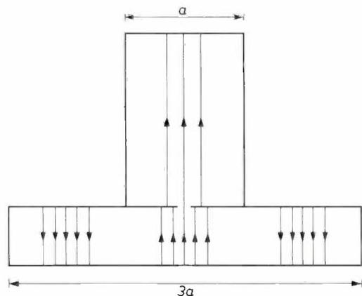
Fig. 8. Transverse cross-section of  $H_{10} \rightleftharpoons H_{30}$  mode transducer. Owing to the equal phase velocities of the  $H_{10}$  mode in the upper guide and the  $H_{30}$  mode in the lower guide, power in one of these modes will be completely transferred into the other in a distance along the guides which depends on the width of the coupling slot.
