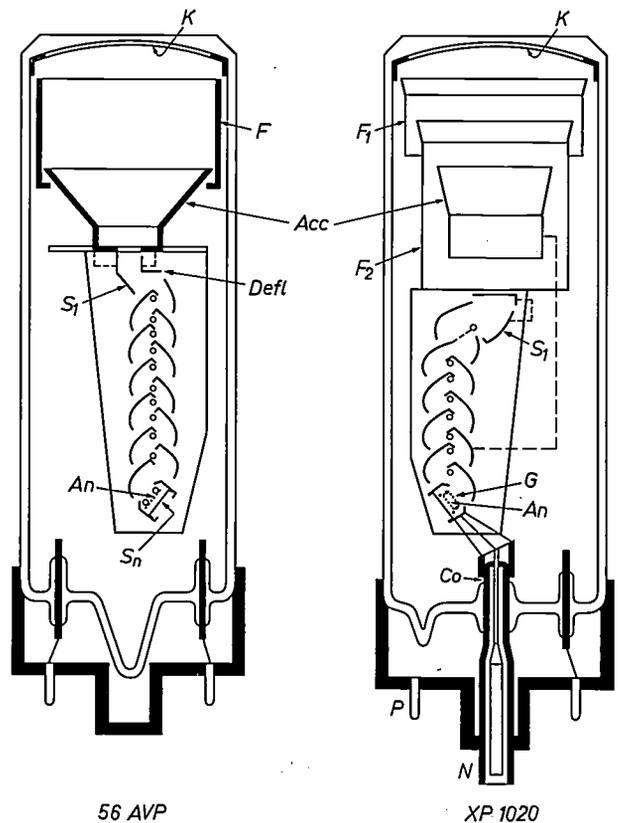
Fig. 14. Section through the 56 AVP and the XP 1020.  $K$  photocathode.  $F_{(1,2)}$  focusing electrodes.  $Acc$  accelerating electrode.  $Defl$  deflector.  $S_{(1...n)}$  dynodes.  $G$  screen grid.  $An$  anode.  $Co$  coaxial feed.  $N$  connection to standard coaxial cable.  $P$  pins.
