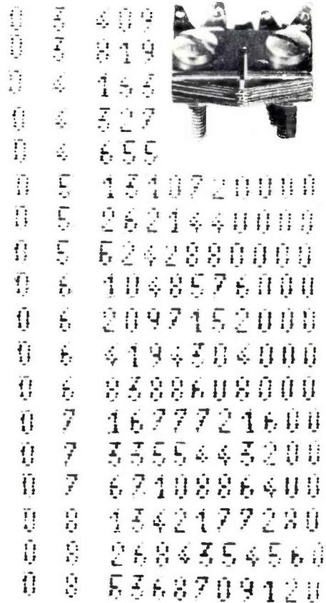
Fig. 5. Thermal printing unit containing 7 printing elements, and figures (results of calculations) printed on thermosensitive paper at a speed of 40 numerals per second in a 4x7 dot mosaic.
