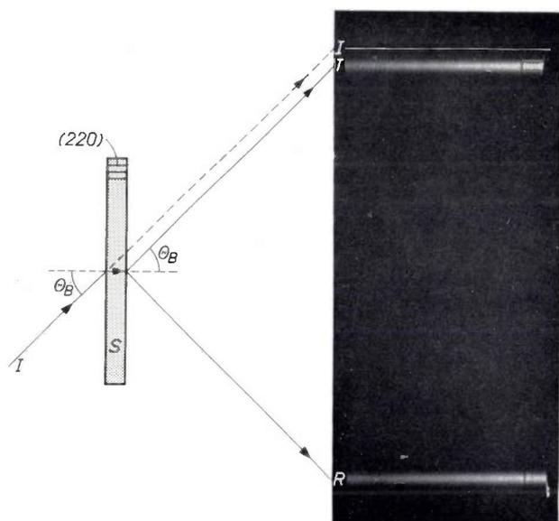
Fig. 1. Anomalous X-ray transmission. The beam geometry on the left explains the image positions seen in the photograph on the right. The X-rays appear to propagate parallel to the diffracting (220) planes.  $I$  incident beam.  $\theta_B$  Bragg angle.  $S$  perfect crystal. The intensities of the reflected beam  $R$  and the transmitted beam  $T$  are much greater than expected from the kinematical diffraction theory.
