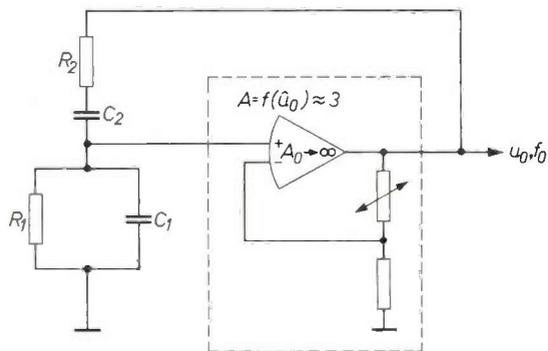
Fig. 1. Wien bridge oscillator, with frequency-determining network consisting of resistors and capacitors. The gain  $A$  required for stable oscillation is controlled by amplitude-dependent negative feedback of a difference amplifier.
