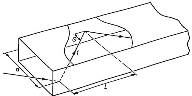
Fig. 11. Filter for the modes  $H_{m0}$  with  $m \geq 2$ . The side walls are made of lossy material. This filter is not ideal in principle as the  $H_{10}$  mode undergoes some attenuation, but the attenuation increases with the mode number  $m$  (cf. eq. 6). To illustrate the derivation of eq. (6) an  $H_{m0}$  mode is represented by the plane wave  $l$  which is reflected in a zigzag path by the narrow walls.
