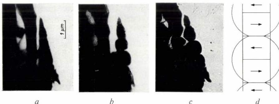
Fig. 5. Electron-photomicrographs of an MnAl particle (dark), *a*) with sharp focus, *b*) with increased focal length. *c*) As (*b*) but with a field of 8000 oersteds, perpendicular to the plane of the drawing. *d*) Domain structure corresponding to the distortion of the needle.
