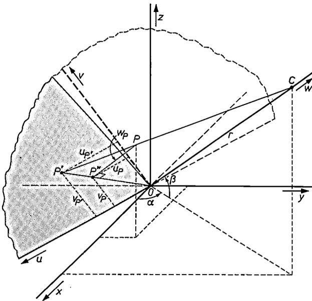
Fig. 3. Diagram for computing the perspective projection  $P'$  of a point  $P$  seen from the centre of projection  $C$ . The projection plane is the plane through  $O$  perpendicular to the line  $CO$ . The  $w$ -axis of a co-ordinate system  $u, v, w$  coincides with  $CO$ , the  $u, v$ -plane with the projection plane. The  $u, v$ -co-ordinates of  $P'$  can be expressed in terms of  $\alpha, \beta, r$  and the  $x, y, z$ -co-ordinates of  $P$ .
