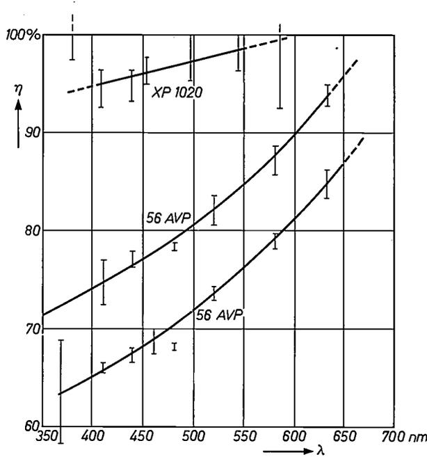
Fig. 15. Variation of collection efficiency  $\eta$  of the 56 AVP (two samples) and the XP 1020 as a function of wavelength.
