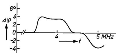
Fig. 13. Phase error  $\Delta\phi$  as a function of frequency.
