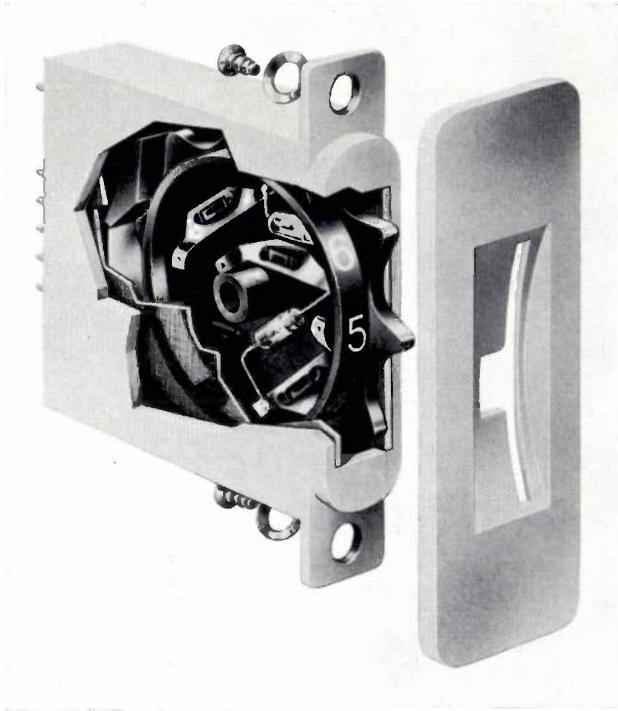
Fig. 10. Cut-away drawing of a thumbwheel switch. When connected to a decade counter, this switch gives a signal when the counter reaches the value to which the wheel has been preset. The diodes of the AND circuit can be seen inside the wheel and also the sliding contacts which make the connections with the counter through code discs on the inside of the case (dimensions 12.7 × 65 × 57 mm).
