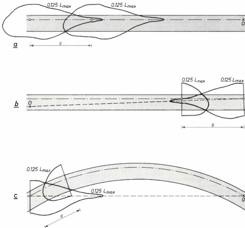
Fig. 6. Isoluminance curves  $0.125L_{\max}$  for two successive lanterns whose spacing  $s$  is such that no point of the road falls *outside* both curves.
