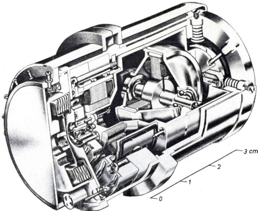
Fig. 11. Cut-away picture of a floating gyro with a single degree of freedom.
