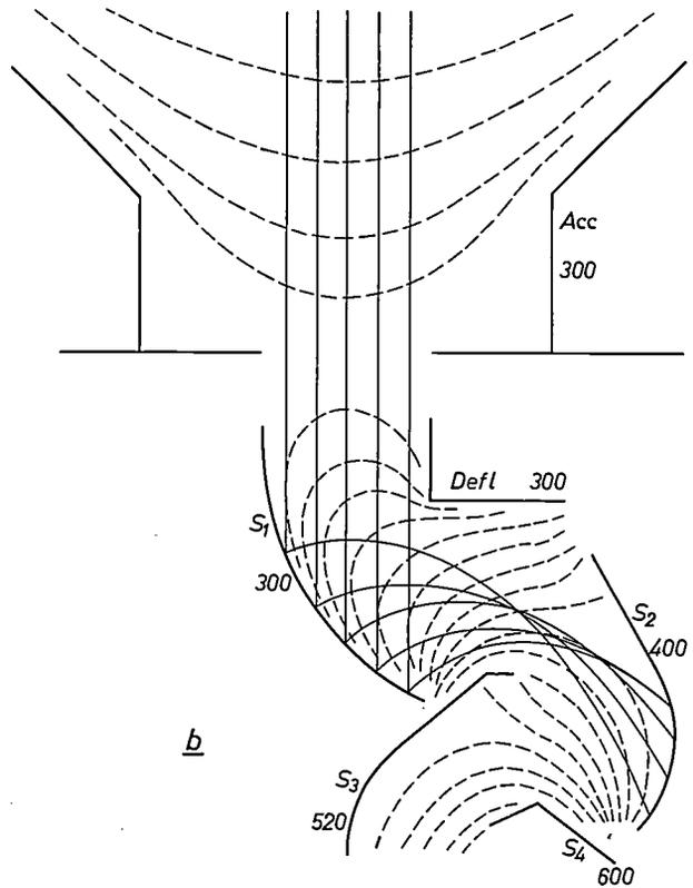
Fig. 12. a) Equipotential surfaces of the input optical system in the 56 AVP. Some paths are shown for electrons coming from the cathode, some without initial velocity and others with an initial transverse velocity corresponding to an energy of 0.3 eV. The diagram gives an indication of the area of the first dynode within which photoelectrons can arrive. (The potential values quoted are relative.)
