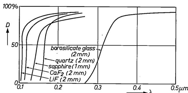
Fig. 7. Optical transmission  $D$  of various windows used in photomultipliers, as a function of wavelength.
