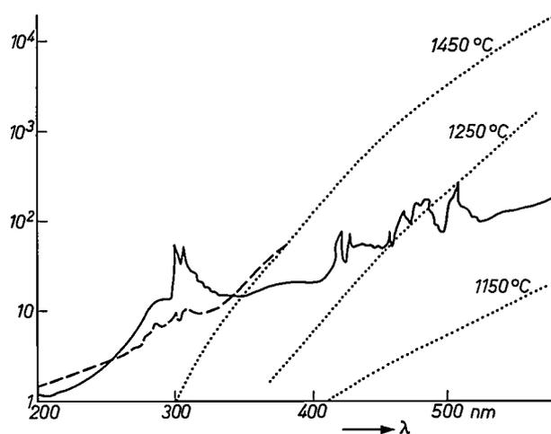
Fig. 1. Spectral intensity distribution (in arbitrary units) of the radiation emitted by a gas flame (solid line), an oil flame (dashed line) and the furnace wall (black-body radiator) at different temperatures (chain-dotted lines).
