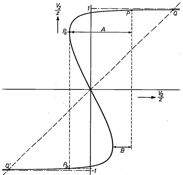
Fig. 3. There are two critical values,  $A$  and  $B$ , for the noise that can occur at an arbitrary operating point  $P$ .
