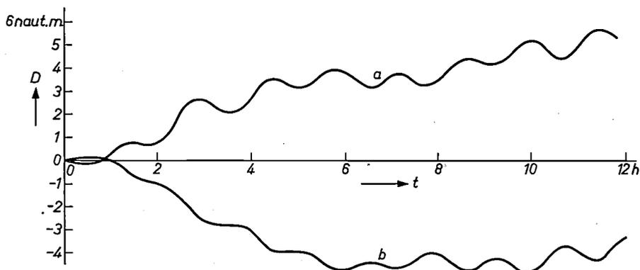
Fig. 19. Errors  $D$  in longitude (a) and latitude (b) during a 12-hour laboratory test. The curves show a half period of a 24-hour oscillation and Schuler oscillations (period 84.4 min). These oscillations are superimposed on a linear gyro drift, which amounts to about 0.5 nautical miles per hour in longitude and 0.3 nautical miles per hour in latitude.
