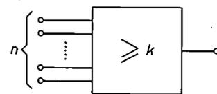
Fig. 8. Block symbol for a threshold-logic circuit. The circuit gives a "1" when  $k$  or more of the  $n$  inputs supply a "1".
