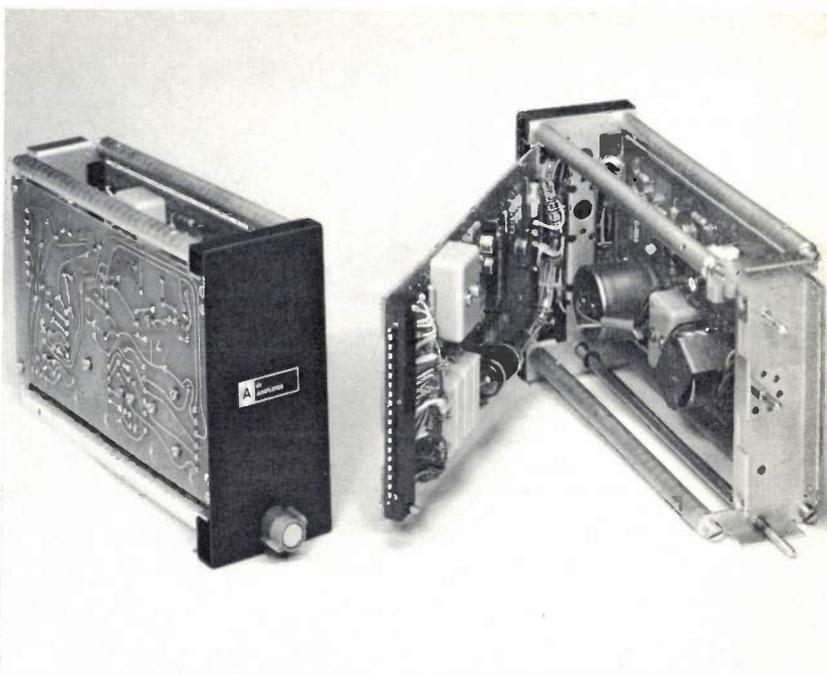
Fig. 15. Standard control amplifier, containing a circuit like that of fig. 14 and a conventional d.c. difference amplifier. The two amplifiers are mounted on printed wiring boards. Note the mu-metal screening around the transformers.
