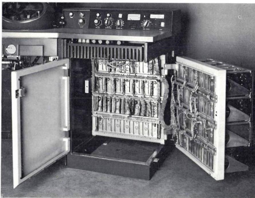
Fig. 13. The electrical circuits are contained in modules that fit into hinged racks.
