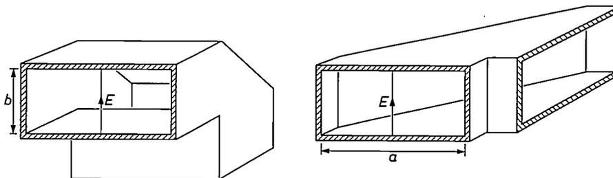
Fig. 14. The  $90^\circ$   $E$ -plane bend (on the left) and the  $90^\circ$   $H$ -plane bend (on the right), designed by the "optical approach", in which the wave propagation is assumed to take place along "rays".
