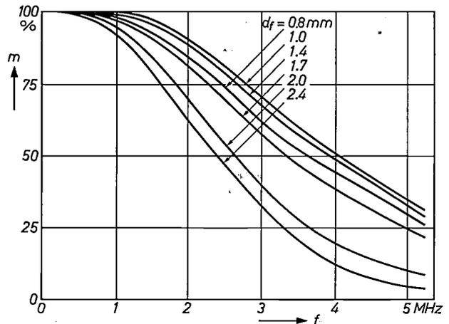
Fig. 7. Modulation depth  $m$  as a function of frequency  $f$  for some values of the diameter  $d_f$  of the beam at the centre of the focusing lens. An optimum value of  $m$  is achieved at  $d_f = 1.0$  mm.
