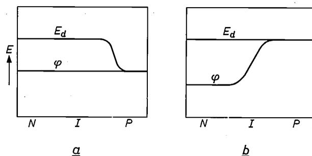
Fig. 2. The threshold energy  $E_d$  for photoemission and the thermionic work function  $\varphi$  as a function of the doping content of a semiconductor, a) in the presence of many surface states at an energy in the forbidden zone, b) in the absence of surface states. From left to right the doping goes from strong N via weak N and weak P to strong P; in the centre (I) the semiconductor is intrinsic.
