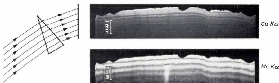
Fig. 5. Fringes corresponding to fig. 4, visible in the intensity reflected from a thin {111} germanium wedge using {220} reflecting planes and  $\text{CuK}\alpha$  or  $\text{MoK}\alpha$  radiation. The fading out of the fringes is due to absorption and the divergence of the incident beam. The angle of the wedge is  $1^\circ 55'$ .
