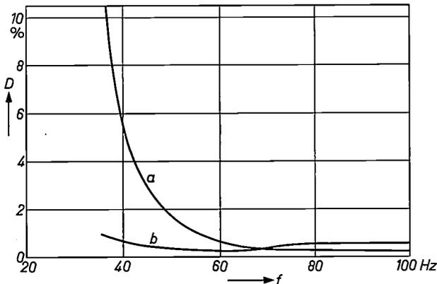
Fig. 14. Non-linear distortion  $D$  as a function of frequency  $f$  for the bass loudspeaker 9710 A under the same conditions as for fig. 14,  $a$ ) without motional feedback,  $b$ ) with motional feedback adjusted to obtain the amplitude characteristic  $d$  of fig. 12.
