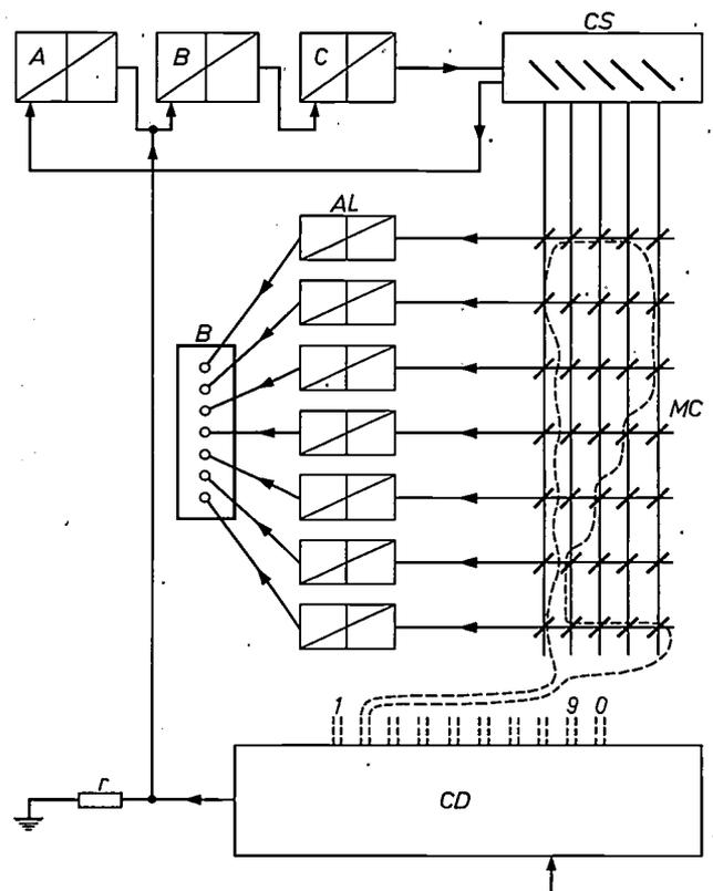
Fig. 11. Diagram of electronic circuits for the serial printer. The wire indicated by the dotted line forms the figure "2" in the mosaic matrix *MC*; there is a corresponding wire for each figure. *B* printing block for a vertical column of 7 dots (illustrated in fig. 10). *AL* read amplifiers, which control the electromagnets of the 7 needles located in *B*. *CD* decoder. *CS* scanning circuit controlled by a series of monostable circuits *A*, *B*, *C*, which give a suitable delay.
