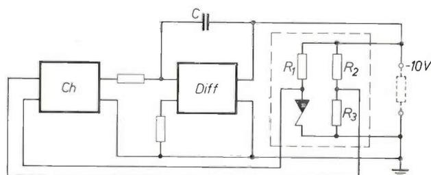
Fig. 16. Generator for the central reference voltage. *Ch* chopper amplifier. *Diff* difference amplifier (see fig. 15). The dashed line encloses a bridge circuit consisting of three resistors and a Zener diode, housed in a thermostat. *C* feedback capacitor for the suppression of fast fluctuations.
