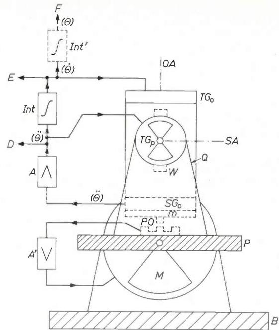
Fig. 10. Layout of a RAMP with slaved platform. The pendulum axis (input axis of the gyro) is perpendicular to the plane of the figure.  $B$  base. The pendulum is carried on a frame  $Q$  on a platform  $P$ , which follows the pendulum with the aid of the signal generator (pick-off)  $PO$ , the amplifier  $A'$  and the servomotor  $M$ .
