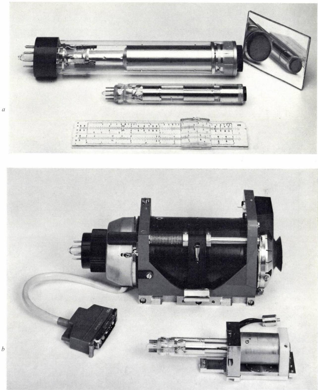
Fig. 2. a) Standard and miniature "Plumbicon" tubes. The dimensions of the tubes are  $200 \times 30$  mm and  $130 \times 16$  mm. b) The tubes mounted in their deflection coils.
