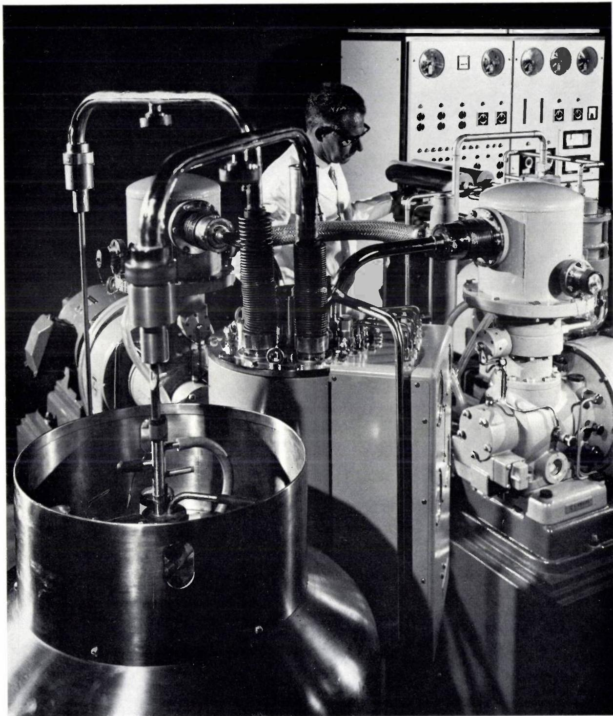
Fig. 5. The Philips helium liquefier. One Philips two-stage gas-refrigerating machine is to be seen on the left in the background and another can be seen at the far right. A Dewar vessel in which the liquid helium is collected and removed can be seen in the foreground. The compressor is behind the right-hand refrigerating machine. The cryostat is at the centre of the picture; the cabinet attached to it on the right contains meters for registering temperatures and pressures.
