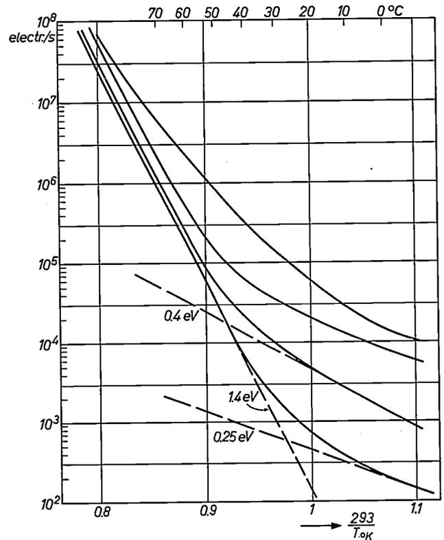
Fig. 8. Variation of the dark current (number of electrons per second) as a function of temperature  $T$  for various photomultipliers. The slope at low temperatures corresponds to a much lower work function (shown in eV) than that at high temperatures.
