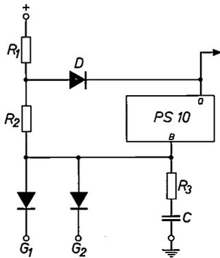
Fig. 14. Square-wave oscillator. As long as  $V_B$  is low and  $V_Q$  is at the "1" level, charge flows into  $C$  through  $R_1$ ,  $R_2$  and  $R_3$ . When  $V_B$  has risen to a value at which  $V_Q$  goes to the "0" level,  $C$  discharges through  $R_3$ ,  $R_2$  and  $D$  until  $V_B$  has fallen far enough for  $V_Q$  to return to the "0" level. The oscillation can be stopped by bringing  $G_1$  or  $G_2$  to the "0" level.
