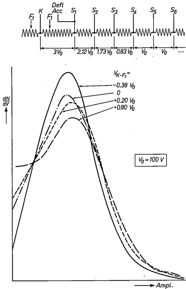
Fig. 13. Effect on the single-electron spectrum of deliberate defocusing by altering the potentials of the input optical system in the 56 AVP. The diagram at the top shows the distribution of the potentials on the different electrodes. Beginning with  $S_4$ , the voltage between successive dynodes is equal to  $V_0$ . The curves 1 to 4 were obtained for four different values of the voltage between photocathode  $K$  and focusing electrode  $F_1$ .
