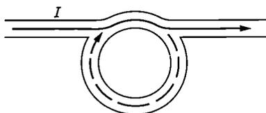
Fig. 9. Buckingham "persistatron". A current  $I$  strong enough to remove superconductivity locally is passed through part of a superconducting ring. The magnetic flux contained by the ring during the flow of  $I$  is enclosed when  $I$  is switched off.
