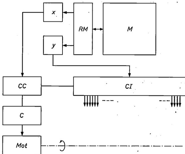
Fig. 19. Block diagram of the electronic circuits of the curve plotter. *M* store in which the co-ordinates of all the points of the family of curves to be plotted are entered. *RM* word register. *CI* printing control circuits. *CC* comparator. *C* counter. *Mot* paper-drive motor.
