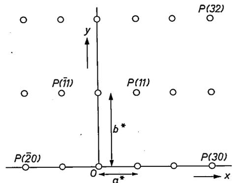
Fig. 5. The end points  $P$  of the reciprocal vectors of planes ( $hk$ ) form a regular repetitive array in what is called reciprocal space. Just as in the case of direct space (fig. 3), the array has a unit cell which is called the reciprocal cell. The  $x$ - and  $y$ -axis of reciprocal space lie in the direction of the edges  $a^*$  and  $b^*$  of the reciprocal cell. ( $\bar{2}$  denotes  $-2$ .)
