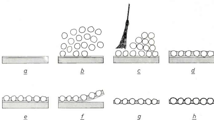
Fig. 1. Diagram showing successive stages in the manufacture of sheets containing monograin layers. *a*) An adhesive is applied to a substrate. *b*) Powder is sprinkled on to it. *c*) The loose, surplus grains are brushed off. *d*) A thermosetting resin is applied. *e*) The top layer is etched away. *f*) The resin is hardened and the resultant sheet is stripped from the substrate. *g*) The adhesive is dissolved and *h*) a thin metal film is deposited on both sides of the sheet.
