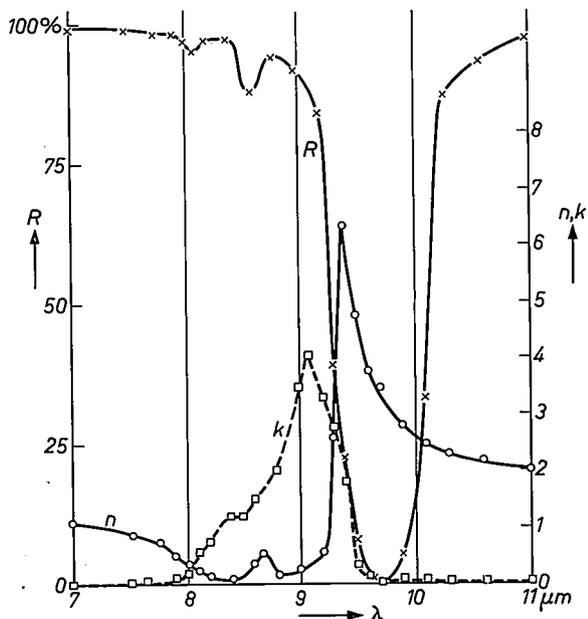
Fig. 6. Change of  $n$  and  $k$  with wavelength for  $\alpha$ -quartz (from [8]). The reflectivity  $R$  has been calculated from these values as a function of wavelength [9] for total reflection at the boundary between silicon and silicon dioxide with an angle of incidence of 45°. The rarer medium (silicon dioxide) has been assumed to extend to infinity.
