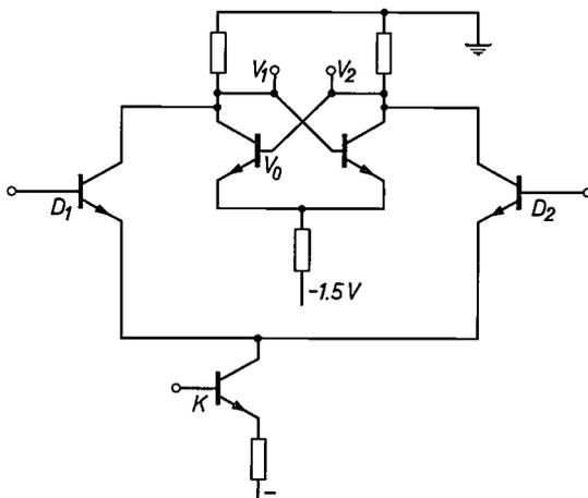
Fig. 10. The basic circuit as a "clocked" storage element. The circuit has two stable states. Which one it assumes can be controlled by making one of the input transistors  $D_1$  or  $D_2$  conduct. The configuration is such that the transistors  $D_1$ ,  $D_2$  can only operate when transistor  $K$  is conducting, during the period of a positive "clock pulse".
