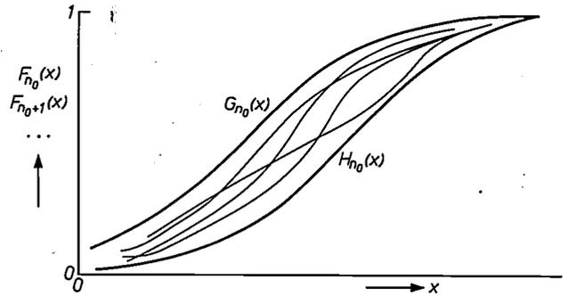
Fig. 13. To approximate to the alarm level, two distribution functions  $G_{n_0}(x)$  and  $H_{n_0}(x)$  are determined which, for every value of  $x$ , are respectively larger and smaller than all functions  $F_n(x)$  for  $n \geq n_0$ .
