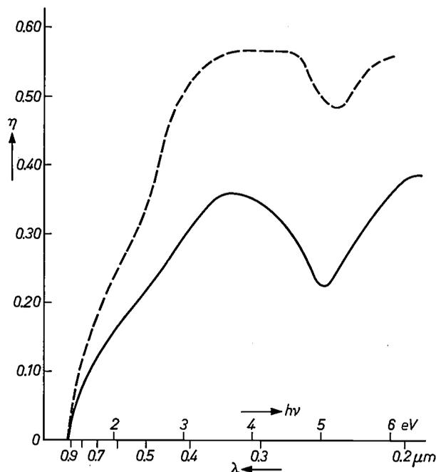
Fig. 18. Spectral distribution of  $\eta$ , the yield per photon, of the photoemission of *P*-type GaAs ( $3 \times 10^{19}$  acceptors/cm<sup>3</sup>) coated with Cs. The solid curve gives the yield in electrons per incident photon, the dashed curve the yield in electrons per absorbed photon.
