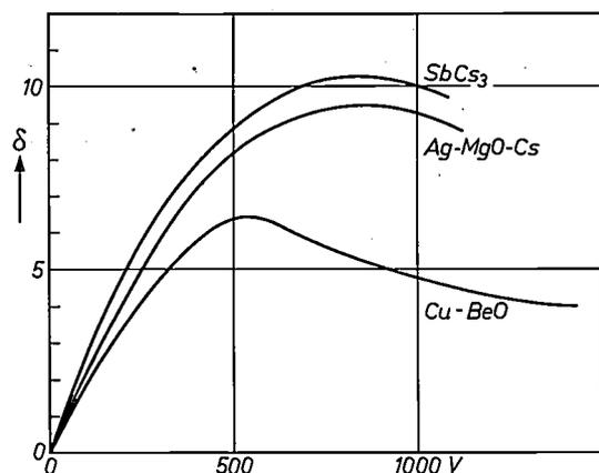
Fig. 4. Variation of the coefficient of secondary emission  $\delta$  as a function of the energy of the primary electrons, for various materials.
