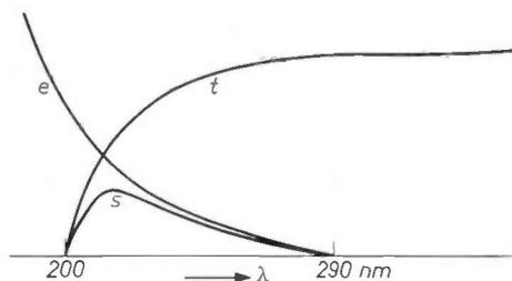
Fig. 3. General spectral distribution of the sensitivity  $s$  of the detector, derived from the quantum efficiency  $e(\lambda)$  of the photoelectric effect at the electrode and the transmission  $t(\lambda)$  of the glass bulb.
