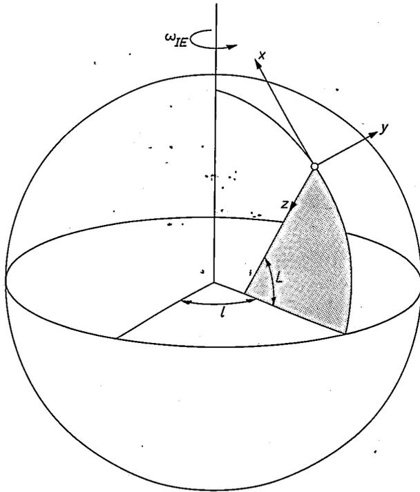
Fig. 26. Geographically orientated co-ordinate system  $x, y, z$ , pointing north, east and downwards.  $l$  longitude.  $L$  latitude.  $\omega_{IE}$  rotation speed of the Earth.
