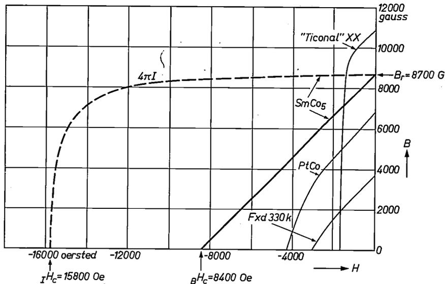
Fig. 1. Flux density  $B$  (solid line) and magnetization  $4\pi I$  (dashed line) of the magnet of  $\text{SmCo}_5$  as a function of the demagnetizing field strength  $H$ . For comparison the  $B$ - $H$  curves for "Ticonal" XX, ferroxdure 330 k and platinum cobalt are also drawn (thinner curves).
