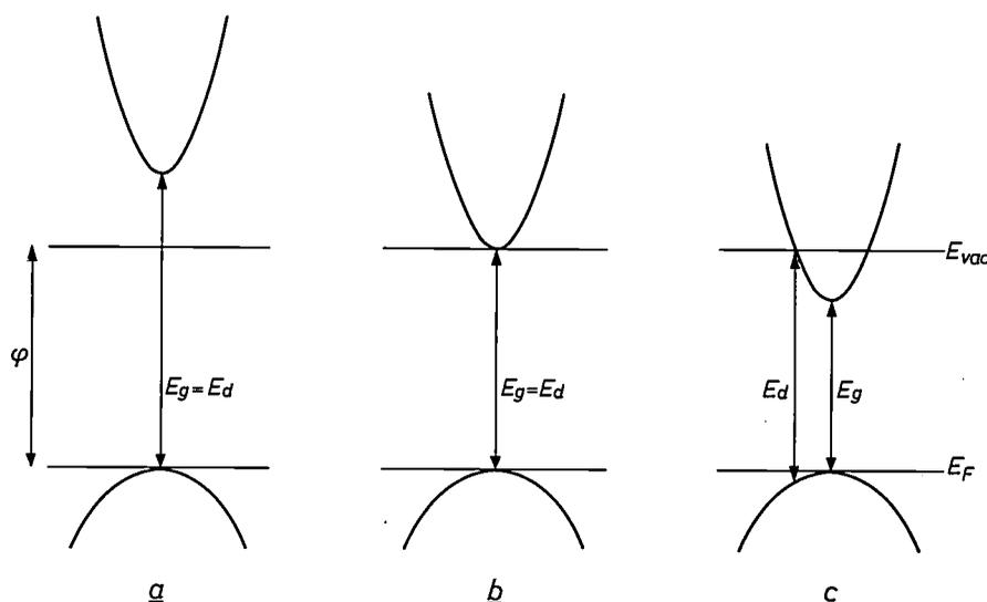
Fig. 17. *P*-doped semiconductors with a simple band structure, with the same value of  $\phi$  (given by the deposited metal) but with different optical energy gap  $E_g$ . a)  $E_g > \phi$ , b)  $E_g = \phi$ , c)  $E_g < \phi$ . Only in case (b) is the threshold for direct transitions equal to  $\phi$ ; both in (a) and (c) the threshold  $E_d$  is greater than  $\phi$ .
