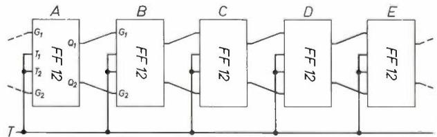
Fig. 12. Shift register built up from FF 12 circuit blocks. The outputs  $Q_1$  and  $Q_2$  of each block are connected to the condition inputs ( $G_1$  and  $G_2$ ) of the next bistable circuit. When a pulse appears on the common trigger input *T*, bistable circuit *B* will take over the state of *A*, *C* the state of *B*, and so on, thus shifting the contents of the register one place to the right.
