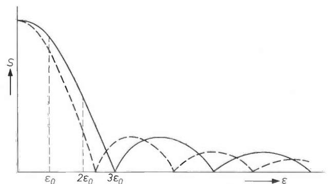
Fig. 8. Magnitude of the signal *S* delivered by a transducer as a function of the angle of incidence  $\epsilon$  of the ultrasonic waves. At a particular angle  $\epsilon_0$  the angle of incidence  $3\epsilon_0$  of the  $3\tau$  reflection is such that the transducer is insensitive to it at the frequency corresponding to the solid curve. At other frequencies (dashed curve) and the same value of  $\epsilon_0$  this does not apply.
