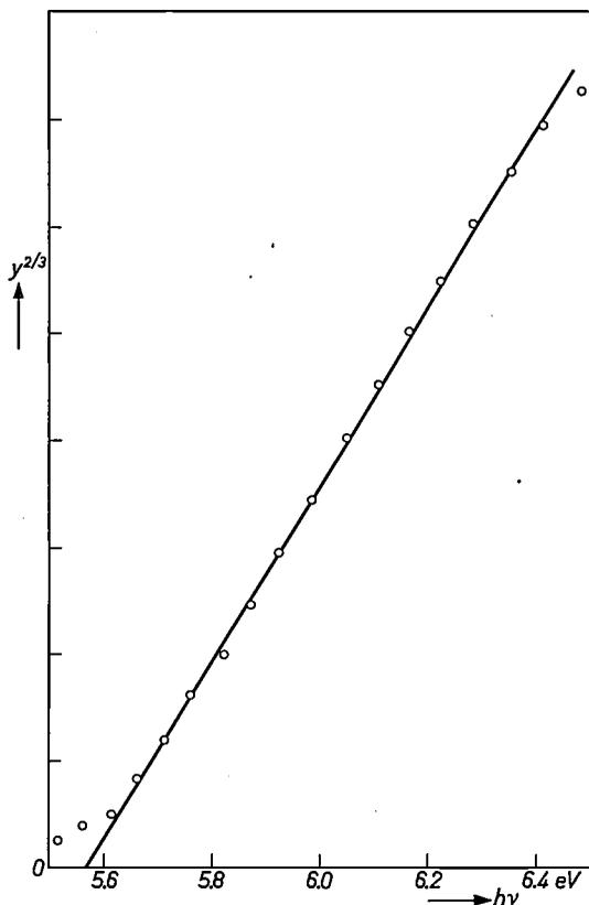
Fig. 9. Photoemission of GaAs with weak *P*-type doping ( $2.5 \times 10^{17}$  acceptors/cm<sup>3</sup>). The  $2/3$  power of the yield  $y$  is given as a function of photon energy  $h\nu$ . The tail emission is of little significance.
