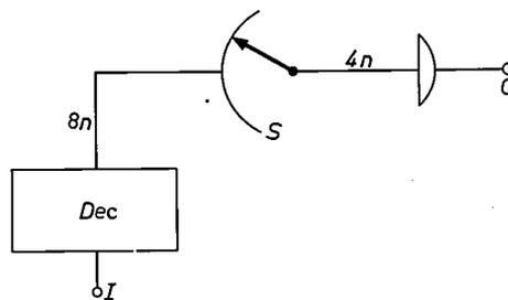
Fig. 20. A symbolic representation for a decade counter *Dec* containing  $n$  decades (i.e.  $4n$  bistable circuits), together with a sensing circuit that will give an output at *O* when the counter reaches the state that was selected by a bank of  $n$  10-position switches, *S*. The AND gate has  $4n$  inputs, one from each bistable circuit, and is partially contained in the switches. *I* is the pulse input.
