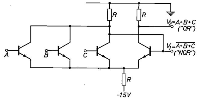
Fig. 7. The basic circuit used as NOR/OR circuit for high voltages (i.e. in "positive logic").
