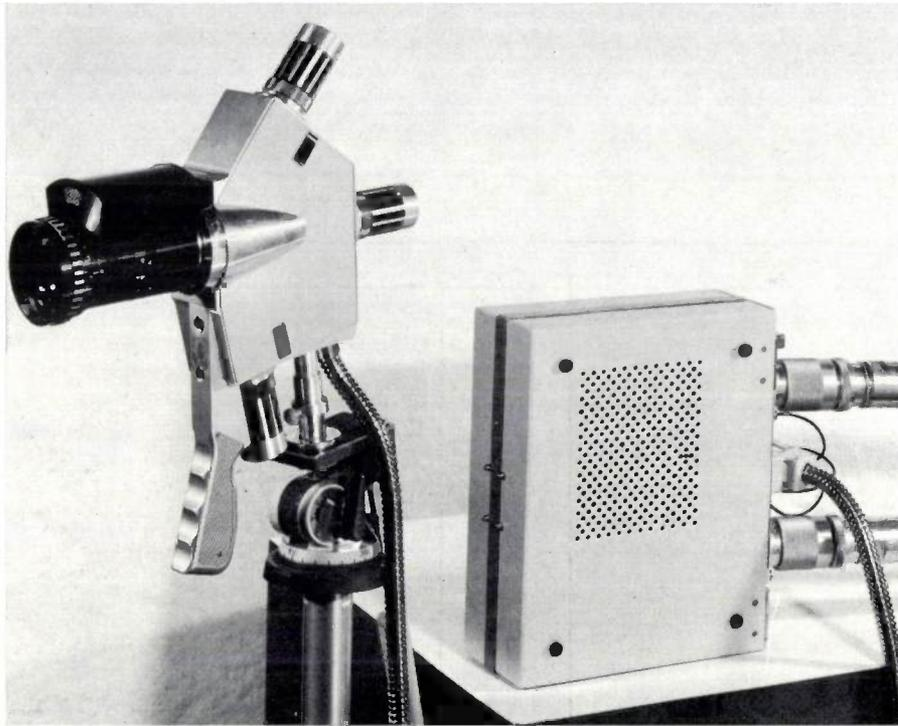
Fig. 11. The miniature camera with the "intermediate unit", which measures  $28 \times 24 \times 10$  cm.
