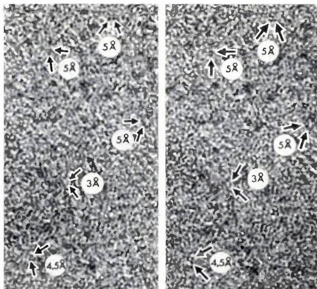
Fig. 3. Two photomicrographs of the same specimen in which details situated 5 Å apart can be distinguished. The fact that the same features are seen on both exposures proves that they are not grains from the photographic emulsion.
