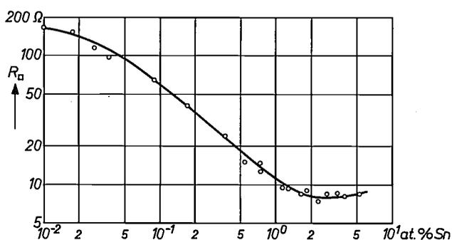
Fig. 1. Resistance per square of indium oxide films as a function of tin doping at room temperature. Spraying temperature 500 °C; film thickness 0.32  $\mu\text{m}$ .
