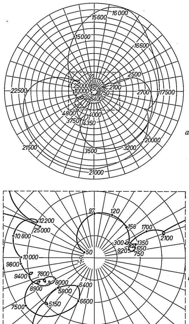
Fig. 8. a) Nyquist diagram for a feedback system like that of fig. 7 when the filter *F*<sub>1</sub> and the integrator *Int* are not included in the circuit. The feedback is made so large that the resonant frequency — 97 Hz without feedback — is shifted to 42 Hz. The figures along the curve indicate the frequency in Hz. Since the curve encloses the point  $-1$ , this system is not stable. b) A magnified view of the region bounded by the dashed line in (a).
