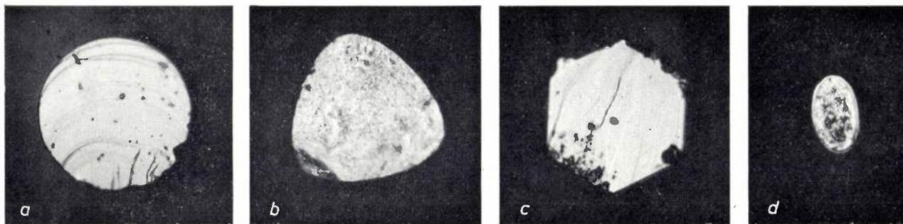
Fig. 2. *a, b, c*) Cross-sections of silicon-carbide whiskers as shown in fig. 1. For comparison, *d*) shows the cross-section of a human hair (magnification 500 $\times$ ).
