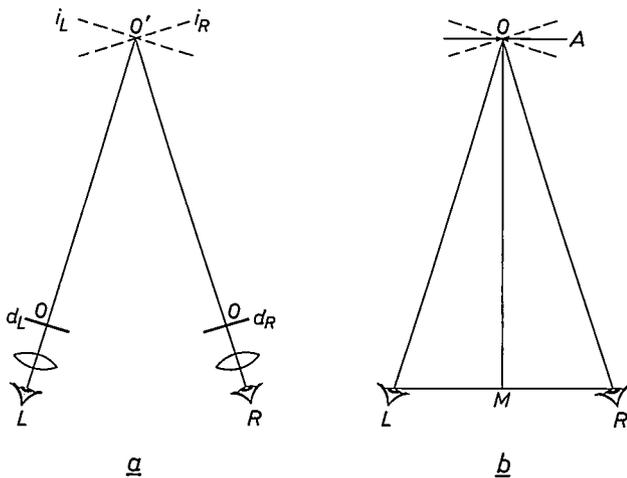
Fig. 8. a) Schematic diagram of a stereoscope.  $L$  and  $R$  are the viewer's eyes. The stereo drawings  $d_L$  and  $d_R$  are observed with the aid of lenses; the eye sees images of these projections at  $i_L$  and  $i_R$ . b) Arrangement of the eyes  $L$  and  $R$  when viewing the anaglyph  $A$ .
