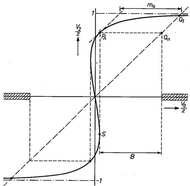
Fig. 5. Optimum shape of the characteristic of the basic circuit. The turning-point  $S$  must lie vertically beneath the point  $P_n$  where the slope is unity. The maximum noise margin is  $m_0 = P_n Q_n$ .
