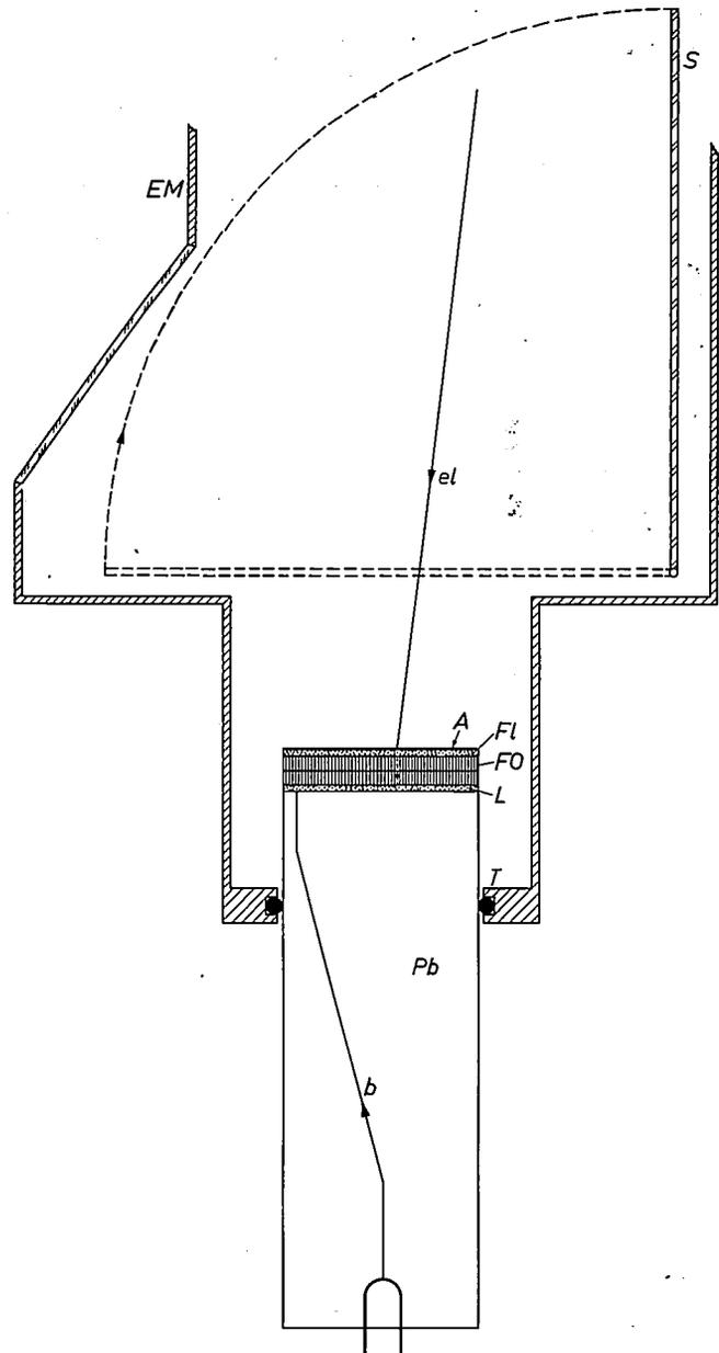
Fig. 1. The fluorescent layer *Fl* converts the electron image into an optical image, which the fibre optics *FO* transmit to the light-sensitive electrode *L* in the "Plumbicon" tube *Pb*. *A* aluminium film. *el* imaging electron beam in the electron microscope. *b* scanning beam of the "Plumbicon" tube. *T* vacuum-tight feed through the wall of the electron microscope *EM*. *S* is the ordinary fluorescent screen, here swung out of the beam.
