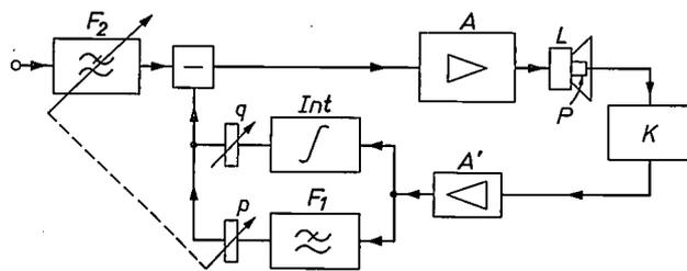
Fig. 7. Block diagram of a circuit for applying motional feedback to a full-range loudspeaker. *A* output amplifier (output power 10 W). *L* loudspeaker. *P* acceleration transducer. *K* cathode follower. *A'* amplifier. *F*<sub>1</sub> and *F*<sub>2</sub> low-pass filters. *Int* integrator. *p* and *q* variable attenuators.
