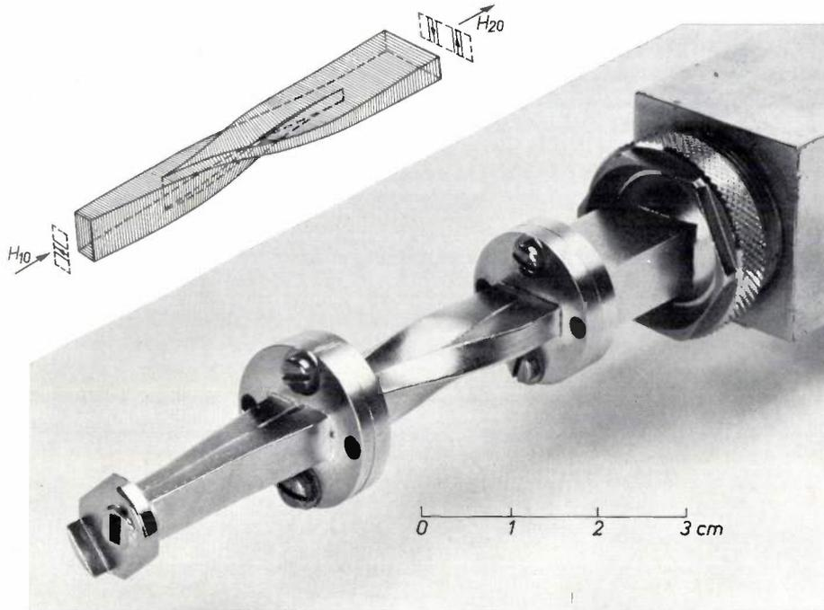
Fig. 7.  $H_{10} \rightleftharpoons H_{20}$  mode transducer.
