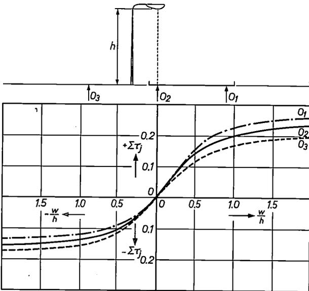
Fig. 11. Graph of  $\Sigma\tau_j$  plotted on the transverse cross-section of the standard installation (*fig. 10*). These curves apply to the lantern whose light distribution is given in *fig. 4* and a road surface of class II. Above the graph there is a diagram of the design used for the calculated example in the text, in the correct situation with respect to the graph and to the correct scale. There are three curves for the three observation positions  $O_1$ ,  $O_2$  and  $O_3$ .
