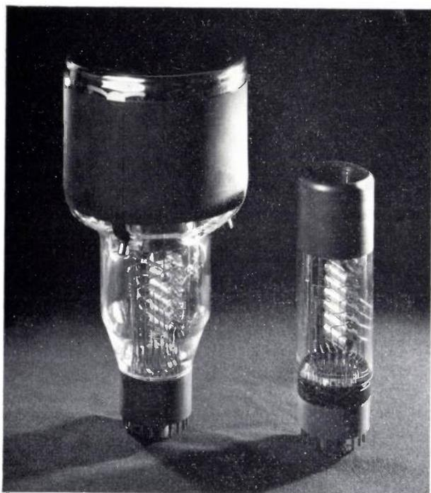
Fig. 19. Fast photomultipliers 56 AVP (on the right) and 58 AVP. Length of tubes 18 and 27 cm, respectively.
