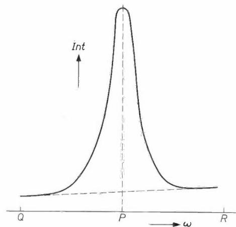
Fig. 13. When the crystal is rotated by a small angle (from *Q* to *R*) about the omega axis, the intensity *Int* of the reflected X-ray beam shows a peak at point *P* which corresponds to the omega position that was determined from the Ewald construction (fig. 6). The integral of the reflection profile, after subtraction of the background radiation, is called the integrated intensity.
