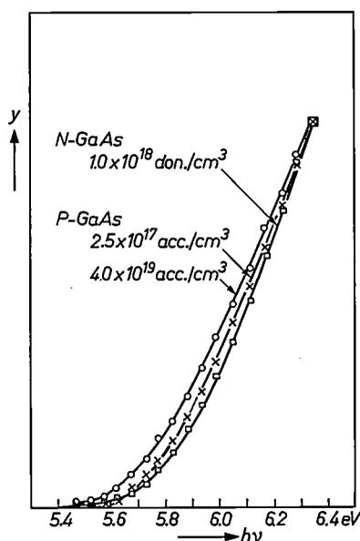
Fig. 10. Influence of volume doping on the photoemission of GaAs. The yield  $y$  is given as a function of photon energy  $h\nu$  for *P*-type material,  $4.0 \times 10^{19}$  acceptors/cm<sup>3</sup> and  $2.5 \times 10^{17}$  acceptors/cm<sup>3</sup> and for *N*-type,  $1.0 \times 10^{18}$  donors/cm<sup>3</sup>. The curves have been reduced to the same  $y$ -value at  $h\nu = 6.35$  eV.
