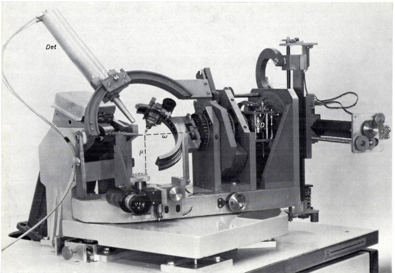
Fig. 12. The diffractometer is shown in the equi-inclination position. The upper base, on which the diffractometer is mounted, has been inclined by an angle  $\mu$  with respect to the stationary lower base. The detector *Det* has been moved along its supporting arc by an angle  $\nu (= \mu)$ . *OD* omega drive.
