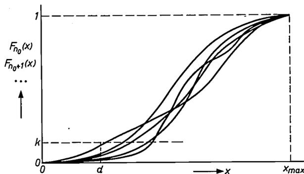
Fig. 11. Possible form of some distribution functions  $F_n(x)$  for  $n \geq n_0$ , and the determination of  $d$  as the highest value of  $x$  where  $F_n(x) \leq k$  for all  $n \geq n_0$ .
