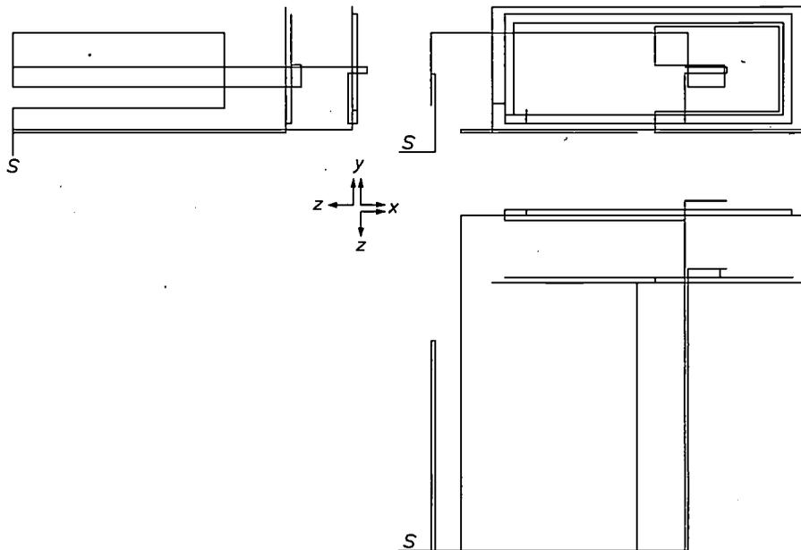
Fig. 2. Check drawing of a workpiece programme for milling a workpiece on a three-axis milling machine, where the displacement of the cutter during the operation always takes place along one axis only. The drawing represents the orthogonal projections on the three co-ordinate planes;  $S$  is the starting point of the cutter path. From drawings of this kind it is very difficult to determine the cutter path. (This workpiece was a frame for an instrument.)
