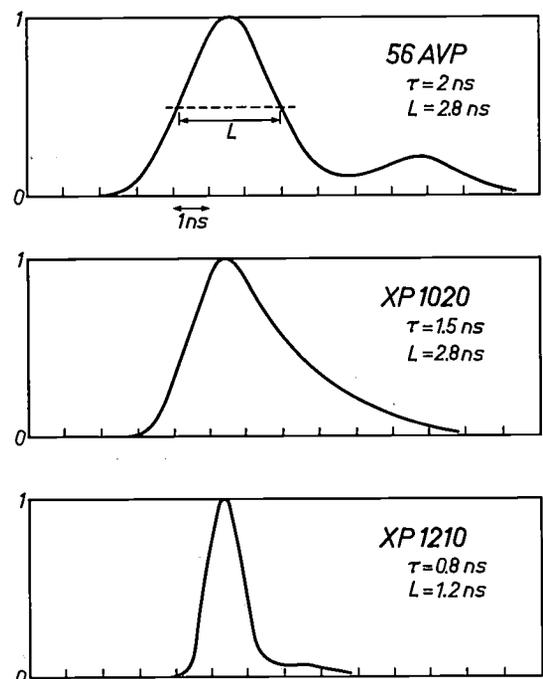
Fig. 16. Pulse response of three fast photomultipliers. In each case the rise time  $\tau$  is indicated and the width  $L$  at half-height of the pulse.
