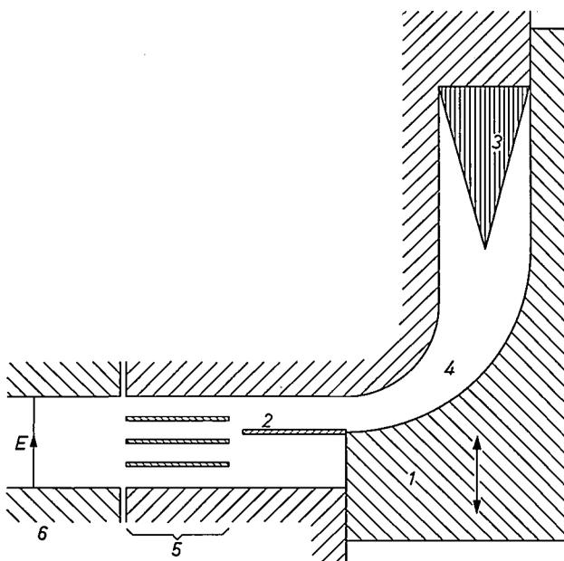
Fig. 21. Termination giving a reflection of variable magnitude and phase. This device, together with the variable phase shifter of fig. 20 (6 in this figure) constitutes a variable impedance. The magnitude of the reflection is varied by vertical displacement of the part 1 together with the resistive sheet 2. 3 is a load, 4 a 90°  $E$ -plane bend, both reflectionless. 5 mode filter. The magnitude of the reflection coefficient is equal to  $y/b$  (cf. fig. 19).
