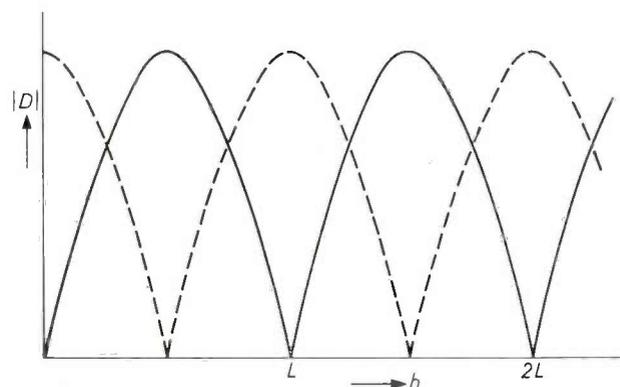
Fig. 4. Amplitude variation  $|D|$  of the reflected beam (solid line) and the transmitted beam (dashed line) as a function of the crystal thickness  $h$ .
