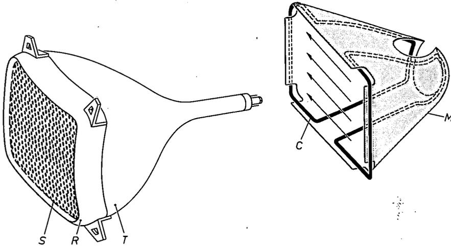
This is done by means of a large field coil, which generates an alternating field near the tube and then after a short time is slowly moved away from the tube. While he is doing this the operator sees the striking display of colour patterns illustrated here, which are produced on the screen by the distorted electron beams. Once the field has been removed and degaussing is complete, the whole of the screen is the same colour all over.
