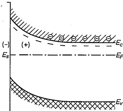
*Fig. 7.* Energy-band scheme of the edge region of an *N*-type semiconductor with a negative charge at the surface. This charge has driven the electrons away from the edge region, giving a positive space charge there, which is carried by ionized donors. In the case illustrated the energy of the surface states  $E_s$  is equal to the Fermi energy  $E_F$ ; half the surface states are then occupied by electrons.
