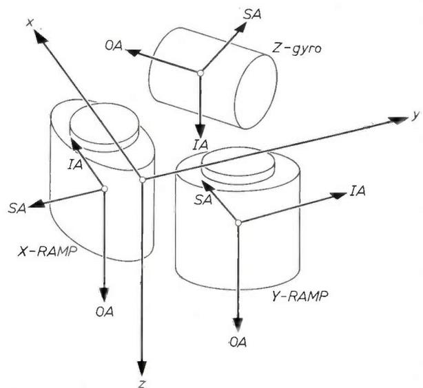
Fig. 14. Arrangement of two RAMP units and a gyro as mounted on the platform in a RAMP navigation system. SA spin axes. IA input axes. OA output axes. The input axes correspond to the co-ordinate system  $x, y, z$  (cf. fig. 26).
