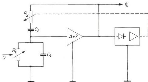
Fig. 2. Wien bridge oscillator for representing a measured quantity  $Q$  by a frequency  $f_0$  (or period  $T_0$ ), with amplitude control via the frequency-determining network.
