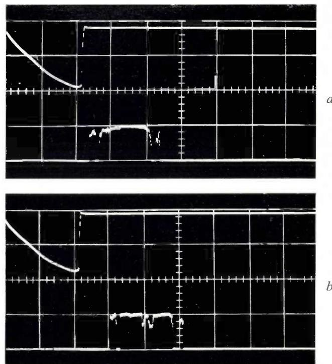
Fig. 9. Checking the time required for the displacement of a needle, using the arrangement of fig. 8 (horizontal scale: one square for 0.5 ms).
