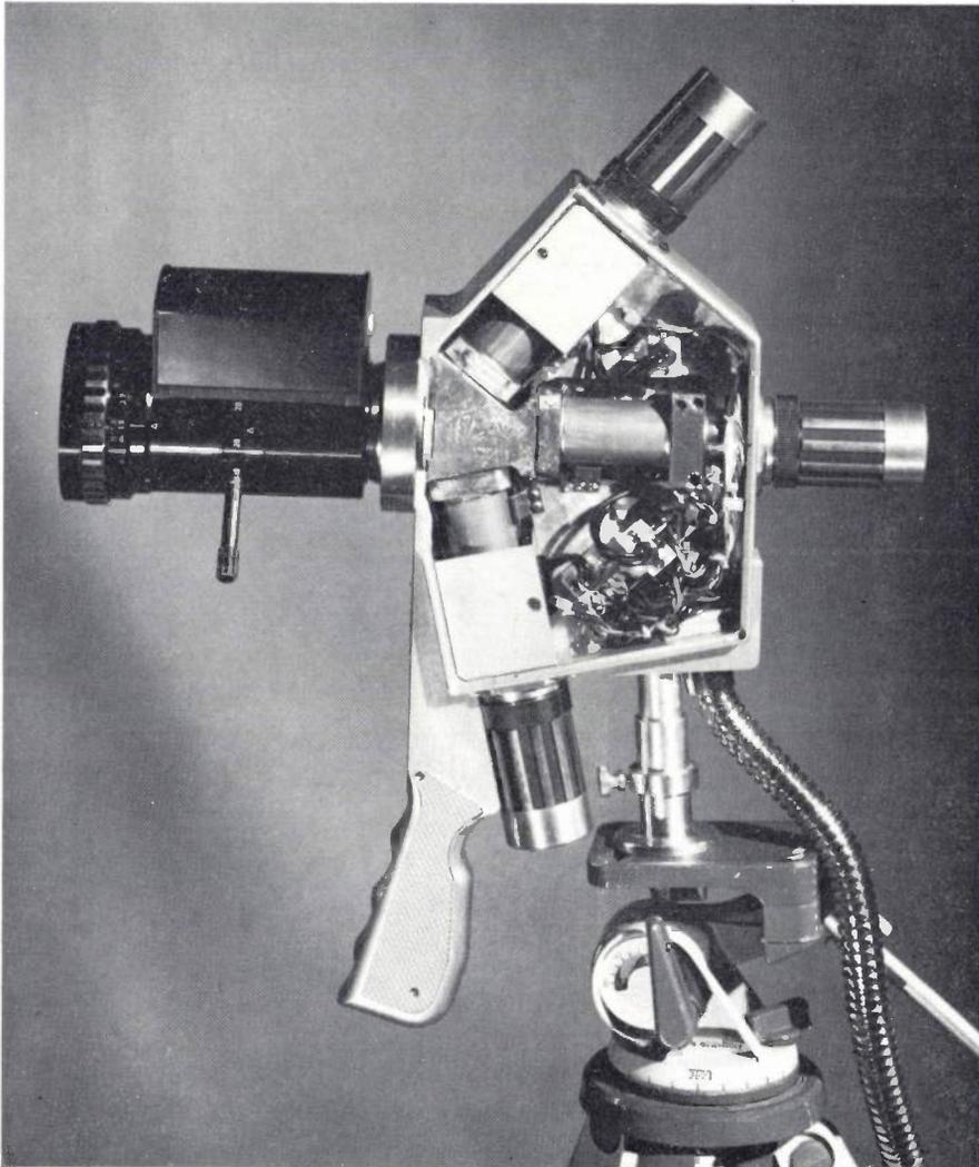
Fig. 12. The camera with a side-plate removed, showing the prismatic colour-separation system and the three "Plumbicon" tubes with their deflection coils. Some of the electronic circuits are on the other side.
