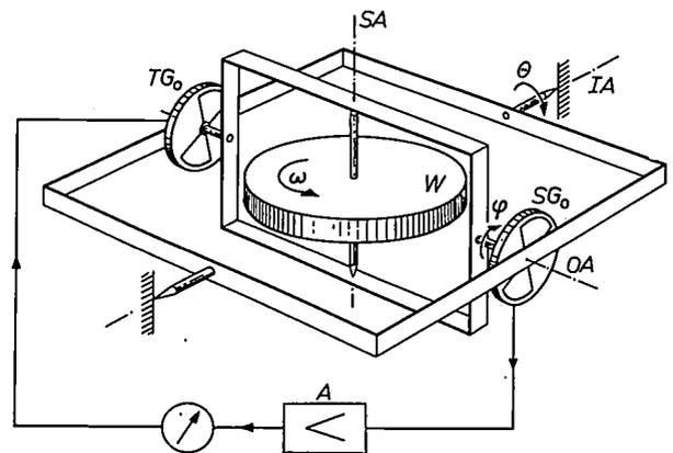
Fig. 7. Schematic diagram of a rate gyro with an electrical feedback system.  $SG_o$  generator, delivering a signal proportional to the rotation angle φ about the output axis OA. A amplifier.  $TG_o$  torque generator. In this case also φ is proportional to the angular velocity  $\dot{\theta}$  about the input axis IA.
