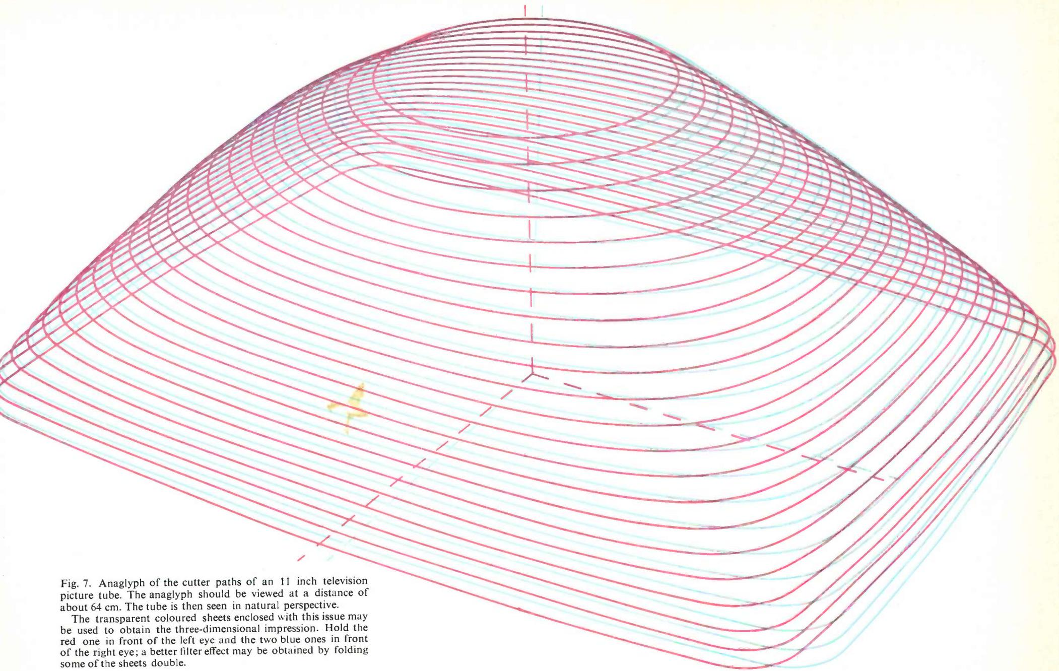
Fig. 7. Anaglyph of the cutter paths of an 11 inch television picture tube. The anaglyph should be viewed at a distance of about 64 cm. The tube is then seen in natural perspective.
