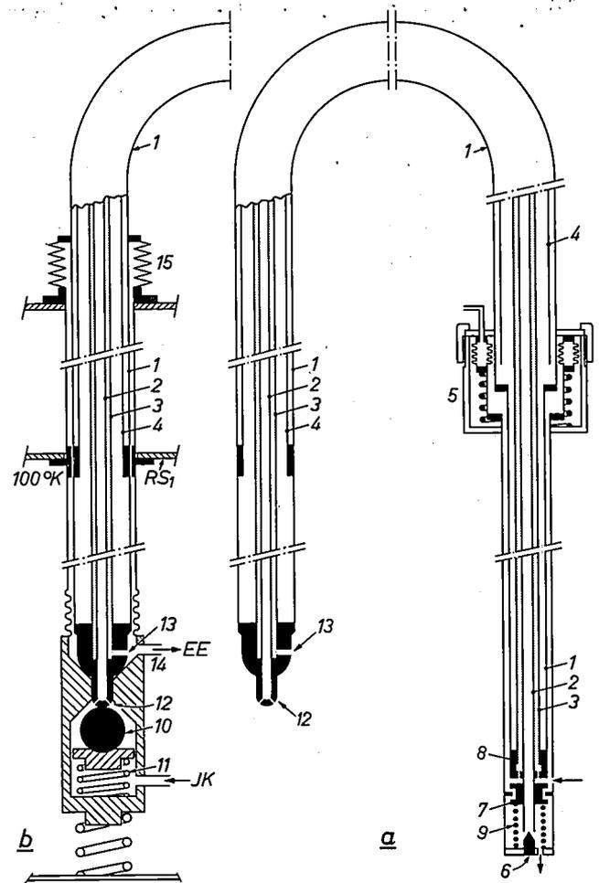
operated by means of the bellows system 5. The other end of the tube reaching into the cryostat can easily be taken out, which automatically closes the line which supplies the liquid and gas to the central tube. A special method of manufacture is used for making the complex assembly of coaxial walls 1, 2, 3 and 4: the structure is fabricated in rectilinear form, all the spaces are filled with water, and it is then cooled in a suitable way to the temperature of liquid nitrogen and bent to shape.
