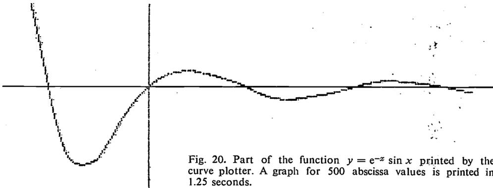
Fig. 20. Part of the function  $y = e^{-x} \sin x$  printed by the curve plotter. A graph for 500 abscissa values is printed in 1.25 seconds.
