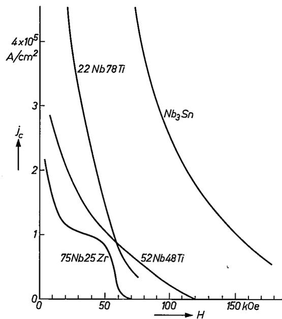
Fig. 5. The critical current density  $j_c$  as a function of  $H$ , the magnitude of a transverse magnetic field at 4.2 °K, measured for short, straight samples of various coil materials. The two curves for Nb-Ti refer to the best materials of this type of alloy at present available.
