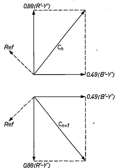
Fig. 1. Vector diagram of the chrominance signals  $C_n$  and  $C_{n+1}$  of two successive lines with the same colour, in a PAL transmission. The phase of the component  $0.88(R' - Y') \cos \omega_s t$  differs in each successive line by  $180^\circ$ . *Ref* indicates the simultaneously transmitted burst, which is used for synchronous detection of the chrominance signals (see [1]).
