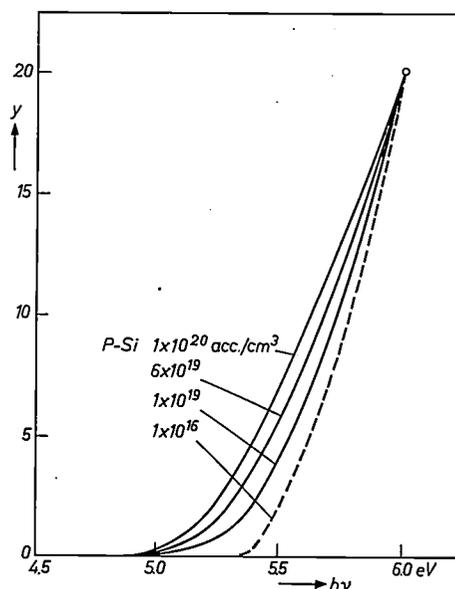
Fig. 6. Influence of doping on the photoemission of silicon. The yield  $y$  is plotted against the photon energy  $h\nu$ , for three volume doping contents:  $1 \times 10^{19}$ ,  $6 \times 10^{19}$ ,  $1 \times 10^{20}$  acceptors/ $\text{cm}^3$ . For comparison the yield for weakly doped material ( $1 \times 10^{16}$  acceptors/ $\text{cm}^3$ ) is also shown (dashed line, taken from fig. 5). The curves are reduced to the same  $y$ -value at  $h\nu = 6.0$  eV.
