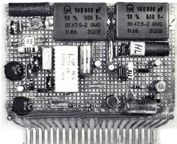
Fig. 3. Experimental version of a resistance-to-period converter based on the circuit shown in Fig. 2. The component HL contains the combination of lamp and photoresistor. The small square component TAA 191 is the control loop amplifier, designed as an integrated circuit. The wiring board is 120 × 100 mm.
