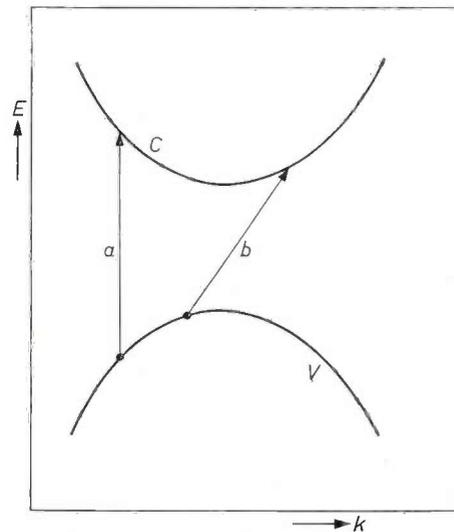
Fig. 15. Energy  $E$  as a function of momentum ( $k$ ) for electrons in a semiconductor.  $C$  is the conduction band,  $V$  the valence band.  $a$  is a direct transition,  $b$  an indirect transition.
