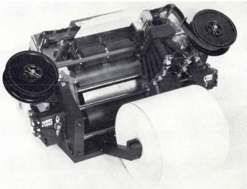
Fig. 12. Experimental model of the serial printer.
