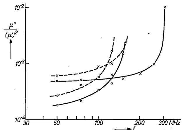
Fig. 8. The figure of merit  $\mu''/(\mu')^2$  as a function of frequency  $f$  for conventionally prepared (dashed curve) and continuously hot-pressed (solid curve) cobalt-containing nickel ferrite and nickel-zinc ferrite [5]. The crosses and circles relate to measurements on  $\text{Ni}_{1.02}\text{Co}_{0.02}\text{Fe}_{2.4+\delta}$  and  $(\text{Ni}_{0.8}\text{Zn}_{0.2})_{1.01}\text{Co}_{0.03}\text{Fe}_{2}\text{O}_{4+\delta}$  respectively (where  $\delta$  is very small).
