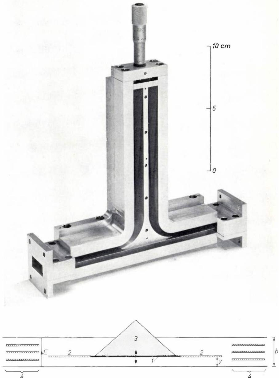
Fig. 19. Variable attenuator derived from the directional coupler of fig. 17. The guide is again divided by a metallic sheet 1 and resistive sheets 2. Power in the upper guide is absorbed in the matched load 3. The attenuation is varied by vertical displacement of the unit consisting of the sheets 1 and 2 and the load 3. Higher-order modes are filtered out, as before, by the mode filters 4.
