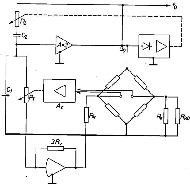
Fig. 7. A small relative change in resistance or bridge detuning  $\Delta R_B/R_B$  is converted into a proportional and larger relative frequency variation  $\Delta f_0/f_0$  by combining the compensating circuit of fig. 6c with the resistance-to-period converter of fig. 2.
