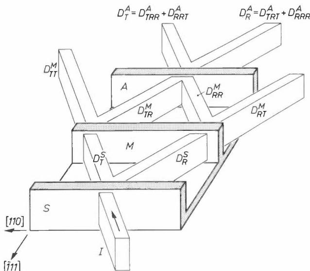
Fig. 17. Illustrating the principle of the X-ray interferometer.
