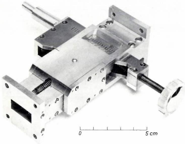
*Fig. 20.* Variable phase shifter (line stretcher). The phase shift between the two ends of a waveguide is varied by varying the length of the line. By turning the knob the part 1 is made to slide in the transverse direction, thereby causing part 2 of the waveguide to slide in the longitudinal direction over the fixed part 3. The top and bottom of the waveguide are partly formed by 1. 4 is a thin metal sheet covering the hole of varying size between 2 and 3.
