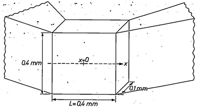
Fig. 2. Thermal process: configuration of conductor (silicon) arranged in the form of a bridge between two current leads. Thermal conductivity  $\gamma = 0.84$  watt/cm s deg; specific heat  $c = 1.76$  joule/cm<sup>3</sup> deg.
