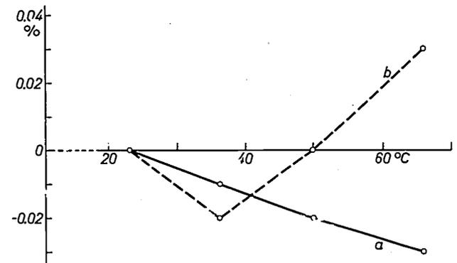
Fig. 10. Temperature drift *a*) of the zero, relative to the maximum load, and *b*) of the sensitivity of the frequency-analogue measuring system.
