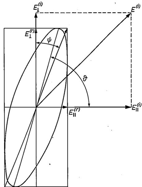
*Fig. 9.* Polarization before and after reflection at an interface with complex reflection coefficient. The light vector  $\mathbf{E}^{(i)}$  of the incident linearly polarized wave is made up from the two components  $E_{\parallel}^{(i)}$  and  $E_{\perp}^{(i)}$ , whose magnitudes change to  $E_{\parallel}^{(r)}$  and  $E_{\perp}^{(r)}$  upon reflection. Since there is a phase shift between the two components on reflection the reflected light will be elliptically polarized.
