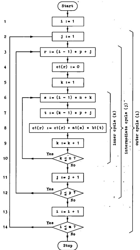
Fig. 9. Flow chart for computing the matrix product in which the variables have at most one index. This is suitable for assembly language coding.
