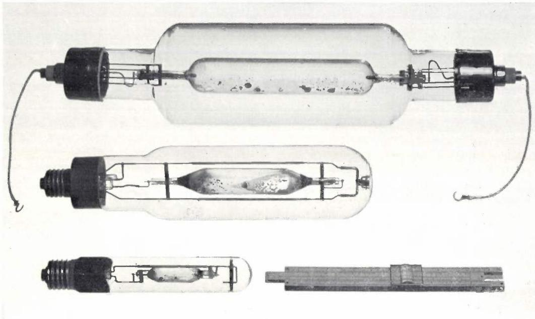
Fig. 1. The 400, 2000 and 5000 W HPI lamps in ascending order. The luminous efficiencies are 80, 95 and 110 lm/W respectively, the operating voltages are 125, 245 and 550 V, and the currents are 3.5, 9 and 10 A. The lamps have a cylindrical outer bulb of hard glass; the inner bulb is of quartz glass. The outer bulb of the 400 W lamp is evacuated and contains a getter; the outer bulb of the 2000 and 5000 W lamps is filled with nitrogen to improve the heat conduction.
