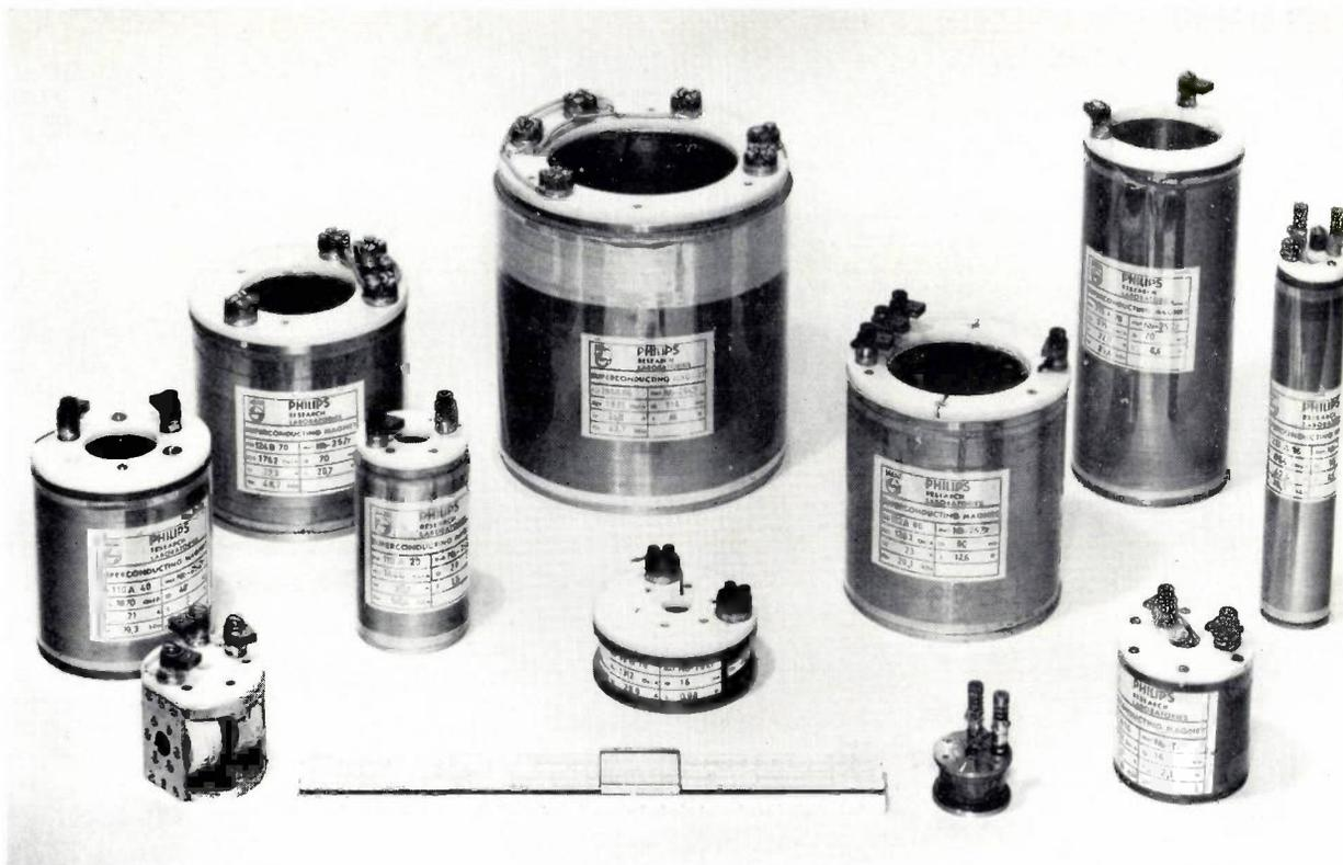
Fig. 2. Some experimental superconducting magnets made at the Philips Research Laboratories in Eindhoven. The small magnet at the front and on the left has an air gap and has been specially made for optical research. The magnet coil at the extreme right gives a highly uniform and readily calculable field, and one of its uses is for calibrating Hall elements for field-strength meters.
