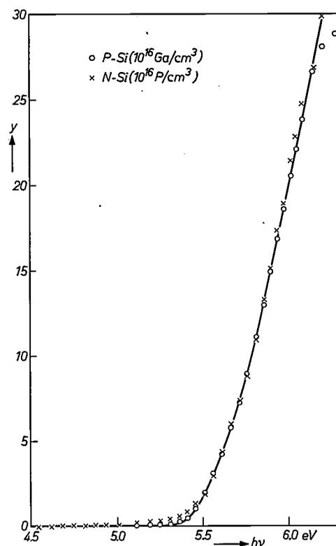
Fig. 5. Yield  $y$  of the photoemission for  $P$ -type and  $N$ -type silicon ( $1 \times 10^{16}$  charge carriers/ $\text{cm}^3$ ) as a function of photon energy  $h\nu$ . The solid curve represents the relation  $y = 42(h\nu - 5.4)^{3/2}$ . The scale for  $y$  is arbitrary.
