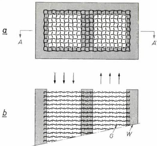
Fig. 2. Principle of the design of a gauze-type heat exchanger. a) Transverse cross-section of the channels. b) Longitudinal cross-section AA' of the channel. G copper gauze. W walls.
