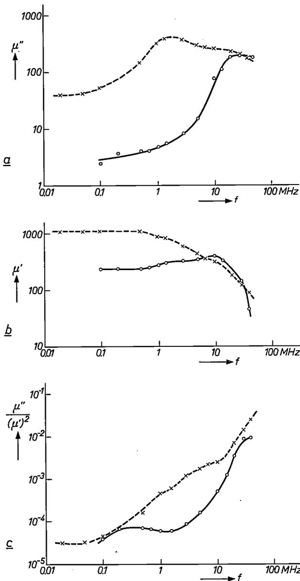
Fig. 7. a) The imaginary part  $\mu''$  of the permeability, which is a measure of the magnetic loss, b) the real part  $\mu'$  of the permeability, and c) the ratio  $\mu''/(\mu')^2$ , which is a figure of merit for the magnetic quality, all plotted as a function of frequency  $f$  for the NiZn ferrite of fig. 6. The dashed curves relate to the conventionally prepared ceramic and the solid curve to the hot-pressed product [5].
