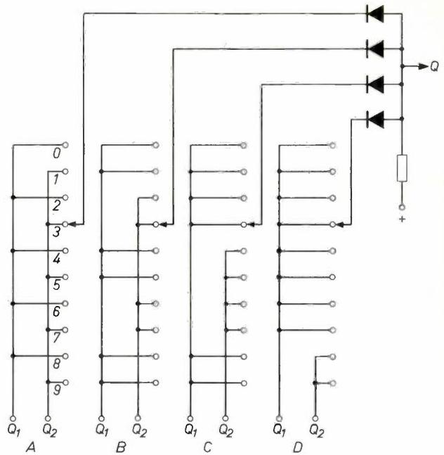
Fig. 11. Basic circuit of a thumbwheel switch. The four inputs of an AND circuit are connected by four contacts to the outputs  $Q_1$  and  $Q_2$  of the bistable circuits *A*, *B*, *C* and *D* of a counter. The output *Q* goes to the "1" level when the counter reaches the preset reading.
