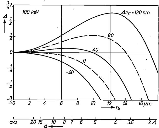
Fig. 6. The wave-front aberration  $\Delta$  in the second focal plane of the objective, caused by spherical aberration and defocusing, as a function of the radius vector  $r_b$ , for an electron beam of 100 keV energy, emitted from the primary focus  $F_1$  or from a point a distance of  $\Delta z_F$  away from it on the optical axis. The scale beneath the figure gives the grating constant  $d$  corresponding to  $r_b$ .
