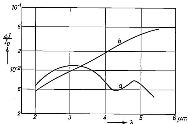
Fig. 14. Spectral dependence of the infra-red absorption of free charge carriers. ( $I_0$  incident intensity,  $\Delta I$  attenuation observed.) Measured by IRS with a modulation of the density of holes (*a*) and electrons (*b*) in the space-charge region of intrinsic germanium in contact with an electrolyte.
