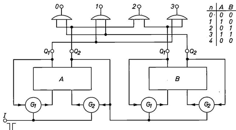
Fig. 19. Two bistable circuits *A* and *B* are connected as a counting circuit with four possible states. The table shows the states of the two bistable circuits after  $n$  input pulses. *I* pulse input.
