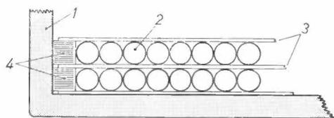
Fig. 11. Method of winding a coil of Nb-Zr wire for an experimental superconducting magnet. 1 coil former. 2 Nb-Zr wire with thin copper coating; outside diameter 0.25 mm. 3 "Mylar" [\*] layer. 4 "Mylar" ribbon, insulating the winding from the coil former.
