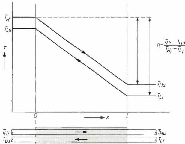
Fig. 5. Variation of temperature  $T$  with distance  $x$  along the channels (length  $l$ ) for a balanced heat exchanger with no insulation losses or longitudinal thermal conduction. The temperatures with a subscript H relate to the "hot" flow which is falling in temperature, and those with the subscript L to the "cold" flow which is rising in temperature. The efficiency  $\eta$  is the ratio of the temperature differences indicated by the two arrows.
