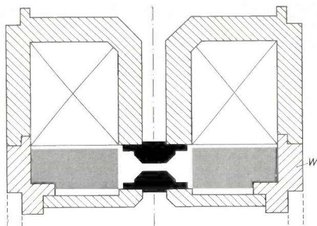
*Fig. 9.* Schematic cross-section of the objective lens and specimen stage (shaded). The pole-pieces are shown black. When the upper part (including the coil) is detached from the ring *W*, the specimen stage can easily be removed. The lower pole-piece can be aligned.
