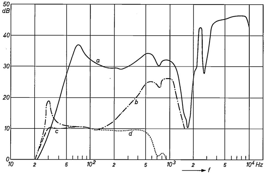
Fig. 12. Amplitude characteristics measured on the system of fig. 10, a) without motional feedback, b) with acceleration feedback, c) with both acceleration and velocity feedback, d) with the addition of a filter for separating high and low frequencies.
