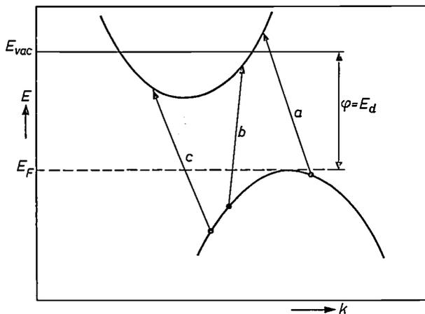
Fig. 16. Indirect transitions in silicon with strong *P*-type doping ( $E_F$  lies at the top of the valence band), coated with Cs ( $\varphi = E_{\text{vac}} - E_F = 1.4 \text{ eV}$ ), *a* is a transition where the electron receives an energy higher than  $E_{\text{vac}}$ ; this electron may be emitted; *b* and *c*, competing transitions where the excited electron cannot be emitted. The energy difference  $h\nu$  for *a*, *b* and *c* is the same, and greater than  $E_d = 1.4 \text{ eV}$ .
