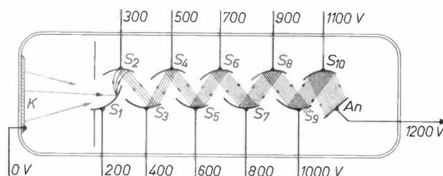
Fig. 1. Principle of a photomultiplier. The photocathode  $K$ , illuminated by the radiation to be detected, emits photoelectrons which are multiplied by secondary emission from electrodes  $S_1$  to  $S_{10}$  as they travel towards the anode  $An$ . The voltages indicated at the electrodes are only intended to give an idea of the kind of magnitudes to be expected.
