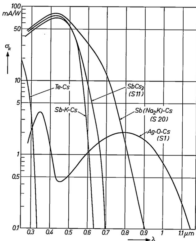
Fig. 5. Spectral sensitivity  $\sigma_k$  of photocathodes in current use.
