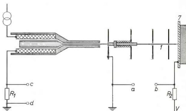
Fig. 8. Diagram of the arrangement used for investigating the movement of the needle in the mechanical printing element. The paper and the inking ribbon are replaced by a metal plate 7. After travelling the required distance, the needle touches the plate, so that the voltage between points *a* and *b* falls to zero. This voltage and the voltage between terminals *c* and *d* of resistance  $R_1$ , which carries the electromagnet current, are applied to a double-beam oscilloscope.
