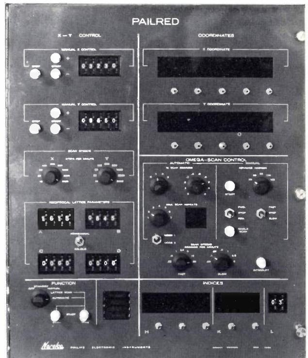
Fig. 25. The experimental parameters of the automatic data-collection process are selected by means of switches located on the control panel. Manual operation of the three motor drives on the diffractometer is also done by means of switches.
