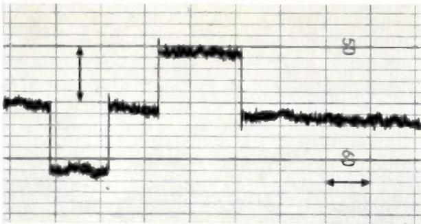
Fig. 18. Recording of lens current. The length of the horizontal double arrow corresponds to a time interval of two minutes, the length of the vertical one to a relative current variation of  $5 \times 10^{-6}$ . The fast current fluctuations and also the drift during one minute are no greater than about 1 in  $10^6$ . During the recording the current was varied twice in steps of  $5 \times 10^{-6}$  (corresponding defocusing 12.5 nm).
