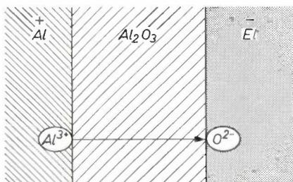
Fig. 3. Illustrating the anodic oxidation of aluminium.
