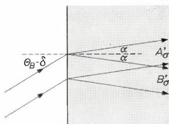
Fig. 7. As the angle of incidence deviates from the Bragg angle  $\theta_B$  (deviation angle  $\delta$ ) two modes are still excited in the crystal but the power flow in each makes an angle  $\alpha$  ( $\leq \theta_B$ ) with the diffracting planes.
