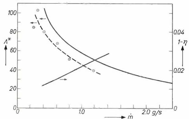
Fig. 7. Variation of the dimensionless quantity  $\Lambda^*$ , which determines the efficiency  $\eta$ , as a function of the mass flow  $\dot{m}$  for a heat exchanger like that of fig. 4. The solid line relates to the calculated values; the values derived from measurements differ only very slightly from them (dashed line). The corresponding curve of  $1 - \eta$  is also shown. The true values of  $1 - \eta$  are about 10% higher because of the cold loss due to longitudinal conduction of heat.
