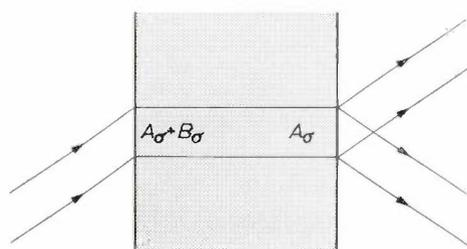
Fig. 6. Diagram showing how in a thick crystal, for the exact Bragg condition, the mode  $A_\sigma$  remains and splits into two waves of equal intensity on reaching the back surface.
