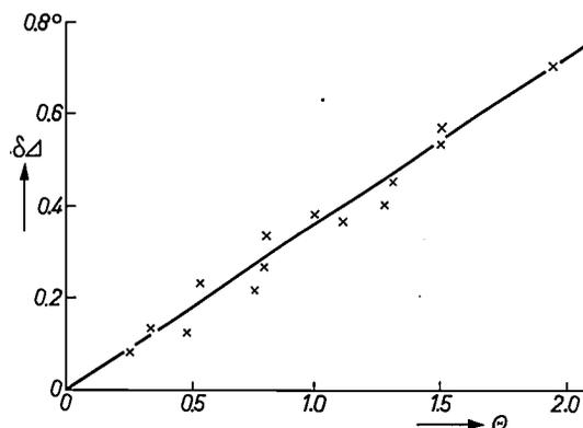
Fig. 15. Change  $\delta\Delta$  of the phase shift plotted against the degree of coverage  $\Theta$  (in monolayers) during the adsorption of krypton on germanium at the temperature of liquid nitrogen, as investigated at Philips Research Laboratories in Eindhoven [20]. All data were taken under equilibrium conditions by varying the gas pressure in the cell containing the germanium specimen.
