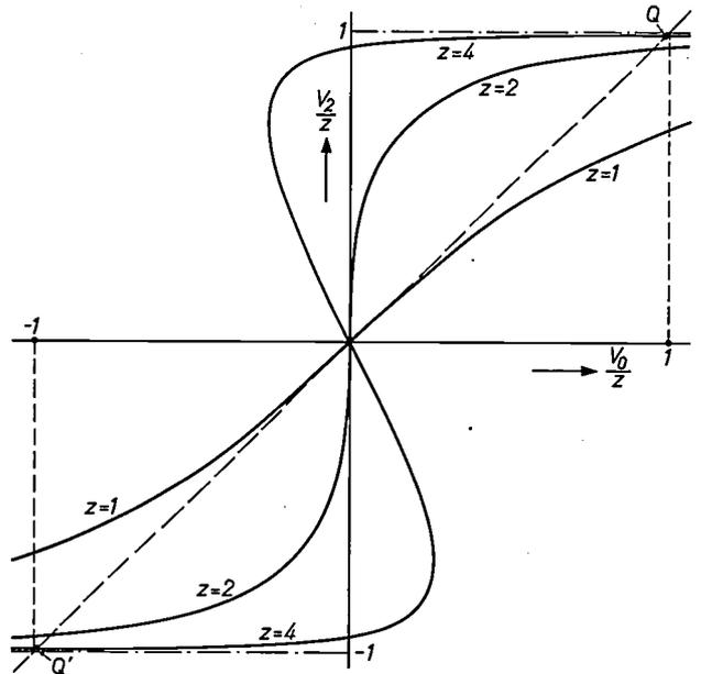
Fig. 2. Idealized characteristics of the basic circuit of fig. 1. Depending on the choice of the parameter  $z$  (half of the "theoretical swing") different types of curve are obtained.
