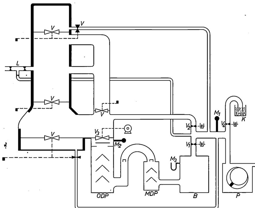
Fig. 12. The vacuum system. The microscope tube, shown on the left, is connected by three broad tubes with the oil diffusion pump ODP, MDP mercury ejector pump, B fore-vacuum vessel, P roughing pump.  $M_1$  Pirani gauge.  $M_2$  Penning gauge.  $M_3$  mercury pressure gauge.  $V$  vacuum valves.  $L$  vacuum lock, which can be separately evacuated.  $K$  vessel with drying agent. Valves  $V_1$ ,  $V_2$  and  $V_4$  are electromagnetic,  $V_3$  is motor-driven.
