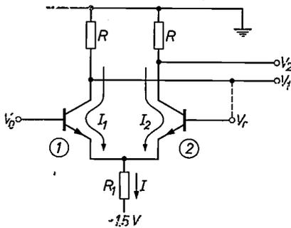
Fig. 1. Circuit of two transistors (difference amplifier, known as a "long-tailed pair") used as the basic circuit for the applications discussed here. The vital feature is the use of positive feedback, achieved by making  $V_T$  equal to  $V_1$ .
