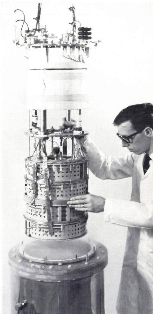
Fig. 14. The coil of the largest superconducting magnet made at Philips Research Laboratories. The inside diameter of the bore is 186 mm. The coil is wound in eight sections arranged in pairs on four coil formers. The maximum current is about 180 A, and the maximum field strength about 40 kOe.
