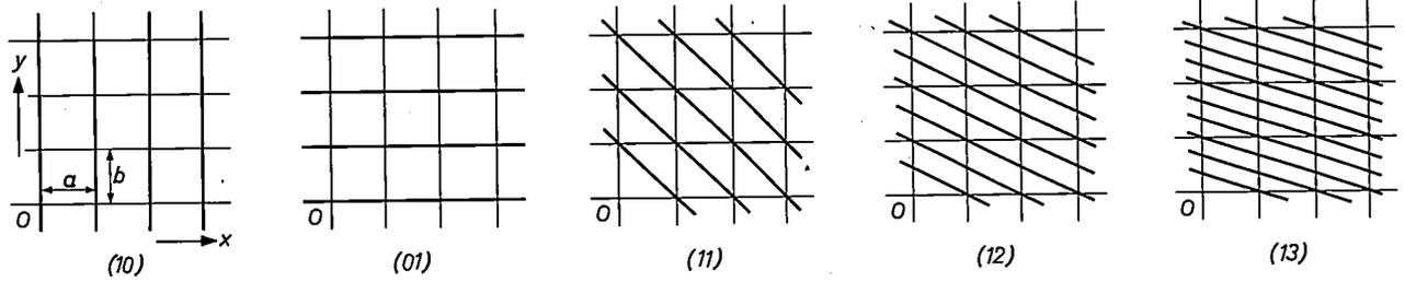
Fig. 3. A two-dimensional crystal is represented as a combination of unit cells (sides  $a$  and  $b$ ) of which only nine are shown. Each set of crystal planes in this repetitive array can be identified by a set of integers  $h$  and  $k$ , the Miller indices. The five figures show five different sets of planes.
