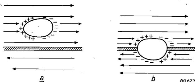
Fig. 8. Effect of inclusions or pores on the energy in a Bloch wall (Néel<sup>13</sup>)
