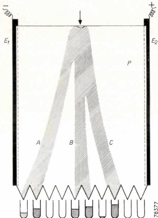
Fig. 5. Paper-electrophoresis arranged as a continuous process. Filter paper  $P$  is held vertically between two electrodes  $E_1$  and  $E_2$ . The solution containing the various ions ( $A$ ,  $B$ ,  $C$ ) is fed in at the top and the ions (still in solution) are collected separately at the bottom end.
