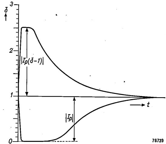
Fig. 12. Method of reading  $\delta$  direct from the oscillogram.
