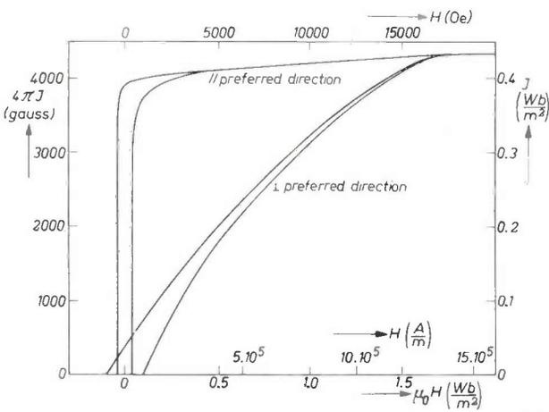
**Fig. 4.** Hysteresis loops (upper half only) of an isotropic Ferroxdure sample sintered at a high temperature, as measured // and  $\perp$  to the preferred direction. The magnetic texture closely resembles that of a single crystal.
