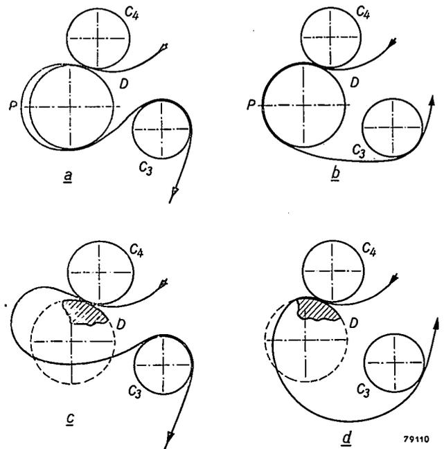
Fig. 13. The film lacing path in the sound-head. *D* is the sound drum, *C*<sub>4</sub> the pressure roller, *C*<sub>3</sub> the guide roller and *P* the sound scanning point.
