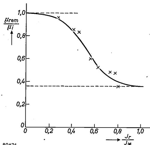
Fig. 9. Relationship between the quantities  $\mu_{rem}/\mu_i$  and  $J_r/J_*$ .
