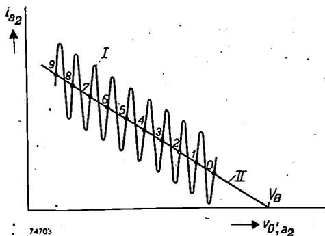
Fig. 3. Undulating line *I*: characteristic of the decade counter tube (anode current  $I_{a_2}$  versus potential  $V_{D, a_2}$  of the right-hand deflector plate and the anode). Line *II* is the diagrammatical equivalent of equation (1). Only those points of intersection of *I* and *II* that are numbered from 0 to 9 represent stable beam positions; all others corresponding to unstable positions.
