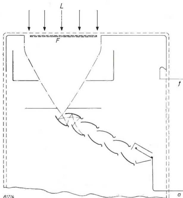
Fig. 4. Diagram showing the construction of the photo-multiplier tube described in this article. The incident light  $L$  falls on the photo-cathode  $F$ . The letters  $f$  and  $a$  indicate the lead-in wires of the photo-cathode and the anode respectively.
