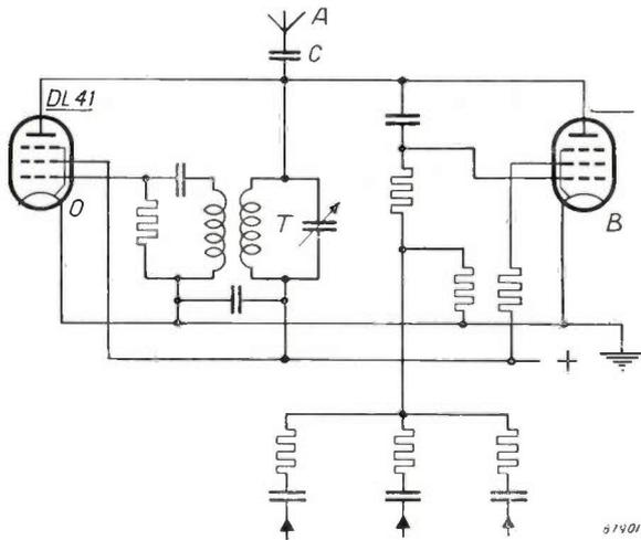
Fig. 8. Circuit diagram of the high-frequency oscillator containing the reactance valve. The three audio-frequency signals are mixed in a potentiometer and applied to the grid of the reactance valve B. The frequency of the H.F. oscillator O is governed by the voltage on this grid. The oscillator is connected across a capacitance C to the  $\lambda/2$  aerial A. The frequency of the oscillator can be adjusted by means of trimmer T just before the ascent of the sonde.
