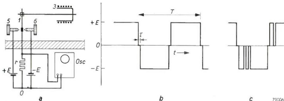
Fig. 5. a) Circuit for testing the vibrator; voltages +E and -E occur alternately across the resistor r. The oscilloscope Osc should show the image given in (b), without interfering pulses as in (c) and with a change-over time τ equal to roughly 2% of the period T. Other references as in fig. 4.
