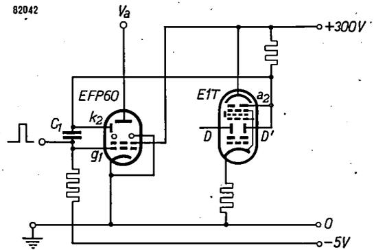
Fig. 10. Diagram showing scaler tube E1T with secondary emission tube EFP 60 to shorten the reset time. Tube EFP 60 is triggered by a positive pulse on  $g_1$  and maintained conductive for the required period by coupling capacitor  $C_1$  between  $k_2$  and  $g_1$ .
