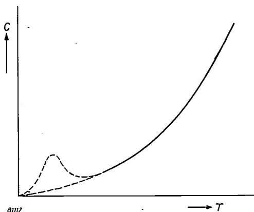
Fig. 4. The calorimetric entropy can be calculated if the specific heat  $c$  is known as a function of the temperature  $T$ . Extrapolation from the lowest attainable temperatures to absolute zero is of course necessary, but it must be noted that this involves the risk of overlooking a peak in the specific heat curve situated below the temperature range in which measurements can be made.
