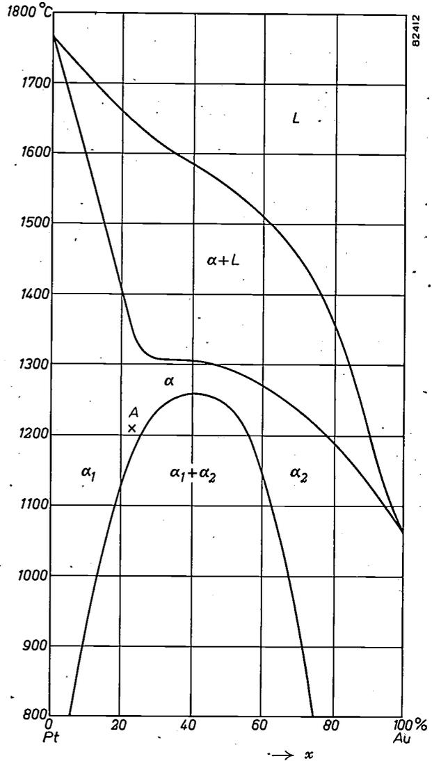
Fig. 6. Phase diagram of the system platinum-gold, which, even in the solid state, shows a complete curve of the type of fig. 5.  $\alpha, \alpha_1$  and  $\alpha_2$  indicate solid phases; the liquid phase is denoted by  $L$ .
