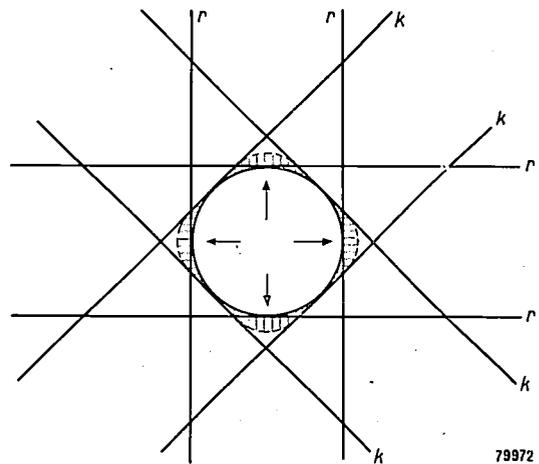
Fig. 4. A hole drilled perpendicular to a cube face is bounded by cube planes *k* and rhombic-dodecahedral faces *r*, as indicated schematically. Wear will occur mainly in the *r*-planes, so that the aperture will eventually assume a square shape.
