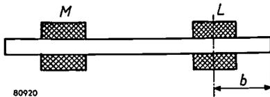
Fig. 23. Medium wave coil  $M$  and long wave coil  $L$  wound on a single rod of Ferroxcube. When, for medium wave reception, the long wave coil is short-circuited, part  $b$  of the rod becomes ineffective.
