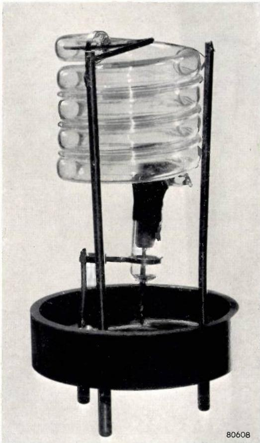
Fig. 11. The LSD. 5 tube, of 1000 joules dissipation. The subsidiary glass helix containing the trigger wire can be seen lying between the turns of the main helix.
