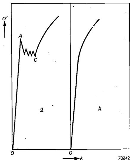
Fig. 5. Stress-strain curve for mild steel. The tensile stress  $\sigma$  is plotted as a function of the elongation  $\epsilon$ . The steel shows a sharp upper yield point at A (fig. 5a). If it is plastically stretched to C and the stress removed, then on renewed loading the material shows a stress-strain curve (b) without a yield point.
