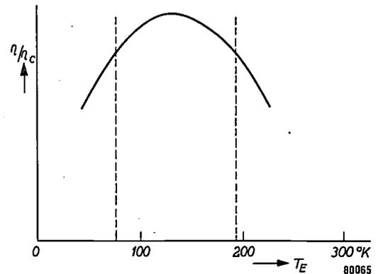
Fig. 2. The "figure of merit"  $\eta/\eta_c$  of the gas refrigerating machine as a function of the temperature ( $\eta =$  efficiency of the actual machine,  $\eta_c =$  Carnot-efficiency, cf. I). The diagram shows how the influence of the losses limits the useful temperature range of the machine.
