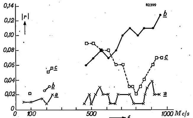
Fig. 18. Measured values of the modulus  $|r|$  of the reflection coefficient in a unshielded polythere twin lead with  $\zeta = 300$  ohms, plotted against the frequency  $f$ . The cable is matched fairly well by a resistance. a) Without deliberately introduced irregularities, b) with one insulator close to the terminating resistor, c) with another insulator about 7.5 cm from the first.
