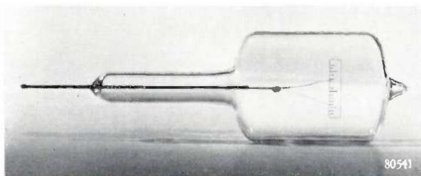
Fig. 5. Electrostatic electrometer for experimental and educational purposes.
