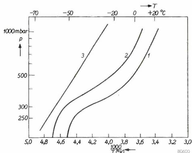
Fig. 2. Variation of temperature with pressure in the "average" atmosphere during summer (curve 1) and winter (curve 2) Line 3 represents the vapour-pressure curve of freon. The pressure of the atmosphere  $p$  is plotted on a logarithmic scale against the reciprocal of the absolute temperature  $T$ , so that curve 3 is then nearly a straight line.
