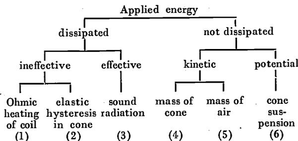
In order to assess the quality of different loudspeakers we examine the frequency response curve to determine the efficiency  $\eta$  (radiated power divided by input power) as a function of the frequency  $f$ .  $\eta$  is usually only a few per cent<sup>4)</sup>.
