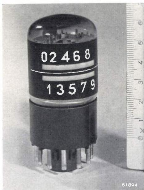
Fig. 1. The EIT decade counter tube. A blue-green fluorescent spot indicates the digit corresponding to the position of the beam in the scaler tube, that is, to the number of pulses counted.
