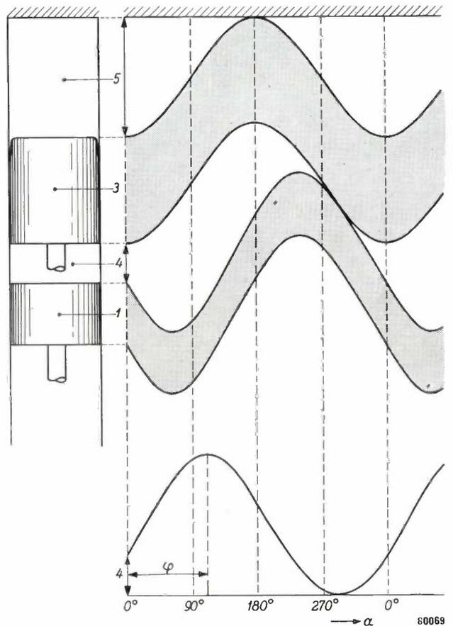
*Fig. 6.* Variations of the volumes of spaces *4* and *5* of *fig. 5* as functions of the shaft angle  $\alpha$ . The constant volumes taken up by the displacer body (*3*) and by the body of the main piston (*1*) are shown in grey. The fixed head of the cylinder is shown shaded. In the lower part of the diagram the volume of space between displacer and master piston has been plotted separately, in order to demonstrate its sinusoidal variation and the phase shift with respect to space *5*.
