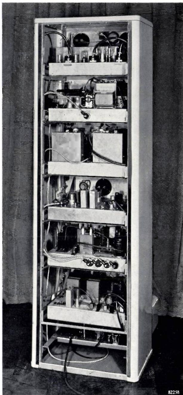
Fig. 11. Rear view of complete instrument. From top to bottom: counting and timing unit,  $\beta$ - $\gamma$  hands unit,  $\alpha$  hands unit, probe unit, E.H.T. power pack for counters (2500 V and 1200 V), power pack for valves (300 V), power pack for relays (50 V). The platform in front of the instrument contains the Geiger Müller counters for measuring  $\gamma$ -activity on the feet.
