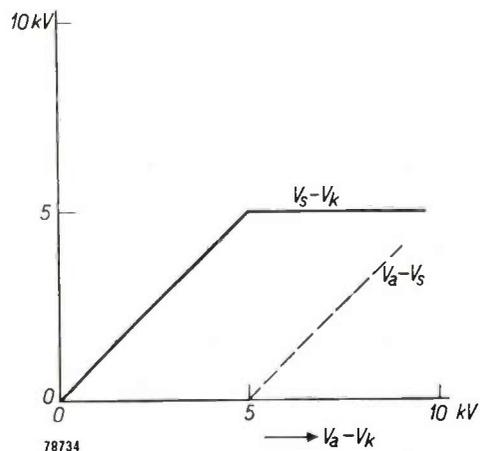
Fig. 6. Potential difference  $V_s - V_k$  plotted as a function of the accelerating potential  $V_a - V_k$  on a tube with plain glass envelope (no screen). The threshold potential (5 kV) is clearly defined. Dotted line:  $V_a - V_s$ .
