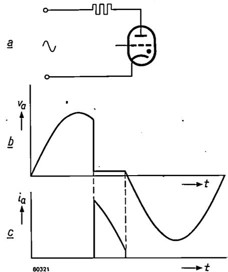
Fig. 4. a) Thyratron with purely resistive load. b) Anode voltage  $V_a$ . c) Anode current  $i_a$ . At current extinction both current decay and inverse voltage build-up are slow, so no high commutation factors can be obtained.
