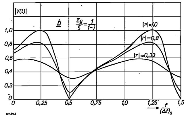
Fig. 12.  $|V(l)|$  plotted against  $f$  when  $Z_g$  does not equal  $\zeta$ . Curves (a) refer to  $Z_g = 2\zeta$  (real), and curves (b) to  $Z_g = \zeta/(1-j)$ ; in both cases  $|r|$  has the values 0.33, 0.80 and 1.0. In (a) the position of the maxima and minima is virtually independent of  $|r|$ . In (b), the position of the maxima is largely determined by  $|r|$ ; for the minima this is not so. It is assumed that  $E$  is unity.
