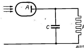
Fig. 3. Anode-circuit of a photo-multiplier tube (with anode  $A$ ), comprising a load-resistor  $R$  and the stray capacitance  $C$ .
