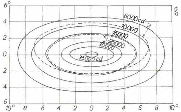
Fig. 16. Isocandela diagram of the 100 W lamp shown in fig. 15, including two curves (dotted lines) from fig. 11c.
