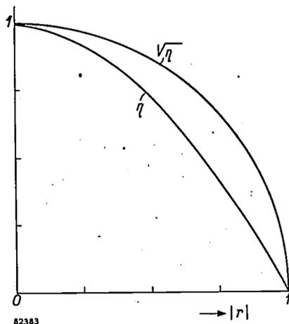
Fig. 2. Efficiency  $\eta$  of the energy transfer, and "voltage efficiency"  $\sqrt{\eta}$ , of a transmission line, plotted against the modulus  $|r|$  of the reflection coefficient. High values of  $\eta$  and  $\sqrt{\eta}$  are possible only when  $|r|$  is small.
