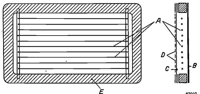
Fig. 2. Proportional counter of flat construction used for the counting of  $\alpha$  activity on the hands.  $A$  tungsten anode wires 0.001" (25  $\mu$ ) diameter,  $B$  metal backing plate,  $C$  aluminized paper window 8  $\mu$  thick,  $D$  protective metal grid. The polystyrene frame  $E$  is about 5"  $\times$  8" (125  $\times$  200 mm).
