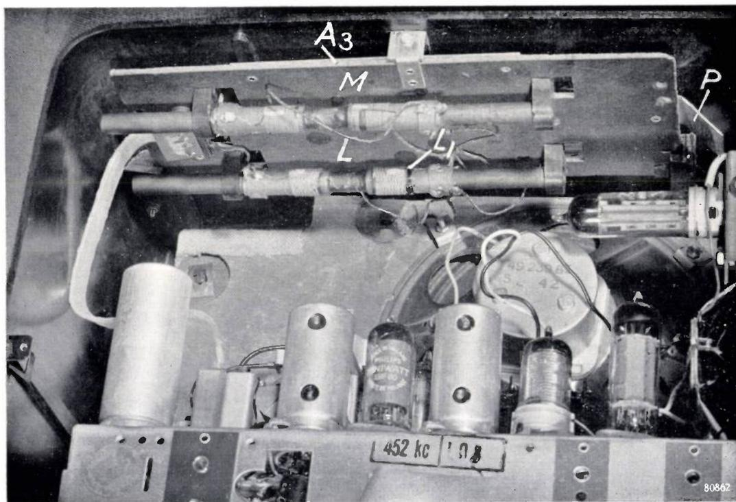
Fig. 11. The receiver BX 321 A-10 has separate Ferroxcube rods for receiving long waves ( $L$ ) and medium waves ( $M$ ). For long wave reception the aerial effect is compensated by means of a compensating coil  $L_1$  and the adjustable plate  $P$  (cf. fig. 13).
