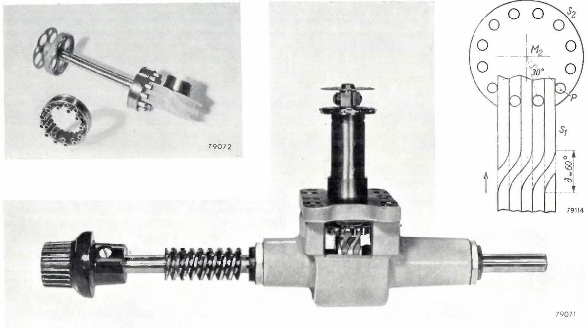
Fig. 8. The intermittent mechanism of the EL 5000. Top left: The most essential parts, viz. a spindle, with at one end the intermittent sprocket, and at the other a disc with projecting pins on its periphery. Meshing with these pins is the grooved actuating cam. The periphery of the disc with the pins positioned around it is included in the photograph to show how correct spacing of the projecting pins is achieved with the aid of shorter pins which do not project beyond the edge of the ring.
