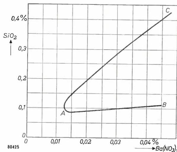
Fig. 2. Curve defining the conditions for adhesion of the fluorescent screen of a cathode ray tube. Vertical axis: concentration (% by wt) of waterglass, i.e.  $\text{SiO}_2$ , in the sedimentation liquid; horizontal axis: concentration of gelatinising medium (barium nitrate). In the area enclosed within the curve *BAC* effective adhesion of the screen is obtained.
