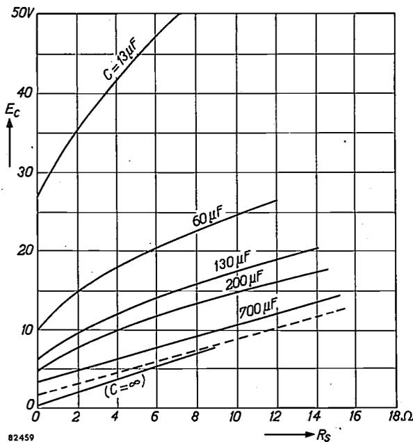
Fig. 6. Maximum permissible series resistance  $R_s$  plotted against battery voltage  $E_c$  for various capacitances  $C$ , as obtained experimentally for capacitor ignition. The line denoted by  $C = \infty$  refers to direct battery ignition with  $R_i = 0$ . The broken line is the calculated curve for the latter case.
