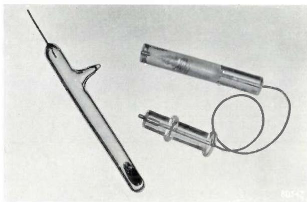
Fig. 6. Two types of mercury friction chargers. The maximum voltage obtainable in the absence of any current leak is about 3 kV.
