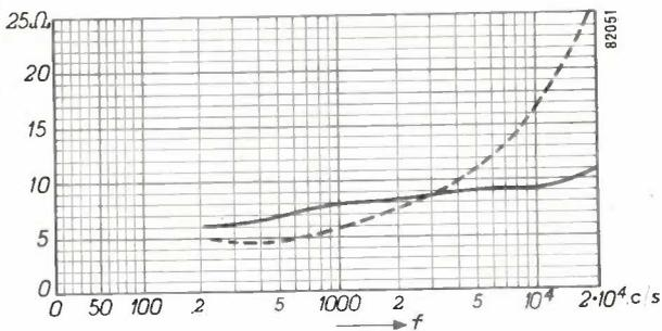
Fig. 5. Speech coil impedance as a function of  $f$  in a loudspeaker with "constant" impedance (continuous line) and, for comparison, the curve for a conventional loudspeaker with rising impedance (broken line).
