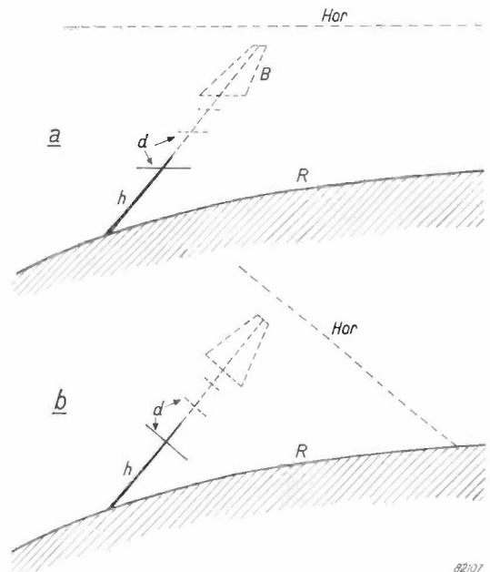
*Fig. 5.* Diagram to illustrate two different situations in which the pilot of an approaching aircraft will see the centre-line (*h*) of a runway (*B*) in exactly the same position relative to his cockpit cut-off. The horizon (*Hor*) is assumed to be completely obscured by fog in both cases. It is only by observing the attitude of the cross-bars (*d*) that the pilot is able to judge his position and direction of movement correctly.
