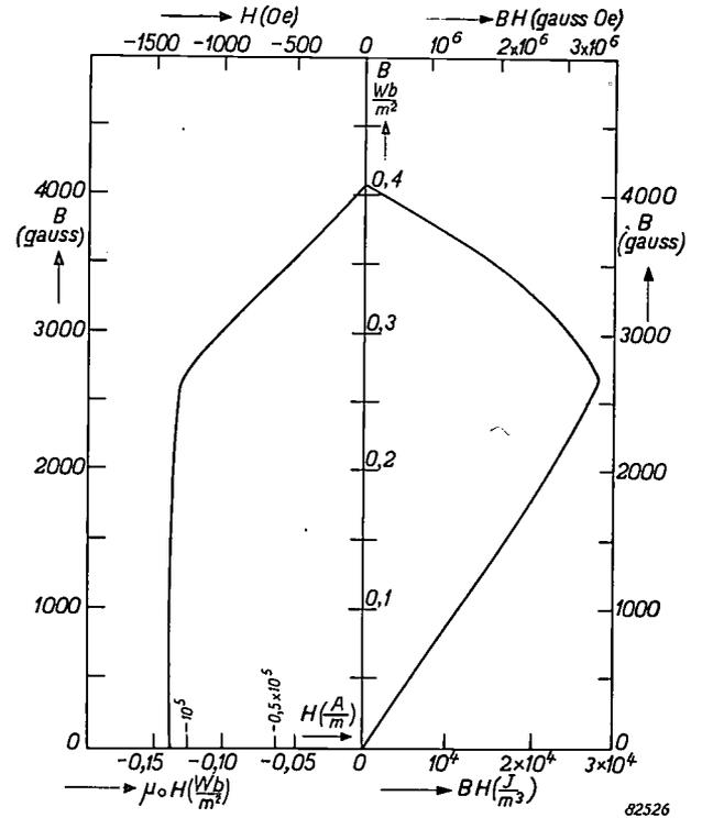
Fig. 8. Demagnetization curve of a particular sample of Ferroxdure II the  $(BH)_{max}$  value of which is 28 000 J/m<sup>3</sup> [ $3.5 \times 10^6$  gauss oersted].
