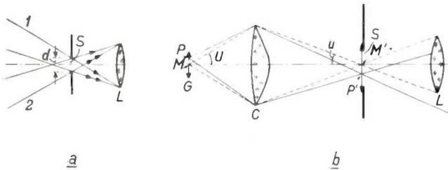
Fig. 3. *a*) To make full use of the objective it would be necessary to illuminate the film gate in such a way that even the light rays proceeding from the corners of this gate completely fill the objective. If *d* be the diagonal of the film gate, light rays 1 and 2 must still be present.
