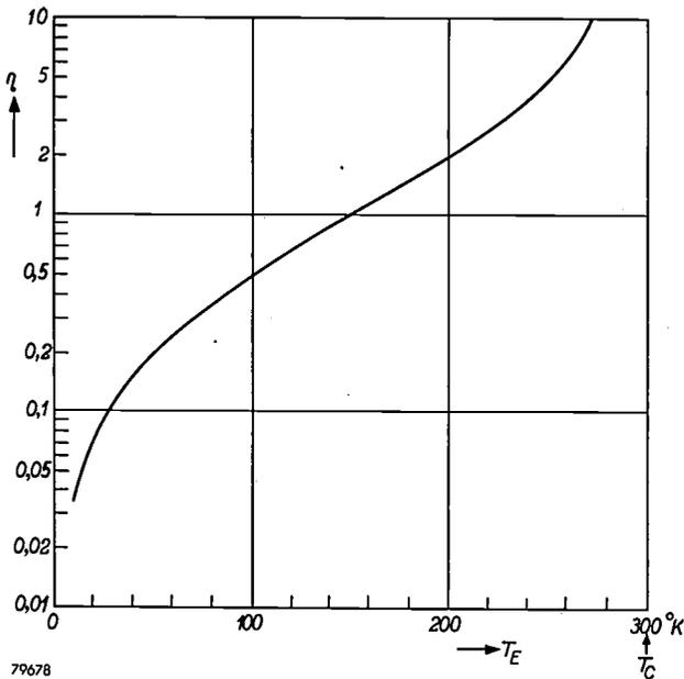
Fig. 4. Theoretical coefficient of performance  $\eta$  of the gas refrigeration cycle (i.e. thermal efficiency of Carnot cycle,  $\eta = \frac{T_E}{T_C - T_E}$ ) plotted against the freezing-temperature  $T_E$ , for an ambient temperature  $T_C = 300^\circ\text{K}$ .
