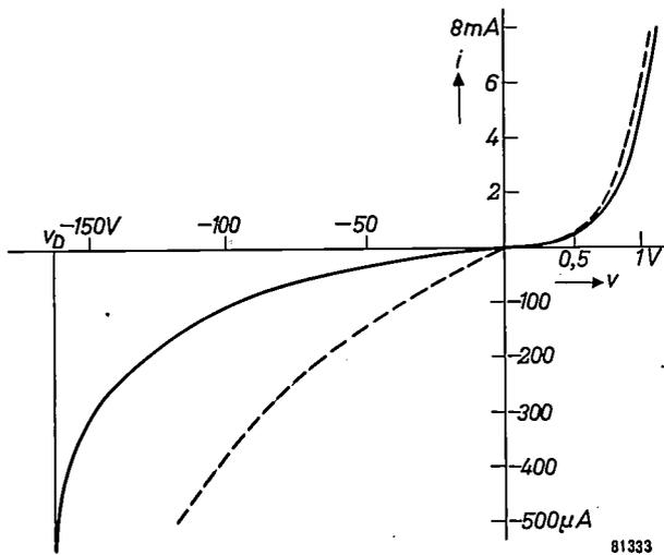
Fig. 9. The rectification characteristic (current  $i$  as a function of the applied voltage  $v$ ) of a point-contact germanium diode (type OA 71).  $v_D$  is the breakdown voltage, at which  $dv/di = 0$ . The dotted curve is the characteristic of the same diode before the forming process. Note the difference in the scales used for the voltage in the forward and reverse directions and also for the forward and leakage currents.
