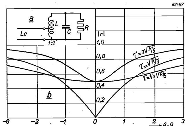
Fig. 15. a) The impedance of a resonant circuit ( $L$ ,  $C$ ,  $R$ ) can be matched to that of the transmission line ( $Le$ ) by employing a suitable transformation ratio ( $\tau$ ). b) Relationship between  $|r|$  and the detuning  $\beta_0$  (the quantity actually plotted is  $\beta_0 Q$ ), for various values of the transformation ratio ( $\tau$ ). The optimum ratio ( $\tau_{opt}$ ) is  $\sqrt{R/\zeta}$ .
