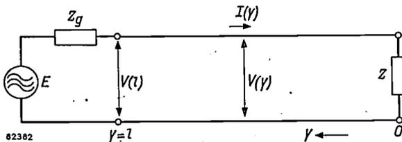
Fig. 1. Transmission line fed by a generator of e.m.f.  $E$  and internal impedance  $Z_g$ , and terminated in an impedance  $Z$ .
