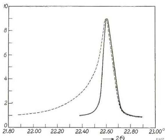
Fig. 10. Profile of a diffraction line with the Geiger counter diffractometer, without the parallel slit systems (broken line) and with the parallel slit systems (full line).
