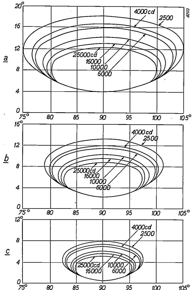
*Fig. 11.* Diagrams showing the required light-distribution (isocandela diagrams) of *a*) initial approach light, *b*) a threshold light, and *c*) a runway light 450 metres (1500 ft) beyond the threshold.
