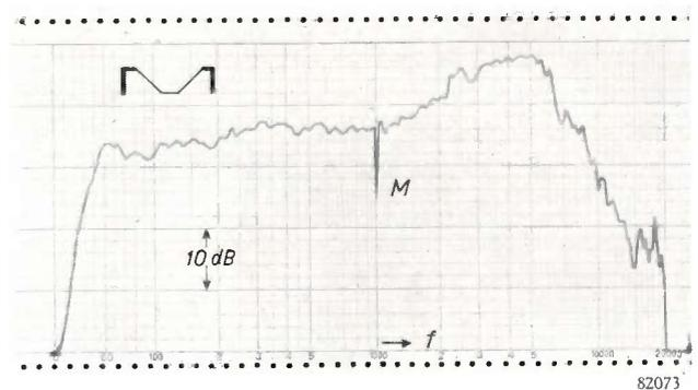
Fig. 3. Response curve of a conventional 8" loudspeaker, showing on a logarithmic scale the sound pressure  $p$  on the axis, for a constant current in the speech coil. The frequency  $f$  plotted horizontally also has a logarithmic scale. The marker  $M$ , obtained by interrupting the speech current (at 1000 c/s) serves to register the curve correctly with respect to the frequency scale.
