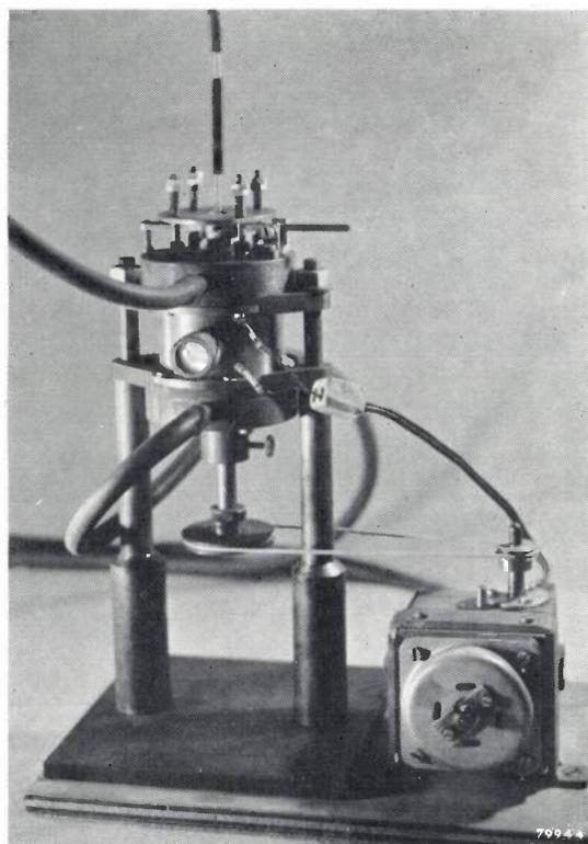
Fig. 7. a) Apparatus for the etching of a diamond by burning with oxygen. The diamond *d* is fitted on a rotatable table *t*. A movable silica nozzle faces the upper surface of the diamond. The whole assembly is placed inside a furnace supplied with a hydrogen atmosphere; the temperature inside the oven is approximately 850 °C. A jet of oxygen is blown onto the diamond through the silica tube.
