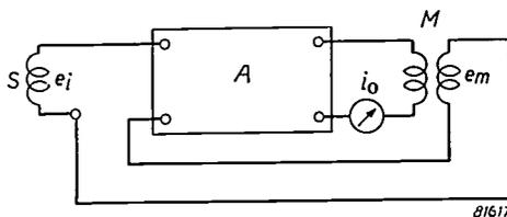
Fig. 7. Basic circuit of the mutual inductance type integrator described by Edgar <sup>2)</sup>.
