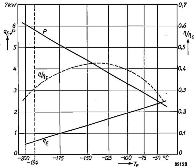
Fig. 10. Measured shaft power  $P$  and refrigerating capacity  $q_E$  of the gas refrigerating machine plotted as functions of the freezing temperature  $T_E$ . The figure of merit  $\eta/\eta_c$  (cf. fig. 2) derived from this, has also been plotted.
