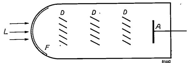
Fig. 1. Diagram showing the basic construction of a photo-multiplier tube in which the dynodes *D* are arranged in the form of a "Venetian blind".
