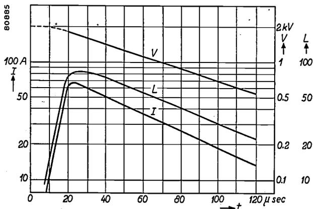
Fig. 10. Curves of voltage ( $V$ ), current ( $I$ ) and luminous output ( $L$ ) plotted logarithmically as functions of time ( $t$ ), for an LSD.3 experimental tube. During the decay period, the current is very nearly proportional to the voltage. The light output follows the current curve very closely, save that the peak of the former persists somewhat longer than that of the current.
