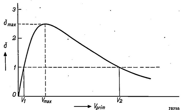
Fig. 1. Variation of the secondary emission factor  $\delta$  of a solid as a function of the accelerating potential  $V_{prim}$  of the primary electron beam.  $\delta = 1$  when  $V_{prim} = V_1$  and  $V_{prim} = V_2$ , and it reaches a maximum ( $\delta = \delta_{max}$ ) between the two, at  $V_{prim} = V_{max}$ .
