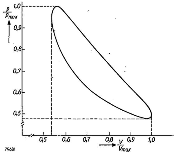
Fig. 7.  $p$ - $V$  diagram for the gas refrigeration cycle operating with a harmonic piston movement. The phases I-IV of the cycle merge to some extent; hence a smooth envelope is obtained instead of the discontinuous diagram shown in fig. 3b.
