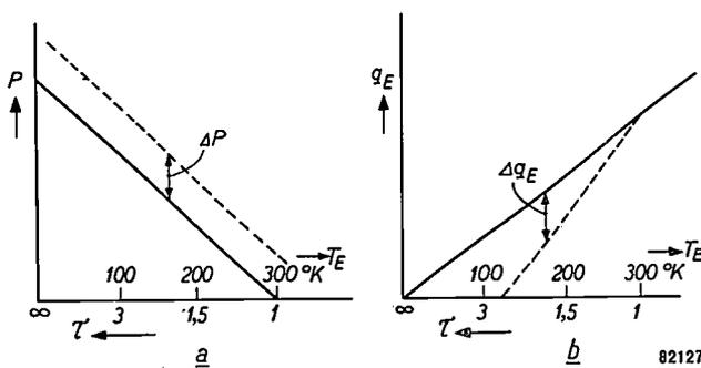
Fig. 1. Graphs of the shaft power  $P$  and the refrigerating capacity  $q_E$  of the gas refrigerating machine as functions of the temperature ratio  $\tau = T_C/T_E$  ( $T_C =$  temperature of the cooler  $\approx 300^{\circ}\text{K}$ ,  $T_E =$  the desired low temperature). The full lines apply to the ideal machine (see fig. 10 in I), the dotted line to a practical machine subject to various losses.
