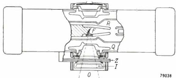
Fig. 13. X-ray tube *R* and shield with built-in ionization chamber *I* for measuring the dosage rate of the tube. *F* focus, *O* beam aperture, *Z* filter mount, *Q* oil-bath for insulation and cooling.
