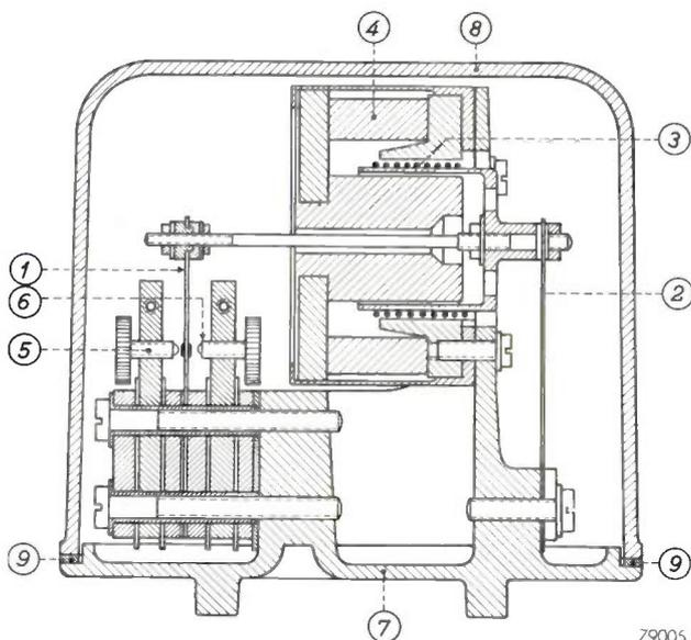
Fig. 4. Cross section of the vibrator. 1 and 2 are flat springs clamped at one end and maintained in vibration by an electrodynamic driving system comprising coil 3 and permanent magnet 4. The spring 1 makes contact alternately with screws 5 and 6. 7 base plate; 8 housing; 9 rubber gasket.
