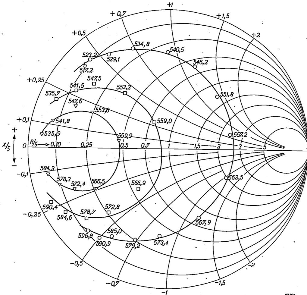
Fig. 17. Impedances as measured in the cases illustrated in fig. 16a, b and c, plotted in Smith's diagram. Theoretically the curves referring to a constant transformation ratio ( $\tau$ ) should be circles. The appropriate frequency (in Mc/s) is indicated at each point.
