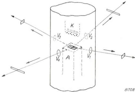
Fig. 4. Arrangement for using four diffraction devices simultaneously with a four-window X-ray tube. Through one pair of windows (spot focus windows  $V_1, V_2$ ) the source is seen as a small square surface, through the other pair as a very narrow line (line-focus windows  $V_3, V_4$ ). (In reality the anode  $A$  is positioned above the cathode  $K$ .)
