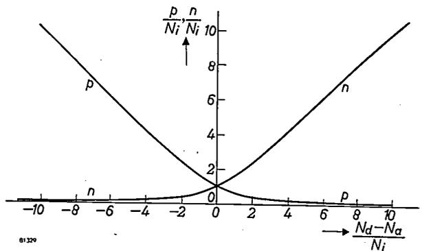
Fig. 2. Equilibrium concentrations of free electrons ( $n$ ) and holes ( $p$ ) in a semi-conductor, plotted as a function of the difference in concentration of donors and acceptors ( $N_d - N_a$ ). The concentration ( $N_i$ ) of free electrons in the pure semi-conductor ( $N_d = N_a = 0$ ) is taken as the unit of concentration for both co-ordinates.
