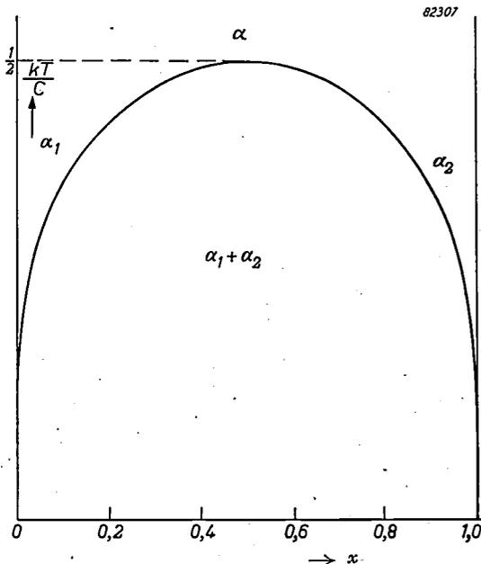
Fig. 5. Solubility curve (segregation curve) according to (III, 23) or (III, 24), giving the relationship between  $kT/C$  and the composition ( $P$  and  $Q$  in fig. 4) of the co-existing phases  $\alpha_1, \alpha_2$ .
