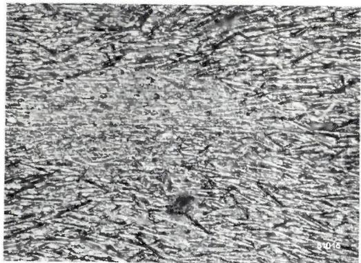
**Fig. 5.** Photo-micrograph of Ferroxdure with crystals aligned. In (a) the hexagonal basal planes are in the plane of the photograph, and in (b) they are at right angles to this plane. Magnification 10 $\times$ .
