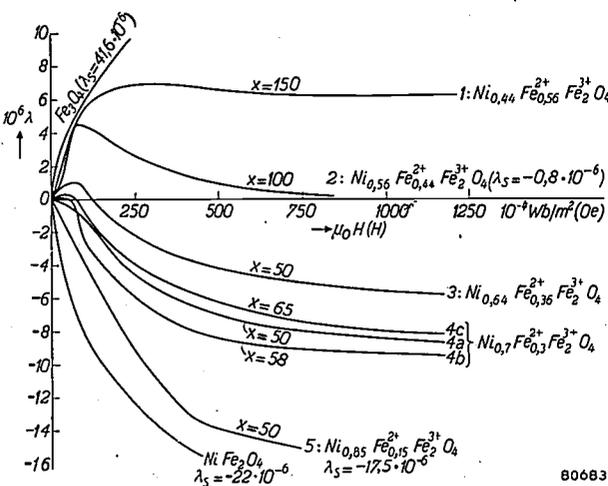
Fig. 5. Magnetostriction as a function of the magnetic field in polycrystalline samples of mixed crystals of nickel ferrous ferrite. All samples were fired at 1350°C, but in gas currents of different composition, viz. 600 ml/min CO<sub>2</sub> + x ml/min of a mixture of 90% N<sub>2</sub> and 10% H<sub>2</sub>. The value of x and the chemical composition of the ferrites are shown in respect of each curve.
