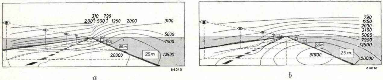
Fig. 2. Light distribution <sup>2)</sup> a) of the new asymmetric beam European headlamp bulb, b) of the latest type of American sealed beam lamp.
