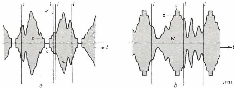
Fig. 2. Vision carrier amplitude as a function of time  $t$ . a) with positive modulation, b) with negative modulation.  $w$  level corresponding to white in the picture,  $z$  black level,  $s$  synchronizing pulses,  $i$  interference pulses.
