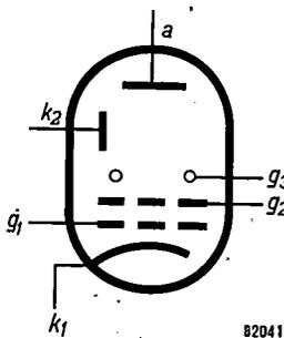
Fig. 9. Schematic representation of a secondary emission tube.  $k_1$  thermionic cathode,  $g_1$  control grid,  $g_2$  screen grid,  $g_3$  suppressor grid,  $k_2$  dynode (secondary emission cathode),  $a$  anode.
