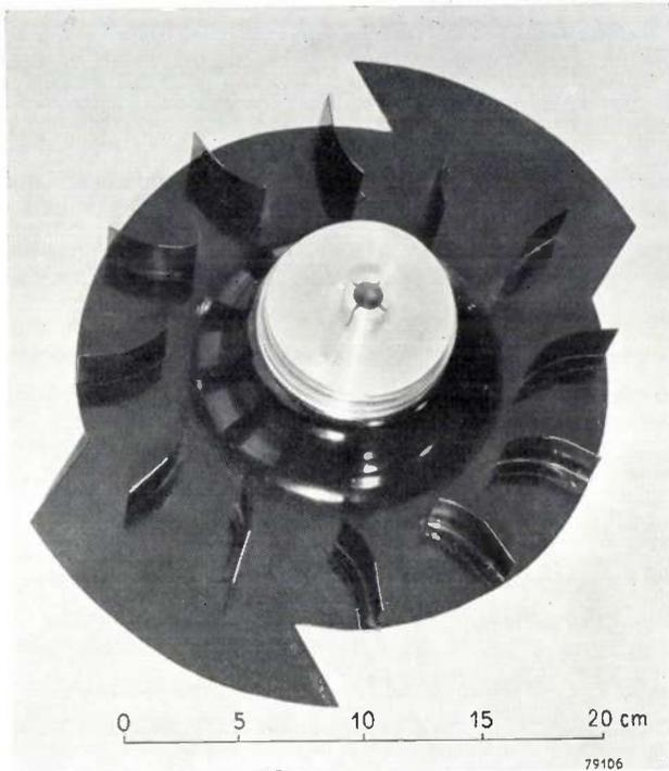
Fig. 6. The two-sector shutter. The frame sector and the flicker sector each cover  $50^\circ$ . The sectors are so shaped that the interception of the beam takes place parallel to the (long) side of the film gate, and therefore at a slightly higher speed than would be possible if sectors with truly radial edges were employed. Note also the large overall diameter, which enables the shutter to be used as a flywheel, and also the vanes which enable it to be used as a fan.
