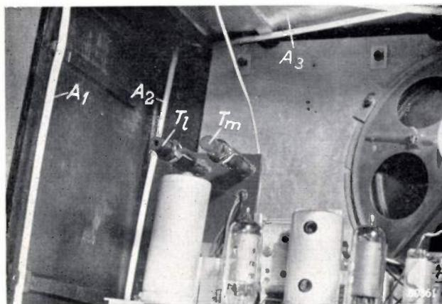
Fig. 8. Interior view of receiver BX 430 A-10. The two crossed frame aerials, ( $A_1$ ,  $A_2$ , each consisting of two turns in this case) are partly visible.  $T_1$  h.f. transformer for long wave reception,  $T_m$  h.f. transformer for medium wave reception, both having Ferroxcube cores.  $A_3$  capacitive plate aerial for short wave reception.
