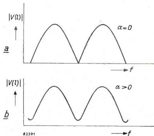
Fig. 11.  $|V(l)|$ , plotted against  $f$  in the case of total reflection a) with linear deflection, but without attenuation, b) with linear deflection and attenuation. In case (b),  $|V(l)|$  remains above the zero line.
