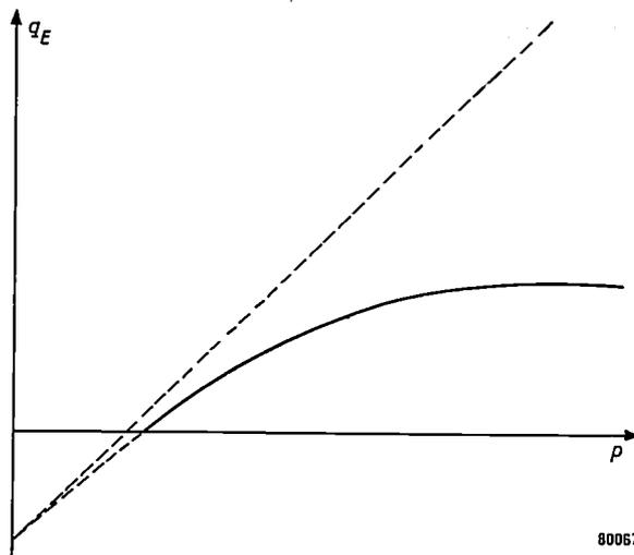
Fig. 4. Variation of the refrigerating capacity  $q_E$  with the pressure  $p$  in the refrigerator. According to the theoretical formula (equation) (13), part I) the dotted straight line would be expected. The measured curve deviates from this straight-line as shown by the full curve. Clearly there is a surprising decline of the refrigerating capacity at increasing pressure in the high-pressure range.
