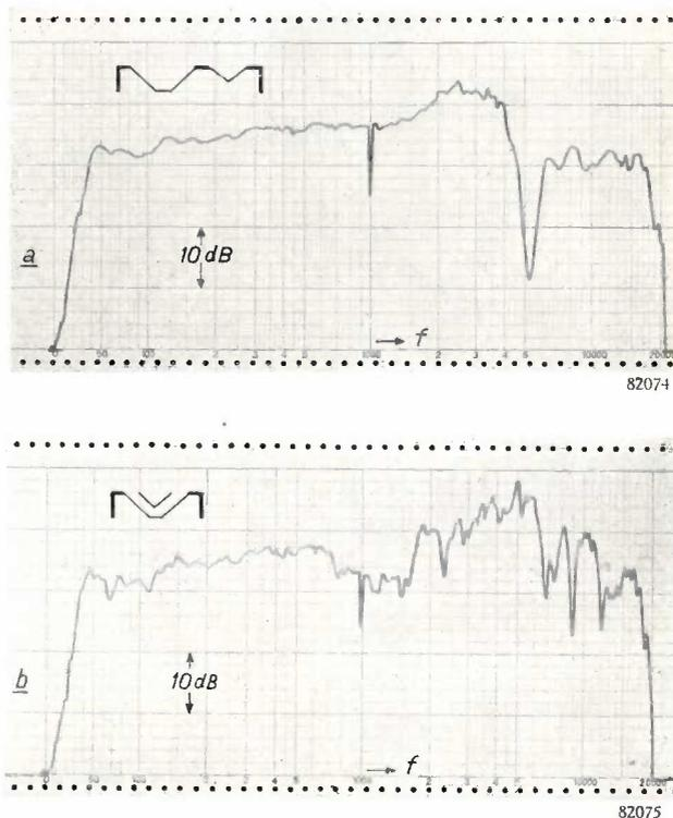
Fig. 6. a) Response curve ( $p$  plotted against  $f$ , for constant speech coil current) for a tweeter and main loudspeaker mounted side by side in the same cabinet. b) Response curve with tweeter placed inside the cone of the large speaker.
