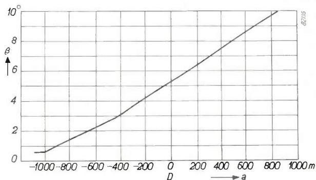
Fig. 23. The required angle of elevation ( $\beta$ ) of the beam axis of individual lights in the approach and runway lighting system, plotted against the distance ( $a$ ) between light and threshold.
