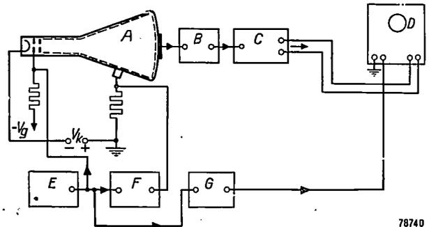
Fig. 13. Block diagram of the electronic equipment used to determine  $\delta$ . A picture-tube, B pre-amplifier, C output amplifier, D cathode ray oscilloscope, E generator for grid pulses, F the same for anode pulses, G time base.
