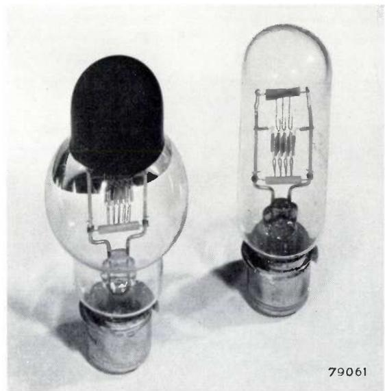
Fig. 4. The lamp employed in the 16 mm projector EL 5000 (left) and a conventional lamp for a 16 mm projector (right). The area covered by the filament of the left-hand lamp is rectangular, (same shape as the film gate), and the bulb of this lamp has a spherical form, part of which is internally silvered. Most of the material vaporised from the filament is deposited in the cylindrical top of this bulb, which is blackened to prevent light from escaping upwards.
