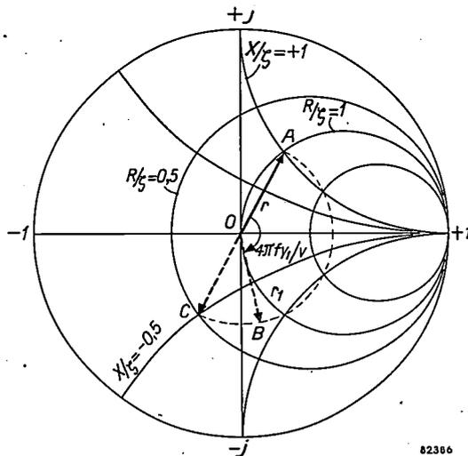
Fig. 5. The reflection coefficient  $r_1 = OB$  of the remainder of the transmission line, shown in fig. 4b, is determined by rotating vector  $r = OA$  in the Smith chart through an angle  $4\pi f y_1 / v$ .
