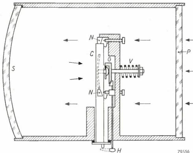
Fig. 3. Diagram illustrating the centering of the film. When the cassette *C* is inserted, the knob of the spherical pressure plate (fig. 2) engages with a bracket *G*. When the crank *H* is rotated a cam bearing on the bracket *G* allows the latter and hence also the cassette to be pulled to the right by spring *V* until the lugs *N* of the cassette rest upon the points of the set screws *J*. *S* is the concave mirror; *P* is the correcting plate.
