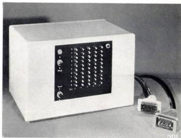
Fig. 7. Programme selector for camera with high-speed film transport. The 50 press-buttons correspond to the 50 periods of  $\frac{1}{5}$  second occurring within 10 seconds. Whether or not the magnetic clutch is to be engaged, i.e. whether or not a photograph is to be taken in any particular period is determined in advance by means of the appropriate button.
