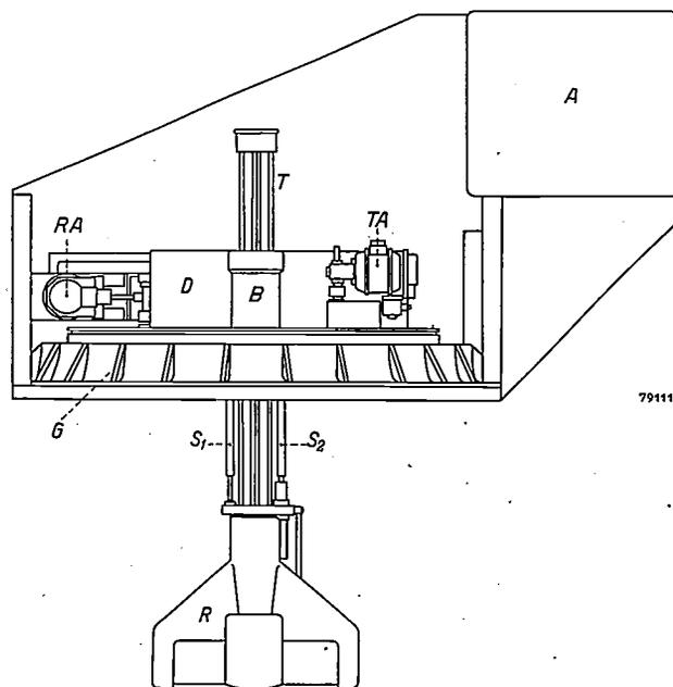
Fig. 6. Top view of main frame and X-ray tube mount with cover plates removed,  $G$  fixed frame, mounted on the same base as the H.T. generator  $A$ .  $RA$  motor unit for rotation,  $TA$  motor unit for traverse, mounted on rotary disc.  $S_1$ ,  $S_2$  threaded shafts, other letters as in fig. 5.
