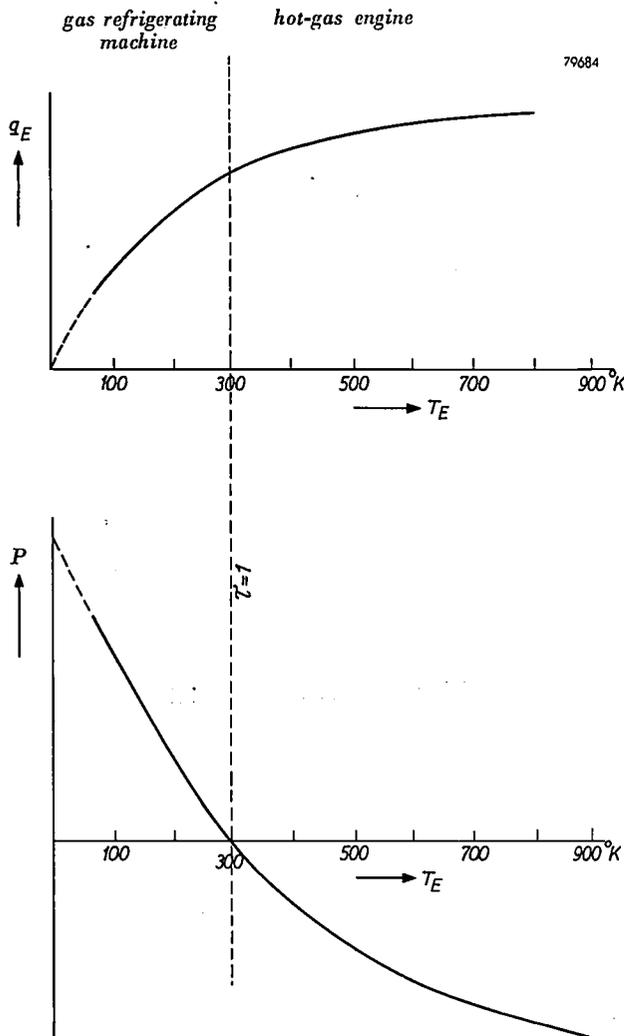
Fig. 10. Refrigerating capacity  $q_E$  and applied shaft power  $P$  as functions of the temperature  $T_E$  of the expansion space (for  $T_C = 300$  °K). One continuous curve is obtained, which applies to both the hot-gas engine ( $\tau < 1$ , to the right of  $T_C$ ) and the gas refrigerating machine ( $\tau > 1$ , to the left of  $T_C$ ).
