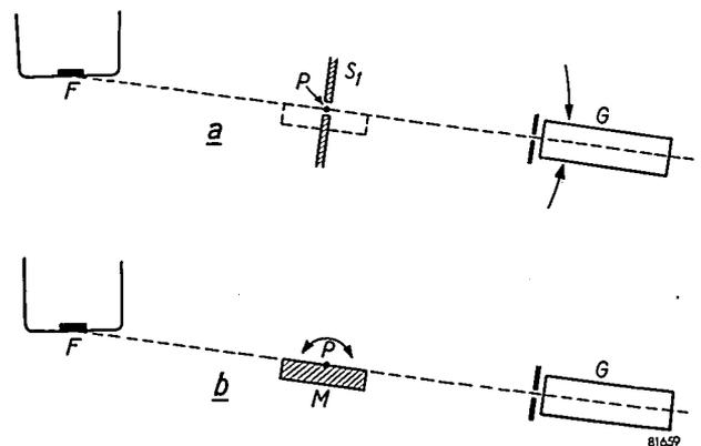
Fig. 14. Alignment and calibration procedure for the goniometer. a) A narrow slit  $S_1$  is placed at the specimen rotation axis  $P$ . The Geiger counter tube  $G$  is turned to the position in which the largest intensity of the direct X-ray beam transmitted by  $S_1$  is recorded ( $F$  = focus of X-ray tube). This is the zero angle position of the goniometer.
