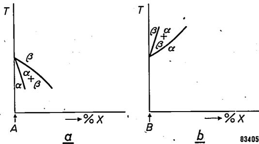
Fig. 1. a) The melting point or a crystallographic transition point of a component (A) moves to lower temperatures by adding a certain component (X), since the solubility in phase  $\alpha$  stable at low temperatures is less than the solubility in phase  $\beta$  stable at high temperatures. b) In the reverse case (B-X system) the melting point or transition point is shifted to higher temperatures.
