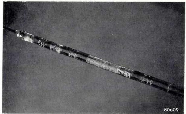
Fig. 7. Photograph of a "sintered" tube. The characteristic crazing of the inner surface of the glass has in this case shown itself in a very regular helical pattern.
