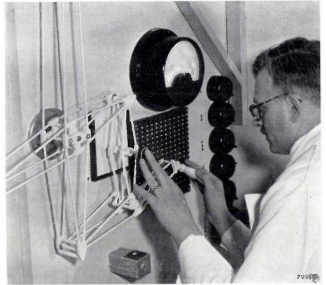
Fig. 4. The examiner at the instrument panel. Top: the voltmeter for checking the voltage of the lamps. With his left hand the examiner presses the needle down. Below: the electric signalling device which shows if the answer is correct.
