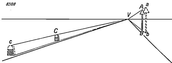
Fig. 6. Diagram showing the field of view of a motorist driving along a straight road.  $V$  is the vanishing point. Note the traffic sign ( $AB$ ) and the mile post ( $C$ ) as seen by the driver at a particular moment, and the same two objects ( $ab$  and  $c$ ) as seen a moment later. From the apparent motion of all points outwards from the vanishing point, the driver is able to judge his own direction and speed.
