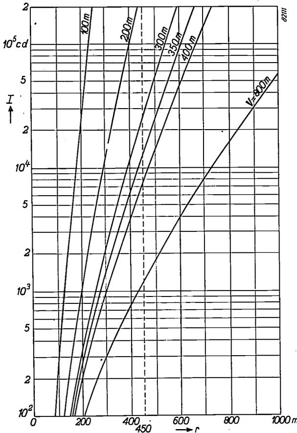
Fig. 9. Diagram showing the relationship between luminous intensity ( $I$ , in candelas) and visual range ( $r$ , in metres) for different meteorological visibilities ( $V$ , in metres). The curves are valid for an eye-illumination level  $E_c = 10^{-3}$  lux.
