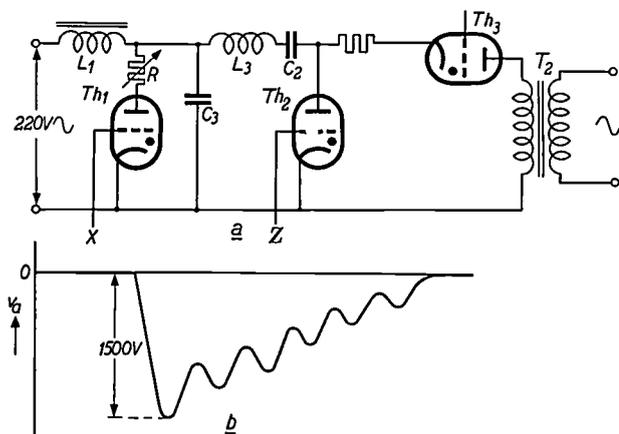
Fig. 8. a) Cheater circuit as in fig. 7a, but with "snubber" circuit  $L_3$ - $C_3$  for limiting the commutation factor to 80 VA/ $\mu\text{sec}^2$ . b) Voltage  $v_a$  appearing across the test valve.
