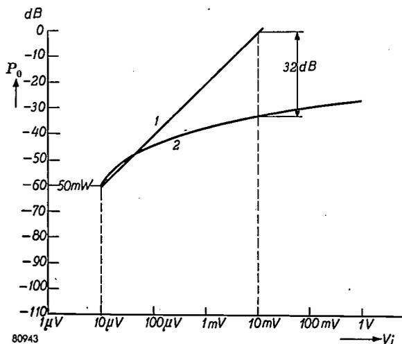
Fig. 16. Output signal  $P_0$  of a radio receiver as a function of the input voltage  $V_i$ , 1 without a.v.c., 2 with a.v.c. At  $V_i = 10$  mV the difference amounts to 32 dB. The vertical scale is made to correspond to the decibel scale of fig. 15.
