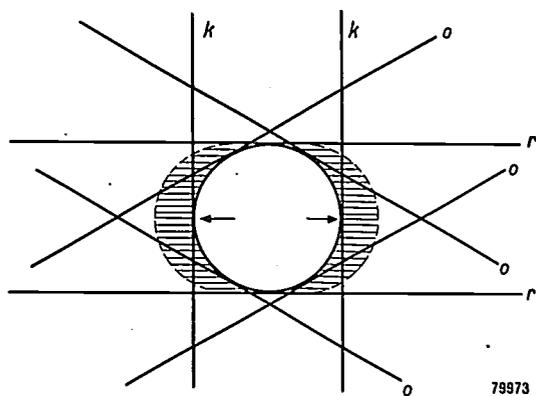
Fig. 5. A hole drilled perpendicular to a rhombic dodecahedral plane is surrounded by crystal planes of all the three main types *k*, *r* and *o* (shown schematically). Wear will occur mainly in the cube planes, so that the aperture will tend to assume an oval cross-section.
