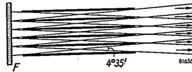
Fig. 8. Parallel slit system consisting of a number of molybdenum foils  $0.025 \text{ mm}$  thick, transmitting X-rays directed parallel to the foils and suppressing rays entering obliquely.  $F$  = focus. (The effect may be compared to that of the well-known Potter-Bucky grid for suppressing scattered radiation in X-ray diagnostics.)
