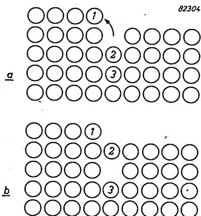
Fig. 2. The vacancies in a solid are assumed to form at the outer surface (a) and subsequently diffuse to the interior (b), this being equivalent to the outward diffusion of atoms (1, 2, 3).
