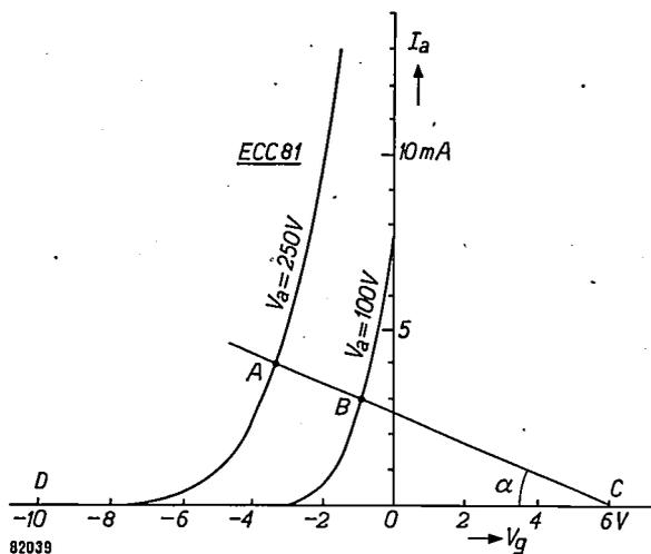
Fig. 7.  $I_a = f(V_g)$  characteristics for  $V_a = 100$  V and  $V_a = 250$  V of one half of double triode ECC 81. Note the straight line drawn through points  $A$  (at 4 mA on the characteristic for  $V_a = 250$  V) and  $B$  (at 3 mA on the characteristic for  $V_a = 100$  V). It will be seen that this line makes an angle  $\alpha$  with the  $V_g$  axis and cuts it at a point  $C$ .  $R_k$  (fig. 6) is equal to  $\cot \alpha$ . The required pulse amplitude is  $CD = 16$  V.
