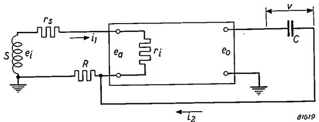
Fig. 9. Basic circuit of integrating unit for the deduction of the circuit equations.
