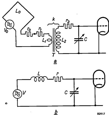
Fig. 17. a)  $L_0$  frame aerial with low impedance, coupled to tuning capacitor  $C$  via an h.f. transformer  $T$ . The voltage induced in the frame aerial is  $V_0$ . The resistance of the frame, of the primary coil (self-inductance  $L_1$ ) and the secondary coil (self-inductance  $L_2$ ) are  $r_0, r_1$  and  $r_2$  respectively. The coupling coefficient is  $k$ . b) Equivalent circuit of (a).
