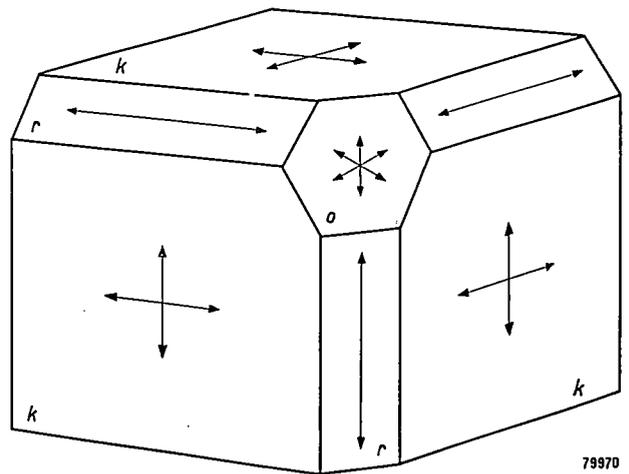
Fig. 2. Schematic diagram of preferred orientations for diamond grinding. The preferred directions on the various crystal faces are indicated by arrows whose lengths are proportional to the ease of grinding. Cube planes are indicated by *k*, rhombic-dodecahedral planes by *r*, and octahedral planes by *o*. (Diagram taken from the article referred to in <sup>2</sup>.)
