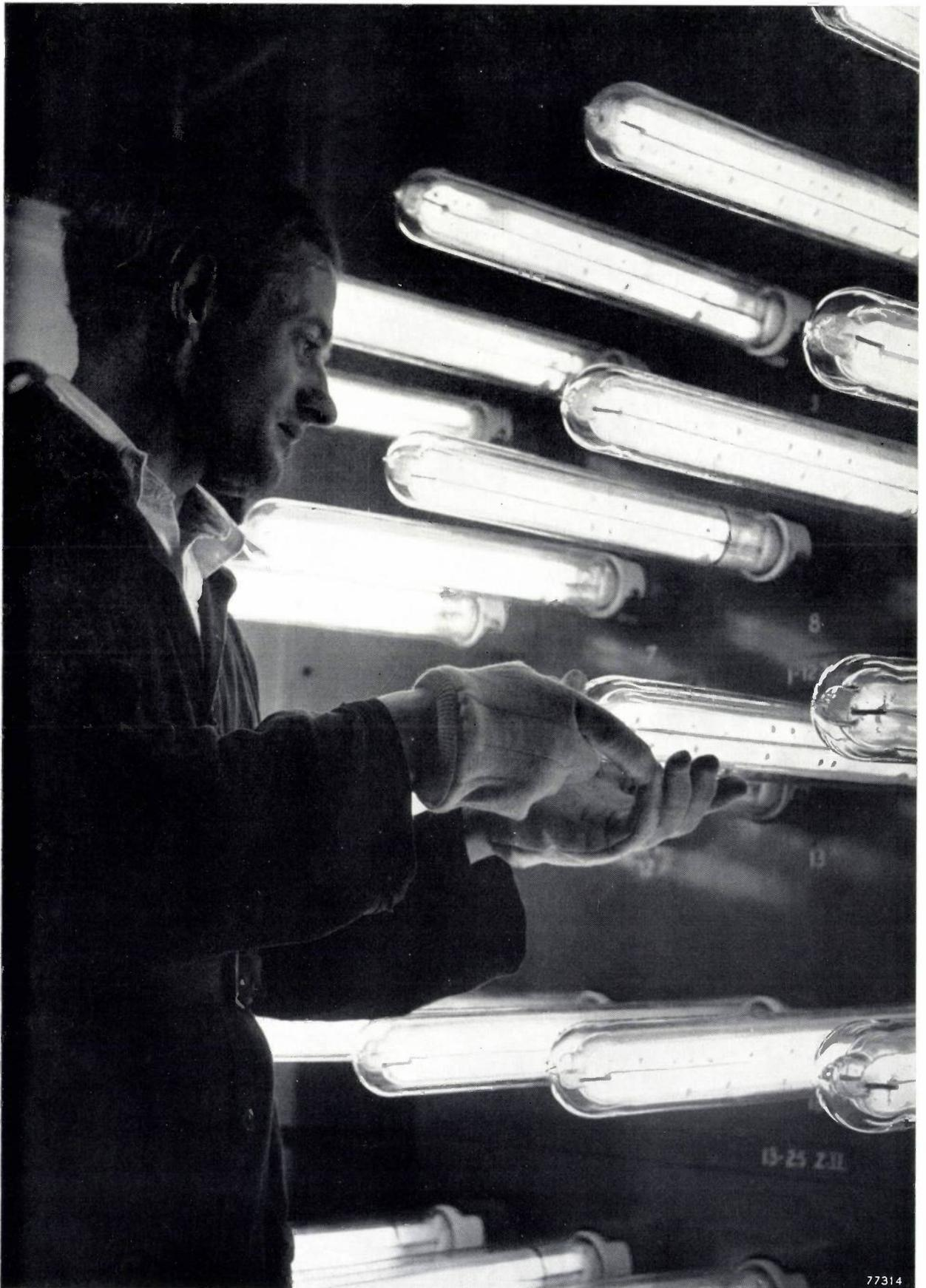
The photograph shows a group of sodium lamps during the "seasoning" process — a stage in the manufacture during which the sodium is distributed in droplets along the discharge-tube, in order to ensure a uniform brightness in the finished lamp.
