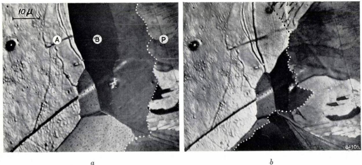
Fig. 3. The boundary between the two austenite crystals *A* and *B* moves in the direction of the approaching pearlite *P*. The dotted line shows the boundary between the pearlite and the austenite.
