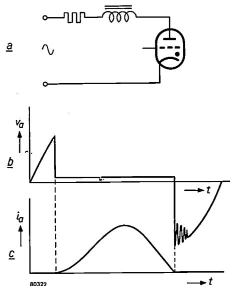
Fig. 5. With a thyratron having a partly inductive load, circuit parameters can be so chosen that conduction ceases near the negative peak of the A.C. voltage. The current decay, however, is slow, so the commutation factor is still not very high. (At current extinction, oscillations are set up in the circuit formed by the inductance and stray capacitance.)
