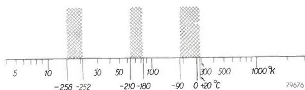
Fig. 1. Temperature ranges covered by conventional refrigerators and liquefiers. Evaporation type refrigerators normally go down to about  $-80^{\circ}\text{C}$ . The equipment used for the liquefaction of air operates in the range  $-180^{\circ}\text{C}$  to  $-210^{\circ}\text{C}$ . Hydrogen liquefiers operate between  $-252^{\circ}\text{C}$  and  $-258^{\circ}\text{C}$ .
