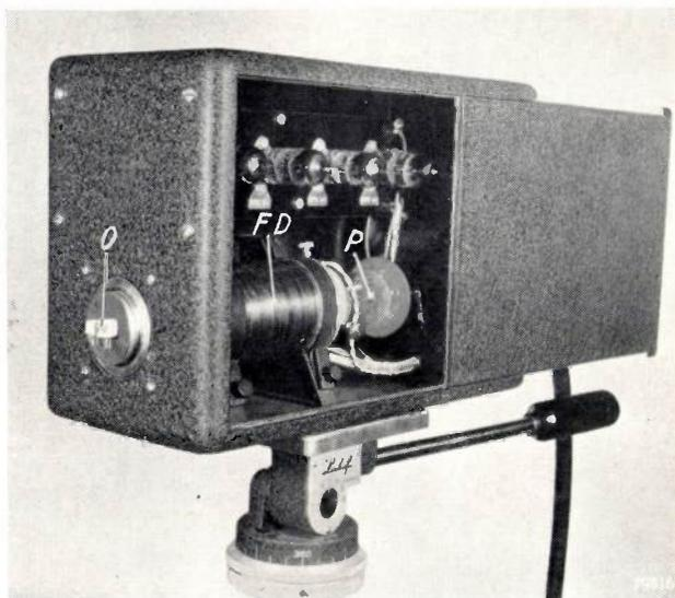
Fig. 3. The camera, showing the camera tube (*P*) and the focusing and deflection coils (*FD*). Above these is the video pre-amplifier. On the front of the camera, fixed over the lens aperture, are the two transistors (*O*), which served as the object in the set-up shown in fig. 2.
