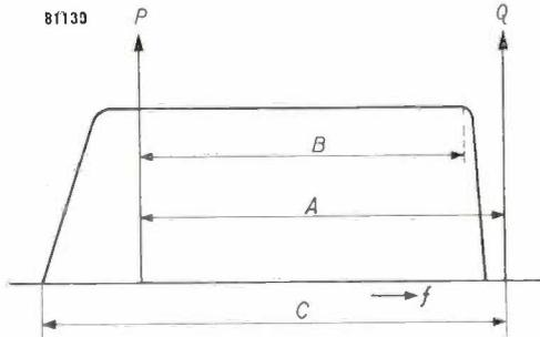
Fig. 1. Frequency spectrum of a television transmitter with asymmetrical side band ("vestigial side band").  $f$  frequency,  $P$  vision carrier,  $Q$  sound carrier,  $A$  frequency-interval between the two,  $B$  bandwidth of complete side band transmitted,  $C$  channel width.
