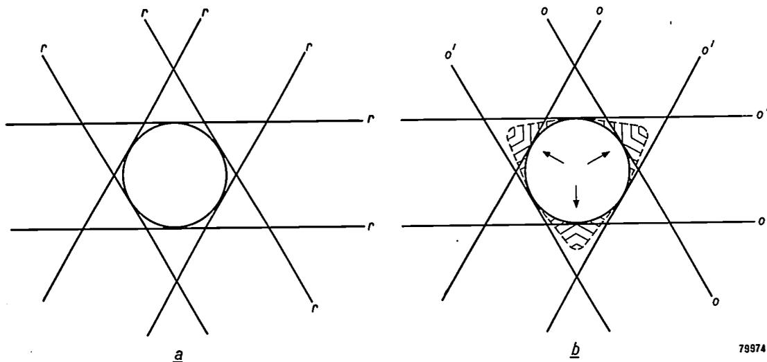
Fig. 6. a) A hole drilled perpendicular to an octahedral plane is surrounded by rhombic-dodecahedral planes *r*, all wearing at a uniform rate. b) It is supposed that, in the course of the wearing process, these planes largely give way to the octahedral planes *o* and *o'*, of which only those marked *o* will wear because of their favourable orientation with respect to the drawing direction. The ultimate cross-section of the hole will be triangular.
