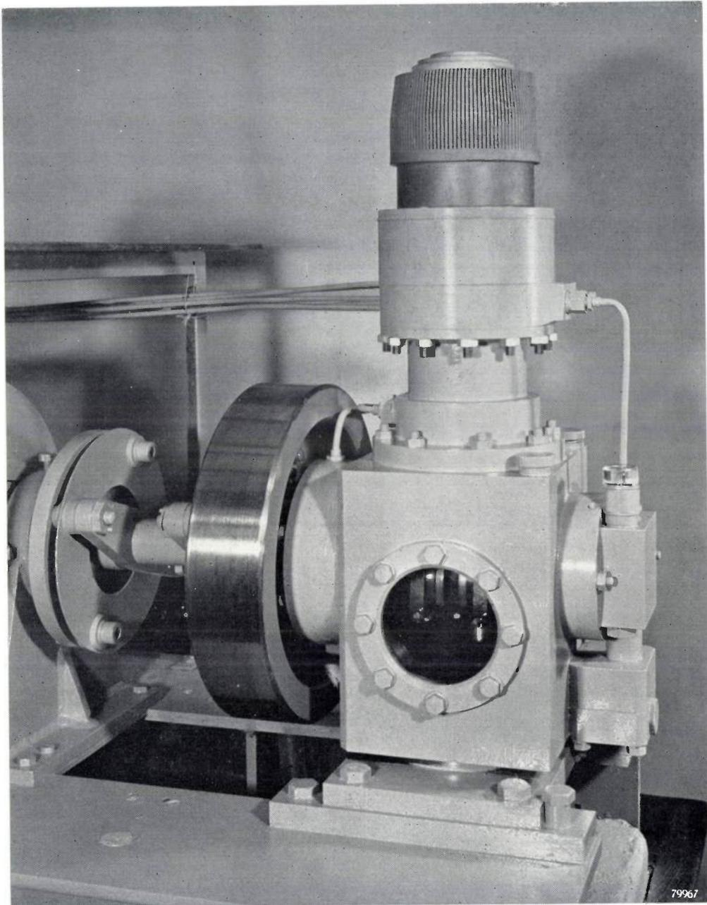
Fig. 8. Photograph of the gas refrigerating machine.
