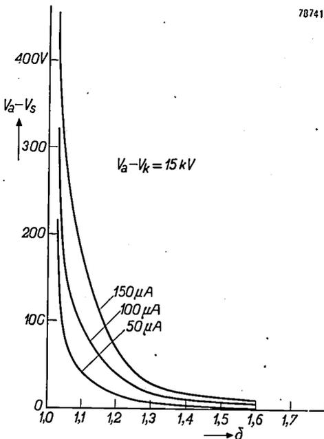
Fig. 14. Potential difference  $V_a - V_s$  between anode and screen as a function of  $\delta$ , for  $I_p = 50 \mu\text{A}$ ,  $100 \mu\text{A}$  and  $150 \mu\text{A}$ . Accelerating potential 15 kV.
