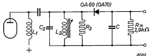
Fig. 9. Video circuit containing a germanium diode type OA 60 or OA 70.
