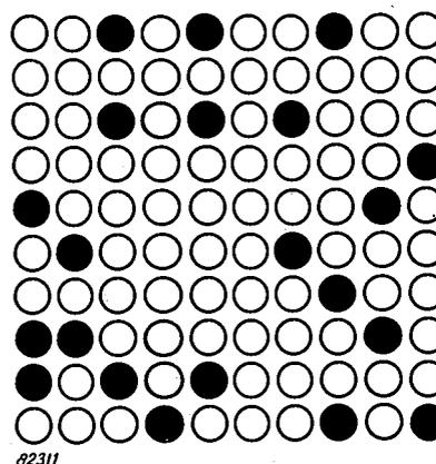
Fig. 11. Schematic representation of a solution of molecules  $B$  (black) in a liquid of molecules  $A$  (white). The molecules  $A$  and  $B$  are of about the same size and are statistically distributed in the quasi-lattice.
