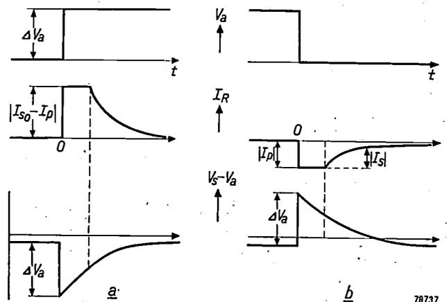
Fig. 9. a) Form of the screen current and potential difference  $V_s - V_a$  when a positive pulse  $\Delta V_a$  is superimposed on the anode potential. b) The same when the anode potential is reduced from  $\Delta V_a$  to zero.
