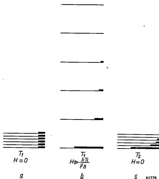
Fig. 4. Adiabatic demagnetization.
