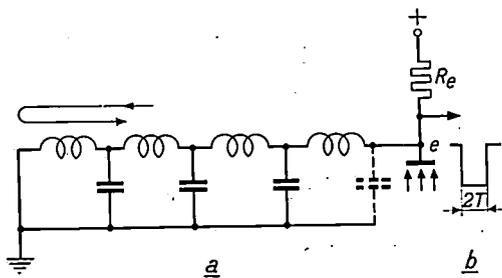
Fig. 16. Diagram showing (a) that if a delay line of characteristic impedance  $R_e$ , short-circuited at the free end, be connected to anode  $e$  (fig. 13), the electron avalanche will produce on this anode square pulses (b), whose duration is twice the delay ( $T$ ) in the line.
