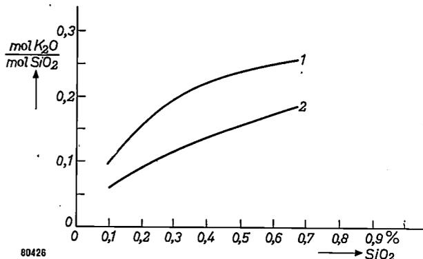
Fig. 3. Relationship between the molecular ratio K<sub>2</sub>O-SiO<sub>2</sub> in the binder, and the silicate concentration (% by weight) in the solution. 1) screens made by the sulphate method, 2) screen made by the barium method.
