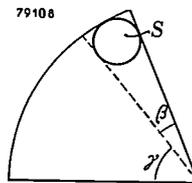
Fig. 5. The covering angle associated with the shutter sectors. The film must not start to move until the light beam (section S) is completely cut off. Hence the sector must be an angle  $\beta$  wider than the angle  $\gamma$  corresponding to the frame-shift period.
