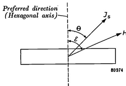
Fig. 2. The state of equilibrium of the magnetization  $J_s$  in a uniaxial magnetic particle when an external field  $H$  is applied at an angle  $\epsilon$  to the preferred direction.
