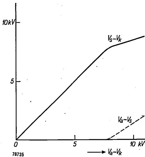
Fig. 7. Potential difference  $V_s - V_k$  as a function of the accelerating potential  $V_a - V_k$  of a tube containing a screen. The threshold potential in this case is about 7 kV, but is not clearly defined. Dotted line:  $V_a - V_s$ .
