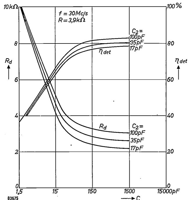
Fig. 10. Effect of the load-capacitance  $C$  on the detection efficiency  $\eta_{det}$  and equivalent attenuation resistance ( $R_d$ ) of the video detector circuit shown in fig. 9. These quantities also depend upon the tuning capacitance  $C_2$ ; the curves for several values of this parameter are given. The curves are valid for a carrier-wave frequency of 30 Mc/s and a load-resistance  $R$  of 3.9 kΩ.
