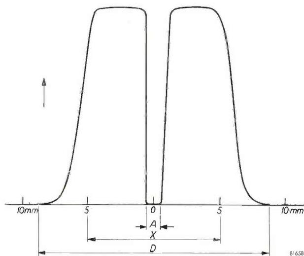
Fig. 11. Radial distribution of sensitivity (in arbitrary units) of chlorine-quenched Geiger counter tube (type 62019).  $A$  = width of the axial anode wire and bead.  $X$  = width of X-ray beam when using the new X-ray optical system.  $D$  = inside diameter of the Geiger tube.
