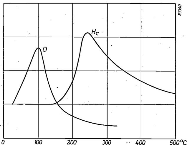
Fig. 11. Rough curves of the mechanical hardness ( $D$ ) and the coercive force ( $H_c$ ) for a mild steel containing 0.07% of carbon, after quenching from 680 °C and heating for one hour at the temperatures indicated on the abscissa (from data of Köster<sup>8</sup>).
