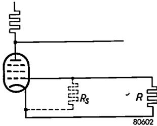
Fig. 7. Equivalent circuit of the grid circuit of the oscillator valve in an  $R$ - $C$  oscillator, showing the apparent resistance  $R_s$  resulting from the flow of grid current.  $R$  is the total terminating impedance of the filter.
