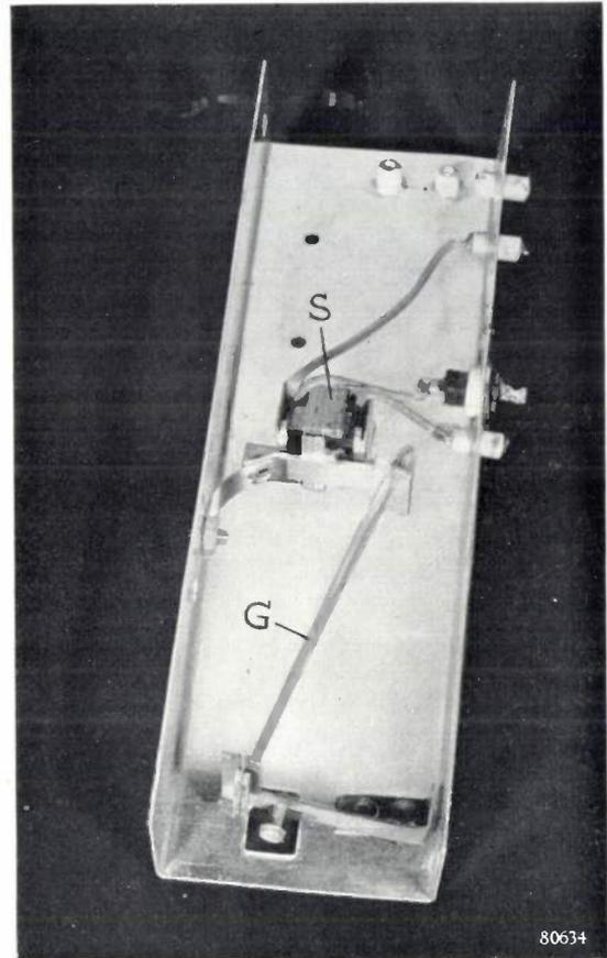
Fig. 4. Hygrometer. The variation in length of a piece of gold-beater's skin *G* is converted into a variation in self-inductance by virtue of the fact that the skin controls the width of the air-gap in the magnetic circuit of coil *S*.
