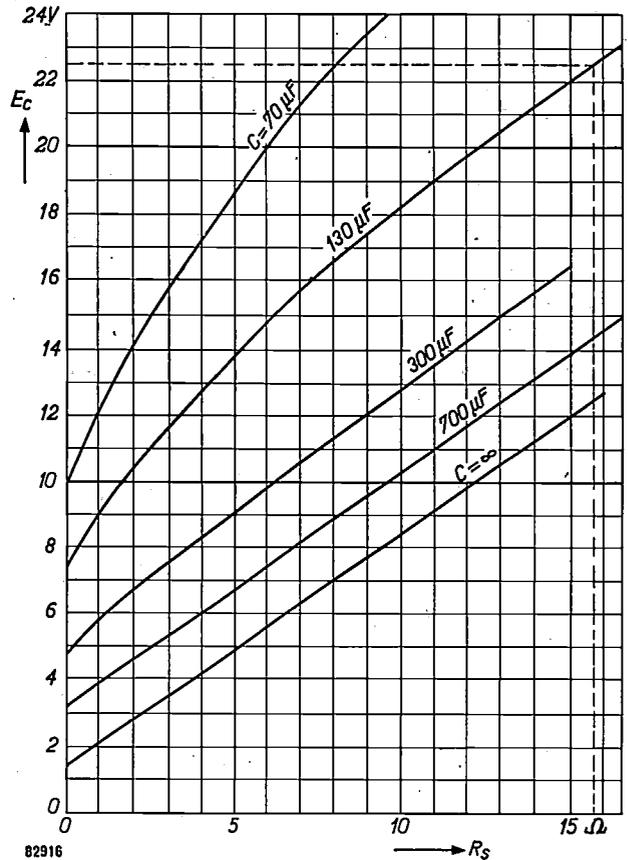
Fig. 5. Calculated values of the maximum permissible resistance  $R_s$  in series with the bulb, plotted against the battery voltage  $E_c$  for various capacitances  $C$ , for capacitor ignition.
