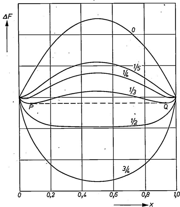
Fig. 4. Free energy of mixing  $\Delta F$ , according to (III, 20) and (III, 21), as a function of the atomic fraction  $x$  for various values of  $kT/C$ . At low temperatures, segregation occurs as this is more favourable from the point of view of internal energy. For a given temperature, the compositions of the two co-existing phases are defined by the points of contact  $P$  and  $Q$  of the (dashed) double tangent to the  $\Delta F$ -curve.
