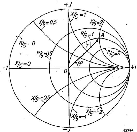
Fig. 3. Smith chart, showing the two orthogonal families of circles, the one referring to constant  $R/\zeta$  and the other to constant  $X/\zeta$ .  $A$  is the point of intersection of the circles corresponding to  $R/\zeta = 1$  and  $X/\zeta = 2$  ( $R$  being the resistance, and  $X$  the reactance of the terminating impedance  $Z$  from fig. 1). Vector  $OA$  is the reflection coefficient  $r$  with modulus  $|r|$  and argument  $\varphi$ .
