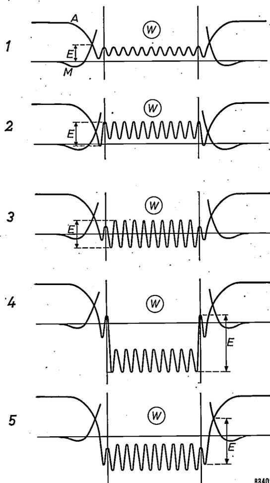
Fig. 12. Schematic representation of the passage of a gas through a metal wall ( $W$ ). The "potential curves"  $M$  and  $A$  give the energy of a gas molecule and of its two separate atoms, respectively, as a function of position. The greatest potential jump occurring ( $E$ ) determines the rate of the whole process. It may occur at any one of five different locations, corresponding to cases 1-5 summarized in the text.
