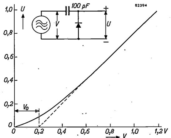
Fig. 13. Relationship between the detected D.C. voltage ( $U$ ) and the amplitude ( $V$ ) of the high-frequency A.C. voltage, for a given germanium diode. The value ( $V_0$ ) at which the straight part of the characteristic (produced by the diode) would cut the  $V$  axis is about 0.2 V.
