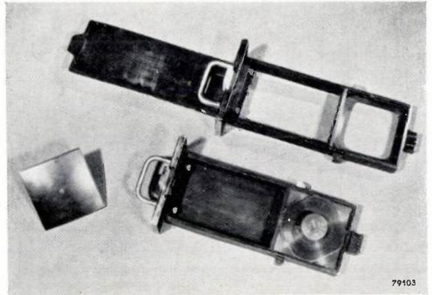
Fig. 2. A cassette (foreground) with the spherical pressure plate inserted; note the three lugs provided to ensure accurate centering. Above, the cassette with the spherical pressure plate (left) removed and the cassette cover withdrawn.
