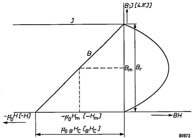
Fig. 1. Demagnetization curve for a material of which  $JH_c = \infty$ . In the case here considered,
