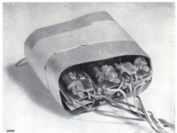
Fig. 9. a) Electronic section of the radio sonde. The three oscillators are mounted on the left-hand panel and the transmitter on the right-hand panel. b) In the assembled sonde the two panels lie back to back and are enclosed in a cardboard cover. The measuring elements and batteries are connected to the panels by flexible leads.
