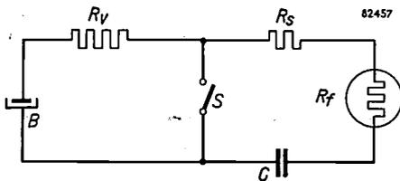
Fig. 4. Ignition with the aid of a capacitor (C). This capacitor is charged by a very small current through the resistance  $R_f$  of the "Photoflux" bulb and the high series resistance  $R_v$ . When the circuit is closed, C is discharged across  $R_f$ .  $R_s$  is the extra series resistance present.
