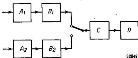
Fig. 17.  $A_1, A_2$  particle counters, and  $B_1, B_2$  their associated pulse shapers. If the pulses produced by  $B_1$  and  $B_2$  differ in duration, another pulse shaper (C) should be added to convert these pulses into pulses of uniform duration. D scaler.
