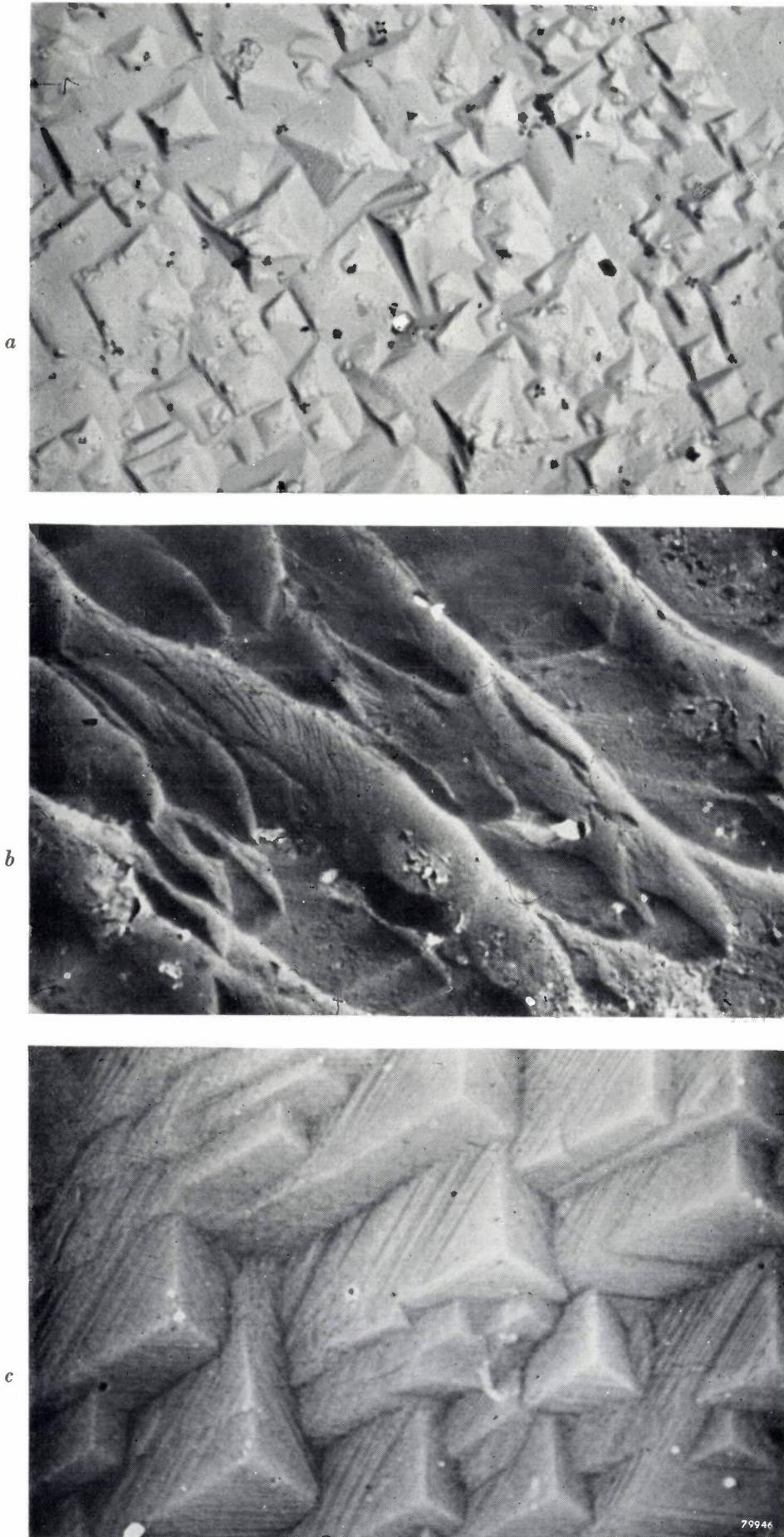
Fig. 9. Electron photo-micrographs of etched crystal faces of diamond. Enlargement 10 000  $\times$ .
