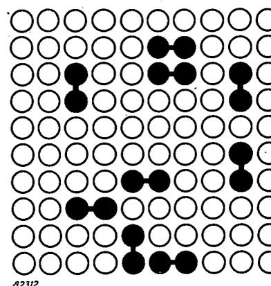
Fig. 12. Schematic representation of a statistical distribution of dumb-bell shaped molecules  $B$  (black) in a liquid of spherical molecules  $A$  (white). The dumb-bell shaped molecules occupy two adjacent sites of the quasi-lattice.
