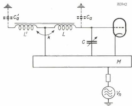
Fig. 13. Circuit for compensating the aerial-effect of a Ferroxcube aerial  $L$ .  $L'$  = compensating coil coupled with  $L$  ( $L_1$  in fig. 11).  $C_a$  and  $C_a'$  = capacitance of  $L$  and  $L'$  respectively with respect to the surroundings. At suitable values of  $C_a'$  and of the coupling coefficient  $k$ , no interference voltage will be produced across the tuning capacitor  $C$  ( $V_n$  = source of interference).  $M$  = chassis.
