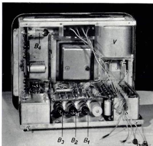
Fig. 3. a) The meter GM 6010 showing the battery compartment. b) the chassis; B<sub>1</sub>, B<sub>2</sub> and B<sub>3</sub> are the amplifier valves; B<sub>1</sub> is the oscillator valve. V is the vibrator.
