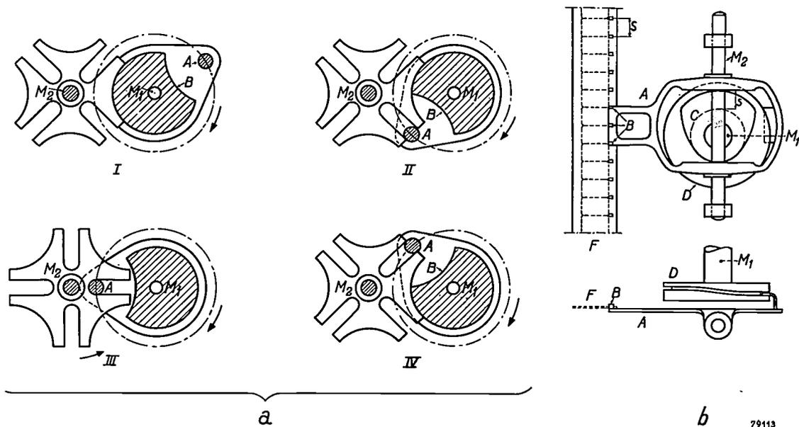
Fig. 7. Principle of the Maltese cross movement and the claw mechanism for intermittent film movement.
