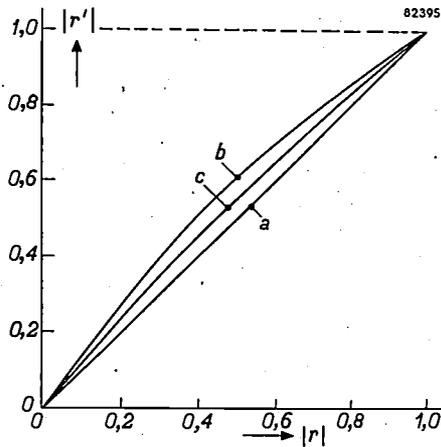
Fig. 14. Given the detection characteristic shown in fig. 13, and with  $E$  of the same order of magnitude as  $V_0$ , the measured value of the reflection coefficient will be too high ( $|r'|$ ); note the deviation of curve *b* with respect to the straight line at an angle of  $45^\circ$ . Attenuation reduces this error, as will be seen from the curve (*c*) referring to  $e^{-2\alpha l} = 0.8$ .
