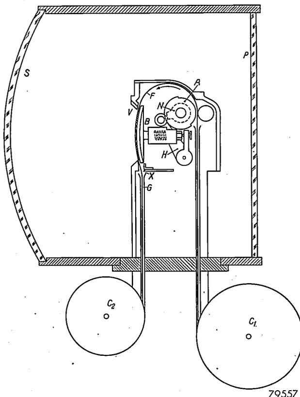
Fig. 5. Section (greatly simplified) of the camera for serial exposures. Note the friction roller *A* which actuates the spherical pressure plate *B* by means of a cam *N* and a lever *H* and aided by a pressure roller, pushes the film strip *F* past the film gate *V*. Also shown are the cutter at *X* and the funnel-shaped guide *G* to the receiver-cassette *C*<sub>2</sub>, which receives the film as fed forward. *C*<sub>1</sub> is the dispenser-cassette.
