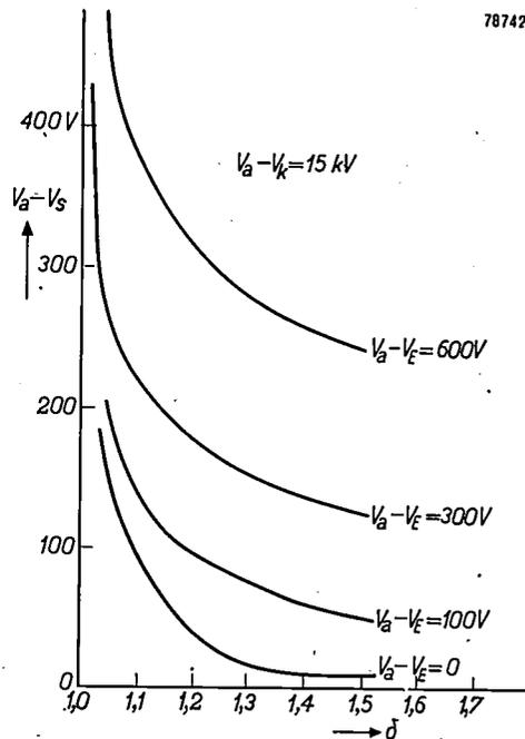
Fig. 15. Potential difference  $V_a - V_s$  plotted as in *fig. 14* for  $I_p = 100 \mu\text{A}$ ,  $V_a - V_k = 15 \text{ kV}$ , for a tube containing a ring-shaped electrode  $E$  between the screen and the inner coating, at different values of the potential difference  $V_a - V_E$ .
