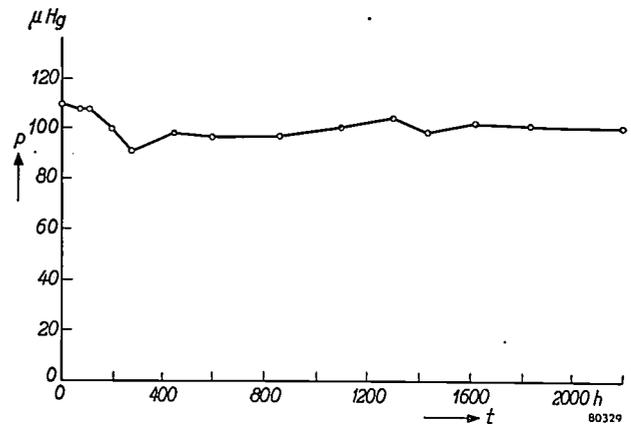
Fig. 12. Gas pressure *p* in xenon-filled Mullard MT 5545 thyatron during a test for gas clean-up. The first 1270 hours the valve was run with a commutation factor *f*<sub>c</sub> = 450 VA/μsec<sup>2</sup>, the rest of the time with *f*<sub>c</sub> = 750 VA/μsec<sup>2</sup>.
