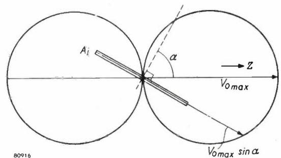
Fig. 14. The figure-of-eight polar diagram of an inductive aerial ( $A_i$ ) having no capacitive component. The signal voltage in the aerial is  $V_{0max} \sin a$ ,  $a$  being the angle between the perpendicular to the plane of the loop and the direction  $Z$  of the transmitter.
