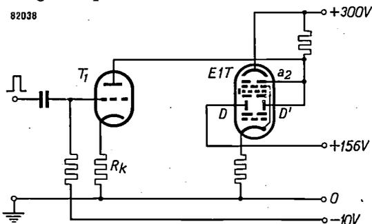
Fig. 6. Circuit to reduce the step-time by means of an auxiliary triode ( $T_1$ , "charging valve") which becomes momentarily conductive when gated by an incoming pulse and then supplies a negative charge to the right-hand deflector plate ( $D'$ ) of the scaler tube. The potential of the left-hand deflector plate ( $D$ ) is constant (156 V).  $R_k$  cathode resistor.
