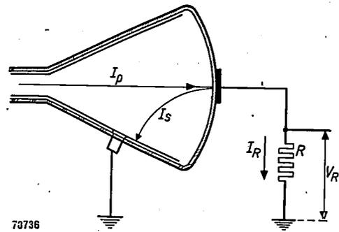
Fig. 8. Method of determining  $\delta$  by means of a current measurement.
