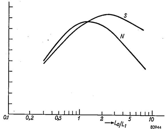
Fig. 18. Sensitivity  $S = Qh$  and signal-to-noise factor  $N = Qh^2$  plotted as functions of  $L_0/L_1$ , for  $k^2 = 0.70$  and  $Q_0 = Q_1 = Q_2$ .
