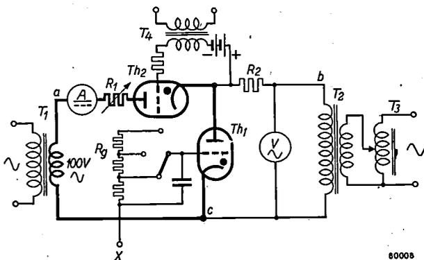
Fig. 4. Cheater circuit for measuring grid current under full operating conditions.  $Th_1$  thyatron under test.  $Th_2$  auxiliary thyatron.  $T_1$  low voltage transformer (100 V).  $T_2$  high voltage transformer, fed from variable autotransformer  $T_3$ .  $R_1$  load resistor.  $R_2$  current limiting resistor in H.T. circuit.  $R_g$  bank of grid resistors. Firing pulses are applied at X and also to transformer  $T_4$  (see fig. 6).
