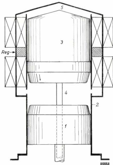
*Fig. 5.* Principle of the displacer machine. *1* = main piston, moving in cylinder *2*. *3* = displacer, causing a periodic flow of gas back and forth between the spaces *4* and *5*. The gas then flows through the annular heat exchangers surrounding the displacer.
