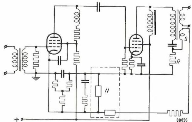
Fig. 6. Simplified diagram of a two-stage amplifier for symmetrical cables. Current feedback is provided by resistor  $R$ , whilst voltage feedback is effected by the secondary winding  $S$ . The equalizing network  $N$  ensures a straight frequency-response curve of cable plus amplifier.
