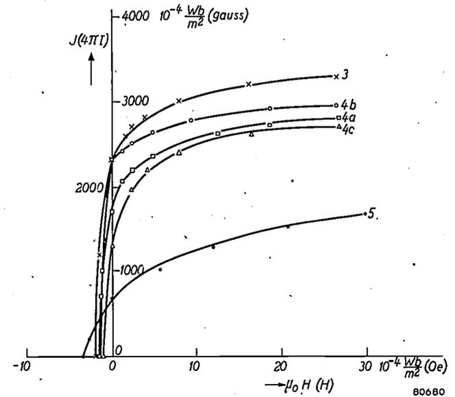
Fig. 6. Upper branch of the hysteresis loop for decreasing fields, for some of the ferrites in fig. 5.
