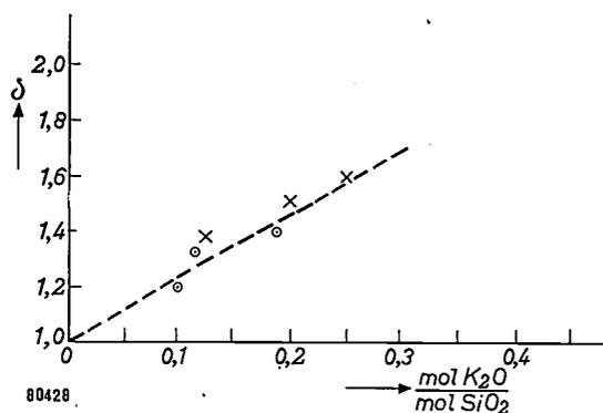
Fig. 5. Secondary emission factor  $\delta$  of the fluorescent screen plotted against the molecular ratio  $\text{K}_2\text{O-SiO}_2$  in the binder. The points denoted by crosses relate to screens prepared by the sulphate method; those shown as circles relate to the barium method.
