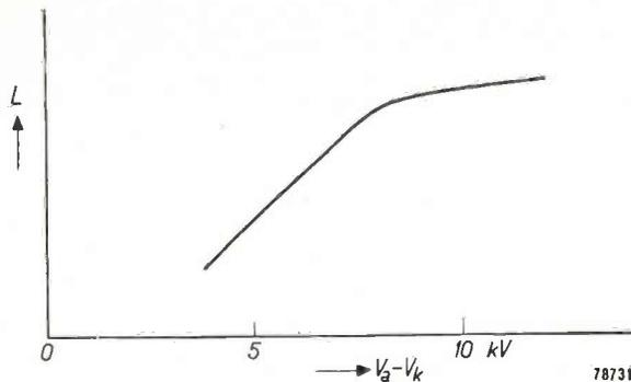
Fig. 3. Luminance  $L$  of the screen (on relative scale) as a function of the accelerating potential  $V_a - V_k$ . The threshold potential (at which the increase in luminance practically ceases owing to the charge on the screen) is here about 8 kV.
