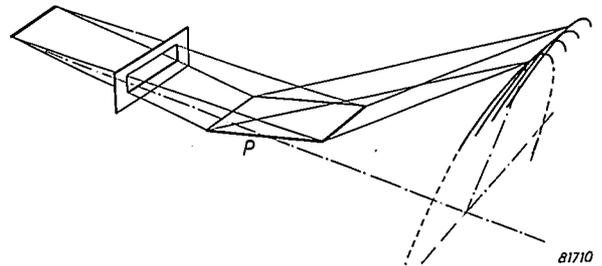
Fig. 9. If the parallel slit systems in fig. 7b are omitted, each point of the line source in a given specimen position produces a diffraction line of its own, covering the whole length of the counter window and being curved as a ring with its centre of curvature in the  $0^\circ 2\theta$  direction. The curved lines of all source points are integrated to form a broadened diffraction line of asymmetric profile.
