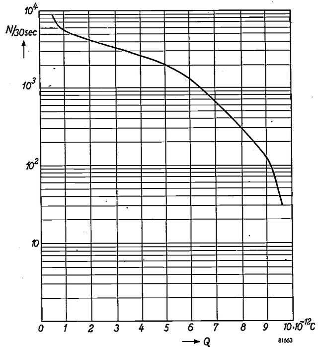
Fig. 7. Number of pulses  $N$  per 30 seconds versus the output charge  $Q$  per pulse in the case of a photo-multiplier not specially designed for radio-spectrometry.
