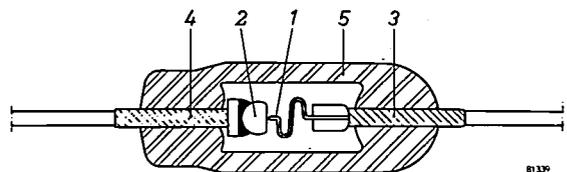
Fig. 8. Construction of a point-contact germanium diode of the latest type. The pointed contact spring 1 presses against the germanium crystal 2. The contact spring and the crystal are secured to supporting pins 3 and 4, sealed into a glass bulb 5 as protection against the atmosphere.
