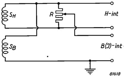
Fig. 8. Input-system for the integrators, suitable for the recording of the magnetization *J* as a function of the field strength. Correction for the wire size of the *B* coil can also be made with this circuit. *S<sub>H</sub>* search coil for the measurement of *H*; *S<sub>B</sub>* search coil for the measurement of *B* or *J*; *R* potentiometer.
