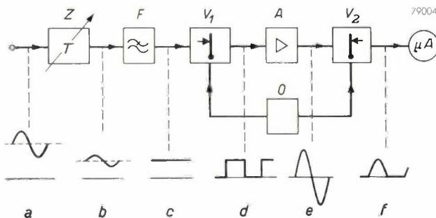
Fig. 1. Block diagram of the D.C. voltmeter GM 6010. *Z* variable attenuator (T-network). *F* low-pass filter. *V*<sub>1</sub> vibrator to convert the D.C. voltage to a square-wave voltage. *A* A.C. voltage amplifier. *V*<sub>2</sub> vibrator to rectify the output current of the amplifier.  $\mu A$  microammeter. *O* oscillator for driving the vibrator.
