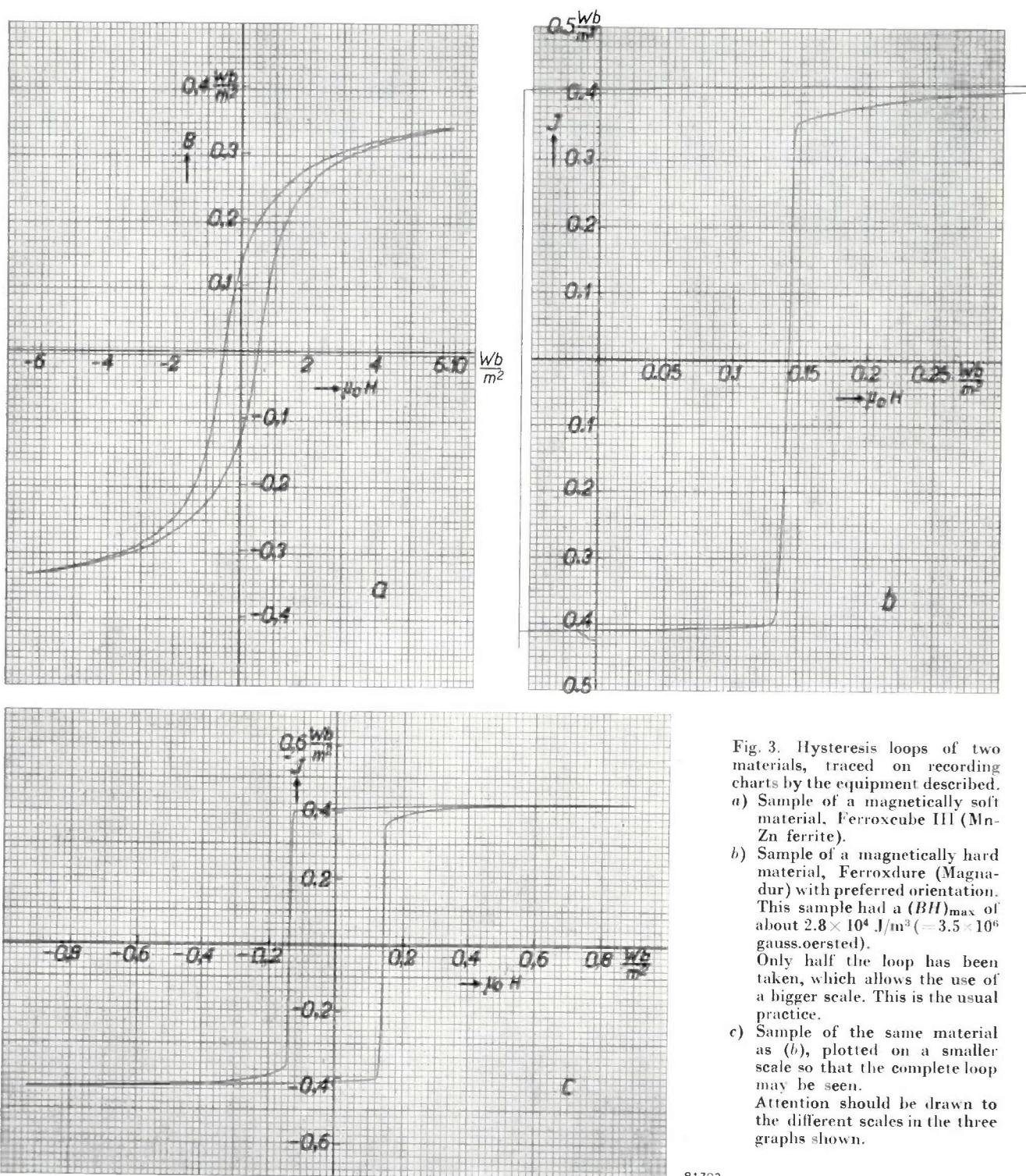
Fig. 3. Hysteresis loops of two materials, traced on recording charts by the equipment described.
