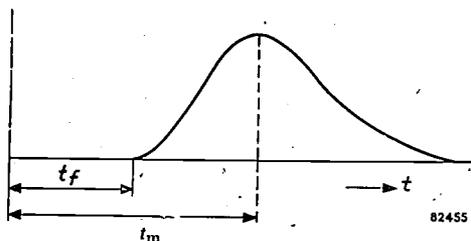
Fig. 2. After the circuit has been closed, a time  $t_f$  elapses before the igniter wire reaches the required temperature (heating time), and a time  $t_m$  before the flash reaches its maximum intensity (time to peak, or time lag).
