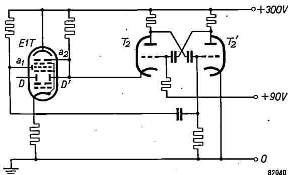
Fig. 8. Diagram showing scaler tube E1T with flip-flop circuit ( $T_2$ - $T_2'$ ) to shorten the reset time. In the steady state  $T_2$  is cut off and  $T_2'$  conductive. This negative pulse produced on the reset anode ( $a_1$ ) when the beam returns from 9 to 0 reverses this situation.
