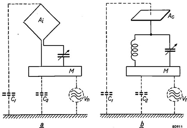
Fig. 2. Schematic representations of (a) receiver with inductive aerial ( $A_i$ ), and (b) receiver with capacitive aerial ( $A_c$ ).  $C_1$  capacitance between aerial and surroundings,  $C_2$  capacitance between chassis and earth,  $V_n$  sources of interference,  $M$  chassis.
