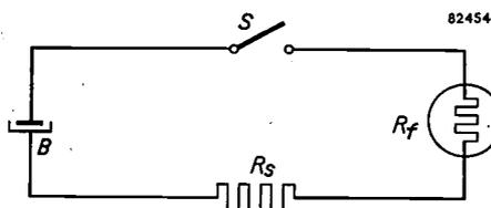
Fig. 1. Ignition of "Photoflux" flash bulb by means of a battery (B).  $R_f$  = resistance of igniter wire in the bulb,  $R_s$  = external resistance in series with bulb, S = switch.
