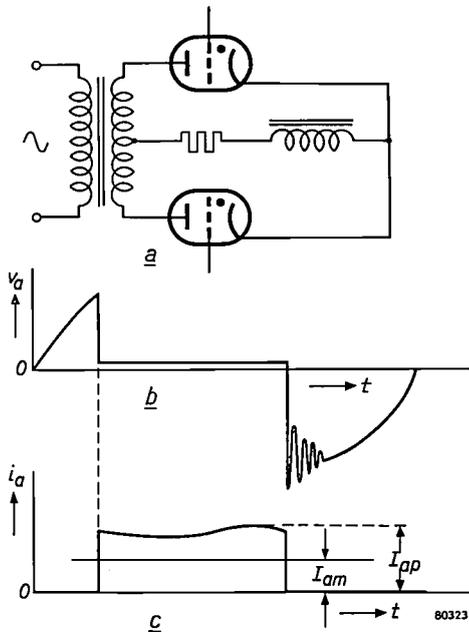
Fig. 6. a) Two thyratrons in full-wave circuit with resistance-inductance load. Both inverse voltage rise (b) and current decay (c) are rapid, but peak-to-mean anode current  $I_{ap}/I_{am}$  hardly exceeds 2, and power consumption is high.
