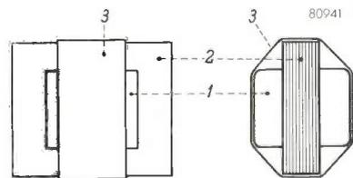
Fig. 6. Mains transformer (1 coil, 2 core) provided with a closed copper loop (3) which prevents the stray field of the transformer from inducing an interference voltage in the frame aerial.
