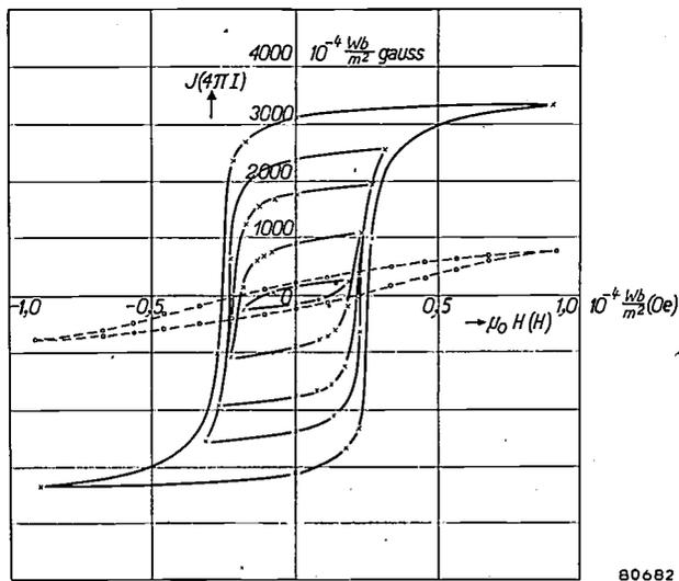
Fig. 4. Family of hysteresis loops for a ring of Ferrocube IVA enclosed by a band of special glass. Dashed curve: hysteresis loop for Ferrocube IVA without glass (see text).
