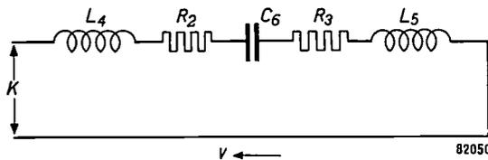
Fig. 2. Electrical analogue of a moving-coil loudspeaker.
