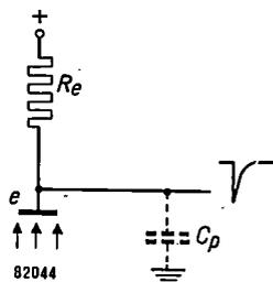
Fig. 13. Each elementary particle striking a particle counter produces an avalanche of electrons on electrode. *e* This, in turn, produces at this electrode a negative voltage step having a steep front and an exponential decay. The time constant of this tail is  $R_e C_p$ , where  $R_e$  is the charging resistance of electrode *e* and  $C_p$  the stray capacitance.
