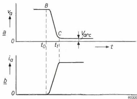
Fig. 2. a) Section BC of *fig. 1*, scaled-up horizontally to show gradual fall of voltage during ionization. b) Corresponding growth of anode current  $i_a$ .
