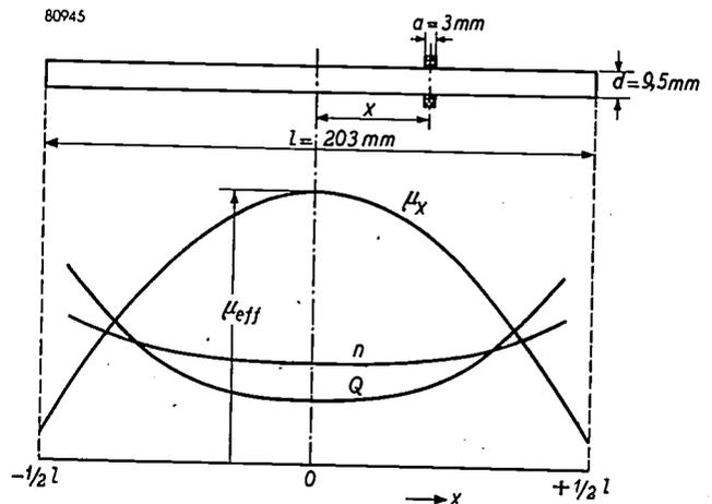
Fig. 19. Above: Ferroxcube rod of length  $l$  with flat coil, placed at a distance  $x$  from the mid-point. The curves represent  $\mu_x$ ,  $Q$  and  $n$  as functions of  $x$ , for a rod of Ferroxcube IV-B of the dimensions shown, wound with a coil of width  $a = 3$  mm and a self-inductance of 200  $\mu H$  at 1 Mc/s.
