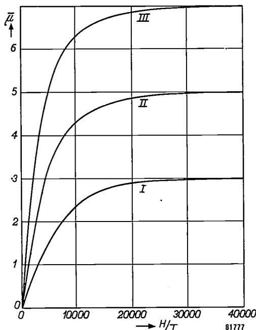
Fig. 2. Average magnetic moment  $\bar{\mu}$  in Bohr magnetons per molecule as functions of  $H/T$  in oersteds per  $^\circ\text{K}$  for (I) sodium-chrome alum ( $s = 3/2$ ), (II) ferric-ammonium alum ( $s = 5/2$ ) and (III) gadolinium sulphate octahydrate ( $s = 7/2$ ). From measurements of C. J. Gorter, W. J. de Haas and J. van den Handel, Proc. Kon. Ned. Akad. Wetensch. 36, 158-167, 1933, and W. G. Henry, Phys. Rev. 88, 559-562, 1952.
