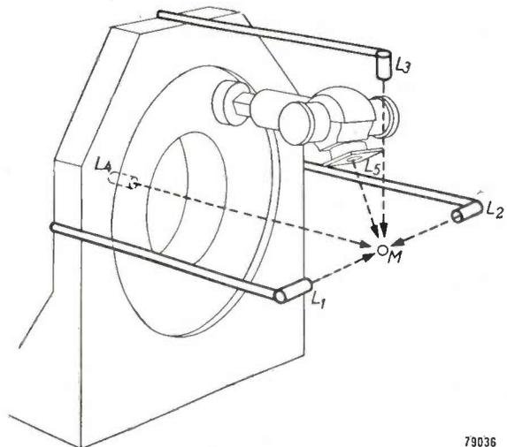
Fig. 10. Method of positioning the patient with the aid of light-beams  $L_1-L_4$ . A light source fitted to the beam aperture of the X-ray tube produces the light beam  $L_5$ , which coincides with the central ray of the X-ray beam subsequently emitted. The lesion (or other specific point in the body of the patient) should be positioned at the point of intersection *M* of all these light beams.
