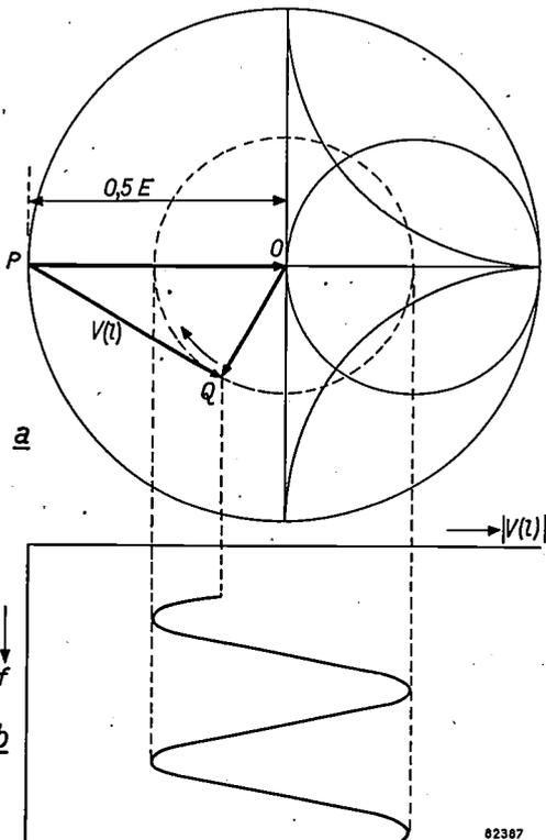
Fig. 6. a)  $V(l) = \frac{1}{2} (1 + r_l) E$  as demonstrated in the Smith chart. When the frequency increases,  $Q$  moves in the clockwise direction around the dotted circle with radius  $\frac{1}{2} |r_l| E$ . b) The modulus of  $V(l)$ , corresponding to line  $PQ$  in (a), plotted against the frequency  $f$ .
