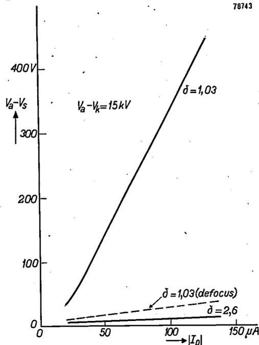
Fig. 16. Potential difference  $V_a - V_s$  as a function of the screen current  $I_p$  (at  $V_a - V_k = 15 \text{ kV}$ ) for screens with  $\delta = 1.03$  and  $2.6$ ; the electron beam is sharply focused. The dotted line represents the corresponding variation for  $\delta = 1.03$  in the case of a defocused electron beam (see note <sup>4</sup>).
