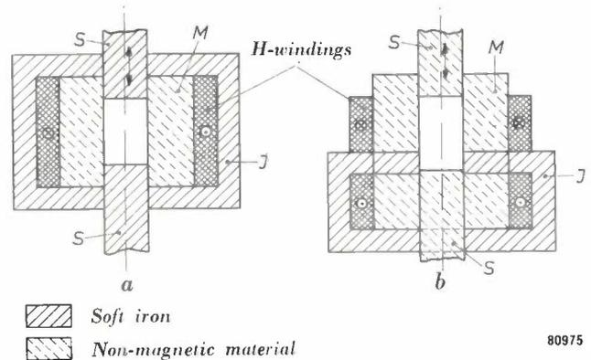
Fig. 3. Diagram of the dies  $M$  used to compress the powder in a magnetic field.  $S$  = plunger.  $J$  = iron yoke.
