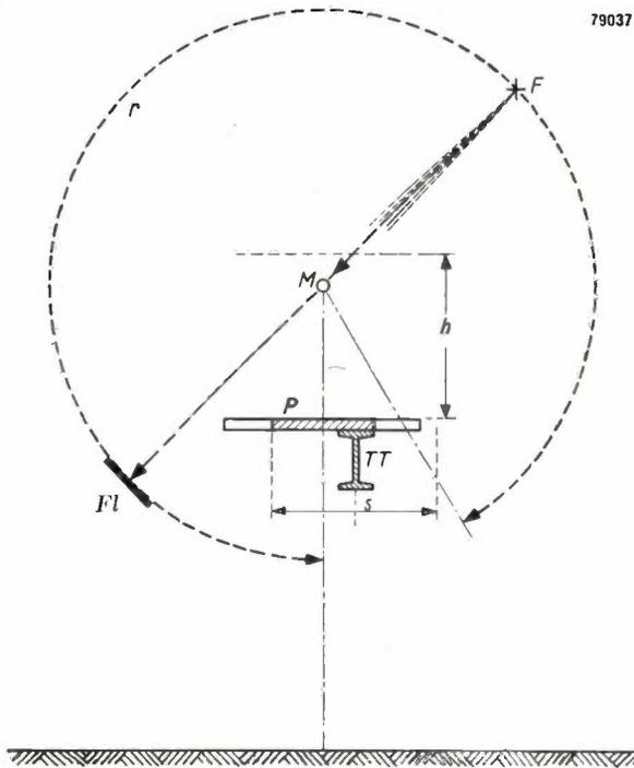
Fig. 11. The top plate *P* of the treatment-table can be moved vertically through a distance *h* and laterally over a distance *s*. *F* is the focus of the X-ray tube and *Fl* the fluorescent screen opposite the tube, with the aid of which the patient can be screen-tested in any position within the angular range *r* of the rotational movement. The iron girder *TT* of the table is placed off-centre to permit the use of the fluorescent screen whilst the X-ray beam is vertical.
