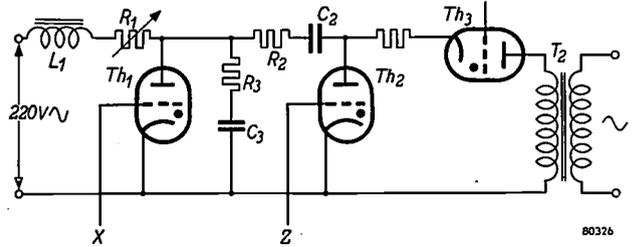
Fig. 9. Cheater circuit as in fig. 7a, but with an RC snubber circuit ( $R_3$ - $C_3$ ), used when commutation factors higher than 80 VA/ $\mu\text{sec}^2$  are required.
