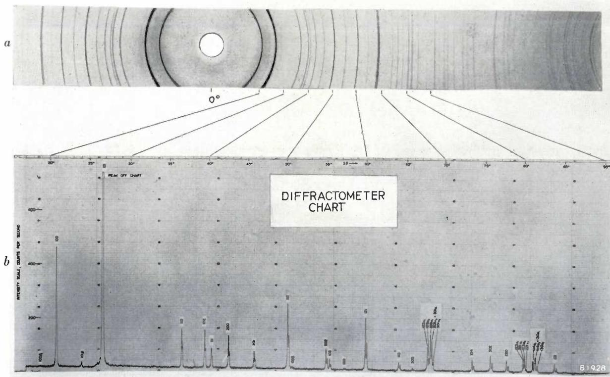
**Fig. 6.** a) X-ray diffraction pattern of quartz powder photographed with a 114.6 mm diameter Debye-Scherrer camera. Filtered CuK $\alpha$  radiation, 40 kV<sub>p</sub>, 20 mA, exposure time 2 hours. b) Automatically recorded chart obtained with the new Norelco X-ray diffractometer using the same X-ray tube conditions. Recording time 4.8 hours.
