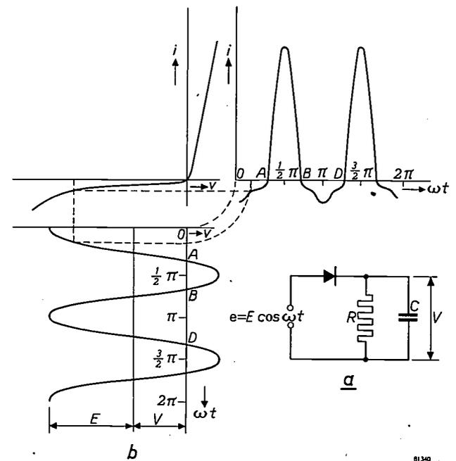
Fig. 4. a) Simple circuit for the detection of amplitude-modulated signals.
