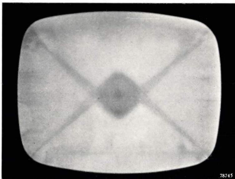
Fig. 2. Photograph of the fluorescent screen of a television picture tube, showing ion burn caused by positive ions.
