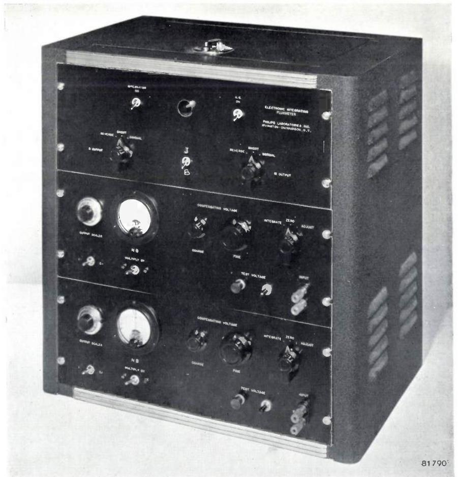
Fig. 2. Front of the instrument for the automatic recording of hysteresis curves, showing two integrator panels (one for  $B$  and one for  $H$ ) and the output control panel (the uppermost one). The instrument is used together with an X-Y recorder of a commercial type.
