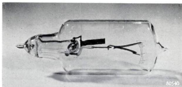
Fig. 3. The electrostatic system of the pocket dosimeter.
