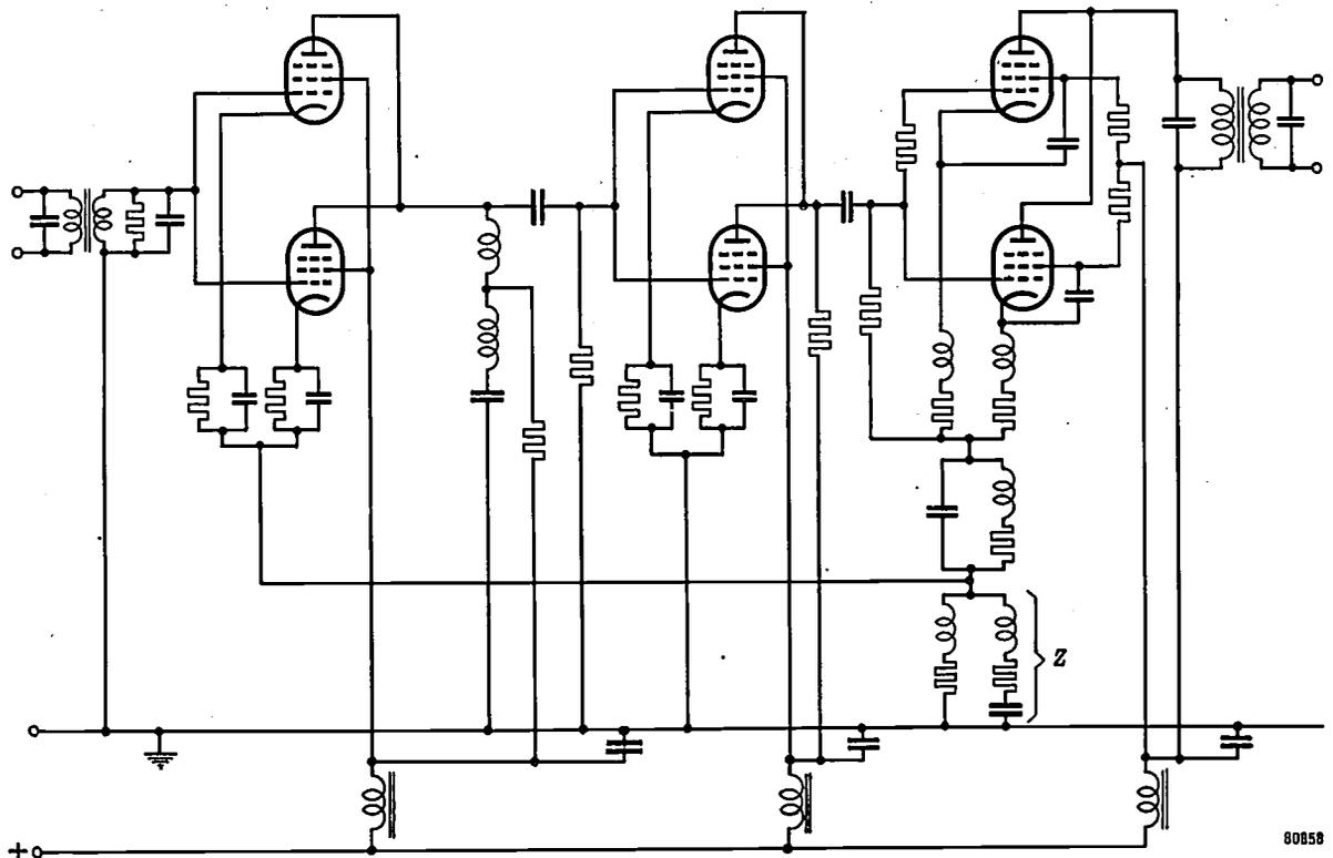
Fig. 8. Simplified diagram of the amplifier for coaxial cables. Current feedback is obtained across the impedance  $Z$ . All tubes work as parallel pairs. The coupling elements are such that approximately 80% of the theoretical maximum value of  $\mu\beta$  can be attained.
