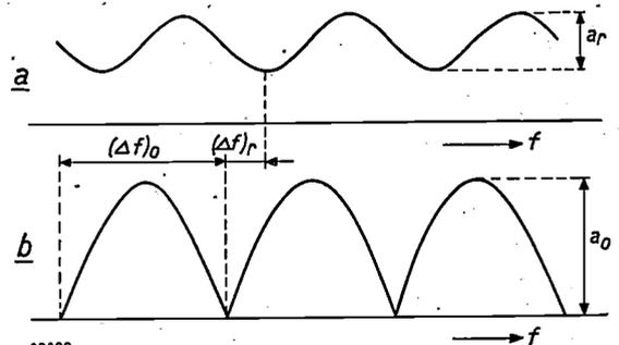
Fig. 9. Oscillograms obtained with the circuit shown in fig. 7, (a) employing an arbitrary terminating impedance. (b) with the end of the test line open. The ratio of the ripple amplitudes ( $a_r$  and  $a_0$ ) is the modulus of the reflection coefficient, and  $2\pi$  times the ratio of the differences in frequency  $(\Delta f)_r$  and  $(\Delta f)_0$  is the argument of this coefficient ( $\varphi$ ).
