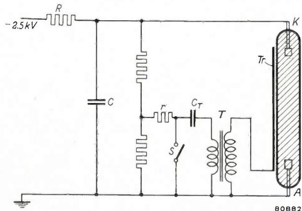
Fig. 3. Basic circuit of a flash tube. *R* charging resistance, *C* main condenser, *C<sub>T</sub>* condenser for trigger pulse, *r* charging resistance for *C<sub>T</sub>*, *S* initiating contact, *T* transformer, *K* cathode. In the usual arrangement (as shown here), the anode *A* is earthed and the trigger electrode *Tr* is held at the same potential. The trigger pulse is then a positive surge.
