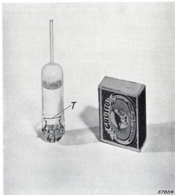
Fig. 3. Hypsometer. This is made from a radio-valve bulb containing freon, the boiling-point of which is measured by means of an N.T.C. resistor  $T$  secured to two lead-in pins in the bulb and completely immersed in the liquid; the latter has access to the outer air through a tube (the exhaust stem) at the top of the bulb.
