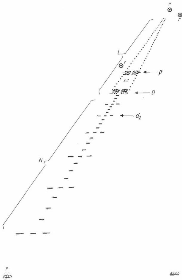
*Fig. 3.* Diagram showing approach lighting (*N*), threshold lights (*D*) and runway-marking (*L*) of runway 23 at Schiphol. *d*<sub>1</sub> is a special cross-bar in the approach lighting system coloured differently from the others (red), the so-called warning sign, and *p* is the so-called touch-down point, specially marked with paint and a number of lights, located 1000 ft beyond the threshold; *r* indicates the various radio beacons associated with the particular landing system.
