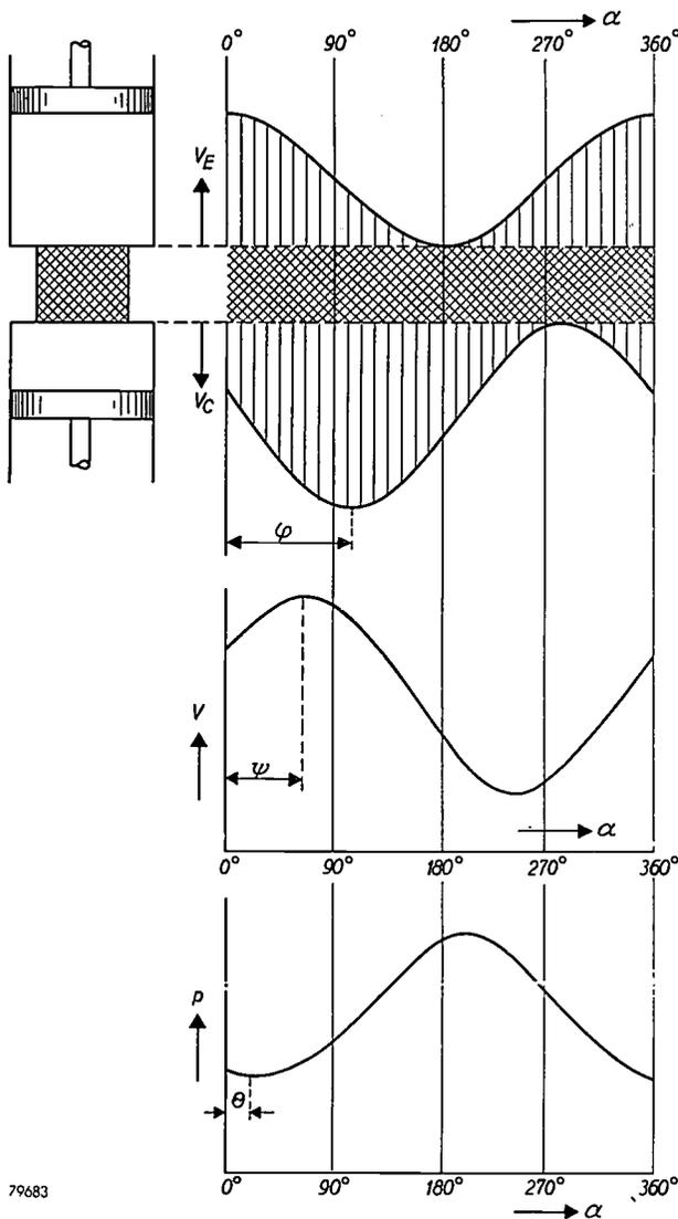
Fig. 9. The variation of the volumes  $V_E$  and  $V_C$ , of the total volume  $V$  ("working space"), and of the pressure  $p$  of the refrigerating machine as functions of the crank angle  $\alpha$ . The phase relationships are clearly seen; the pressure variation is almost sinusoidal.
