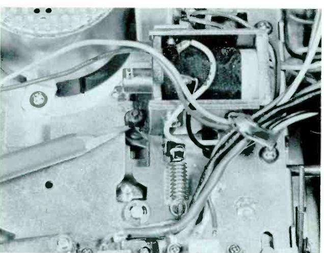
**Step 10.** As the mechanism tray swings to the rear, a rubber-rimmed idler wheel presses against takeup spindle and flywheel (or capstan wheel, in some units). A spring near the wheel, under the baseplate, maintains this contact. Naturally, if the spring is weak or has been knocked loose, tape takeup becomes erratic. The same symptom might result if the idler lever twists.
