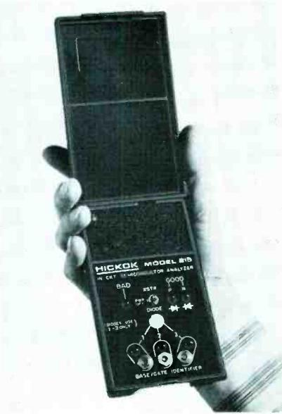
The tester reportedly determines proper lead configuration instantly and automatically, and indicates in bright LED displays if the semiconductor is good or bad. If good, the model further identifies which lead is the base, and whether it's NPN or PNP.
