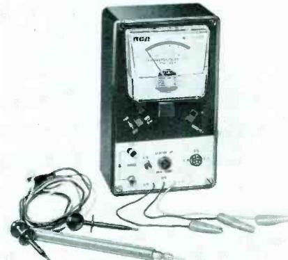
One extended range for all tests is possible with a special "square-law" meter. Relative gain readings are indicated on a good/bad color-coded scale.
