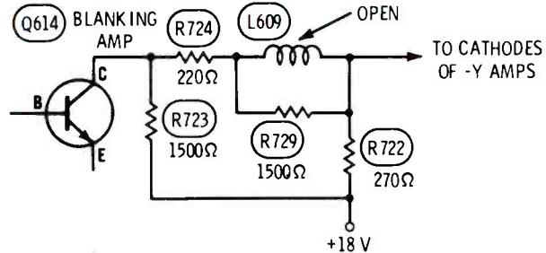
**Symptom**—Insufficient brightness; poor gray-scale tracking
