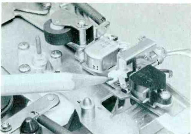
**Step 5.** A slightly-different automatic-shutoff system mounts on this head plate. The shutoff actuator is part of a switch. It presses against the moving tape, which has some slack. At the end of the cassette, tape tension increases and pushes the actuator back, closing the switch. That de-energizes a relay, cutting off AC power to the motor. However, in this automatic shutoff setup, all playback assemblies stay put until you move the function knob.
