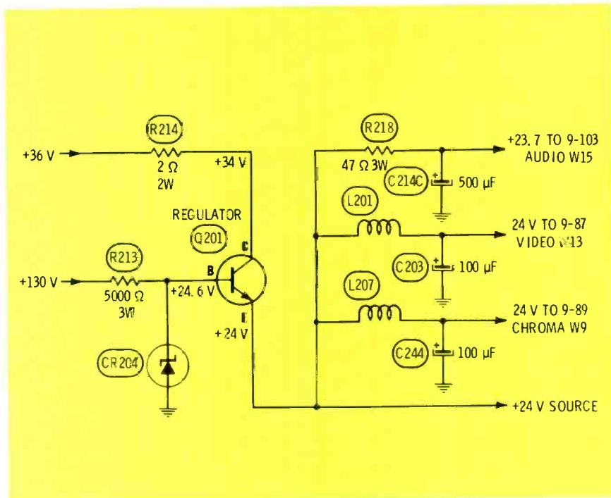
Fig. 7 The collector/emitter resistance of Q201 is used as a variable series resistance to regulate the 24-volt supply. Base voltage is clamped by the zener diode, CR204, so the emitter voltage determines the forward bias. Notice the many circuits powered from this source.
