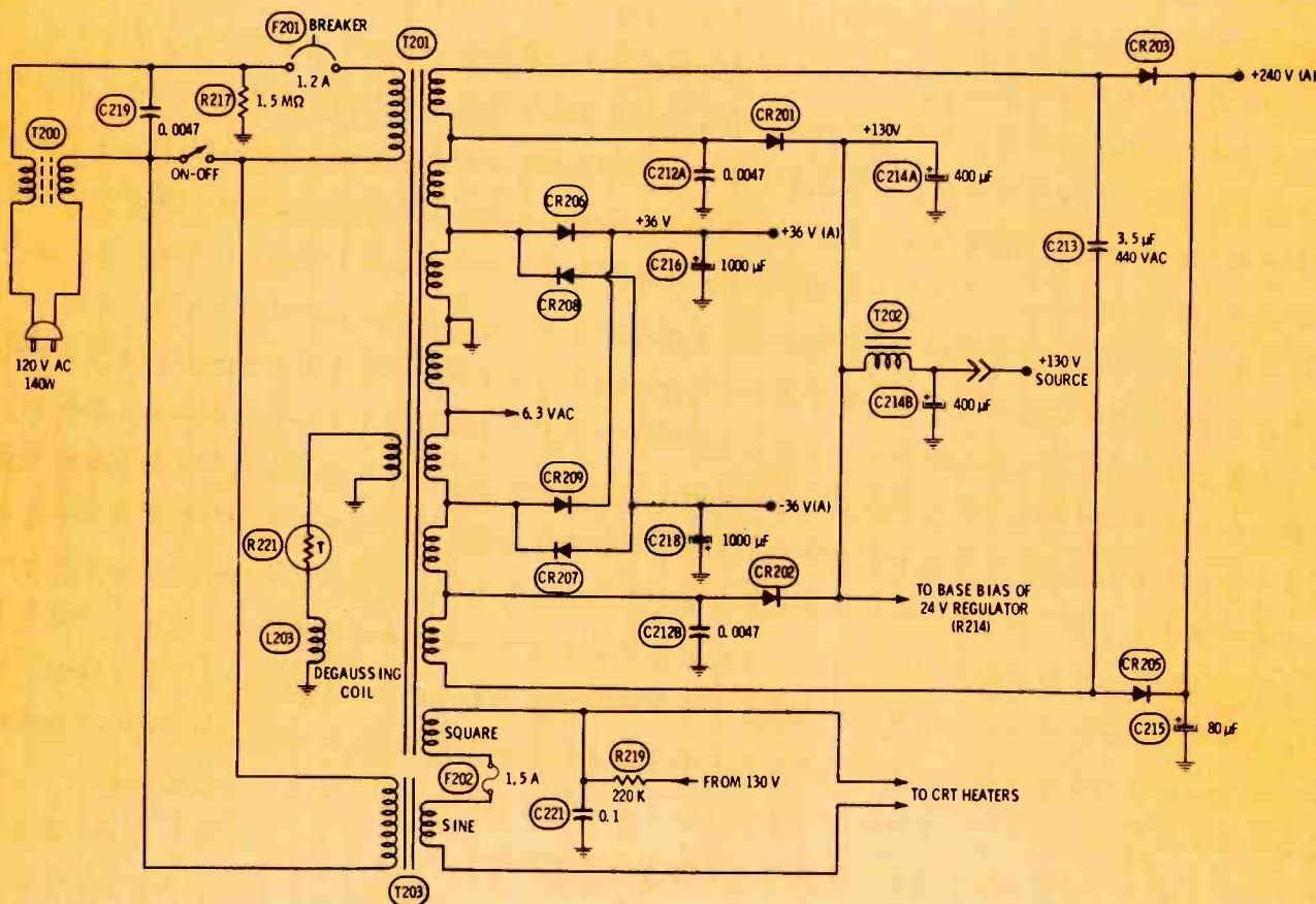
Fig. 5 This complete schematic of the power supply (less the 24-volt regulator) shows the unique CRT heater wiring, and the four rectifier circuits using eight diodes.
