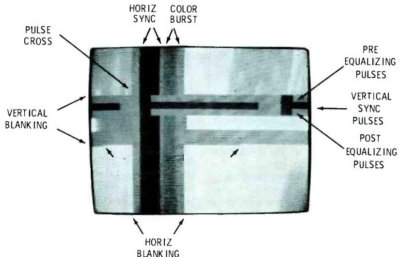
**Fig. 11** Important parts of the pulse-cross display are marked on this photograph taken from a Tektronix Model 650 Video Monitor. Unmarked arrows show half-lines of video. Interlace is proven by all 18 lines in the hammer. Vertical blanking occupies 42 lines. In the monitor, sync pulses are shifted in phase to permit a stable display of the sync areas normally blanked out and not seen on receiver screens.
