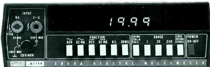
Resolution is 100 microvolts, 100 nanoamps and 100 milliohms
