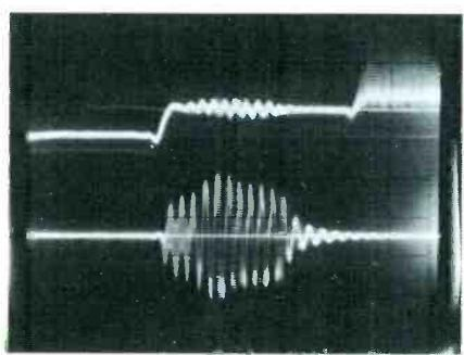
**Fig. 4** The horizontal width variable EXPANDER can be used to spread out any portion of a waveform. For example, the dual-trace waveforms of the picture at the top showing video and color burst signals can be widened (bottom picture) enough to permit counting each cycle of the burst. It's likely the parts of the waveform not shown are compressed. But that's not important, for the sections you can see are very linear.
