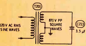
Fig. 4 Power transformer, T201, is built with loose coupling between primary and secondary windings, and arranged so the core around the primary does not saturate, but the core around the secondary does. Therefore, the secondary waveform is a clipped sine wave, or roughly a square wave, that varies little in amplitude with different primary voltages. C213 rounds the edges of the square wave and increases the p-p voltage.
