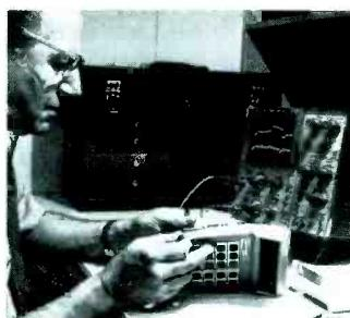
loscope. (Ask for the D67 article reprint, *Another Step Forward*.) Its sister scope, the D66, offers all features but delayed sweep at an even lower price. Both feature a SUM mode with normal/invert capability that improves visibility of small signals in the presence of common mode noise.
