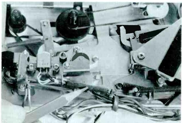
**Step 4.** The pinch roller also mounts on the head plate in this kind of machine. Rotating the function knob to Play presses it against the capstan. Symptoms of too much or too little pinch-roller pressure were explained in Session 3, Step 7. The cure, on this particular machine, is a new tension spring (you can't adjust pinch-roller pressure).
