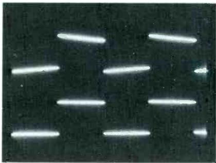
**Fig. 1** Top waveform shows the small amount of tilt produced by AC operation of the vertical amplifier with 20 Hz square waves. The bottom trace was made under the same conditions, except the coupling was DC.
