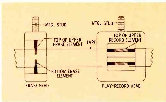
Fig. 11 Proper head height location.
