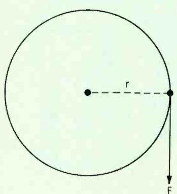
**Fig. 6** Illustration of twisting force called torque.
