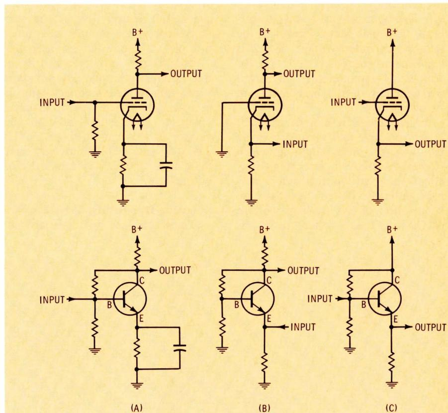
**Fig. 1** Basic tube and transistor configurations. A.) Common cathode and common emitter. B.) Grounded grid and common base. C.) Cathode follower and emitter follower.
