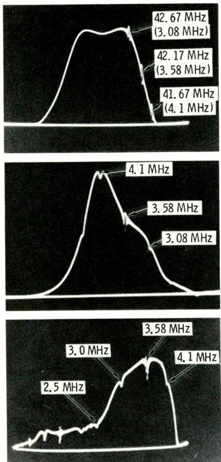
**Fig. 5** Adding the color-carrier side of the IF curve (A) to the overall chroma IF curve (B) produces the VSM curve (C) at the chroma demodulators.
