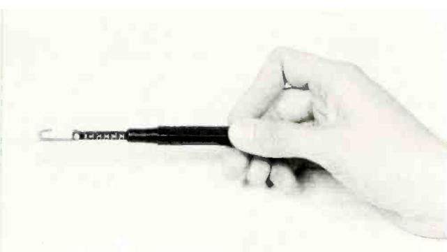
**Fig. 5** A spring scale, which measures forces up to 8 ounces, for making torque and pressure measurements.
