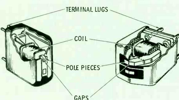
Fig. 10 Detail of typical erase (A) and record (B) heads.
