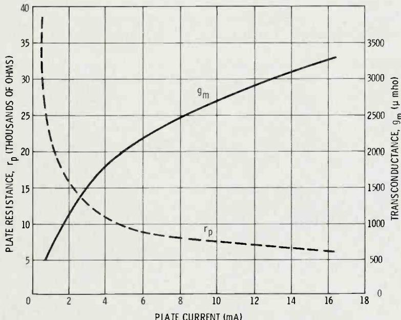
Fig. 9 Triode transconductance and plate resistance versus plate current.
