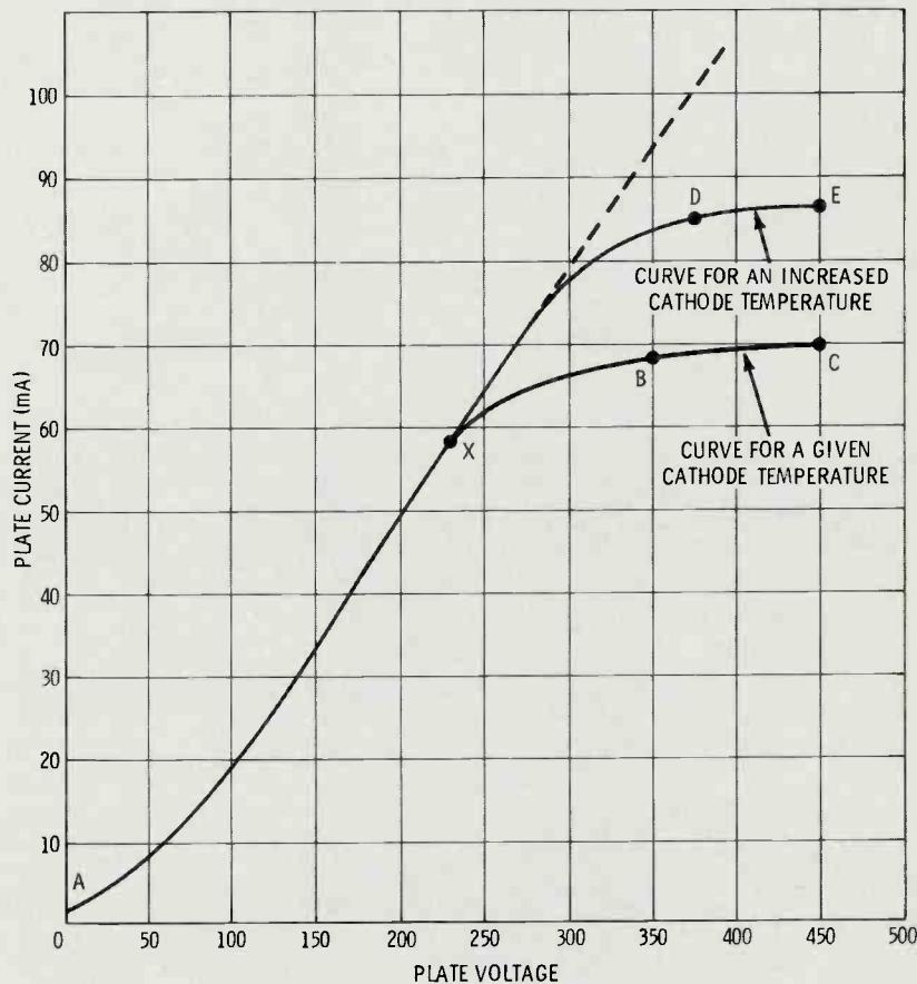
**Fig. 6** Plate-current plate-voltage characteristic curves.
