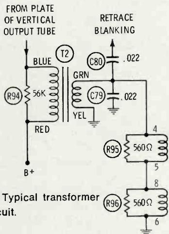
(b) Typical transformer circuit.
