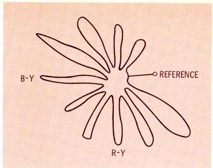
**Fig. 6** When cathodes of CRT are driven, phase of the vectorgram is rotated 180 degrees.
