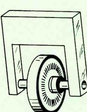
**Fig. 7** A typical tape strobe for measuring speed.
