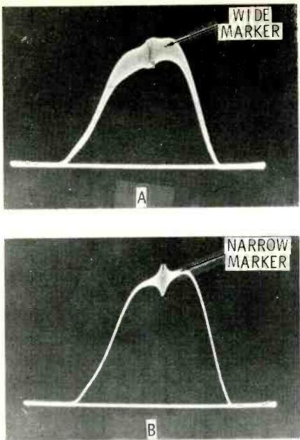
**Fig. 2** Photos illustrating the advantage of using a low-pass filter between the probe and the input of the scope. (Probes shown in Fig. 1 have a built-in low-pass filter.) A.) Curve produced using a probe without a low-pass filter—the marker covers the whole curve. B.) Curve produced using a low-pass filter in the probe—marker is much sharper.
