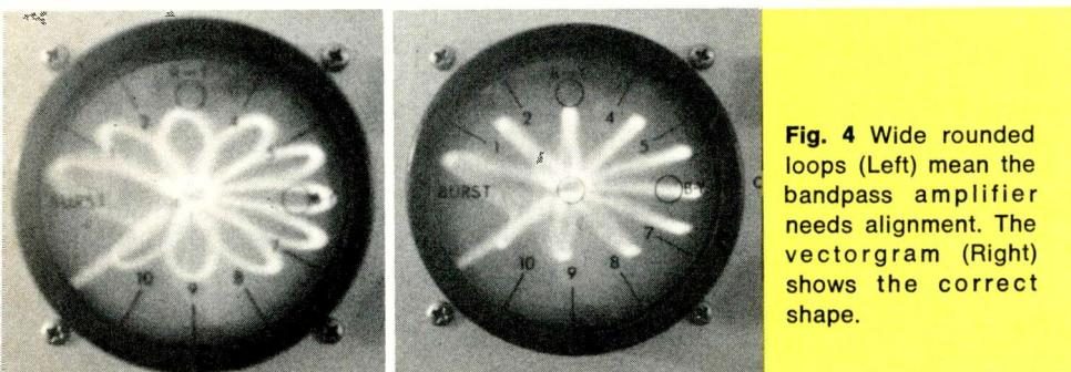
Fig. 4 Wide rounded loops (Left) mean the bandpass amplifier needs alignment. The vectorgram (Right) shows the correct shape.
