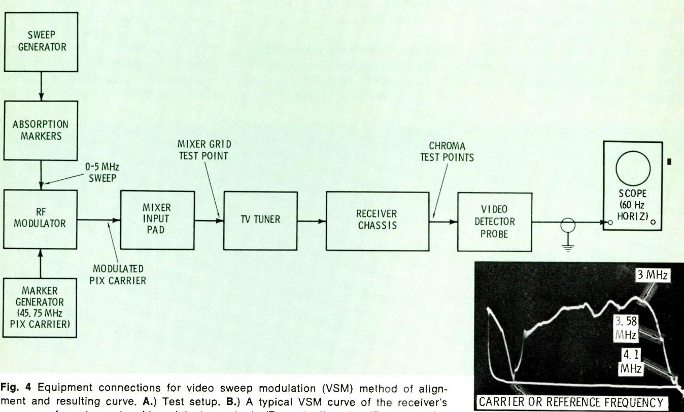
**Fig. 4** Equipment connections for video sweep modulation (VSM) method of alignment and resulting curve. **A.)** Test setup. **B.)** A typical VSM curve of the receiver's response from tuner to video detector output. (Do **not** align the IF's using this curve.)
