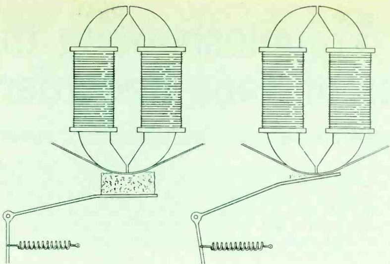
**Fig. 4** New pressure pad compared to worn pad.
