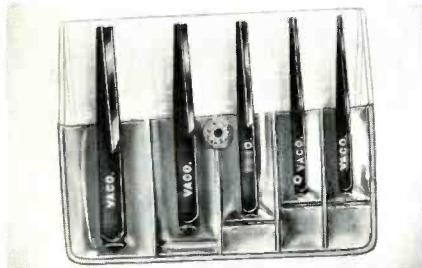
or buried stud, pounding in the correct size extractor which has special ground flutes for gripping, then unscrewing with a plier or wrench. The set, Vaco Kit No. 70007, handles all screw sizes from  $\frac{1}{4}$  inch to  $\frac{5}{8}$  inch and costs \$6.50.
