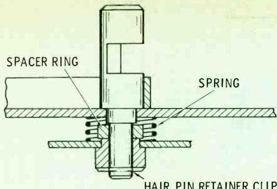
Fig. 8 A tape guide with a stop control pin assembly.
