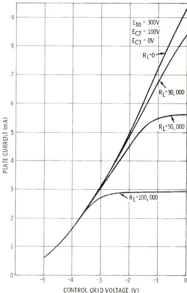
**Fig. 8** Overload characteristics for a pentode.
