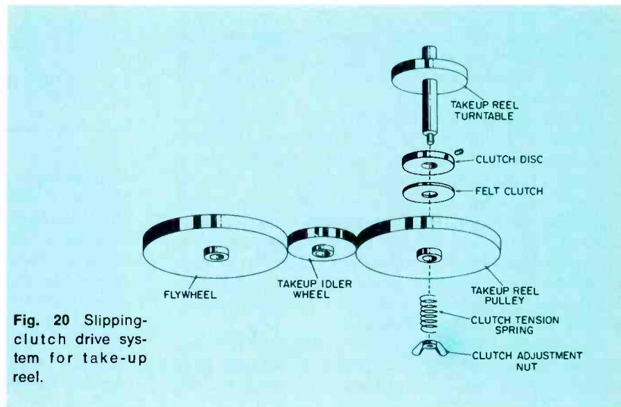
**Fig. 20** Slipping-clutch drive system for take-up reel.
