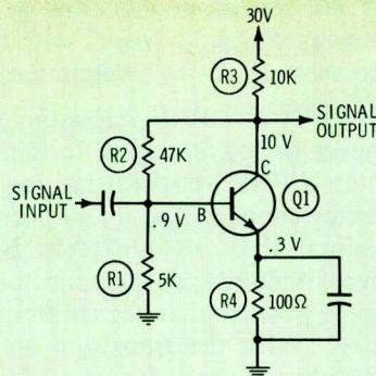
**Fig. 3** Example of a transistorized amplifier.
