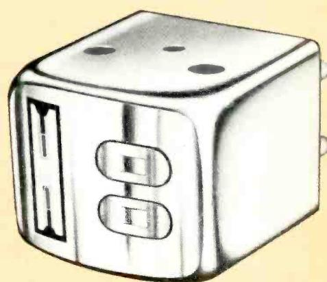
Fig. 3 Modern stereo recording head.
