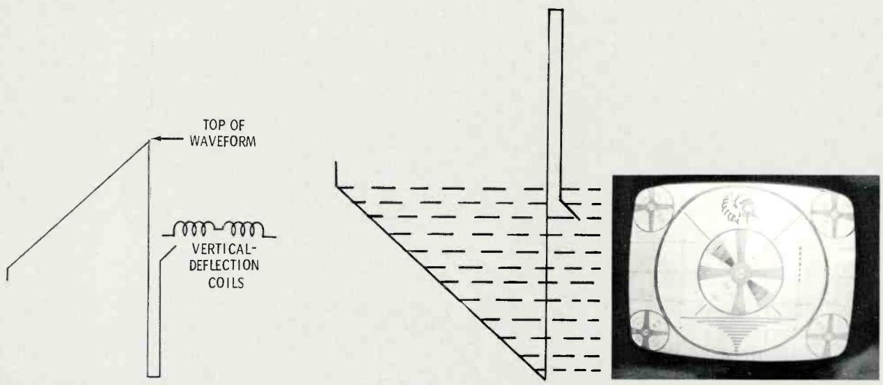
**Fig. 7(a)** Vertical-output waveform applied across yoke.
