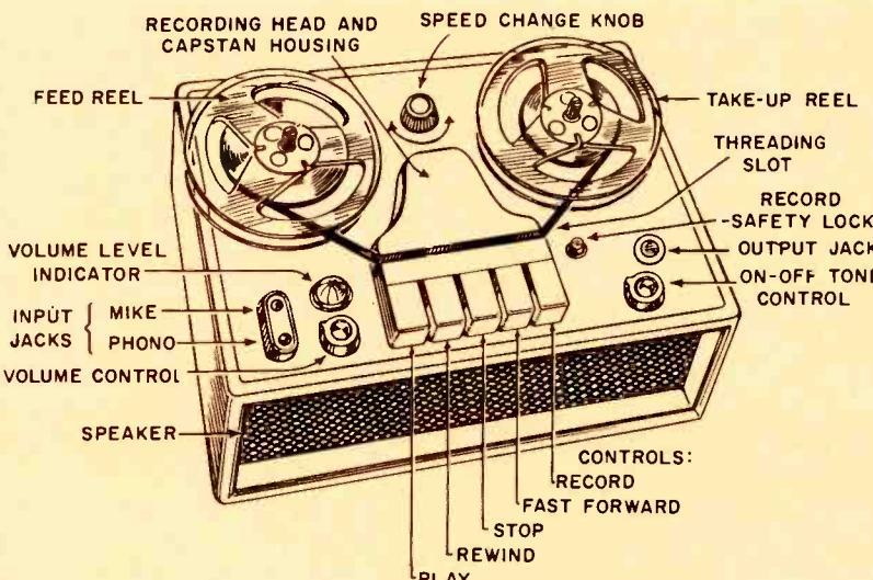
Fig. 1 Typical two-speed recorder with principal features indicated.
