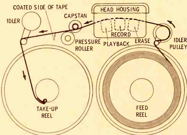
Fig. 2 Top view of a motorboard showing major components.
