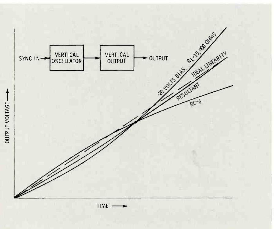
Fig. 4 Resultant of exponential waveform, linearized (approximately) by a dynamic transfer waveform.
