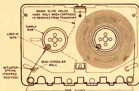
Fig. 13 Design of conventional tape cartridge.
