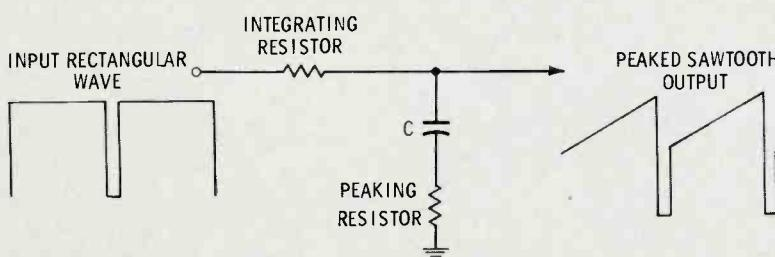
Fig. 10 Resistance-type peaking circuit.
