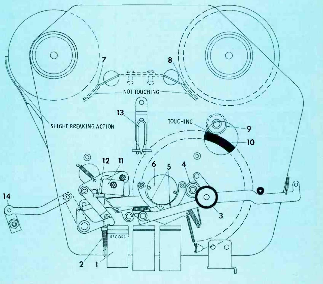
**Fig. 21** Top view of tape transport mechanism in "Record" position (3 3/4 in./sec.).
