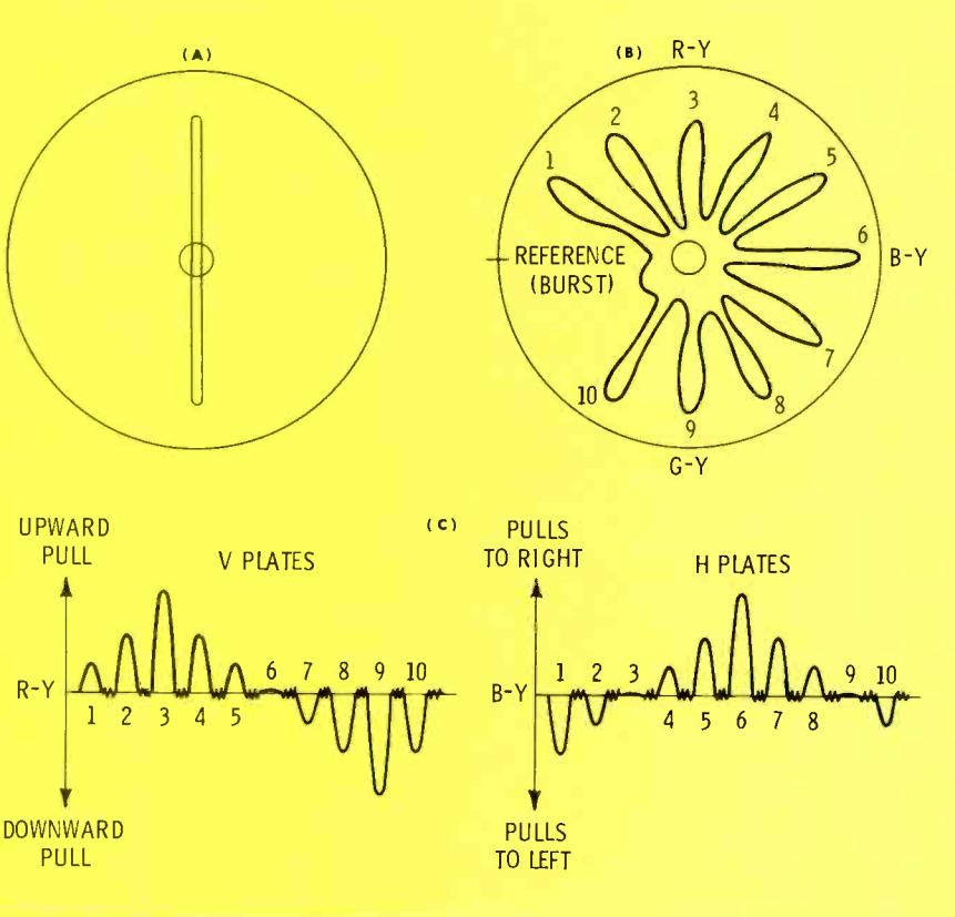
Fig. 2. How vectorogram is formed on vectorscope CRT. (A) R-Y connected to vertical deflection plates. (B) B-Y connected to horizontal deflection plates matrixes with R-Y to form "starburst" or "daisy" display. (C) The two signals as you'd see them on an ordinary wideband servicing scope; they combine in vectorscope to form the display.
