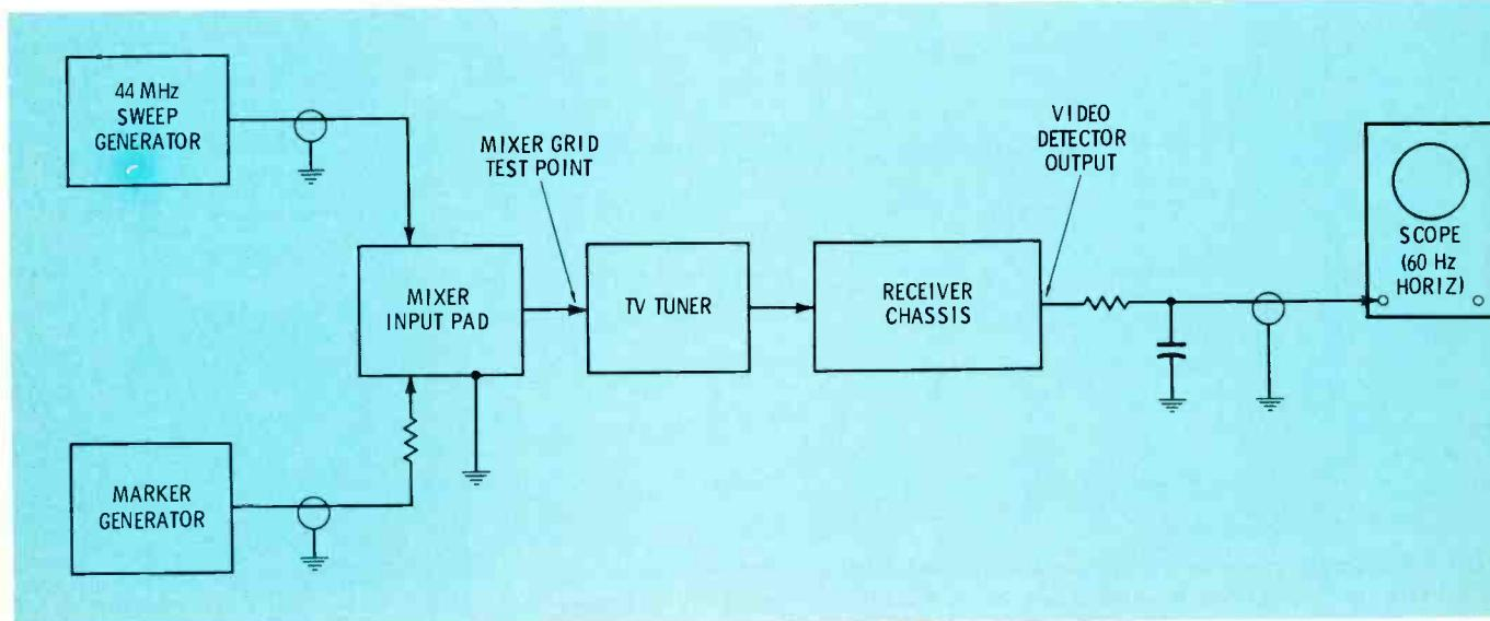
**Fig. 3** Equipment connections for IF-sweep curve alignment.
