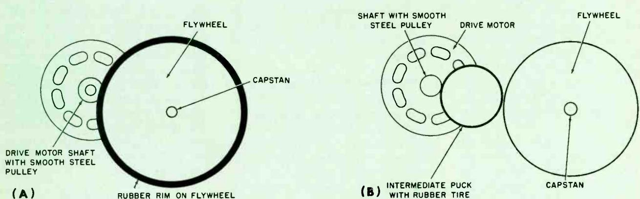
Fig. 16 Two methods of capstan drive. (A) Rim drive to flywheel. (B) Intermediate-puck drive.
