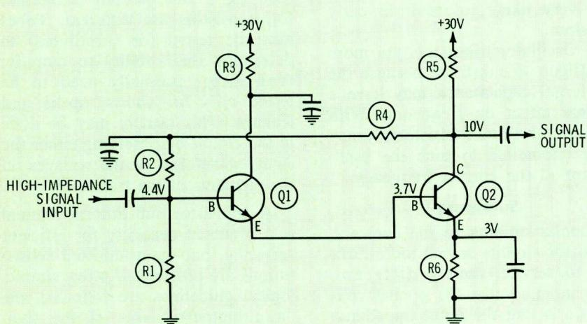
**Fig. 4** Two-stage amplifier with feed-back bias stabilization.
