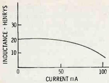
Fig. 11(a) Magnetizing inductance of vertical-output transformer versus current.
