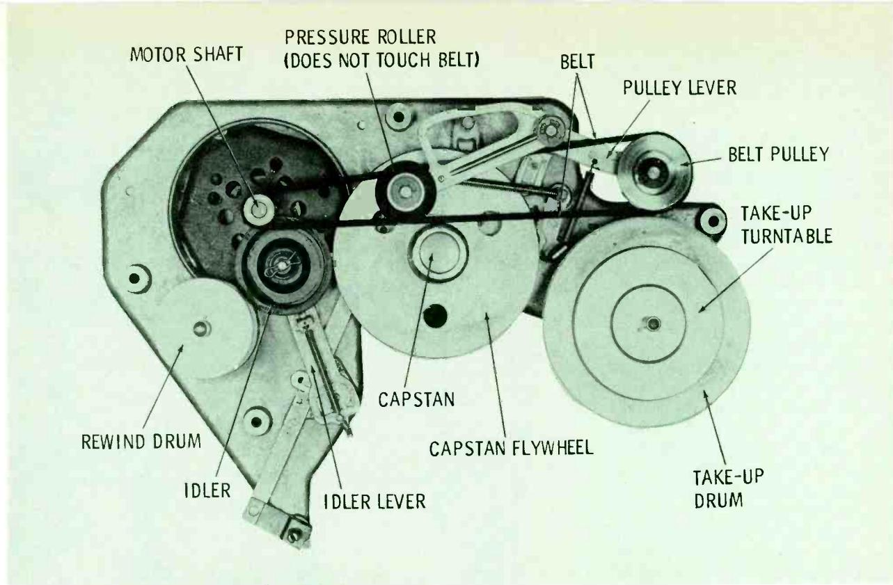
Fig. 15 Transport mechanism of a conventional tape recorder.
