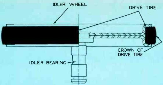
**Fig. 17** Details of an intermediate-puck wheel.
