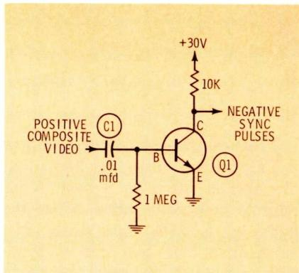
Fig. 5 A simplified sync separator.
