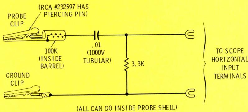
Fig. 3 Homemade probe for adapting any servicing scope to vectorscope servicing.
