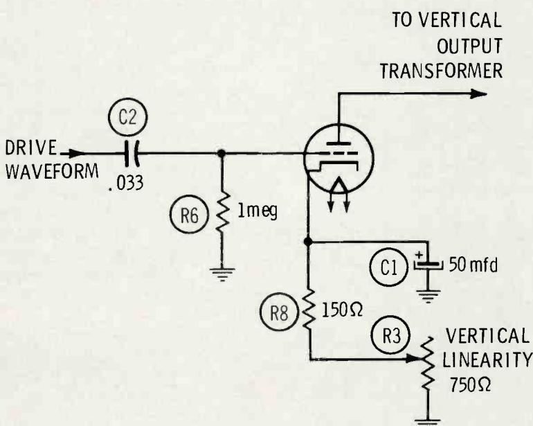
Fig. 12 Capacitors  $C_1$  and  $C_2$  affect vertical linearity.
