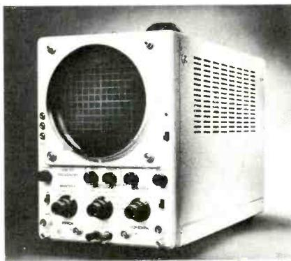
is designed for educational, laboratory and servicing applications. It is capable of accurate phase comparison and measurement involving Lissajou functions and differential
