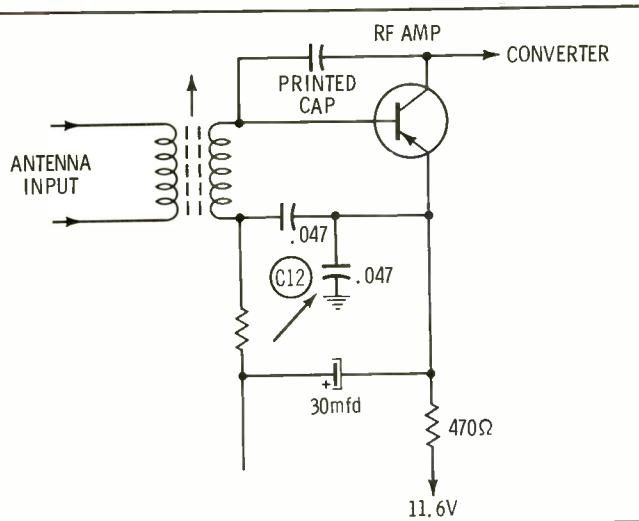
a defect in it was not directly responsible for the varying collector voltage. I then measured the emitter voltage; it was varying from 11 volts to less than 7 volts. I checked the voltage across the emitter resistor; it was varying from approximately .4 volt to over 5 volts. Again, the noise disappeared and the radio returned to normal operation.
