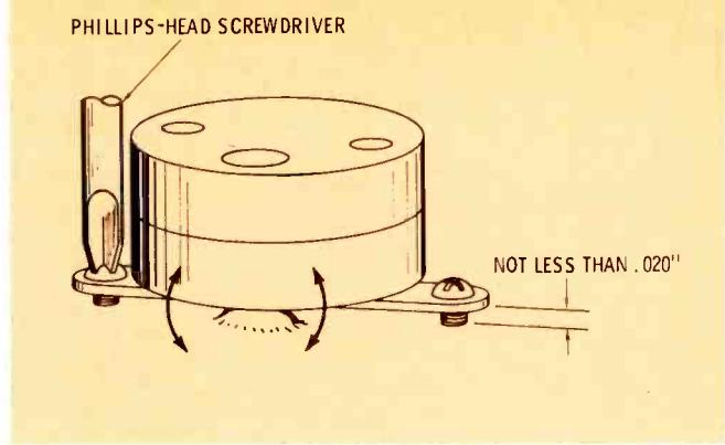
Fig. 12 Typical azimuth-adjusting screws.
