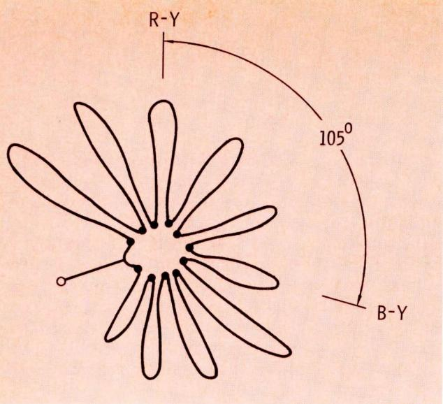
**Fig. 5** This leaning, elliptical vectorgram is the pattern formed from 105-degree demodulator.
