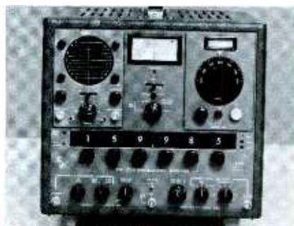
Included is a "dial-in" feature that allows users to "dial-in" any frequency in the FM communications spectrum. Once the frequency is selected, frequency error and FM deviation can be read simultaneously. The whole process takes less than 10 seconds. Frequency accuracy is better than .000075% long term.
